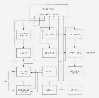
Fig. 3. Block diagram showing the functional arrangement of and linkage between the modules.
