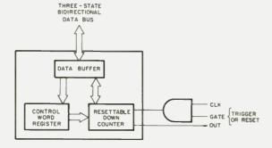
Fig. 2. Functional diagram of each of the three 16-bit interval timers in the 8253 chip. The gate input acts alternatively as a gate, trigger, or reset input, depending upon the mode chosen.
