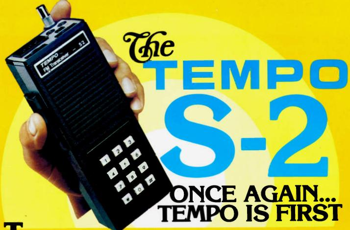
his time with a superior quality synthesized 220 MHz hand held transceiver. With an S-2 in your car or pocket you can use any 220 MHz repeater in the United States, It offers all of the advanced engineering, premium quality components and exciting features of the S-1. It is completely synthesized, offering 1000 channels in an extremely lightweight but rugged case.
