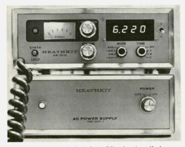
HW-2036 with digital modification installed.
