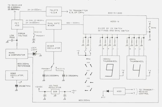
Fig. 2. 2m synthesizer block diagram.
