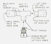
Fig. 1. Details of center insulator.
