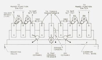
Fig. 5. Wiring diagram, nine-lug terminal strip.
