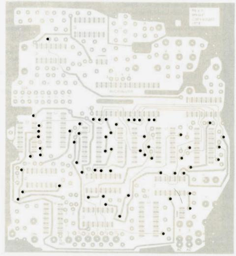
Fig. 7. "Z"-wire placement, along with method of installation.
