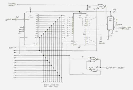
Fig. 2. Schematic diagram of the decoder section of the complete control system. In this and the following schematics, the arrowheads indicate connections contained on the printed circuit board, while circles indicate those lines which go off the circuit board. The \* is available but not used.
