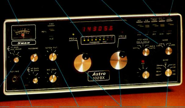
Variable AGC Decay Continuously variable to suit your preference. Passband Tuning with 16 Pole Filters
