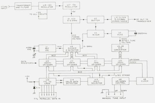
Fig. 1. Block diagram of the MICROSIZER. All parallel data bits are normally high between data words for at least 1 µs. Valid data should be held for a minimum of 4 µs. All digit values are BCD. Digit selector: 100 Hz = 00; 1 kHz = 10; 10 kHz = 01; 100 kHz = 0111.
