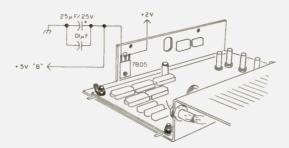
Fig. 5. +5-volt "B" supply regulator location inside transmitter area.
