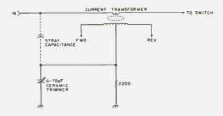
Fig. 3. Capacitive voltage divider with current transformer.
