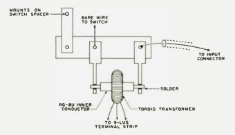
Fig. 4. Mounting the current transformer.
