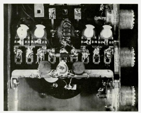
Photo C. A closeup view of nine-lug terminal strip and current transformer. The input SO-239 connector is on the lower right.
