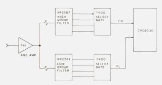
Fig. 3. Block diagram of the DTMFR.
