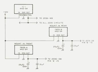
Fig. 3. 7805 voltage regulator schematic.
