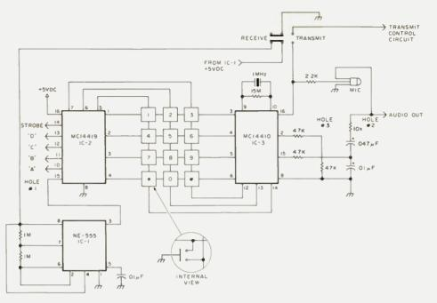
Fig. 2. 2036-MB MicBoard schematic.
