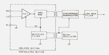
Fig. 2. Block diagram of an isolated ECG preamplifier.
