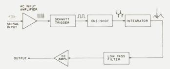
Fig. 4. Block diagram of a pulse-counting FM detector.
