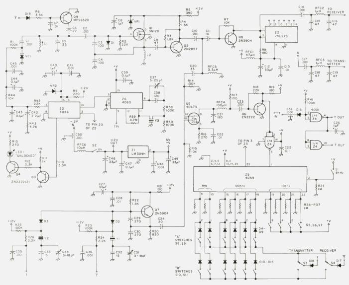
Fig. 1. 2m synthesizer schematic diagram.
