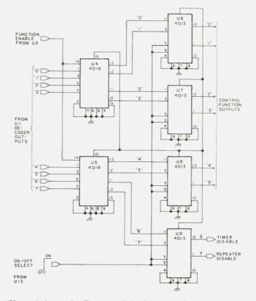
Fig. 3. Schematic diagram of the function decoder section of the control decoder. The control functions 0 through 5 go off the board for whatever auxiliary use may be needed.
