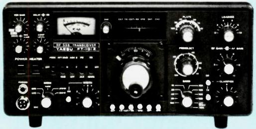
If economy is an important consideration, and you don't need the frequency counter and digital display, then choose the FT-101Z. The precision VFO gear mechanism is coupled to an easy-to-read analog display, providing resolution to greater than 1 kHz. All other features—the variable IF
