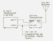
Fig. 1. Transverter connections.
