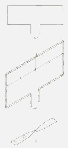
Fig. 1. (a) Schematic of Mobius-twist<sup>TM</sup>, folded dipole, hanger-hung receive system. (b) Isometric presentation showing the location of the twist, with  $Z_1:Z::Y_1:Y$  (see equation in text). (c) Detail of the twist.
