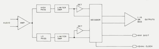
Fig. 1. Simplified block diagram of the Telenetics 7516 tone decoder. We obtained these and the address selectors direct from Telenetics, Inc, 4120 Birch St., Newport Beach CA 92660.
