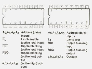
Fig. 8. Seven-segment decoder/drivers. Either device may be used, although 2k pull-up resistors will be needed with the SN74LS48s.
