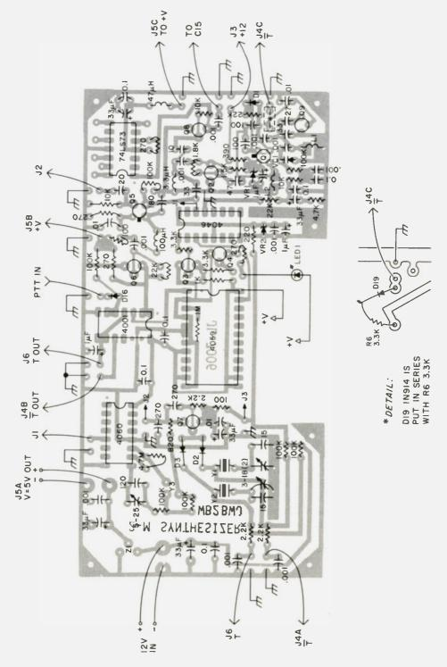
Fig. 4. Component placement.
