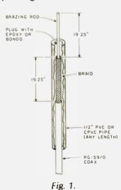
to enlarge the diameter to about twice its normal size (but don't unravel the braid). Now, work the braid down over the top of the outer covering of the coax. so that the braid is folded back over itself over the outer covering. When it is all smoothed down, trim the length of the braid to one-quarter wavelength for the frequency you want (19.25 inches for 146 MHz). Tie or tape the braid in place.
