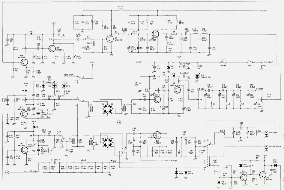
Fig. 3. Shielding beads are indicated by FB. Unless otherwise specified, resistors are in Ohms, capacitors in picofarads, and inductors in microhenrys.
