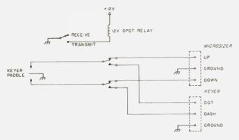
Fig. 8. Method for switching the keyer paddle between MICROSIZER tuning and keyer operation.
