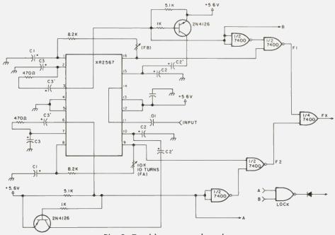
Fig. 2. Dual-loop tone decoder.
