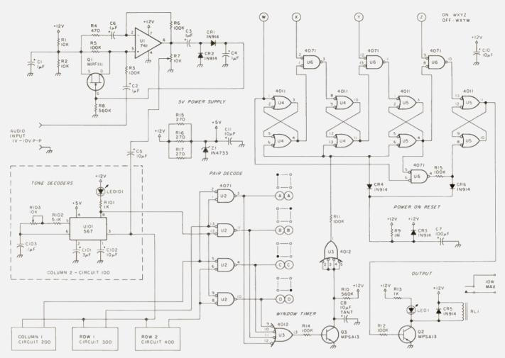
Fig. 1. Schematic of remote-control decoder. All resistors ¼ W, 5% unless otherwise stated. On all ICs, connect pin 14 to +12 volts and pin 7 to ground unless otherwise stated. Circuits 100, 200, 300, and 400 are identical except that part 101 becomes 201, etc.
