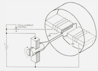
Fig. 1. Simple dc shunt motor with field-current rheostat for speed control. An elementary setup, to be sure, but which way should R be adjusted to increase motor speed?
