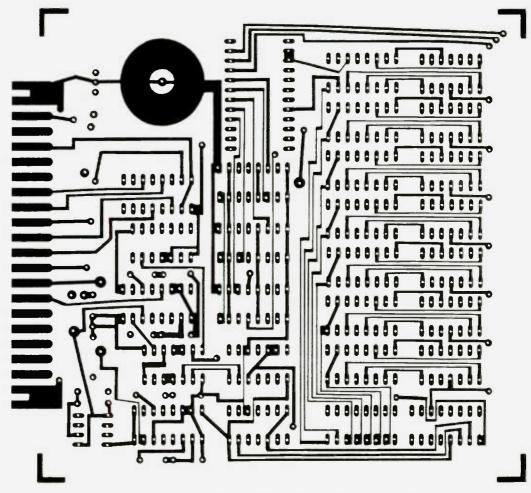
Fig. 4(b). Printed circuit board layout, bottom side.
