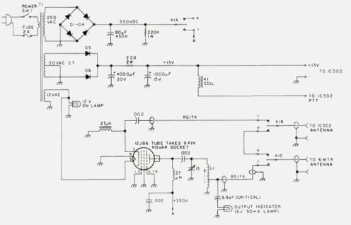
Fig. 1. Circuit diagram. T1 — vibrator/ac power transformer from 12 V CB tube radio with 250 V ac, 20 V ac c-t, and 12 V ac secondaries. K1 — 3PDT miniature relay with 12 V dc coil. D1-4 — 1000 piv 1-Amp diodes. D5, 6 — 50 piv 3-Amp diodes. L1 — 8 turns #20 on 3/8" slug form tapped 1 1/2 to 3 turns from ground end (adjust for max output).
