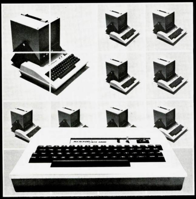
Truly a new dimension in digital communications, the ATR-6800 is more than a superb CW and RTTY machine. It includes a user programmable microprocessor designed to fully automate your station.
