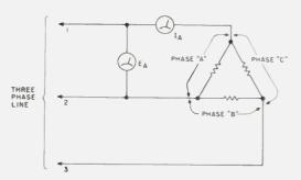
Fig. 2. A three-phase balanced load with a voltmeter and ammeter in one phase. A little common sense suggests that the total power consumed by the delta-connected load is 3 x  $E_A$  x  $I_A$ . A more adequate dose of common sense refutes this simplistic solution!
