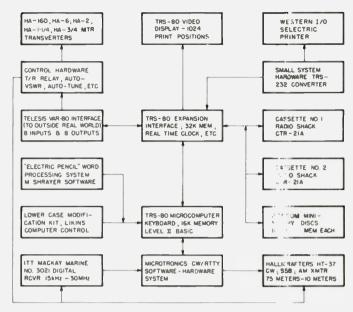
Fig. 1. Block diagram of a TRS-80 microcomputer-controlled ham station.
