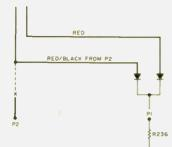
Fig. 7. Adding diodes for conversion of LSB to USB.
