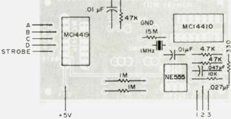
Revised Fig. 10, "An LED Display for the HW-2036."
