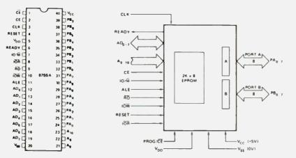
Fig. 1. Block diagram and pin configuration for the 8755 read-only memory used in 8085-based systems.
