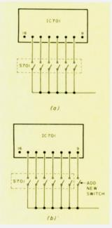
Fig. 5. 640-kHz jump modification: (a) before; (b) after.
