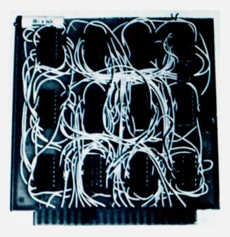
The entire keyboard is contained on one 12-chip prototype board, as shown here.
