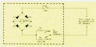
Fig. 1. Simple audio volt-Ohm detector.  $S_{NLT}$ -Mallory SC628 Sonalert.<sup>®</sup> D<sub>1</sub> through D<sub>4</sub>-1N5061 or equivalent. (Any general-purpose diode or package bridge rectifier with a piv rating of 500 V or more should work.)
