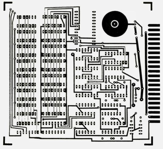
Fig. 4(a). Printed circuit board layout, top side.
