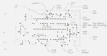
Fig. 1 Front view of the DPM showing how parts are installed
