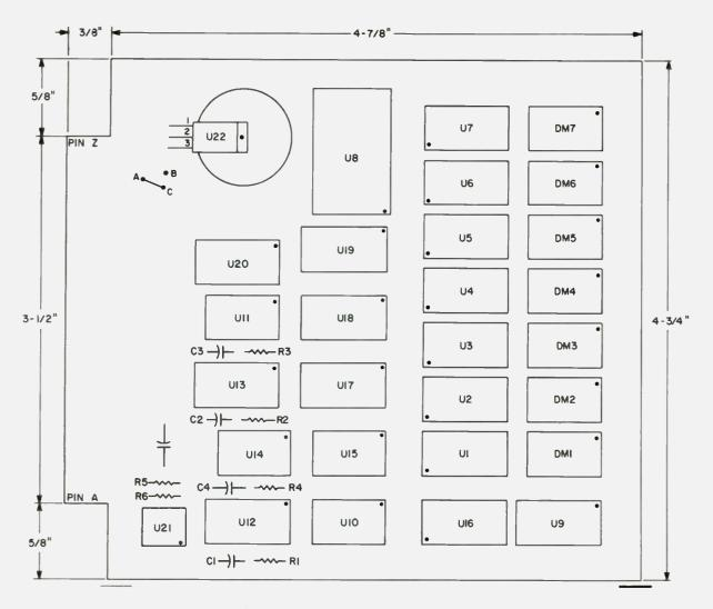
Fig. 2. Printed circuit board component layout and dimensions.
