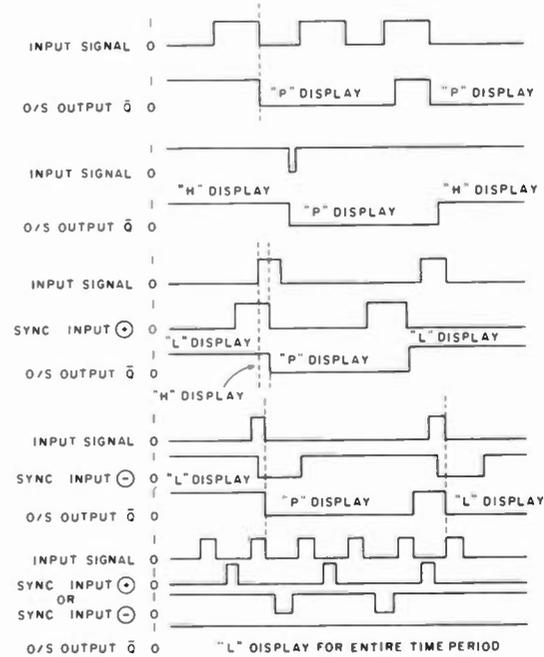
Fig. 2. Timing diagram for logic probe.
