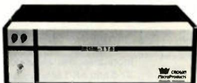
Supports any 8-level serial printer or modem \* Baud rate keyboard selectable \* Expansion interface not required for operation of serial printer or modem.
