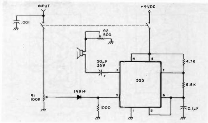
Fig. 2. Voltage-to-frequency converter schematic.
