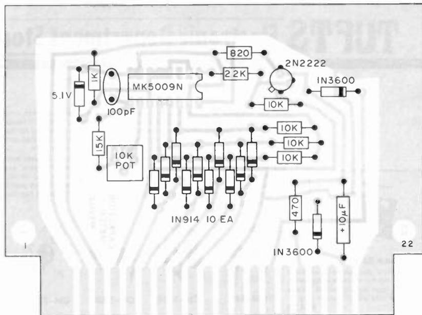
Fig. 2. Capacitor meter parts layout.
