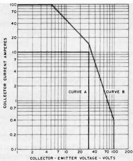
Fig. 4. Operating areas for the electronic load: Curve A indicates the rated operating area for the load. Curve B shows the composite safe area of the four TIP 35C transistors used as the load element. The rated operating area (Curve A) is well inside of the safe area.
