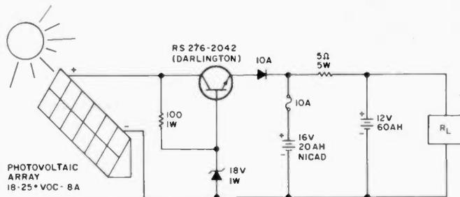
Fig. 2. Power conditioning and storage circuit.
