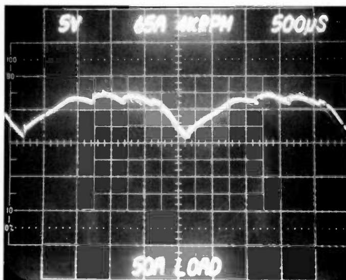
Photo C. Result of open diode in an alternator.
