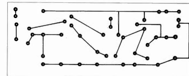
Fig. 2. Foil side of the circuit board.
