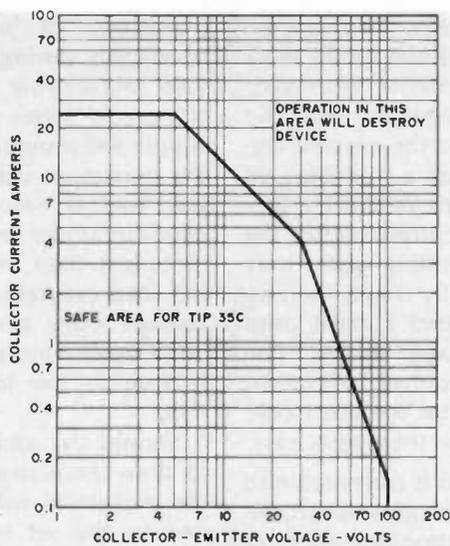
Fig. 3. Safe-area curve for TIP 35C. Safe operation is limited to the area below and to the left of the curve. Operation beyond the safe area will destroy the transistor.
