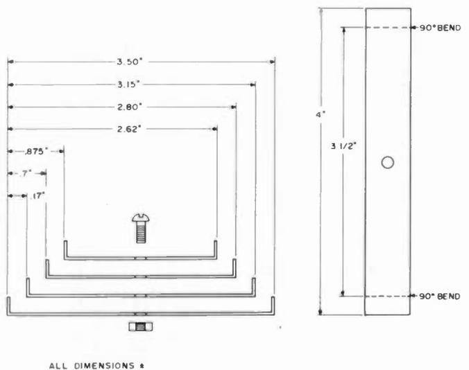
Fig. 2. Heat sink construction details.
