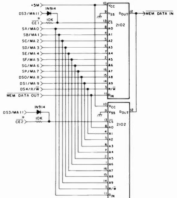
Fig. 3. Memory circuit for a 24-number (or fewer) system. It can be built on header chip and attached to the 18-pin socket.
