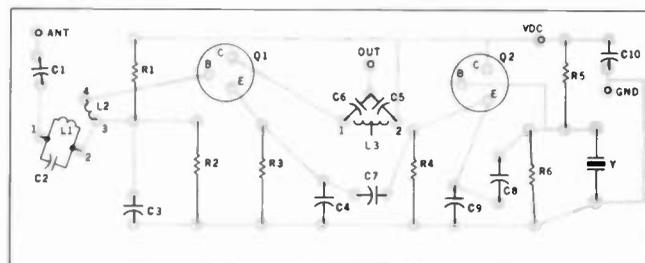
Fig. 3. Parts placement guide (foil side shown).
