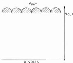
Fig. 2. Three-phase full-wave bridge output.
