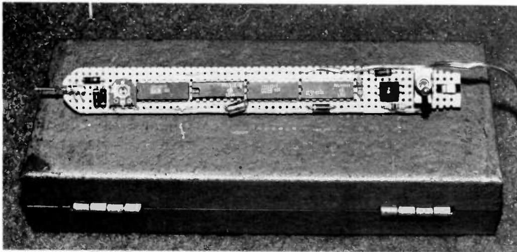
Components are mounted on 0.1" perfboard shaped to fit inside cigar tube.
