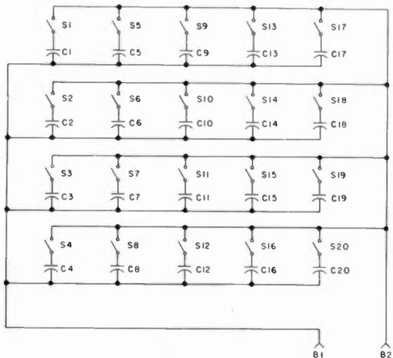
Fig. 2. Schematic for capacitor substitution box.
