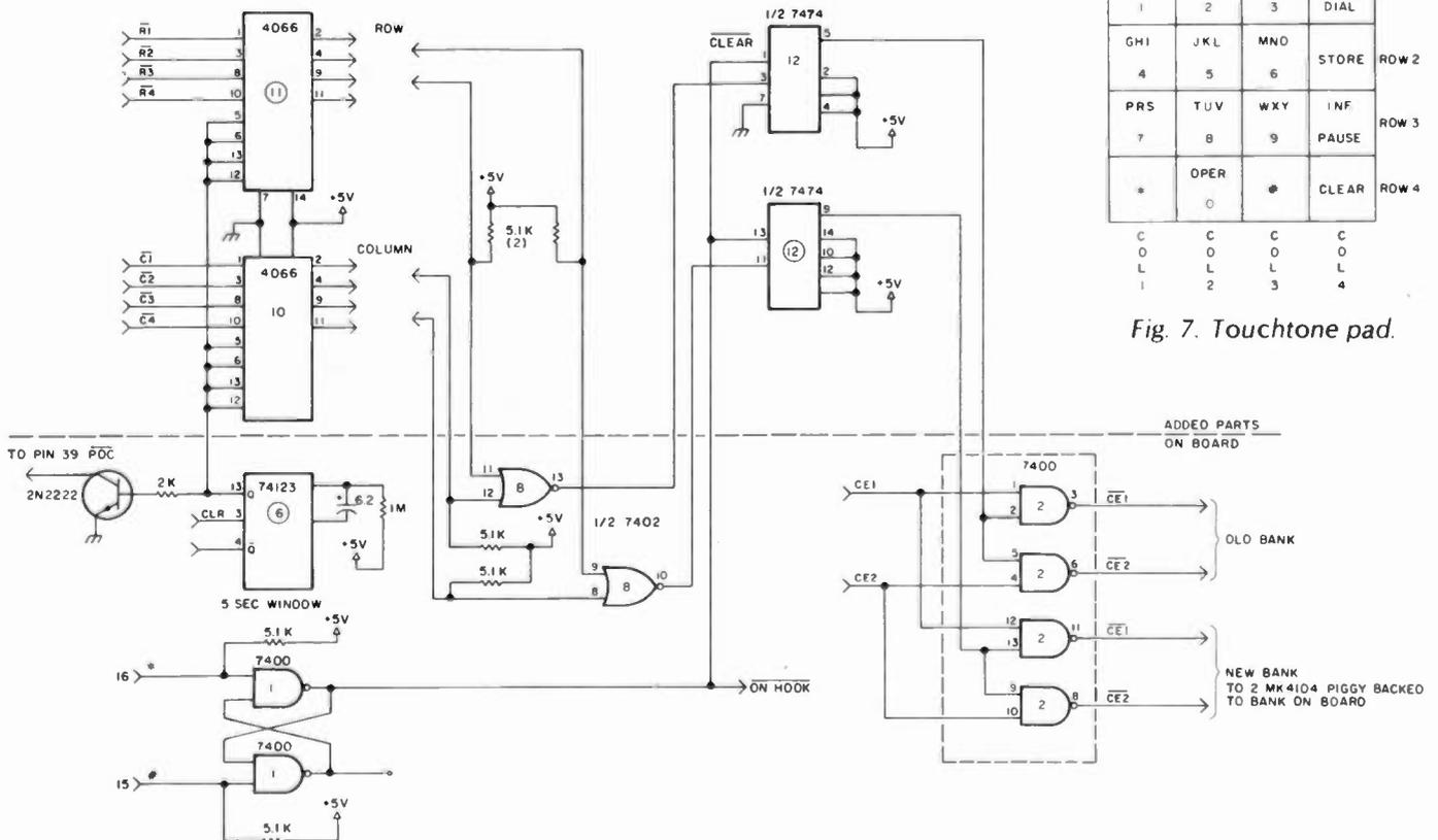
Fig. 8. Expansion circuit for a 200-number system.
