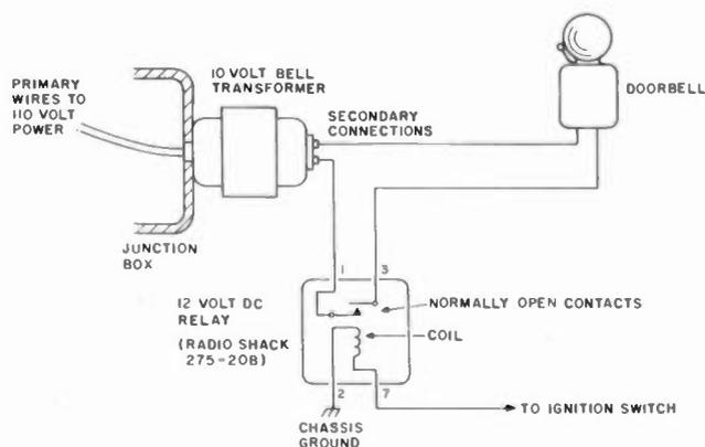
Fig. 1. Wiring diagram of the cord alarm.
