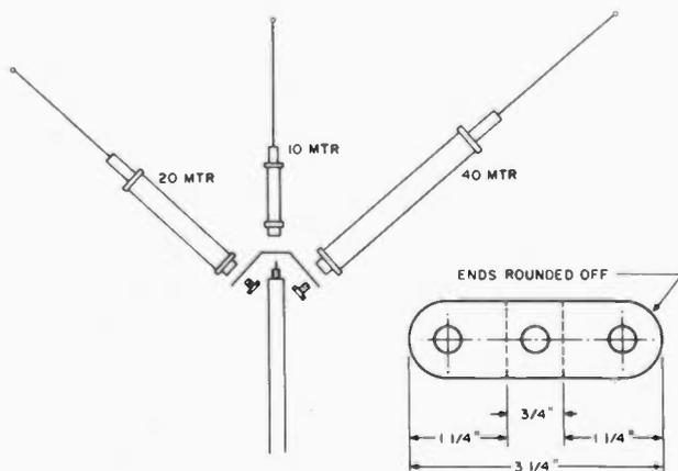
Fig. 1. Four-band mobile antenna construction details.
