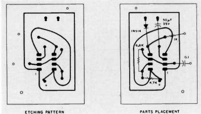
Fig. 3. PCB layout and parts placement.
