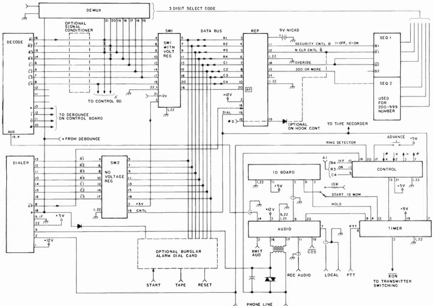
Fig. 5. Basic repeater control system with repertory dialer.
