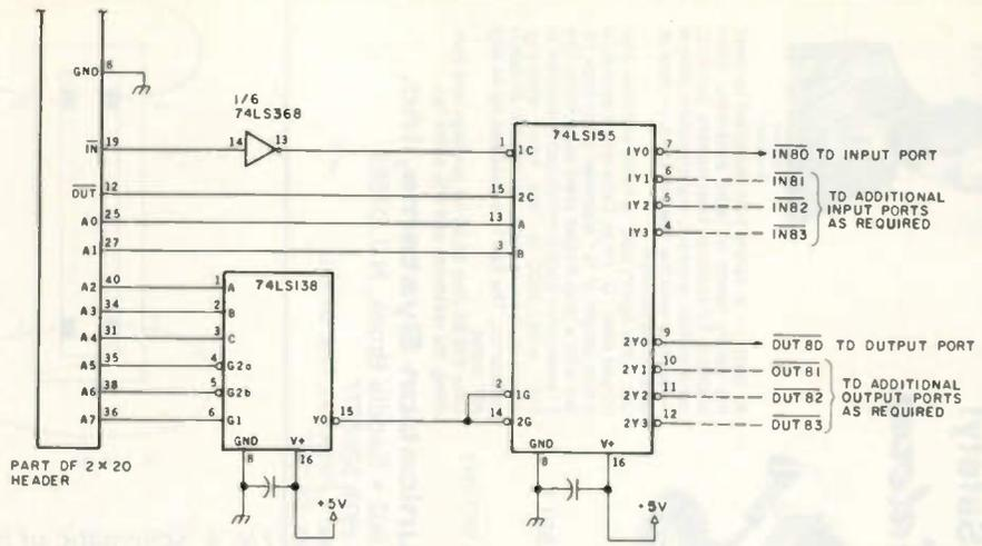
Fig. 1. Schematic of strobe generator circuit. Unmarked capacitors are 0.1- $\mu$ F, 25-volt disc ceramic.
