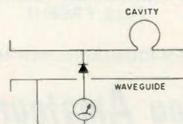
Fig. 2. Cavity wavemeter circuit diagram.
