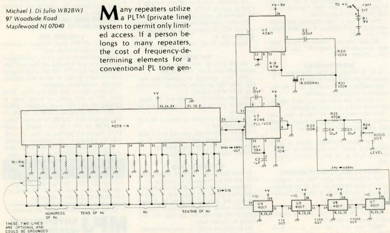
Fig. 1. Synthesized tone generator schematic.
