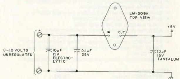
Fig. 3. Schematic of power-supply regulator. The 10- $\mu$ F capacitors are tantalum and electrolytic; the 0.1- $\mu$ F capacitor is disc ceramic.
