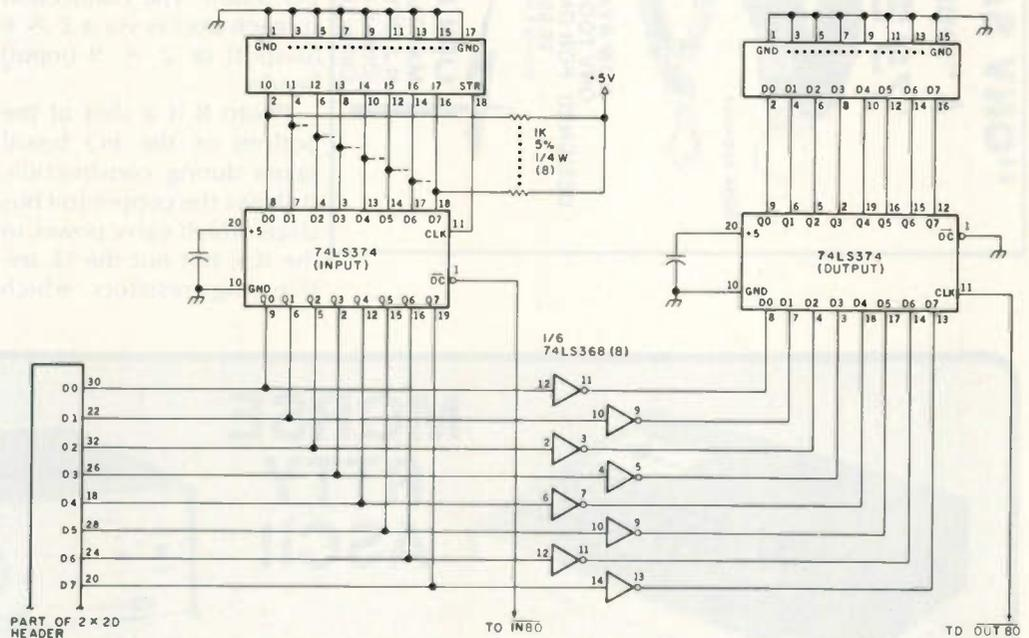
Fig. 2. Schematic of port function circuit. Unmarked capacitors are 0.1- $\mu$ F, 25-volt disc ceramic. Tie enable inputs (pins 1 and 15), unused data inputs (pins 2, 4, and 6), and ground pin (8) of the 74LS368s to ground. Tie +5-volt pin (16) of each 74LS368 to +5 volts and bypass to ground via a 0.1- $\mu$ F, 25-volt disc ceramic capacitor.
