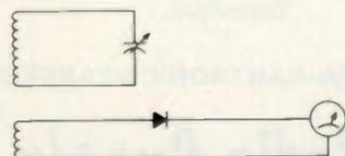
Fig. 1. Parallel resonant equivalent circuit of wavemeter.
