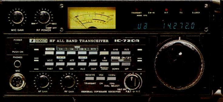
Multi mode operation includes CW/AM/ SSB/RTTY — Normally used side band selected automatically.
