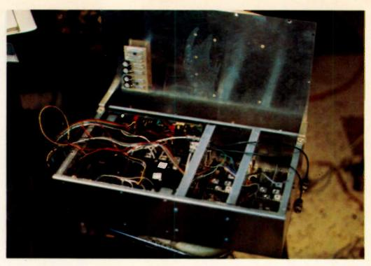
The repeater package with two receivers in the left-hand compartment and the transmitters in two separate compartments on the right.
