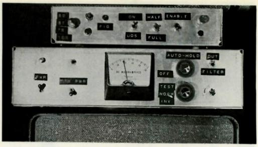
Photo A. TU with Baudot/ASCII converter on top.
