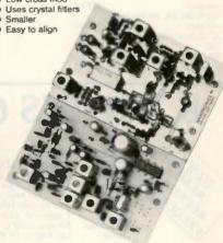
R75A\* VHF Kit for monitor or weather sattelite service Uses wide L-C filter. -60dB at ± 30 kHz. ...
