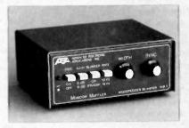
This extremely useful accessory is designed for direct insertion between your receiver (or transceiver) and the antenna. It is both MORE EFFECTIVE than I.F. type blankers and requires NO MODIFICATIONS to your receiver! The unit operates from a 13 VDC  $\pm 2$ VDC power source at less than 575 mA. (AEA AC wall unit AC-1 will operate the blanker.)
