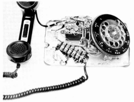
Photo C. Modified telephone set. Note the push-to-talk button in the handset and the resistor-capacitor combination mounted on the added terminal strip.
