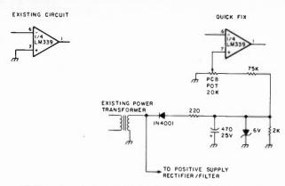
Fig. 3. Eliminating residual negative-voltage effects.
