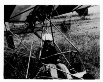
The author intently strapping into the flying harness prior to donning stopwatch, camera, and hand-held. Some of the wire bracing that rigidifies the aircraft structure is clearly visible. The 15-hp engine is mounted below the wing and drives the prop (located behind the wing) through a belt reduction system.
