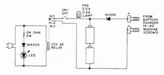
Fig. 1. Schematic of the emergency-lighting project.
