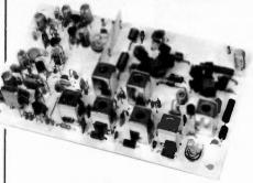
T51 VHF FM EXCITER for 10M, 6M, 2M. 220 MHz or adjacent bands. 2 Watts continuous, up to 21/2 W intermittent, \$68/kit.
