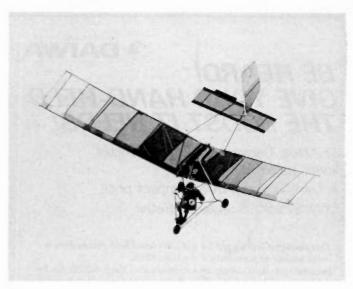
The author photographed during a landing approach. Landings are typically made at low throttle with pilot weight shifted well forward to keep the nose down and the airspeed up. Note the bent knees to achieve this attitude.
