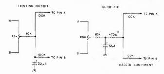
Fig. 4. Input changes to reduce excessive negative voltage.
