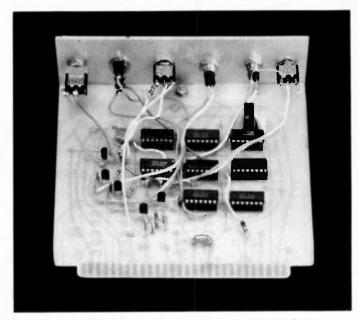
Photo B. Controller built on plug-in card.
