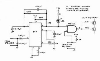
Fig. 2. 73 Morse receive schematic.
