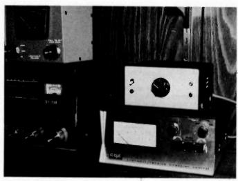
Photo A. The completed beam aimer sits atop the rotator control box at the W4RNL operating position. The ac switch and power LED are to the left and the clockwise and counterclockwise LEDs are to the right. The center knob is the direction control prior to the addition of calibration markings.
