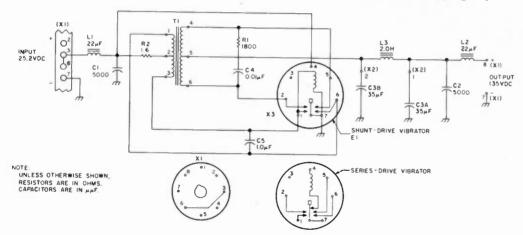
Fig. 1. Original power supply.
