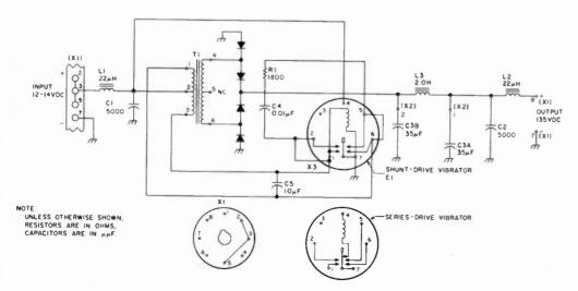
Fig. 2. Power supply modified for 12-14 volts dc.
