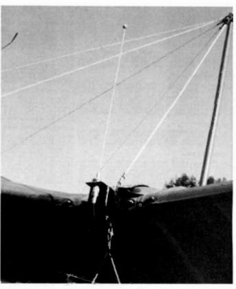
A 2-meter quarter-wave whip anchored to the forward end of the fuselage provides increased range over a rubber duckie partially shielded by the tubular frame of the aircraft.
