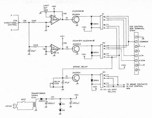
Fig. 1. The original K9AZG automatic beam aimer (redrawn).
