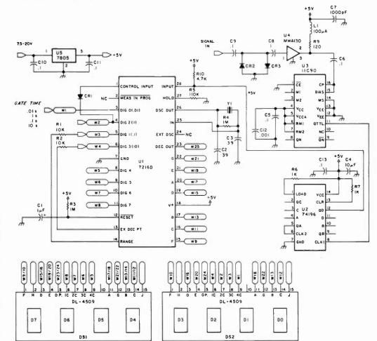
Fig. 2. Frequency counter schematic.
