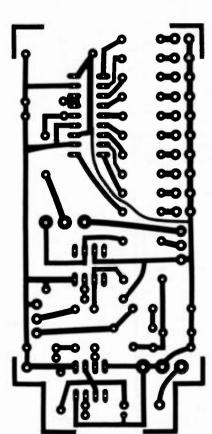
Fig. 3. PC board, foil side.
