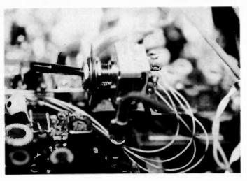
Mounting bracket formed from a bent spring clip.
