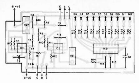
Fig. 4. PC board, component side.
