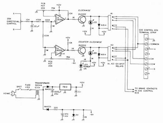
Fig. 5. A simplified beam aimer for the CD-44 and similar rotators.
