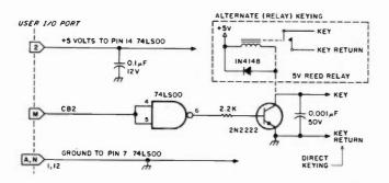
Fig. 1. 73 Morse transmit schematic.
