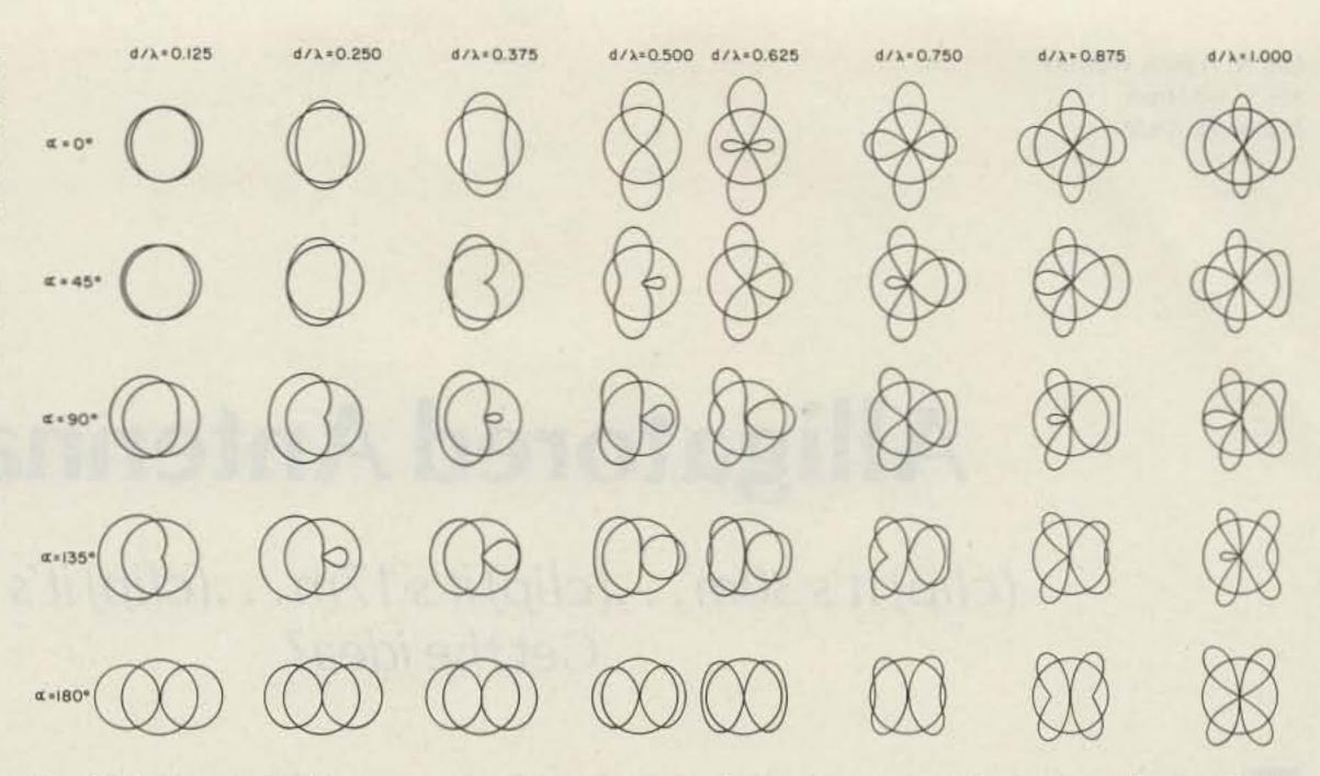
Fig. 2. Horizontal radiation patterns for an array of two antennas fed with equal magnitude currents.
