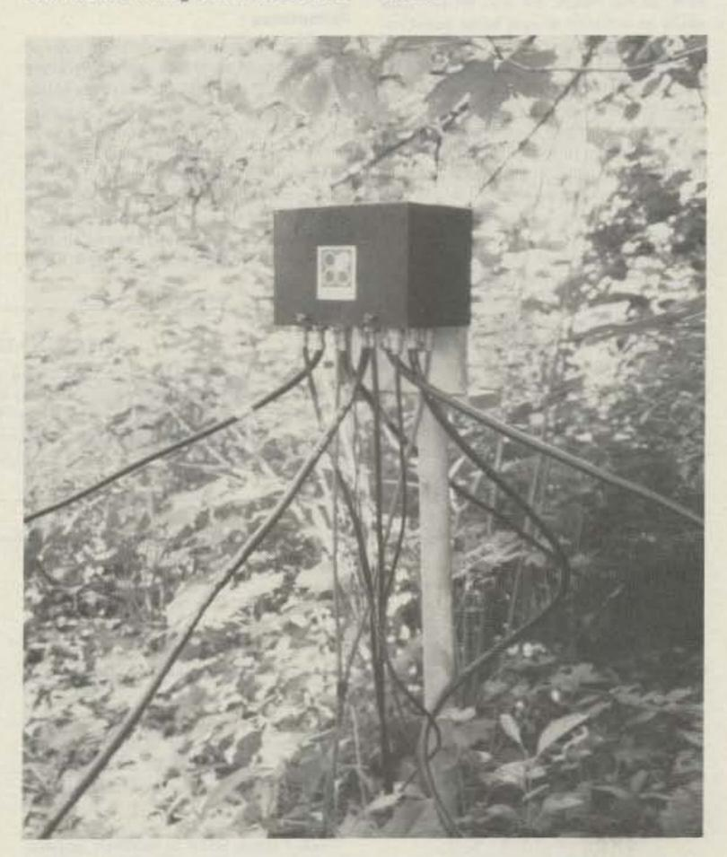
Photo B. Outdoor relay box mounted on owner-supplied pipe. SO-239 connectors are protected from the weather, but ColAtchCo recommends a plastic trash can, too. Phasing lines came pre-cut. No dummy load is evident because I ran an RG-58 line back into my cellar where I put a Heathkit Cantenna.
