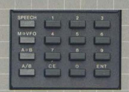
Keyboard Entry. ICOM introduces a unique feature to shortwave receivers...direct keyboard entry for simplified operation. Precise frequencies can be easily selected by pushing the digit keys in sequence of frequency. The frequency will be automatically entered without changing the main tuning control.
