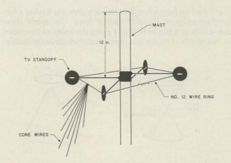
Fig. 4. The ring for the apex of the cone is constructed using no. 12 wire and four clamp-and-screw-type TV standoff insulators. The cone wires are attached in bunches of eight, one bunch to the center of each side of the square.
