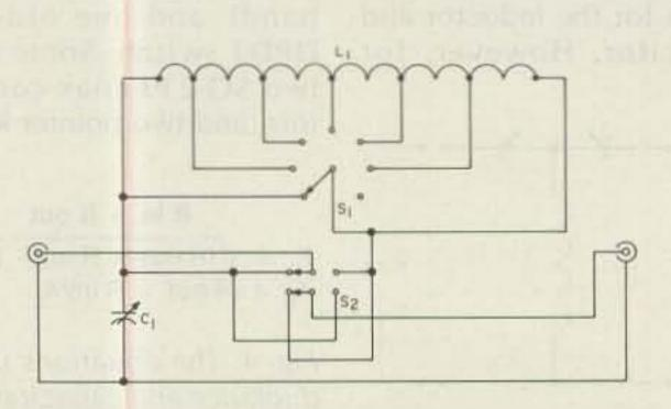
Fig. 6. Schematic of lunchbox L-network antenna tuner described in the text.  $L_1$ —multi-tapped inductor,  $C_1$ —variable capacitor,  $S_1$ —multiple-pole rotatable switch,  $S_2$ —DPDT switch.
