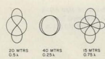
Fig. 2. Theoretical radiation patterns for three bands.
