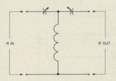
Fig. 3. The T network is known for its poor harmonic attenuation. It sometimes becomes a high-pass filter.
