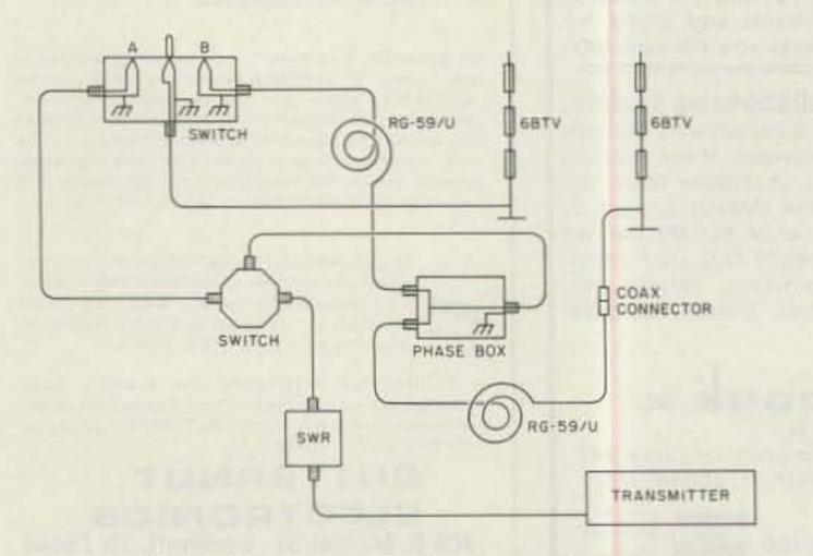
Fig. 1. Phased-vertical system diagram.
