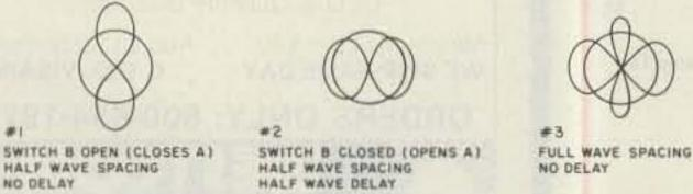
Fig. 1. Switching diagram.
