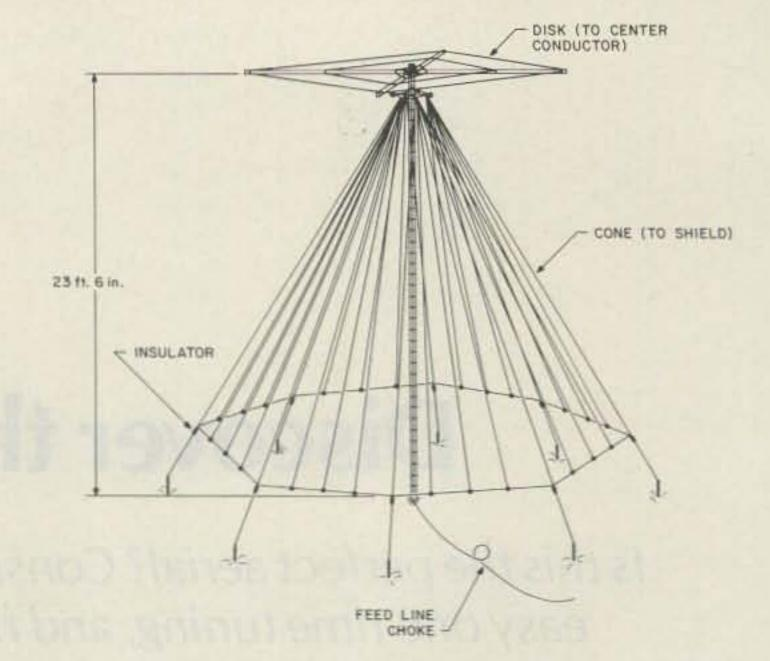
Fig. 3. Construction of the 10-30-MHz discone. The slant height is 23 feet, 8 inches; the square disk has a diagonal radius of 8 feet. The supporting mast is 23 feet, 6 inches high.
