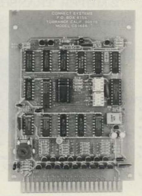
Our new CS-1688 is the most powerful touch tone controller in the industry! DIP switch programmability allows you to choose any of these ten mode/function combinations...
