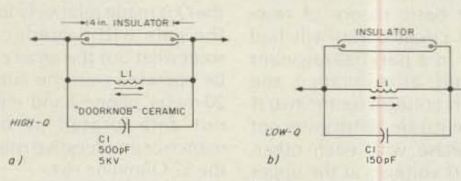
Fig. 5. Phase-shift circuit details. L1 in a) is three turns 1/4" copper tubing, 2-1/2" diameter, 4" long. Spread or compress turns as indicated by arrows to resonate circuit to desired frequency. Narrow bandwidth but easier to load. L1 in b) is seven to eight turns of same-dimensions tubing, spread or compressed, providing greater operating bandwidth.
