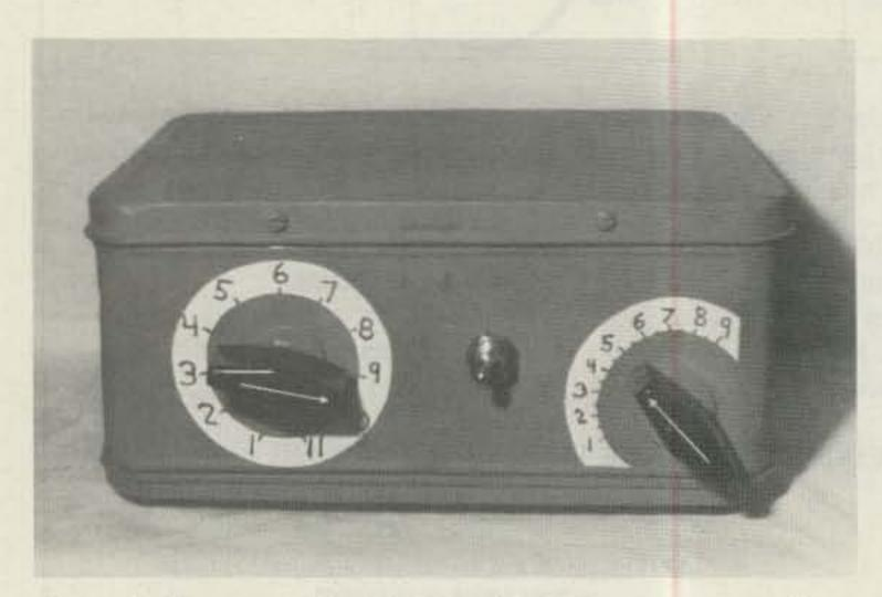
Photo A. Front panel of the lunchbox antenna tuner. Controls, from left to right, are: inductor taps, R-in/R-out switch, and variable capacitor.
