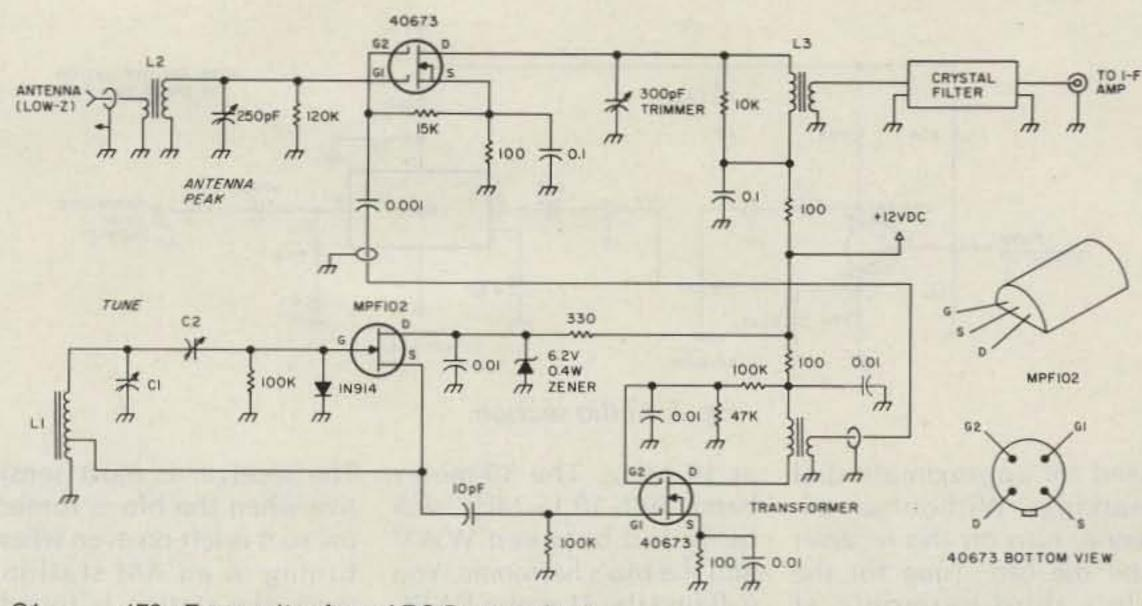
C1 170-pF capacitor from ARC-5 transmitter
