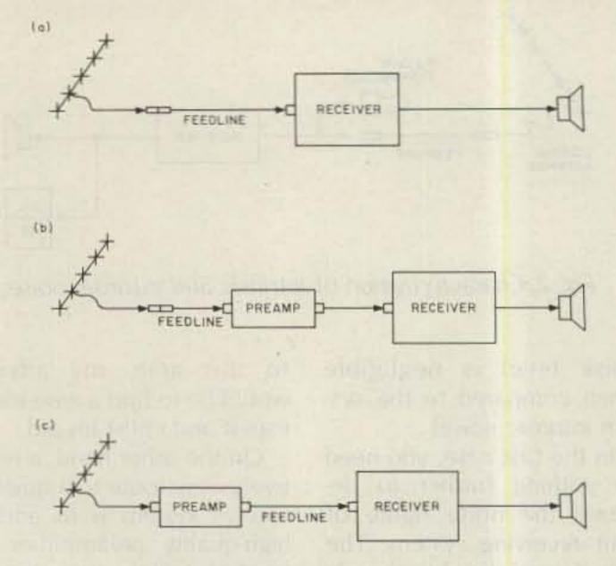
Fig. 3. System configurations.
