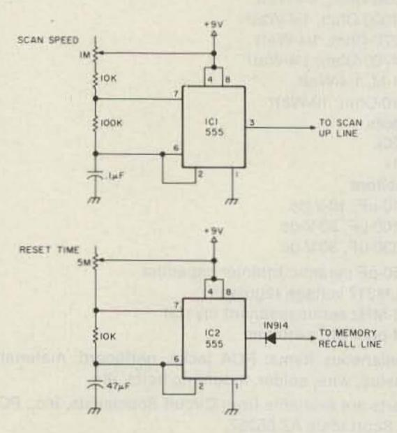
Fig. 2. Simple scan and reset circuit.
