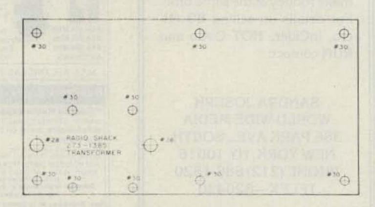
Fig. 2. Perfboard, hole placement
