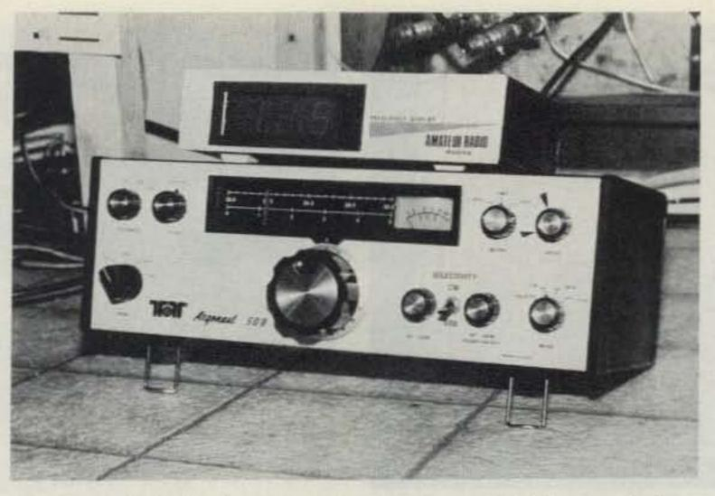
The four-digit display gives the Argonaut 100-Hz resolution.
