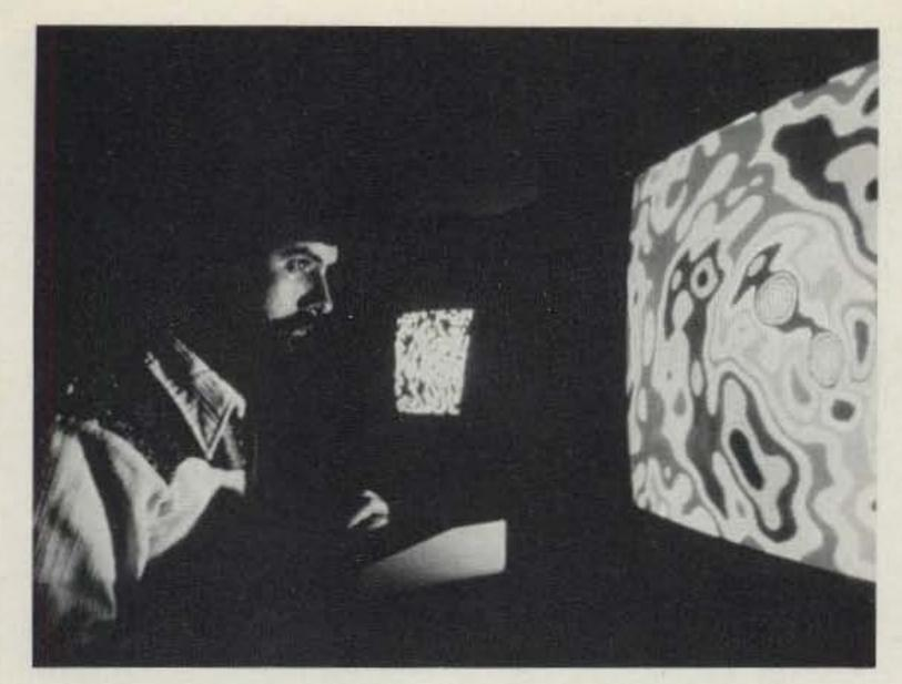
Most of the observations from the VLA are processed into radio images or maps. The color graphics are produced by VLA computers. Colors are used to depict varying intensities in the radio images.
