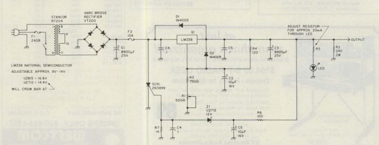
Fig. 1. 12-V-dc power supply with crowbar protection.
