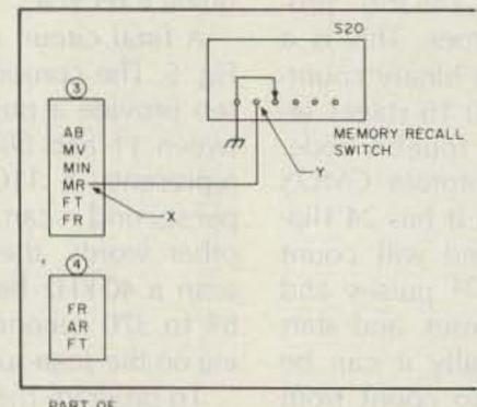
TACK SOLDER A WIRE TO POINT X OR Y ON SWITCH UNIT M PC BOARD, OTHER END OF WIRE TO AN UNUSED PIN ON MIC CONNECTOR.
