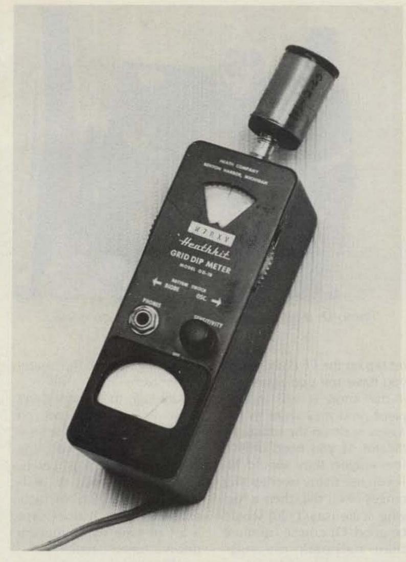
Photo A. By adding an F connector and winding coils on plastic film cans you can recycle older grid-dip meters when you can't get the original coils.
