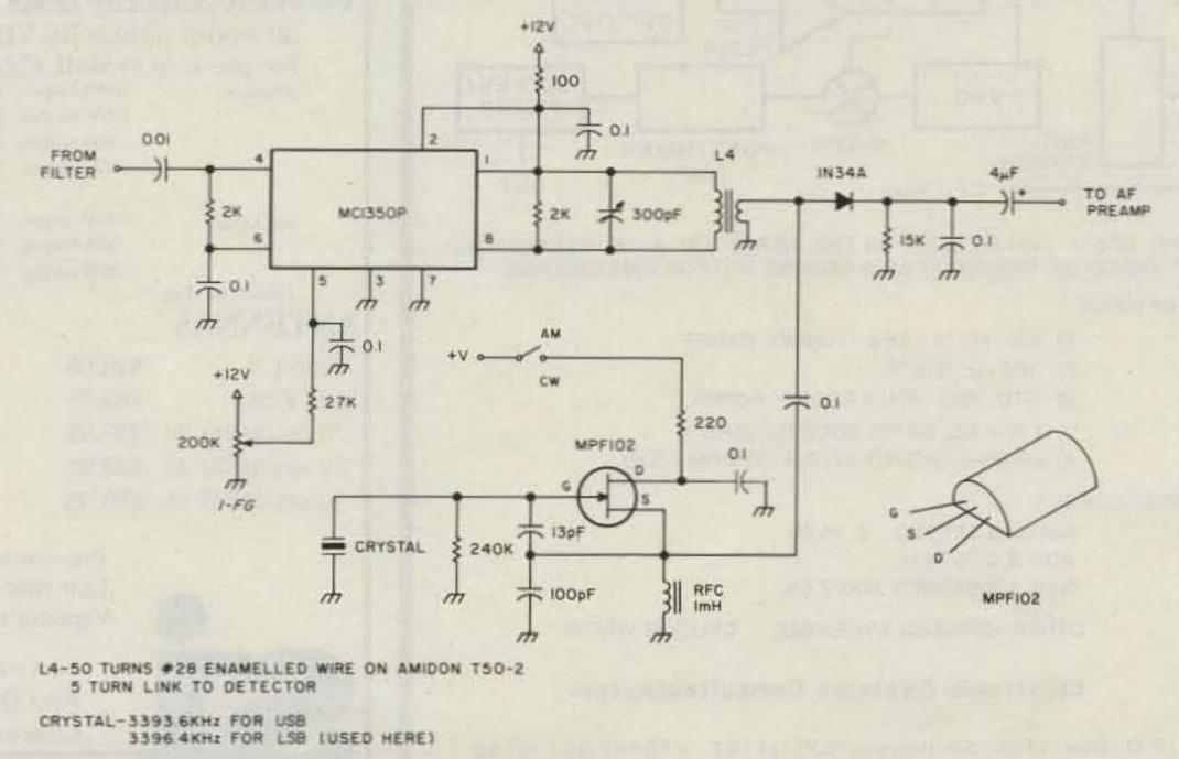
Fig. 3. Detector, i-f amplifier, and bfo schematic.
