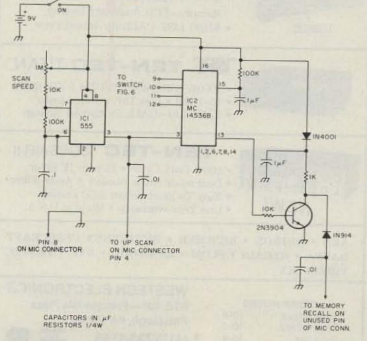
Fig. 5. TS-930S scan circuit.
