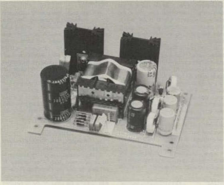
The Adtech CS-1307 switching power supply.
