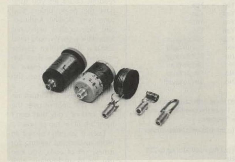
Photo B. Some of the HF and VHF coils (going up to over 200 MHz).
