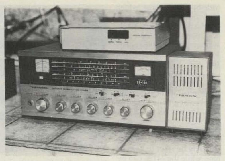
The slide-rule dial on the DX-160 is used only to determine the frequency to the nearest megahertz. The simple threedigit display resolves to 1 kHz.
