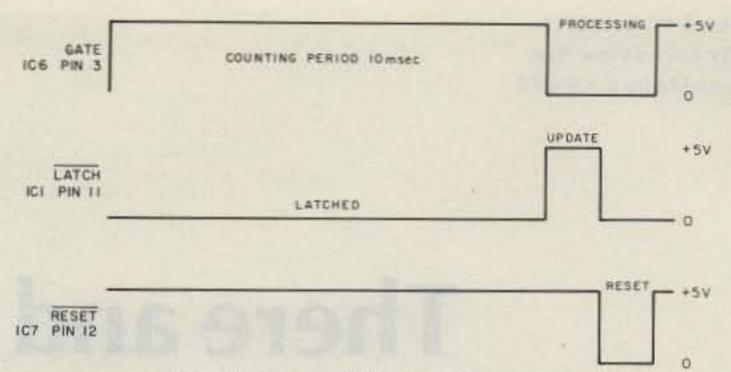
Fig. 5. Control timing diagram.
