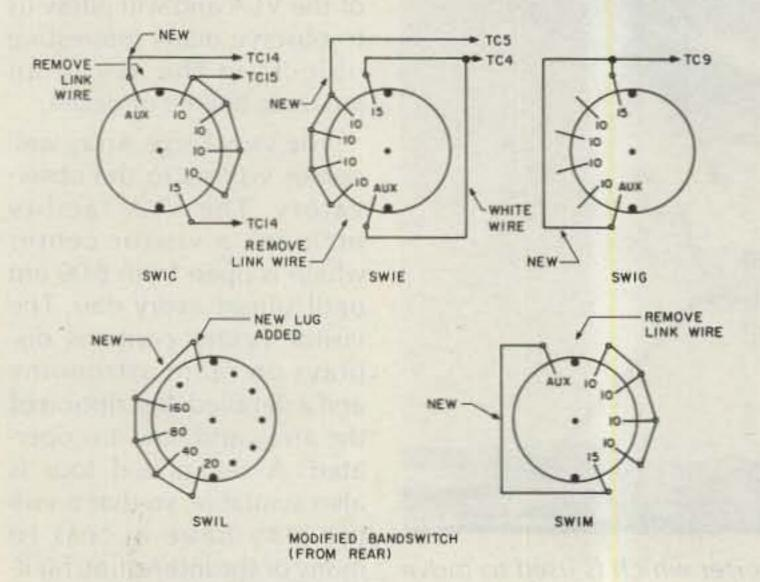
Fig. 1. Modified bandswitch (from rear).
