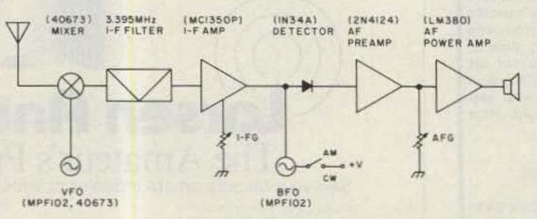
Fig. 1. Block diagram. The receiver operates on 12 V dc, uses low-impedance earphones or a speaker, and requires a low-impedance antenna.
