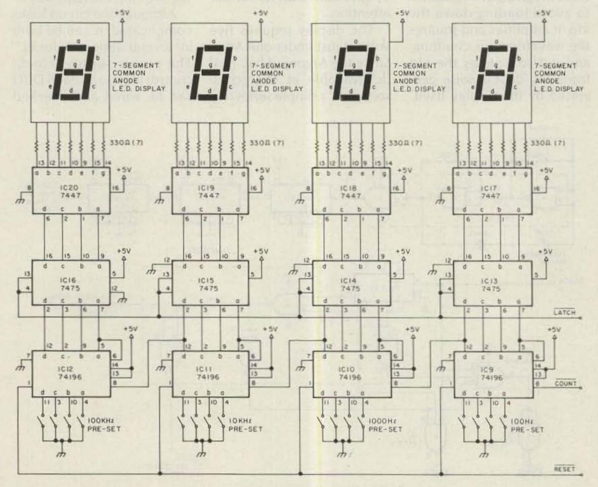
Fig. 4. Counter and display logic.
