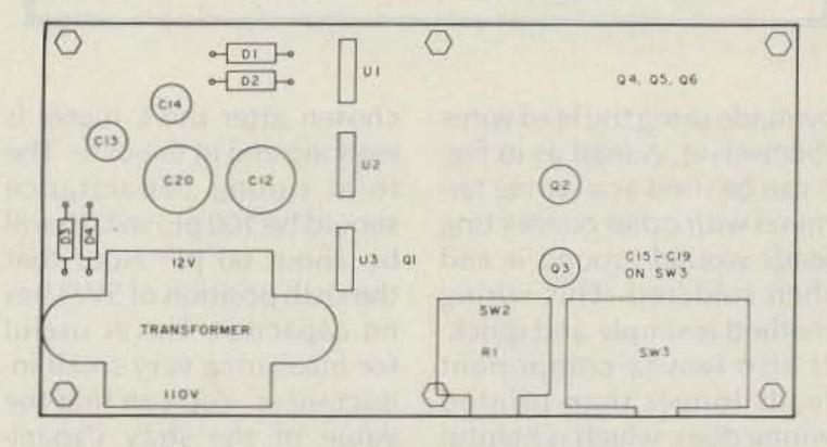
Fig. 4. Parts placement, bottom view.
