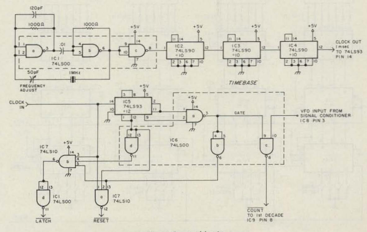
Fig. 3. Control logic.
