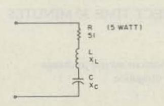
Fig. 2. Special dummy load.
