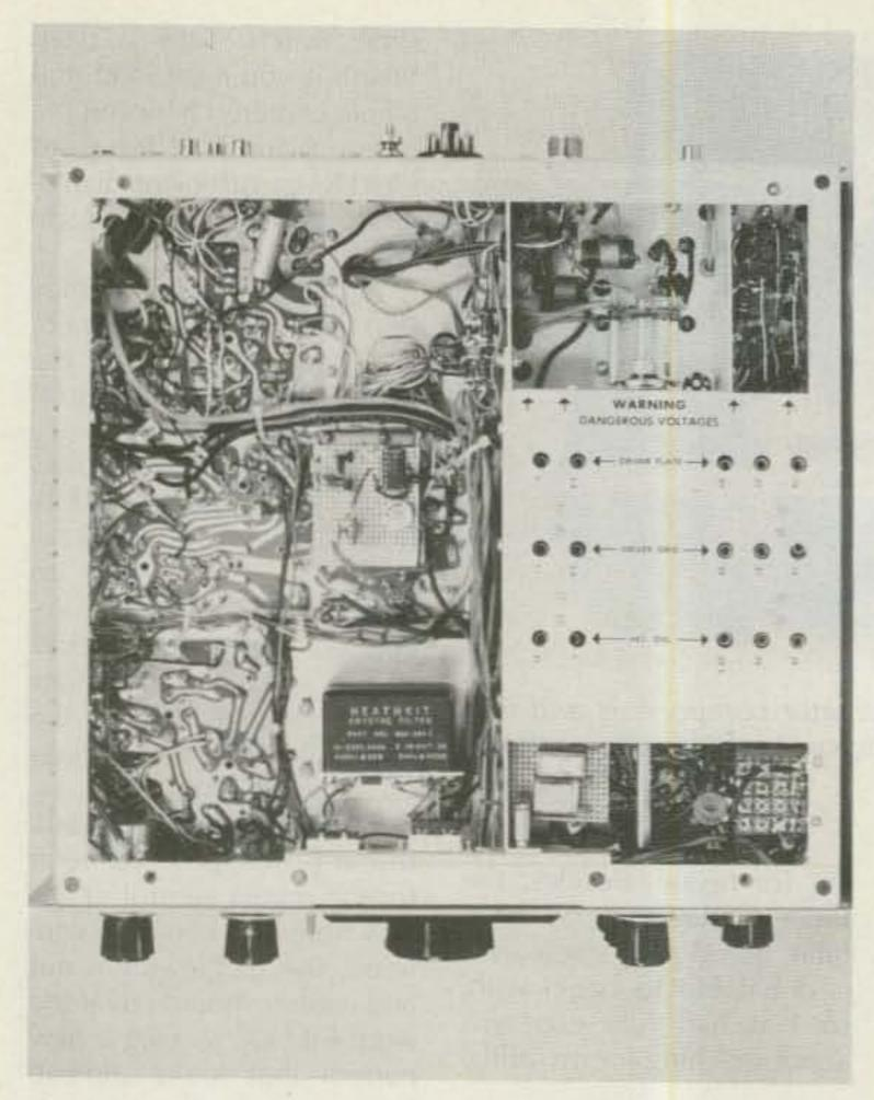
Photo D. Bottom view, showing placement of dc power supply, calibrator, crystal-filter relay, WWV board, and microphone preamp.
