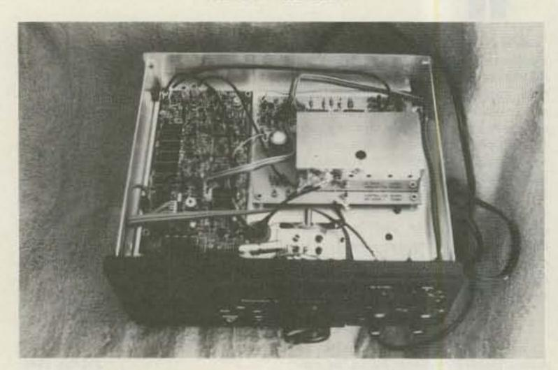
Inside the SW-7800. The receiver PC board is mounted below the sub-chassis.
