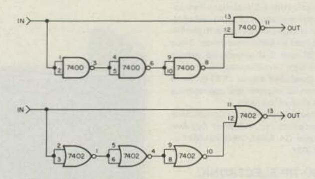
TWO-WAY EDGE DETECTION: When you need an edge-detector for a positive- or a negative-going change and don't want to use a one-shot, try this circuit. Using NAND gates will yield a single LOW pulse when the input goes from LOW to HIGH. Using NOR gates, a single HIGH pulse is generated when the input switches from HIGH to LOW. Any odd number of gates can be used in the delay leg feeding the final gate. The more delay gates used, the longer the output pulse.—Paul Selwa N9CZK, Brownsburg IN.
