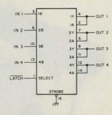
scheme will not work due to the switching delays within the IC.
