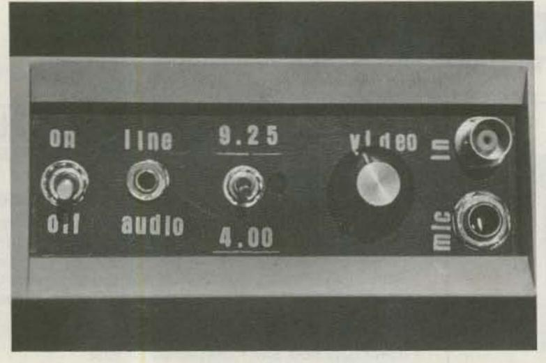
Photo F. Panel layout. The bezel (see text) shields the switches from accidental tripping.
