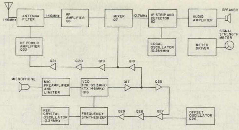
Fig. 1. Block diagram of the DSE Commander.
