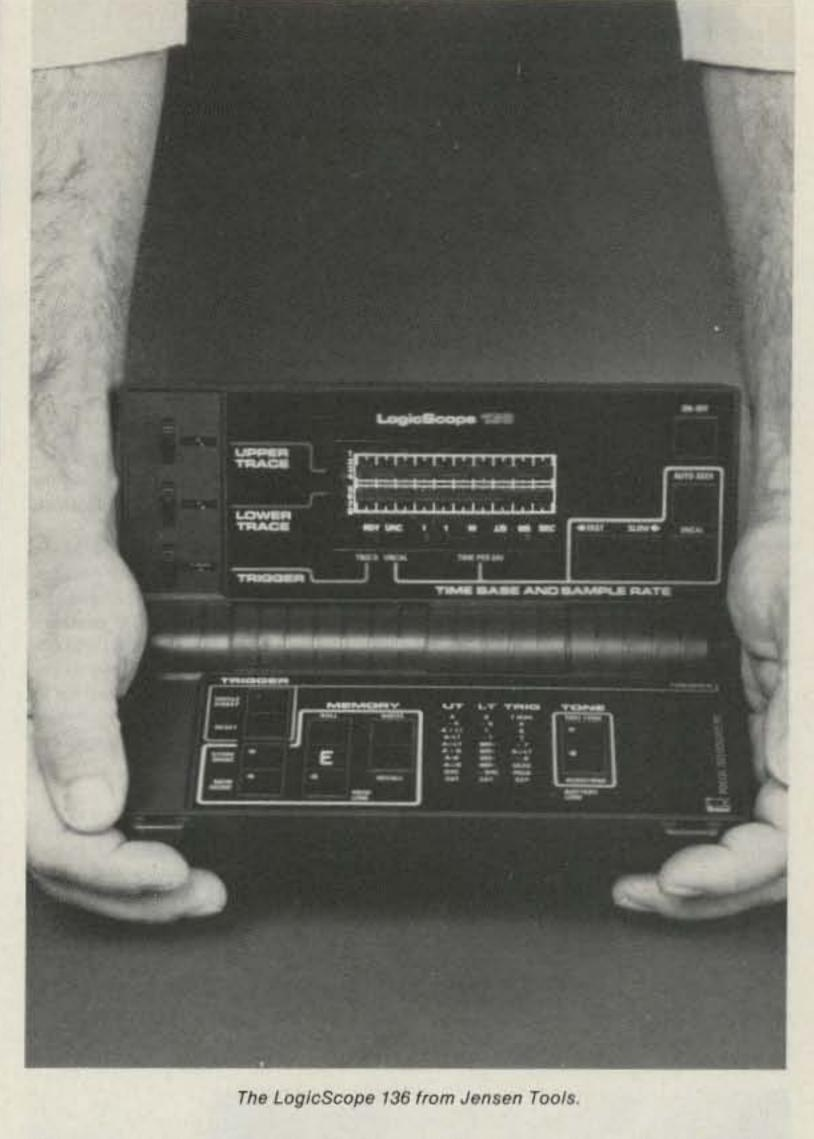
mits the simultaneous display of two waveforms. It can be operated in real-time or memory mode. Memory mode permits acquisition and storage of up to twentyfour 128-bit waveforms. Waveforms can be recalled and logically compared (AND, OR, exclusive OR) to other stored or input waveforms. An RS-232 port provides for a modem link capability for signal transfers as well as for future expansion features.
