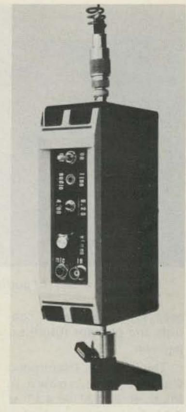
Photo B. The ready-to-use 1-Watt video transmitter supported by a tabletop photographic tripod. The optional bezel is described in the text.
