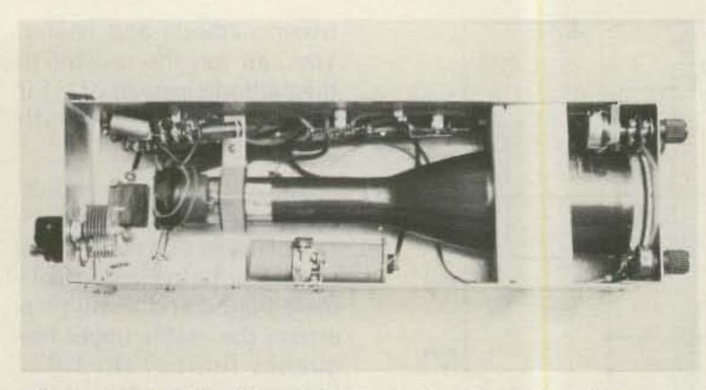
Photo C. Details of the CRT mounting. Note the clamps on the neck and the styrofoam block on the body of the CRT.
