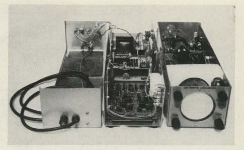
Photo B. Interior view of the monitor scope. The power supplies are at the rear.
