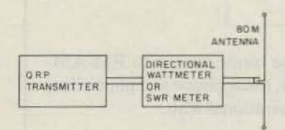
Fig. 1. QRP transmitter hooked through directional wattmeter or swr meter to 80m antenna.
