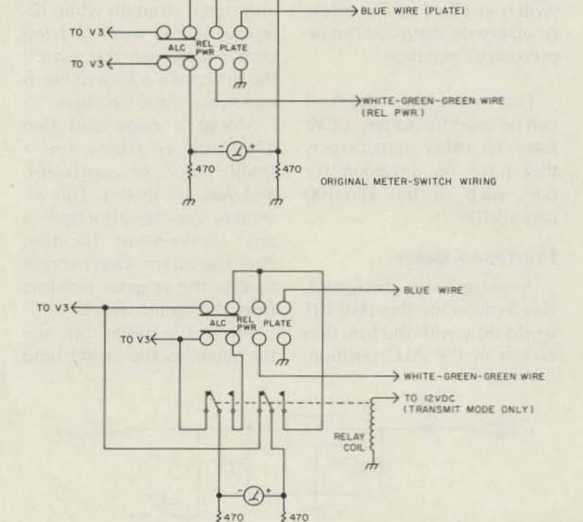
Fig. 6. The new relay makes the S-meter independent of the meter switch. Observe meter polarity when connecting relay to switch.
