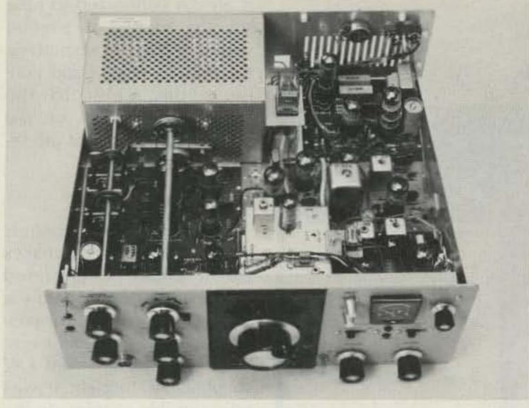
Photo C. Note "missing" calibrator components and rearpanel sidetone control. The relay on the rf cage is for outboard vfo control.
