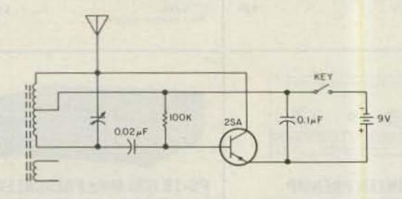
Fig. 1. The original rf oscillator circuit.
