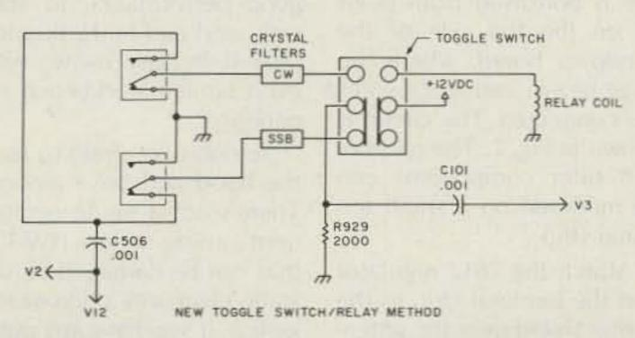
Fig. 5. The unreliable and noisy slide switches are replaced with a toggle switch and relay for crystal-filter selection.
