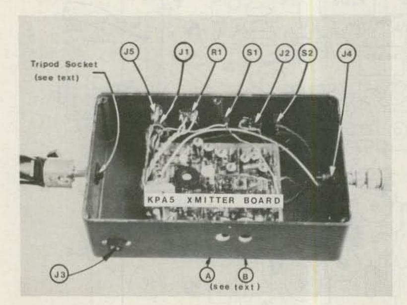
Fig. 2. A middle-of-the-road approach to packaging the transmitter board. Video-level control is brought out to the panel as are connector jacks and switches. Audio levels are screwdriver-adjusted through access holes A and B.
