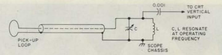
Fig. 5. Coupling rf to oscilloscope.
