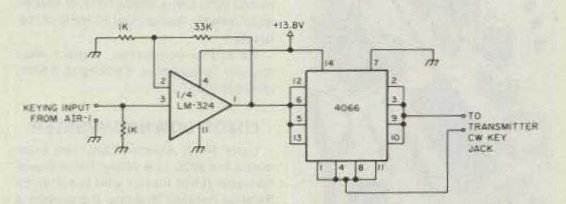
COMPUTER-TO-RIG INTERFACE: I needed a circuit to allow my VIC-20/AIR-1 to key an FT-707, which requires a set of closed contacts such as a straight key. The keying output of the AIR-1 is 0–0.6 V dc, which drives one quarter of an LM-324 op amp. The 13-V output of the LM-324 activates a CMOS switch, keying the rig. The four CMOS switch contacts are wired in parallel to reduce the "on" resistance.—Dave Ball WA4PQD, Barrington NH.
