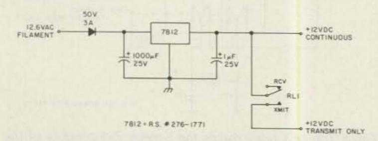
Fig. 7. Regulated power supply for modifications. Don't overlook the 1-μF capacitor at the 7812 output.
