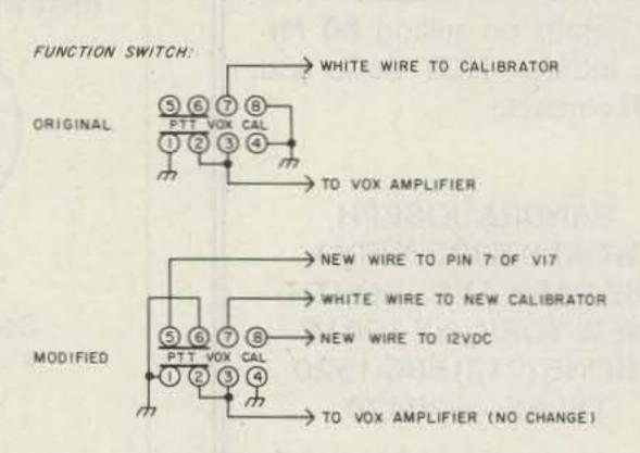
Fig. 1(b). Modified function switch.
