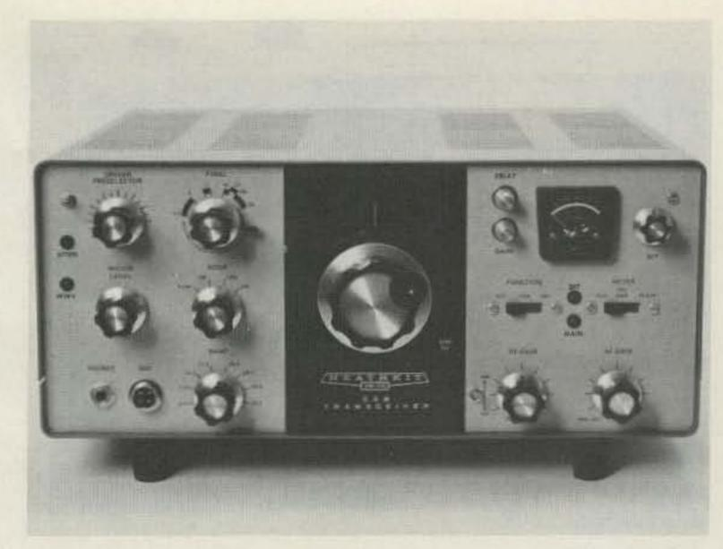
Photo A. The finished product with new controls, LED status indicators, and spinner knob.
