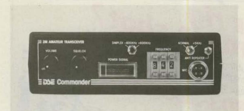
Photo A. The DSE Commander two-meter transceiver kit.
