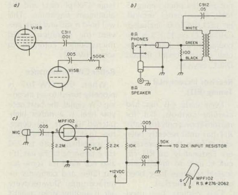
Fig. 4. The SB-102 sidetone level control is at A. At B, the audio transformer output is rewired for 8-Ohm output to speaker and phones. C shows a simple microphone preamplifier.
