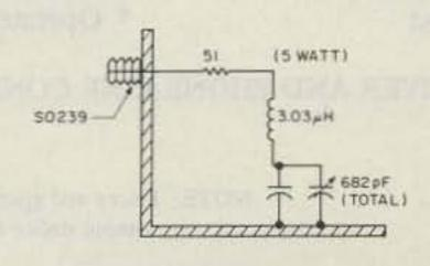
Fig. 3. Construction of special dummy load.
