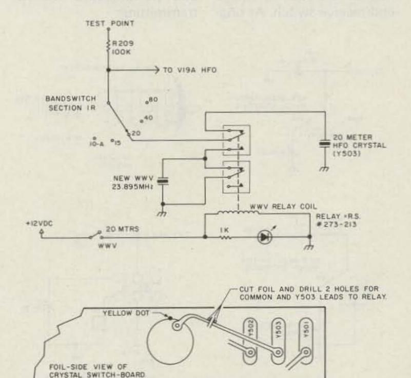
Fig. 2. Modification of hfo circuit for 15-MHz WWV reception.
