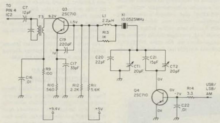
Fig. 2. Unmodified oscillator/doubler.
