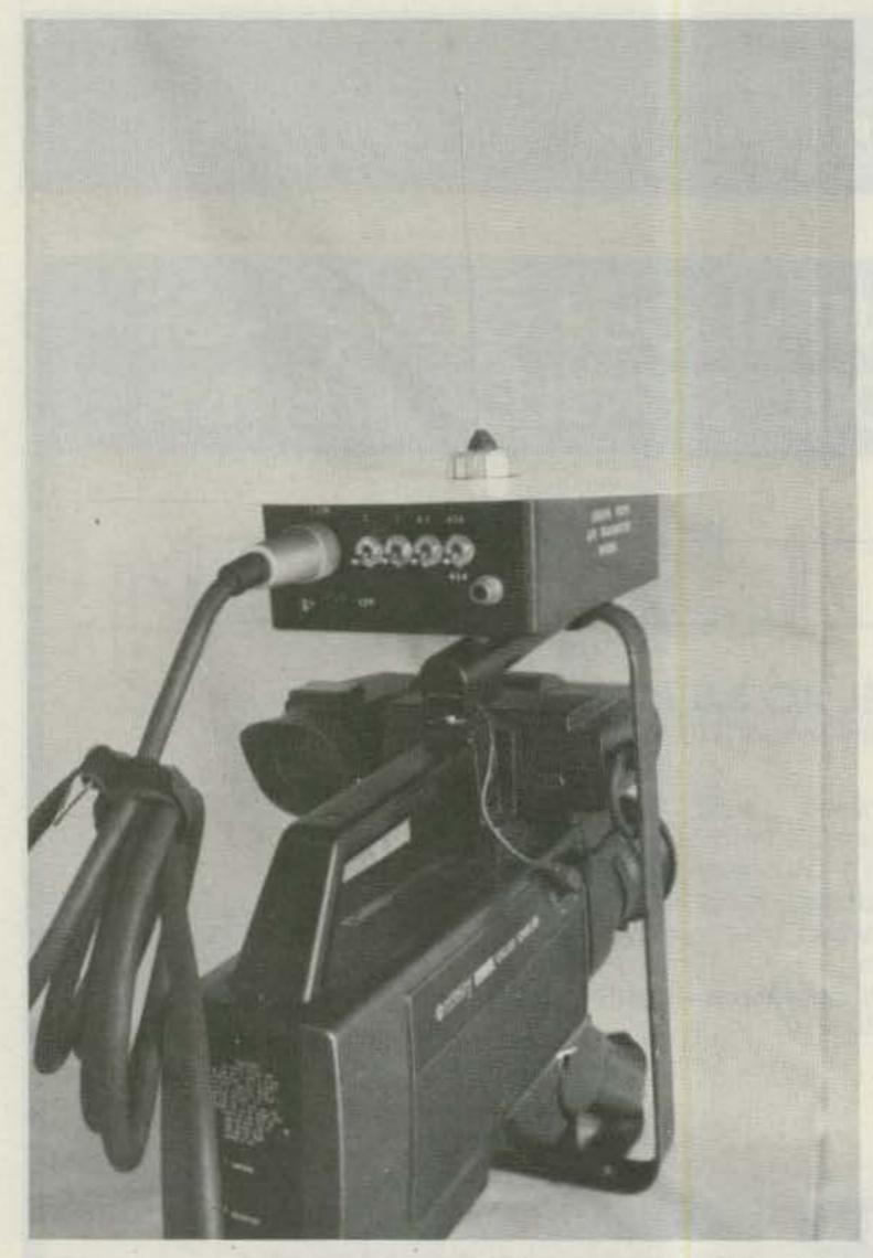
Photo A. Camera with transmitter in a Hammond #1590D housing. Also shown is the thirteen-inch ground-plane disc needed with most cameras for an rf shield. (Photo by P.C. Electronics)
