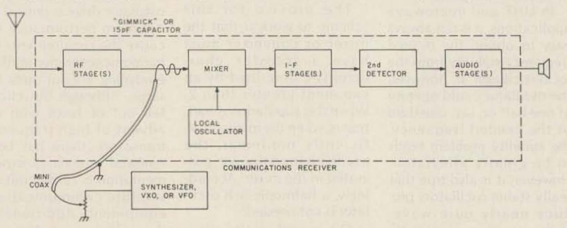
Fig. 10. A somewhat better arrangement for receiving SSB signals with an older set. In this setup, the signal-frequency injection takes place following one or more rf stages. Also, the use of a synthesizer is suggested.
