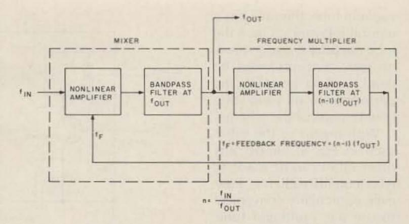
Fig. 3. Block diagram of the regenerative modulator. The amplifiers can be either tube or solid-state devices. The bandpass filters can be simple parallel-resonant circuits. The basic function of this arrangement is that of a frequency divider. Unless the proper frequency is applied to the input  $(f_{IN})$ , there is no output.
