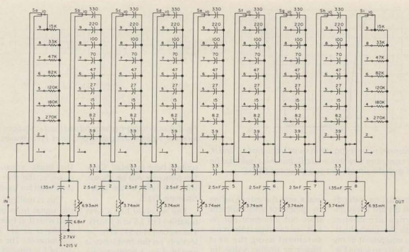
Fig. 3. The actual circuit diagram of the filter with selectable bandwidth. Capacitor values in picofarads unless designated nF (nanofarads). Sa through Si are the decks of the bandwidth-selector switch.
