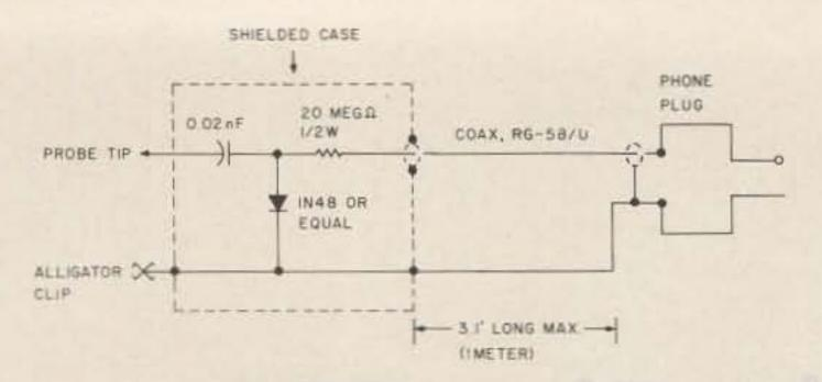
Fig. 2. Rf probe circuit.
