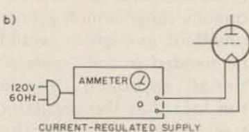
Fig. 8. Traditional and proposed methods of lighting up your transmitting-tube filaments: (a) the "good old way" and manually-adjusted voltage across tube socket may not have been so good after all; (b) proposed technique.
