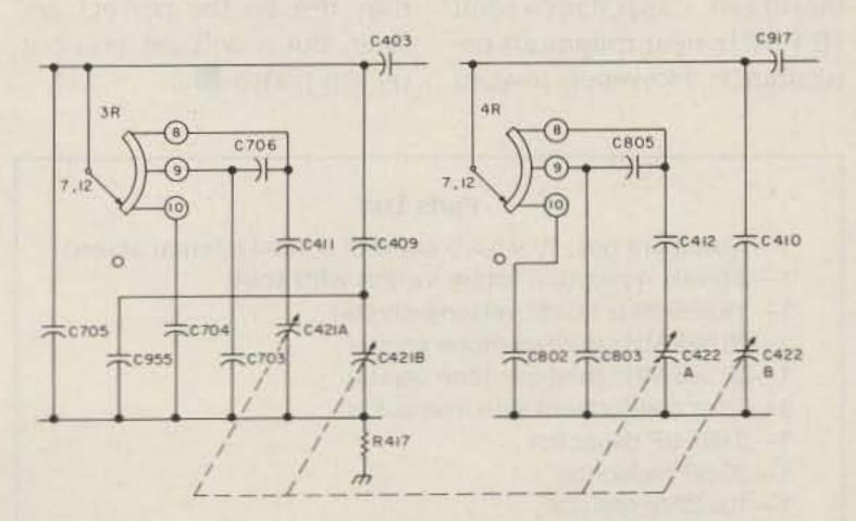
Fig. 2(b). Tuned circuits (inductors omitted) of driver input and output after modification to enable 7 and 10 MHz to be tuned with one inductor.
