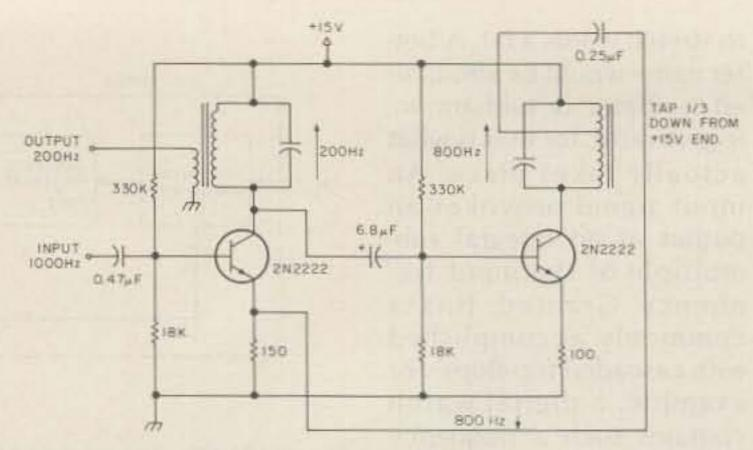
Fig. 5. An experimental transistor version of a regenerative modulator. Although this example circuit operates at low audio frequencies, the basic idea is applicable to radio frequencies as well.
