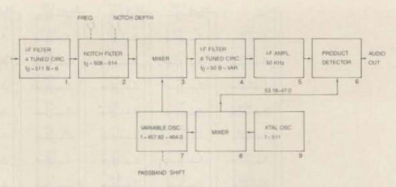
Fig. 5. Block diagram of second and third i-f sections in PAØSE's receiver, incorporating passband shift. Frequencies in kHz.
