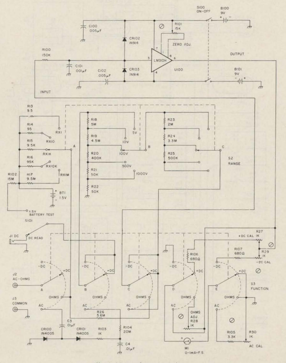
Fig. 1. Meter after conversion.
