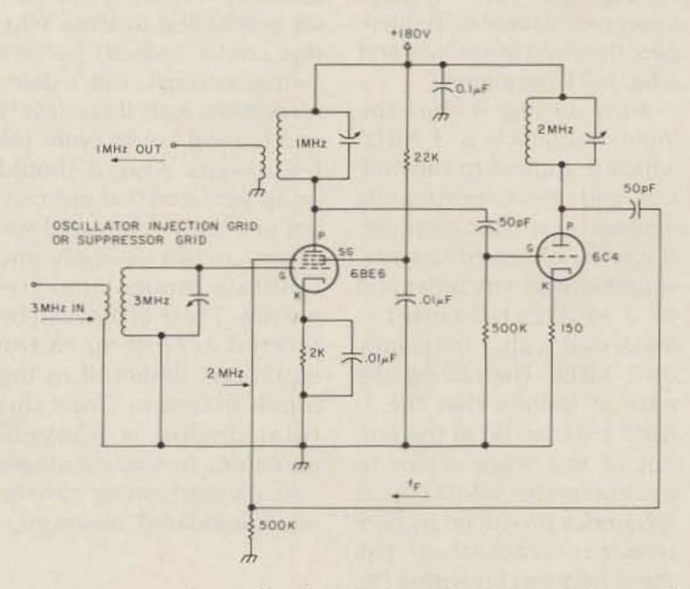
Fig. 4. An experimental tube version of a regenerative modulator. Strong drive is needed so that the tubes are operated in their nonlinear regions. The first tube can be any of a variety of multi-grid tubes such as converters, pentodes, etc.
