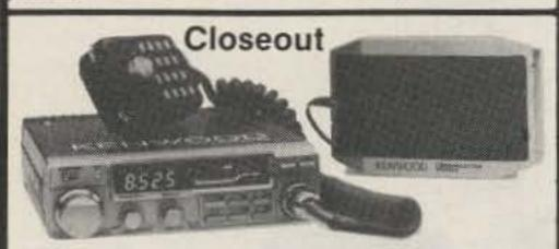
KENWOOD TM-401A 440 MHz FM Xcvr Ultra compact! Covers 440-449.975 MHz in 25 kHz steps, 12W out. GaAs FET RF amplifier, dual digital VFO'S, 5 memories plus "com" channel w/back-up. Priority alert scan, memory and programmable band scan. Yellow LED display, LED S/RF meter, Ext. spkr, 16-key TTP UP/DN mic, mobile mt. 5%"w×1%"h× 7%"d, 2.8 lbs. List \$39995... CLOSEOUT \$27995
