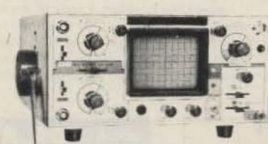
Ideal for field/bench applications, this scope can display up to 15 MHz signals. Internal battery pack allows up to 2 hours operation on a single charge. Features include . built-in battery charger • 5X horizontal magnification high brightness CRT • front panel trace rotator . internal rechargeable
