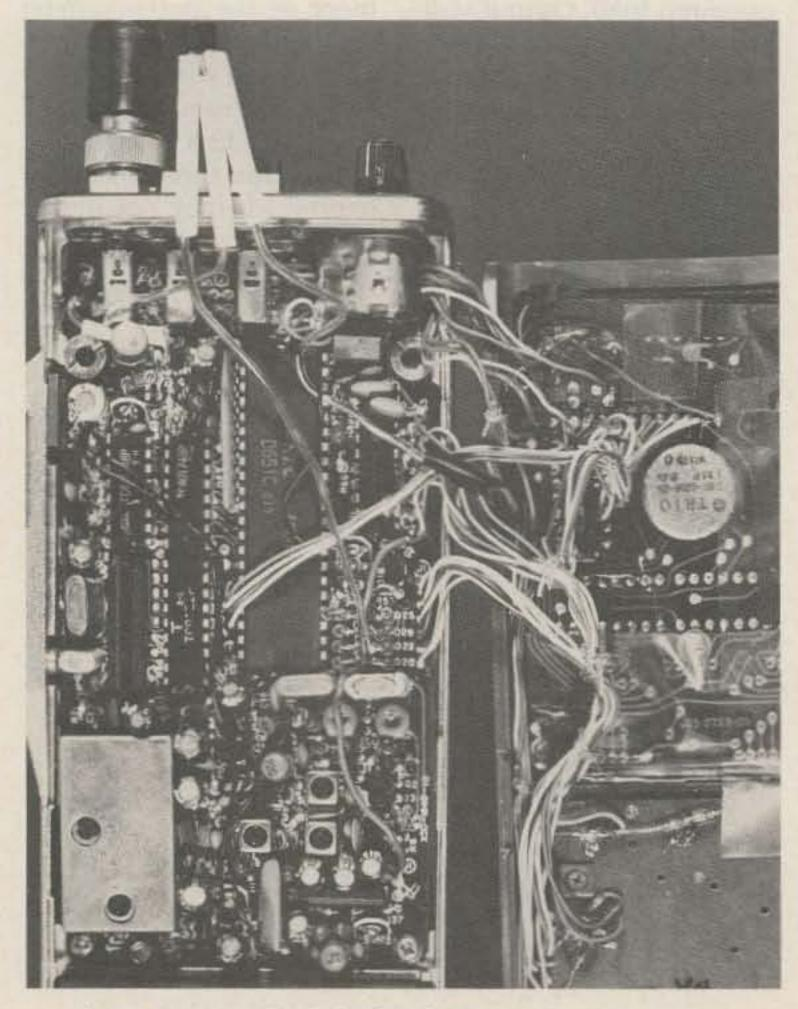
Photo A. Tape all of the leads to avoid a short circuit.
