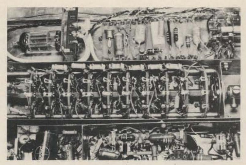
Photo B. View of the filter from the bottom of the receiver. Coupling capacitors and loading resistors are mounted directly on the switch decks.
