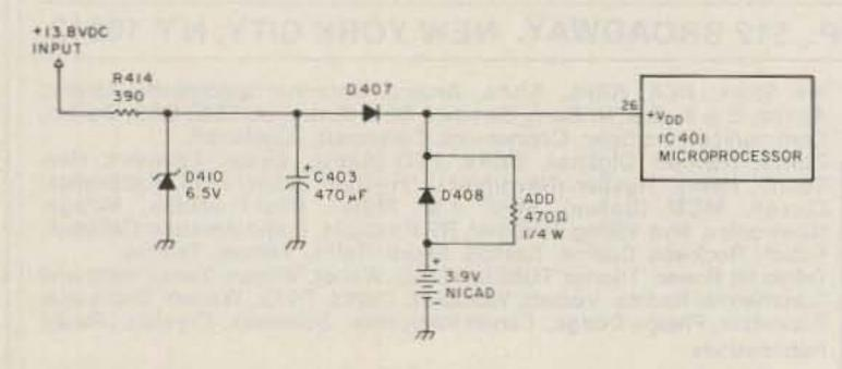
Fig. 2. Modified memory-protection circuit uses a three-cell nicad pack instead of the silver-oxide cells. Adding a 470-Ohm resistor across D408 allows the nicad pack to charge whenever the radio is operated.
