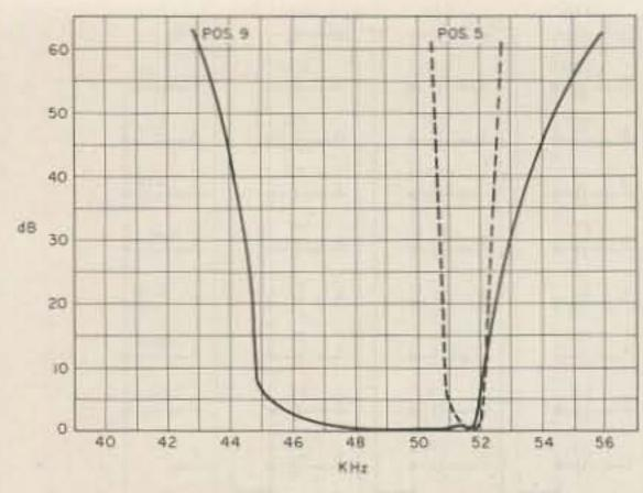
Fig. 4. Measured filter response in switch positions 5 and 9. Response continues beyond -60 dB, but this could not be measured with the simple test equipment at PAØSE.
