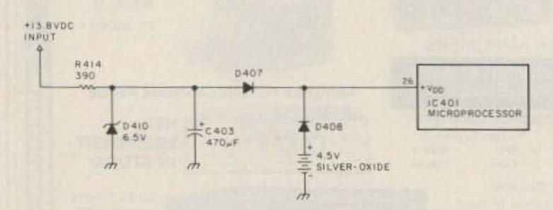
Fig. 1. Original memory-protection circuit uses three silver-oxide cells and charge-protection diode D408 to apply power to the microprocessor while the main power is off.
