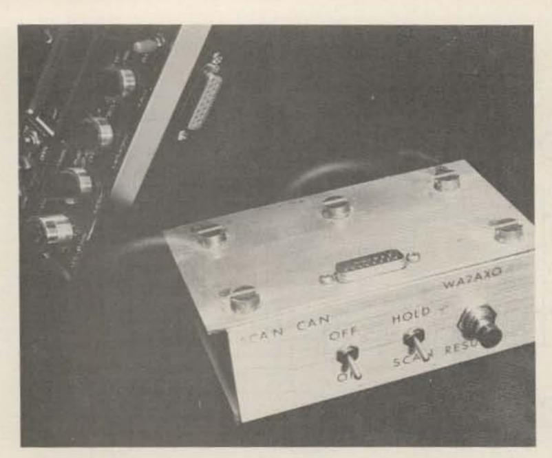
Photo C. View of the underside of the KDK. Note the positions of the connectors on the two units and the magnets.
