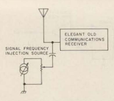
Fig. 9. Signal-frequency injection technique for SSB reception using an older receiver. The signal-frequency source is adjustable in frequency and in amplitude.
