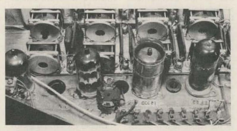
Photo A. The filter mounted in PA@SE's homemade hamband receiver.
