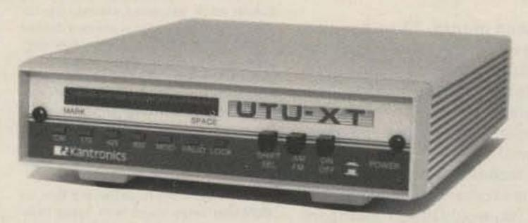
UTU-XT is also compatible to any computer with an RS232 or TTL (C-64) serial port — the circuit is built in. This allows you the flexibility to change computers at any time.
