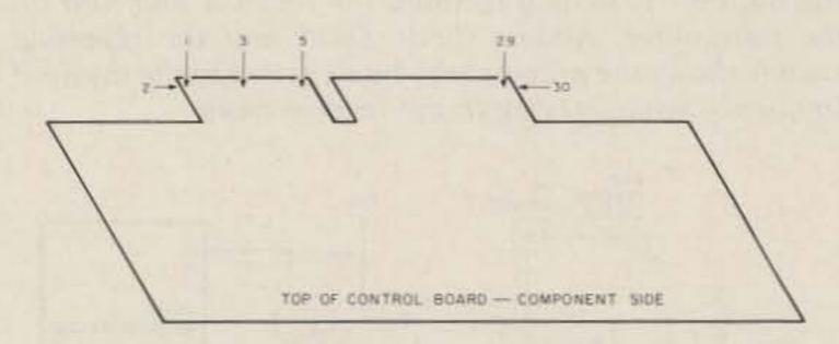
Fig. 4. Numbering sequence for control-board card-edge connector. Odd numbers are on top; even numbers are on the solder side.
