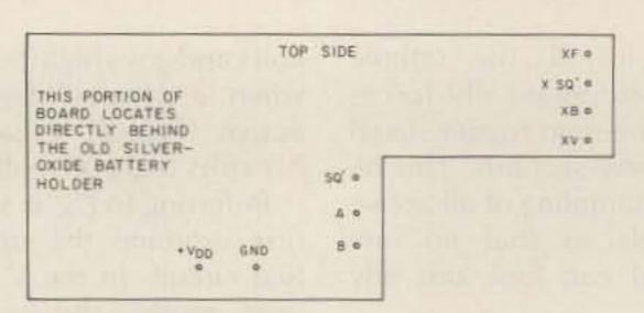
Fig. 10. Constructing the new scan-control circuits on a board this size and shape will allow them to fit neatly inside the control head between the control board and the potentiometer mounting board. The board is shown here as it would be viewed looking from the front of the Azden, down through the existing control board.
