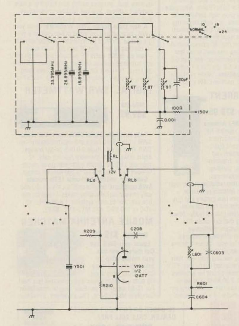
Fig. 1. Modified hho circuit of the HW-101. Third-overtone crystals are used, inductances wound on 7mm formers with turns spaced the diameter of the wire.
