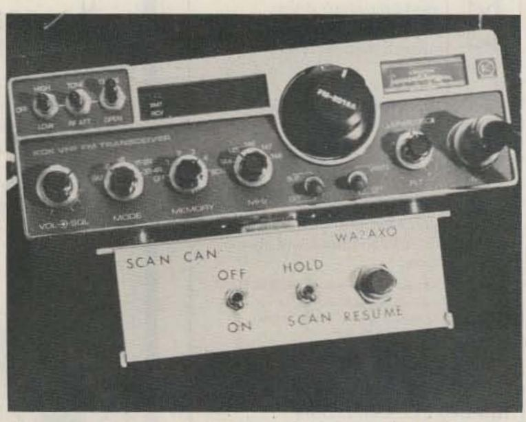
Photo B. The Scan Can mounted in operating position on the KDK.
