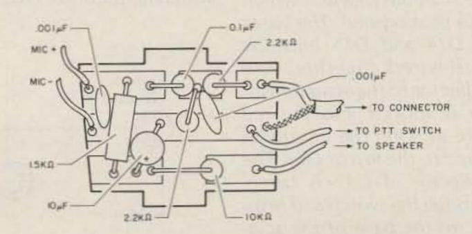
Fig. 3. Parts placement, external microphone.
