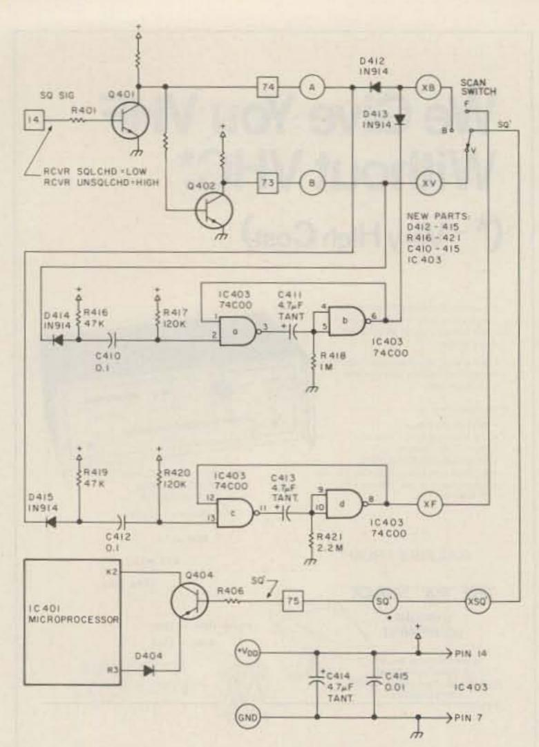
Fig. 9. Scan-control circuits after modification. Numbers in squares refer to existing control-board pin or pad gates such as the CD4011 pins were limited to levelnumbers. Numbers in circles refer to inputs and outputs on the new board. IC403A and B and IC403C and D are wired as monostable multivibrators triggered by D414 and D415, respectively. Squelch activity enters through pin 14, upper left. Scanning is stopped while Q404 is turned on; it resumes when turned off, lower left.
