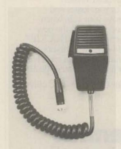
Photo A. Completed speaker/ microphone. The mike cartridge is the dark circle in the white strip in the middle of the microphone.
