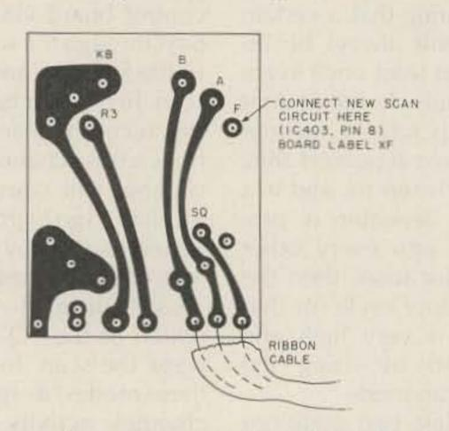
Fig. 11. Rear view of scan-mode switch showing point of connection from new scan circuit.
