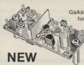
GaAsFET Preamps with features similar to LNG, except designed for LOW COST and SMALL SIZE: only 5/8 W x 1-5/8L × 3/4H. Easily mounts inside many radios.
