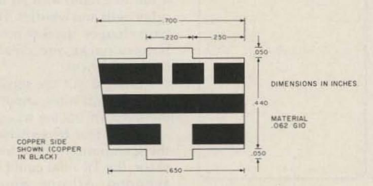
Fig. 2. PC board, external microphone.
