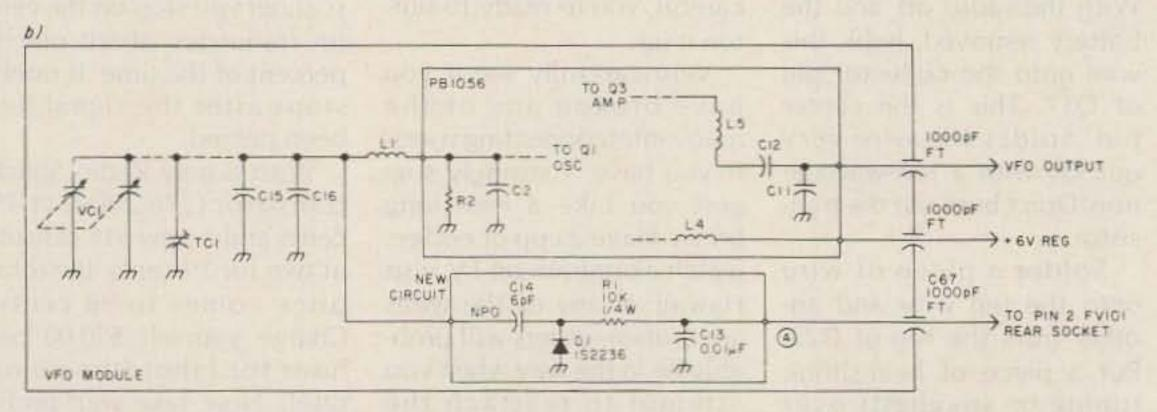
Fig. 1. Partial schematic drawings of FV-101 vfo before (a) and after (b) modification to include RIT circuitry. Components on the added board are indicated in (b).
