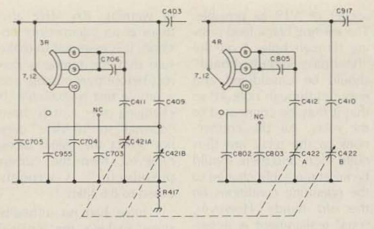
Fig. 2(a). Tuned circuits (inductors omitted) of driver input and output before modification.
