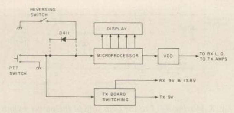
Fig. 5. Engaging the PTT switch causes the microprocessor to change the vco to the transmit frequency and causes the transmit switching to mute the receiver and turn on the transmitter. Adding diode D411 and the reversing switch allows the processor to be switched to the transmit frequency while staying in the receive mode.
