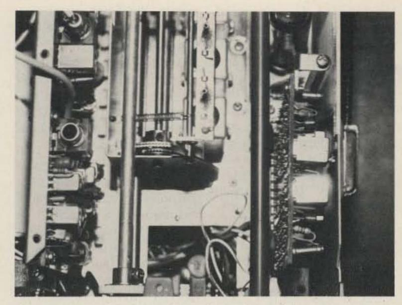
Photo C. The local board on the right and the premix board on the left, near the front of the FT-101Z.
