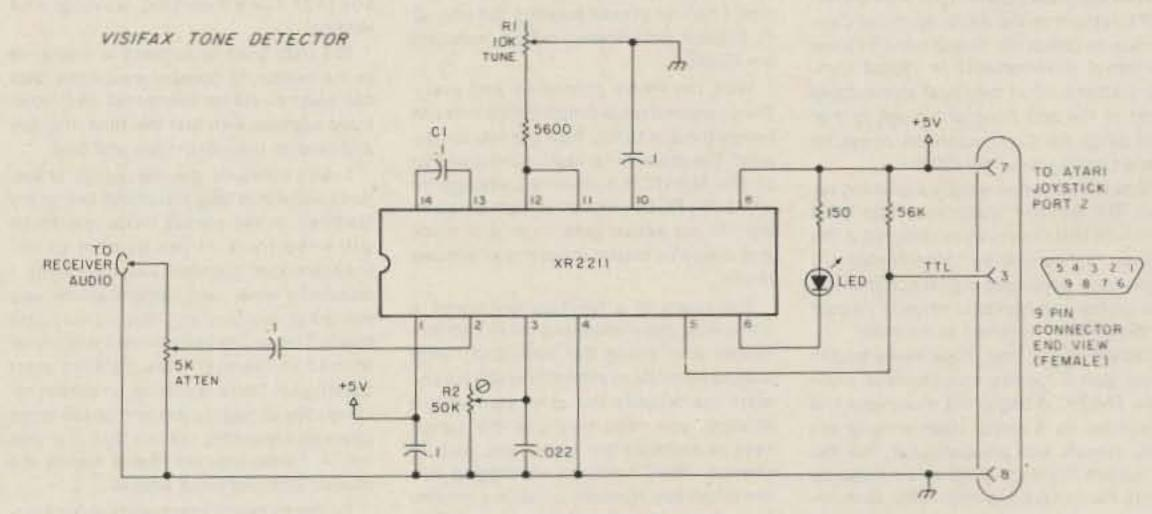
Fig. 1. Tone-detector schematic.
