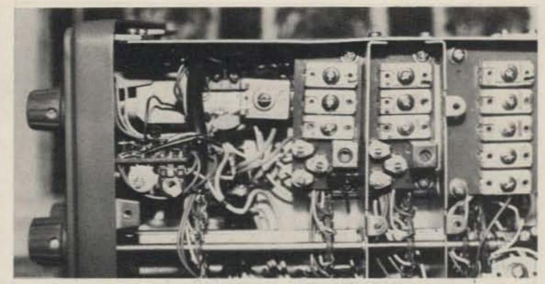
Photo D. The new trimmer capacitor may be soldered directly to the trimmer unit A circuit board.
