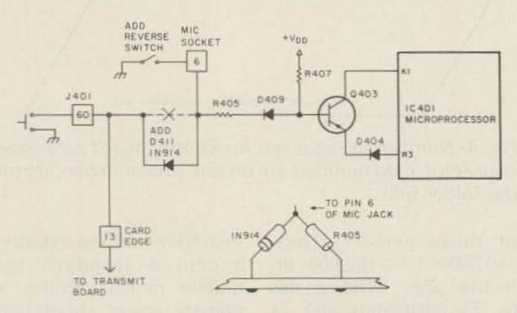
Fig. 6. Reversing switch is mounted in the microphone case. Lift one end of R405 and add D411 as shown.
