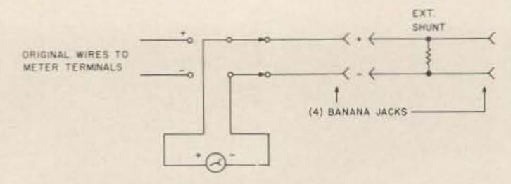
Fig. 3. Milliammeter circuit.
