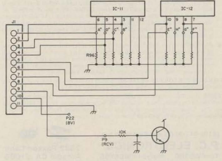
Fig. 2. The Scan-Can-to-KDK interface.
