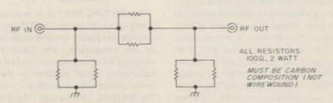
Fig. 1. A simple attenuator for padding down 10-Watt exciters to drive transverters.
