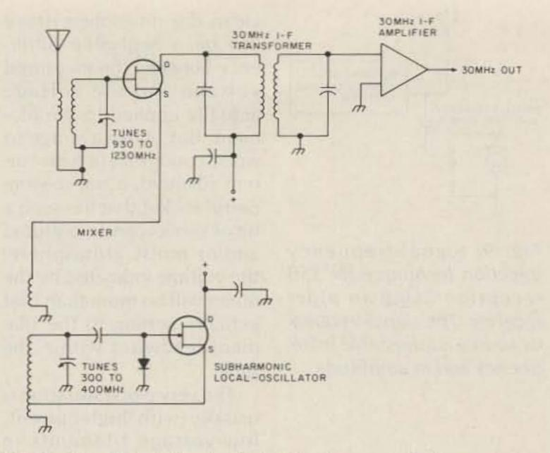
Fig. 7. Simplified circuit of the "business end" of a superhet, with subharmonic oscillator. Contrary to common assumption, the oscillator does not provide harmonics of its fundamental frequency. Rather, the needed frequency multiplication takes place in the mixer.
