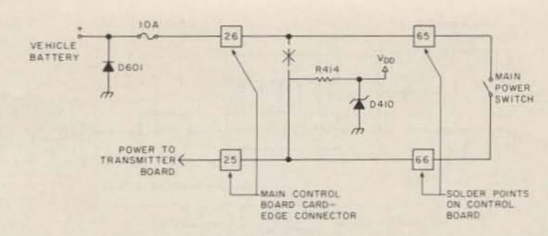
Fig. 3. Moving R414 to the cold side of the power switch eliminates current drain from the vehicle battery when powered off.
