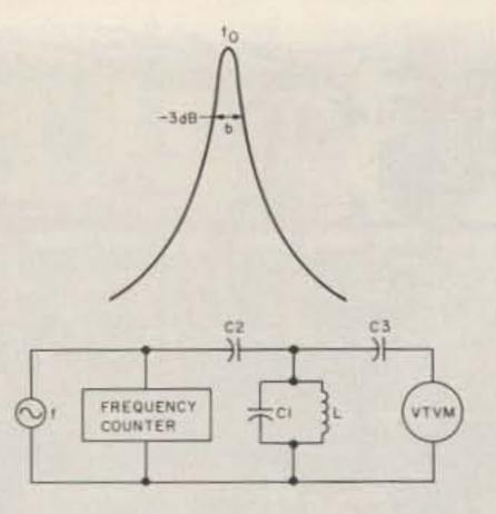
Fig. 2. How unloaded quality factor Qo is measured.
