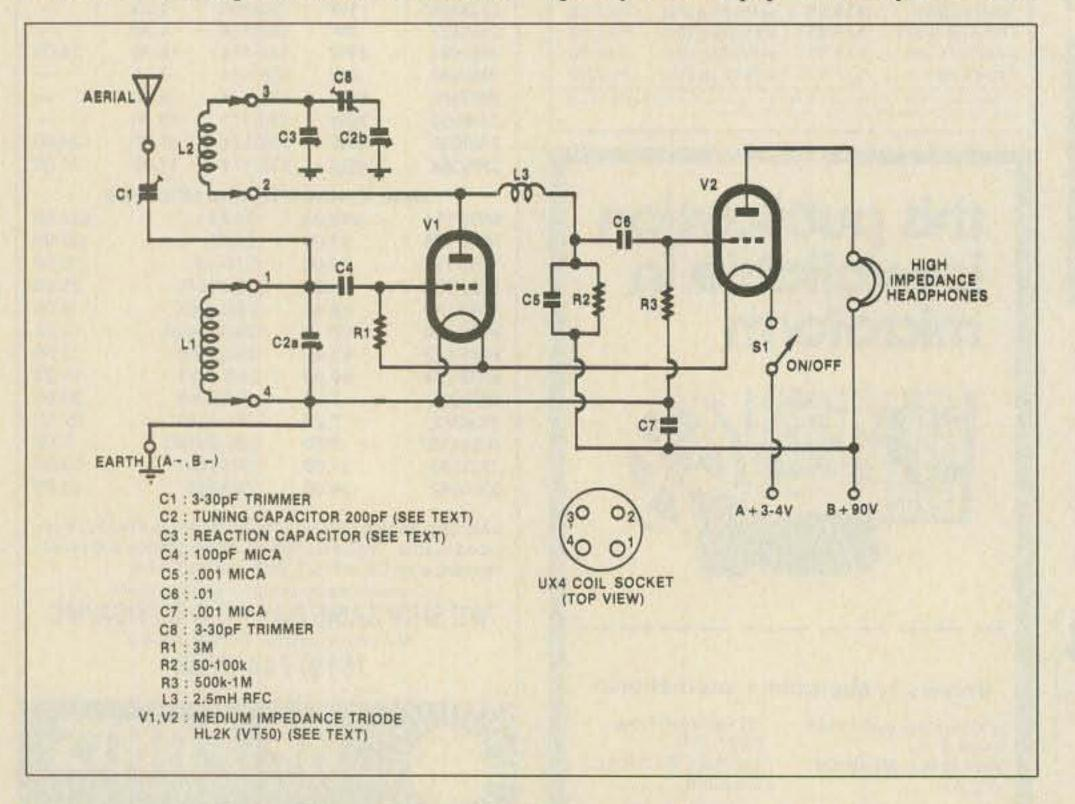
Fig. 1. Schematic diagram of the Reinartz all-wave receiver.
