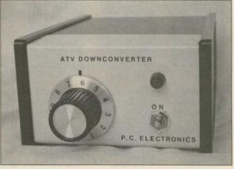
900-MHz ATV downconverter available from P.C. Electronics.
