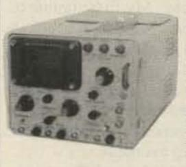
OS-106/USM-117 PORT-ABLE SCOPE, rugged military DC to 6 MHz unit with MX-2996 high-gain plug-in. Sweep 0.1 us to 0.1 sec in 19 steps. Sensitivity 0.01 to 20 V/div in 11 steps. 115 VAC 60 Hz; 8.5 × 9.8 × 15, 20 lbs
