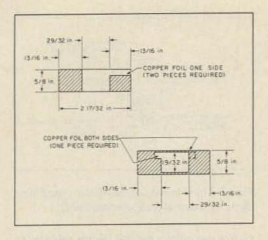
Fig. 2. Plates for 50-pF capacitor assembly.
