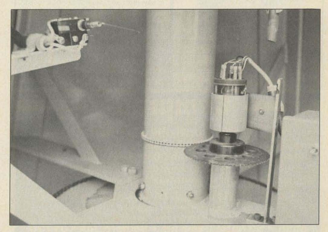
Photo D. The reduction gear mechanism for driving the selsyn direction indicator. A limit switch is visible at upper left. (Photo by KT2B.)
