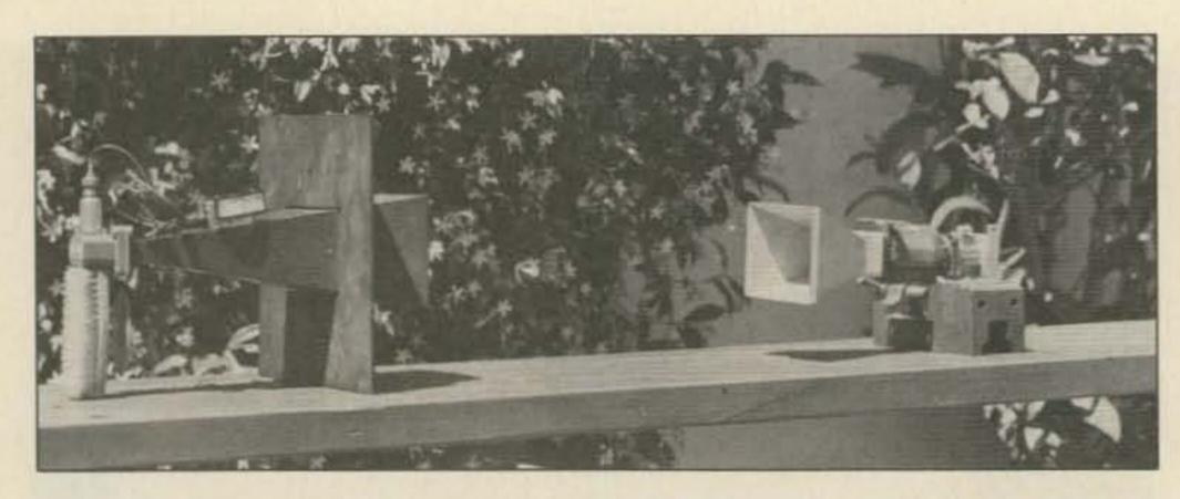
Photo C. Horn-antenna test adjustment range. A suitable distance would be 10-20 feet for small horns.
