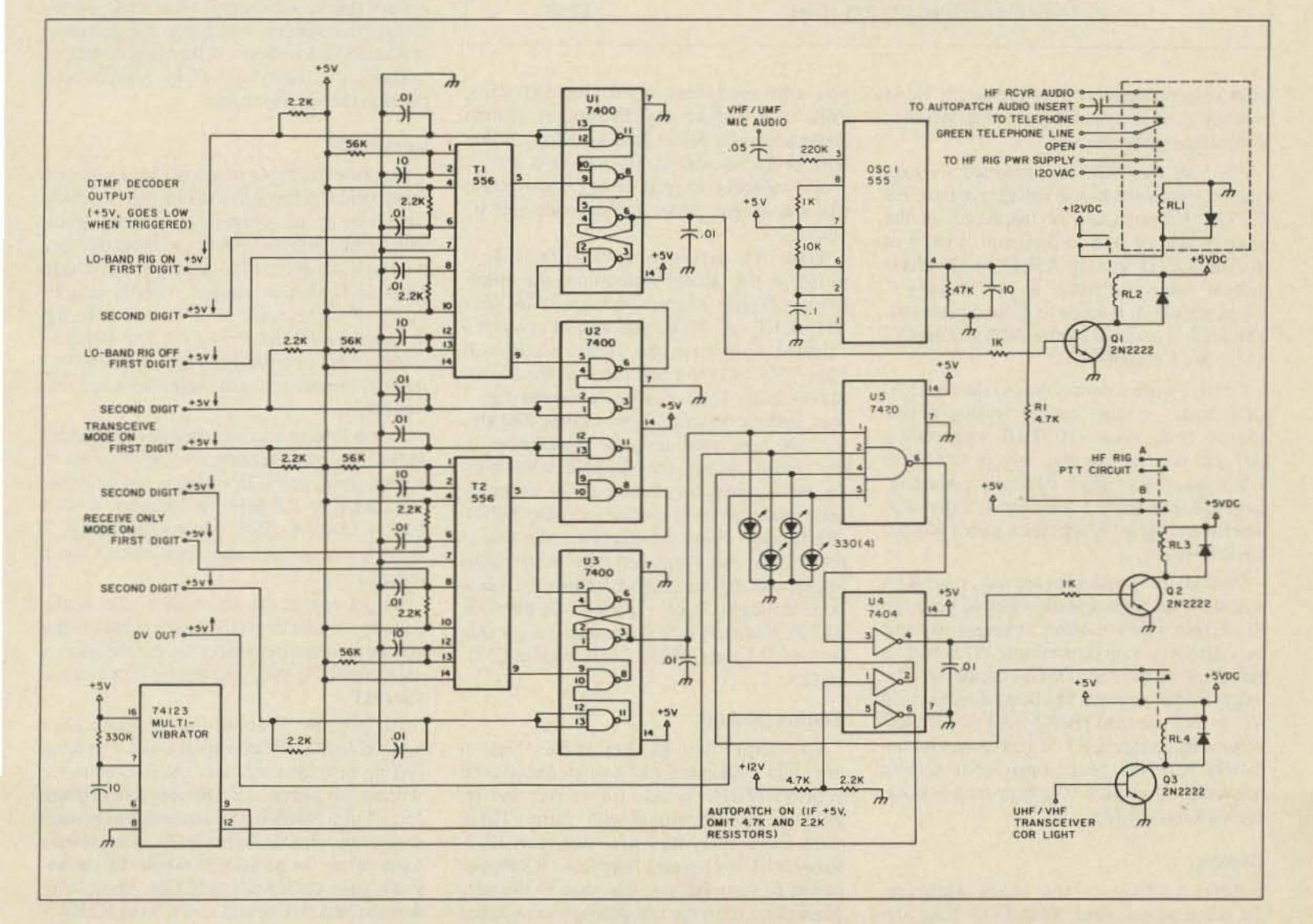
Fig. 2. Schematic of the WB2REM low-band link.
