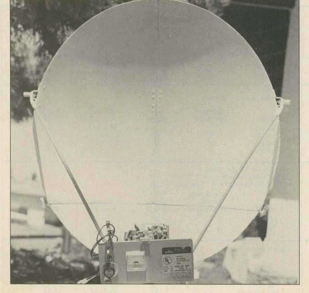
Photo A. Off-center-feed 10-GHz dish with original transceiver mounted at focus. Used for Mount Soledad to Mount Helix contacts.
