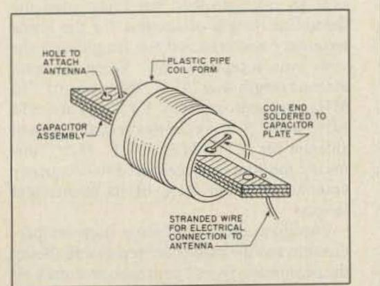
Fig. 4. Trap assembly.
