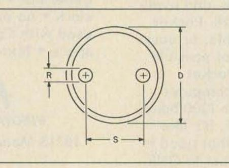
Fig. 2. Shielded parallel line.
