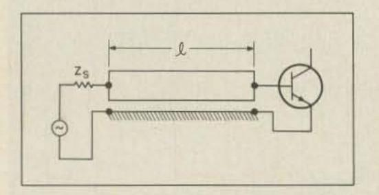
Fig. 5. Schematic representation of a microstrip transmission line.
