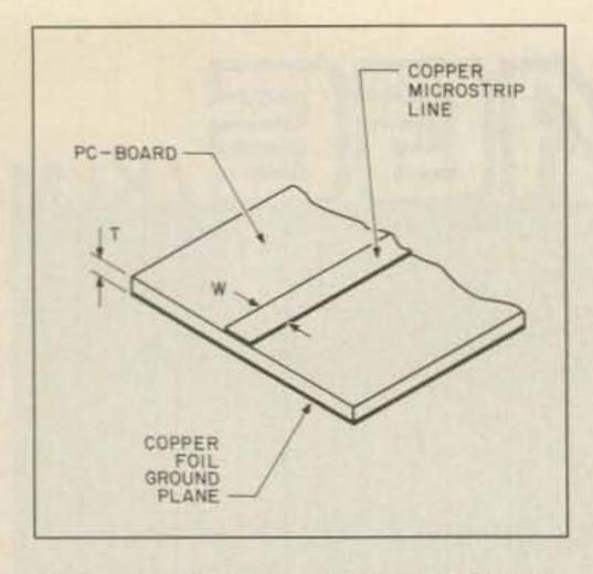
Fig. 4. A common microstrip configuration.
