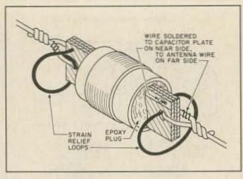
Fig. 6. Connecting the trap to an antenna.
