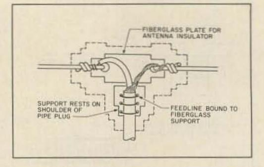
Fig. 7. Interior view of the plastic pipe fitting showing antenna feedpoint assembly.
