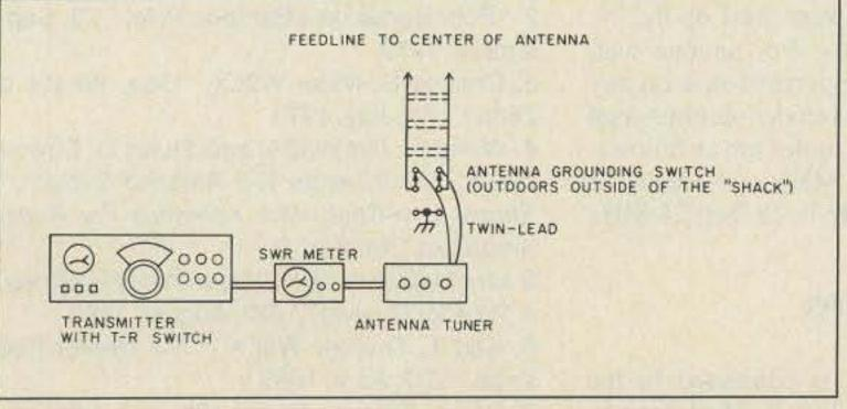
Fig. 4. The antenna system's connections to the transmitter.
