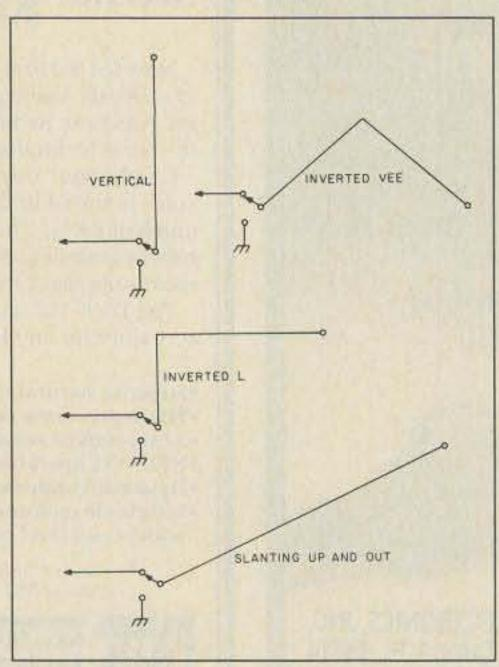
Fig. 3. Some endfed-antenna configurations.
