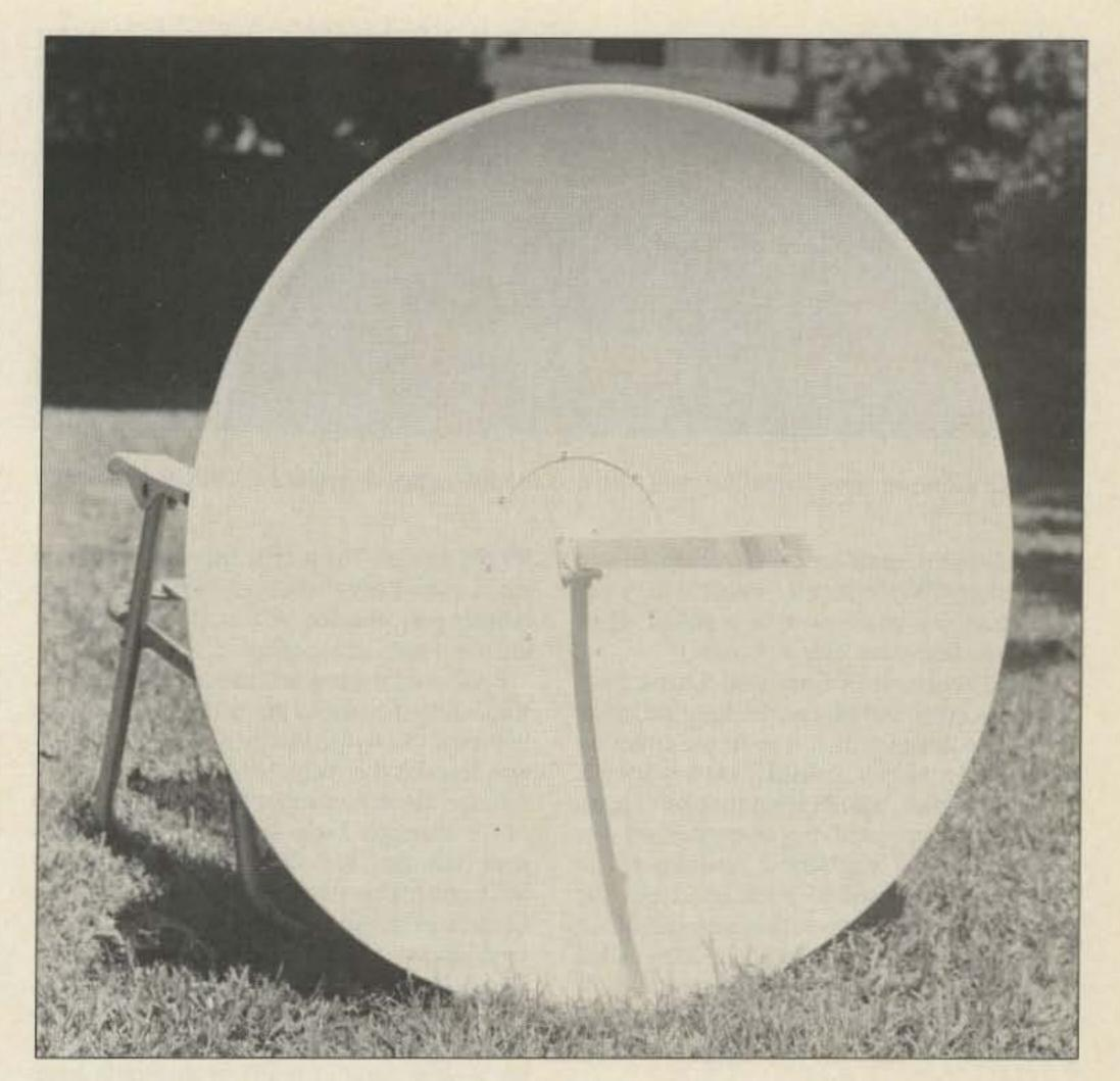
Photo B. 10-GHz dish antenna with dipole feed and dielectric resonator (plastic bag) in place.
