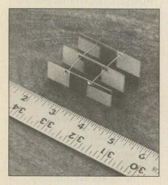
Photo A. Capacitor assembly strung on jumper wires; ready to be glued together.
