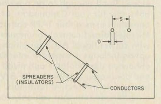
Fig. 3. A parallel feeder.
