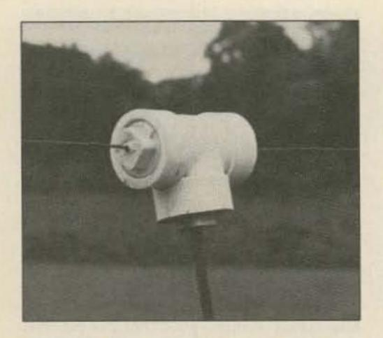
Photo E. Feedline protection using plastic pipe fitting.
