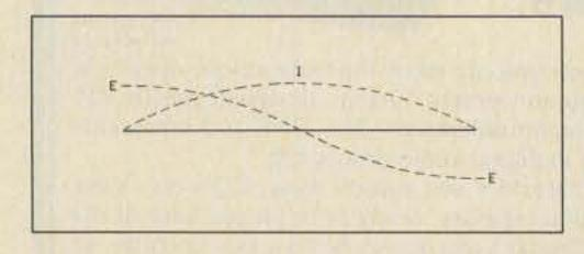
Fig. 1. Rf voltage and current distribution on a half-wave resonant antenna.
