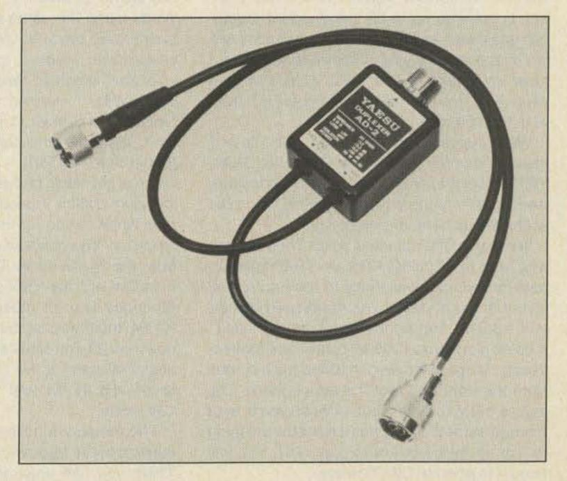
FT-2700RH/FT-726R duplexer allows use of single VHF/UHF antenna. 73 Amateur Radio • September, 1986 21
