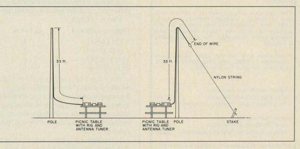
Fig. 6. Twenty-meter vertical resonant-wire antennas.
