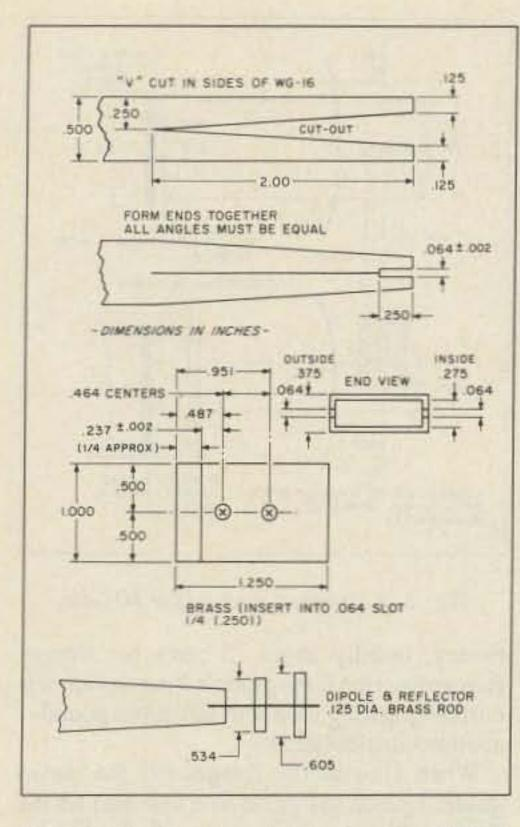
Fig. 1. Construction details for the 10-GHz dipole feed.
