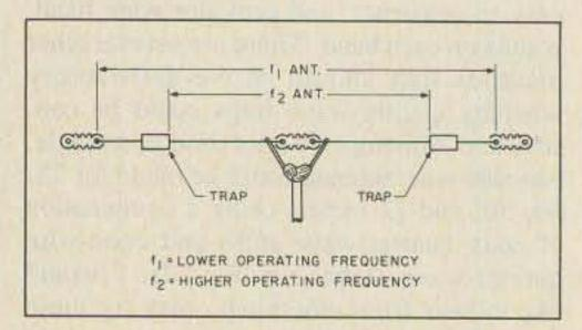
Fig. 1. Trap-tuned dipole antenna.
