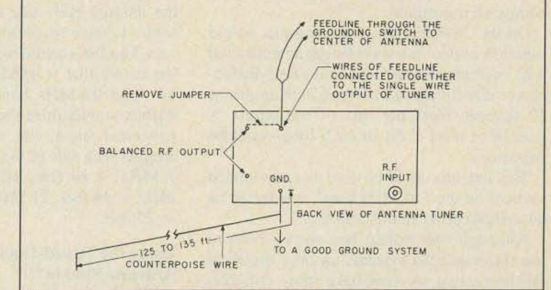
Fig. 5. Connections for using the antennas as top-loaded vertical antennas.
