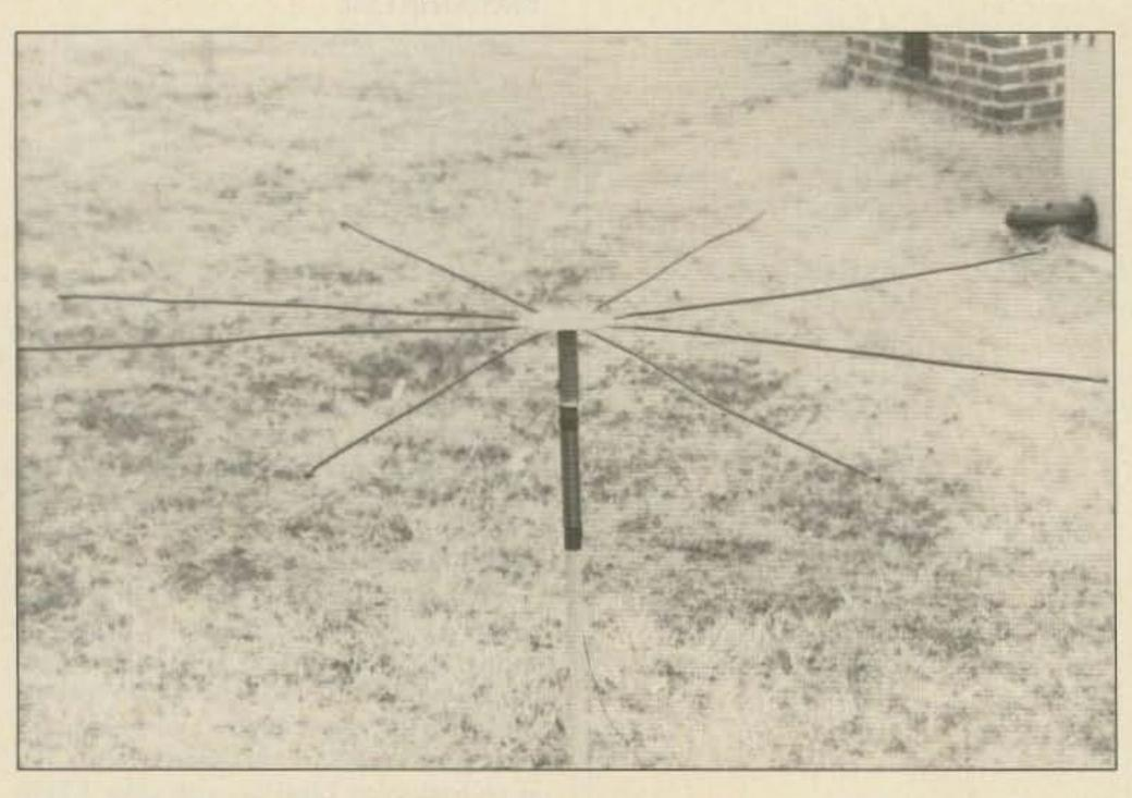
Photo A. Bird's-eye view of the quarter-scale top hat and loading coil.
