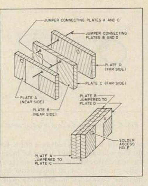
Fig. 3. Capacitor assembly detail.
