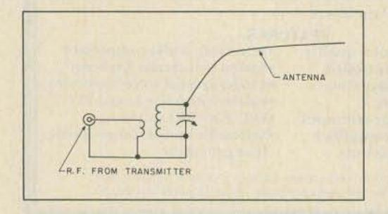
Fig. 2. Feeding rf voltage to the end of a resonant antenna (parallel-tuned coil to give rf voltage).
