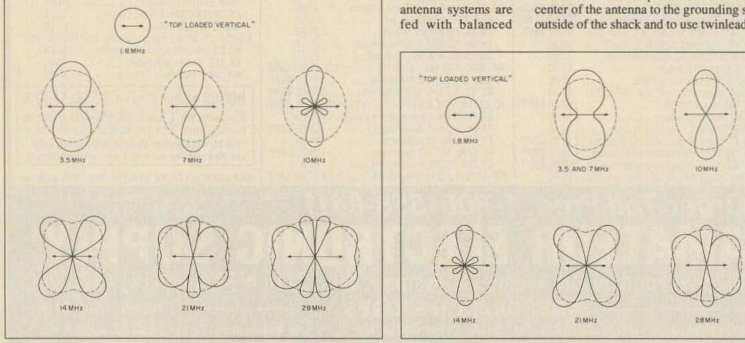
Fig. 1. Approximate directional patterns for antenna number one (66 feet each side of the center). The dotted lines show the patterns when the antenna is in the form of an inverted vee.
