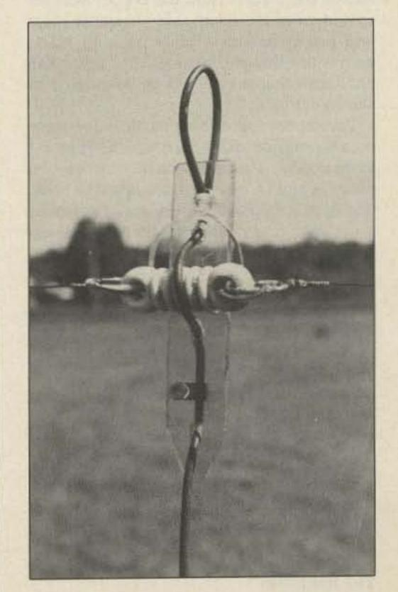
Photo D. Feedline protection using the PY8ZAC/W8VOH method.
