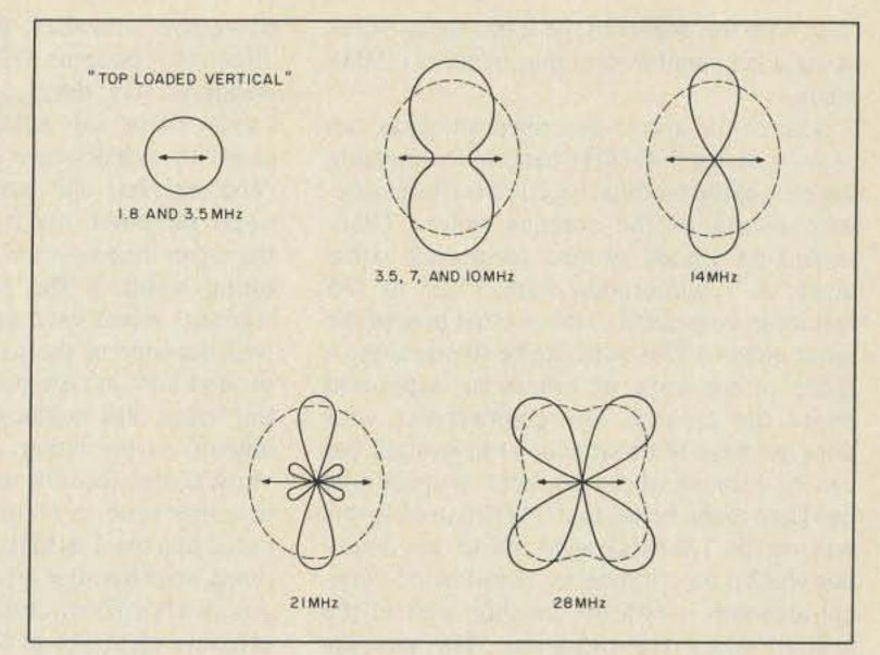
Fig. 3. Approximate directional patterns for antenna number three (33 feet each side of the center). The dotted lines show the patterns when the antenna is in the form of an inverted vee.
