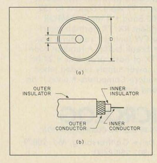
Fig. 1. Coaxial cable. 36 73 Amateur Radio • September, 1986 We frequently bandy about the "impedance" of transmission lines. We refer to 52-Ohm or 75-Ohm coaxial cable, for example. Just what is this impedance? Note that two terms are used for transmission-line impedance: characteristic impedance and surge impedance. As far as I can tell from my literature search, they are the same and so will be used as such here.
