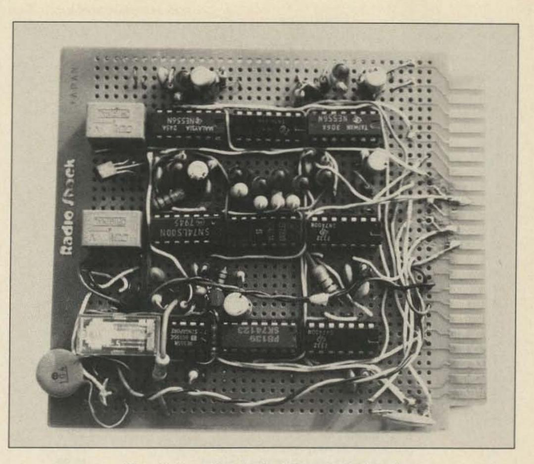
Photo A. A complete simplex link on one tiny board.
