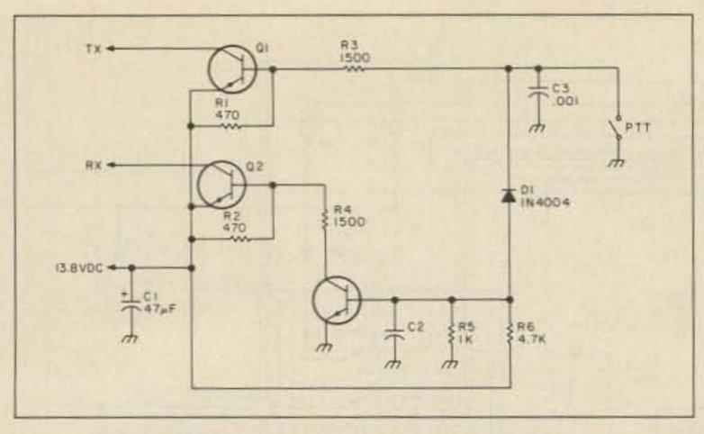
Fig. 5. Complete TX/RX voltage switching circuit.
