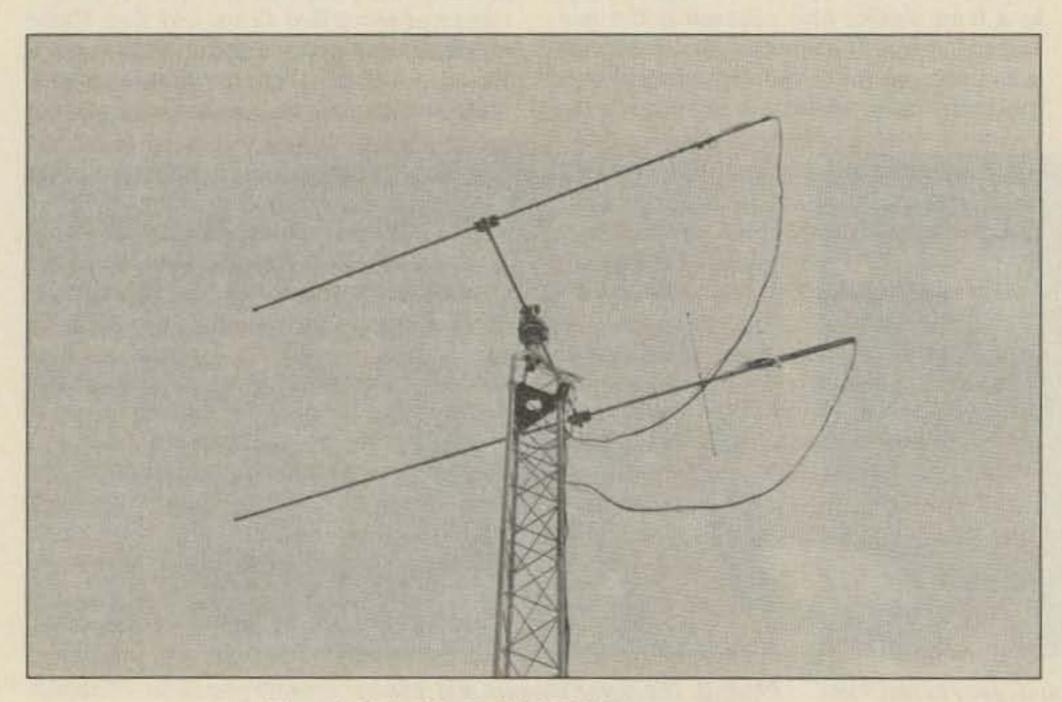
Photo A. Telex/Hy-Gain's OSCAR antenna system.
