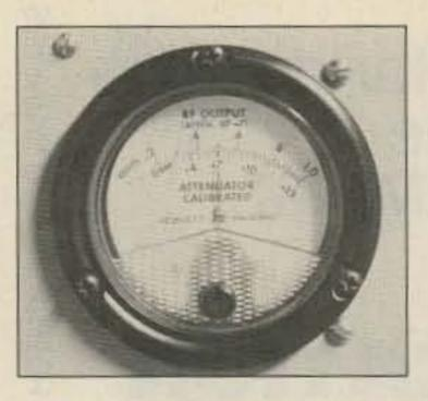
Photo C. Close-up of leveling indicator on HP-608F. Output will remain constant from 10 MHz to 450 MHz.
