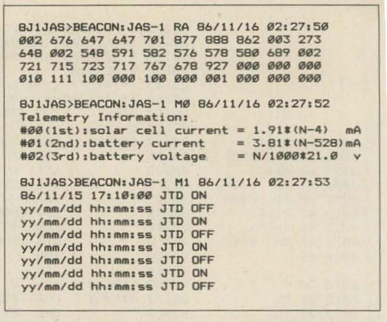
Fig. 1. Fuji-OSCAR 12 telemetry and information received from the digital beacon. AX.25 protocol with PSK modulation.
