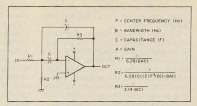
Fig. 2. Layout and design equations for a single-stage active-bandpass filter. Three such stages are used in the interface circuit.
