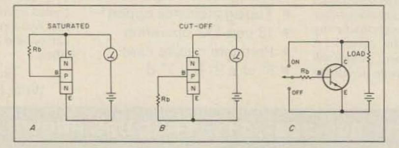
Fig. 1. Transistor saturation (a) and cut-off (b) make the device useful as a switch. The circuit in (c) is a simple way to switch a load on and off.
