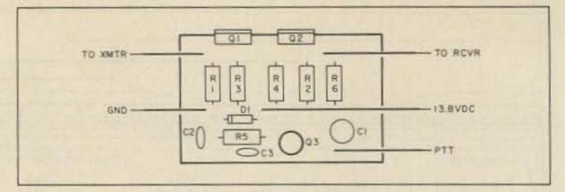
Fig. 6. Parts placement diagram for the switch.
