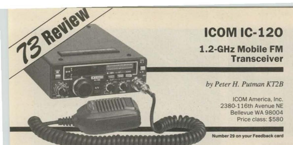
COM of America has been making great strides toward a full product line of UHF radio equipment in recent years. Along with their IC-1271A (reviewed in September, 1986), ICOM also offers the IC-120, a mobile, 1-Watt, synthesized transceiver for the 1260-1300-MHz range.
