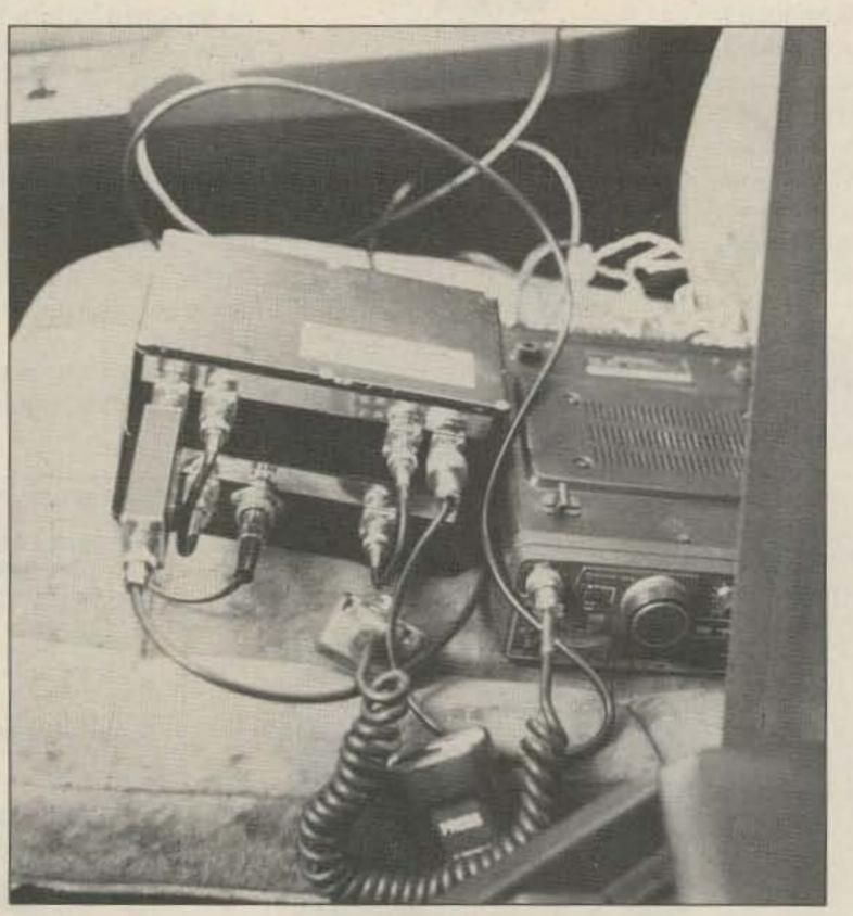
Photo B. The companion setup on 1296-MHz FM-an MMT-1296/144 and TR-9000 exciter. A Larsen antenna was also used here.
