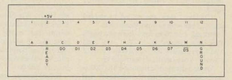
Fig. 3. Rear-view connector to VIC-20 user I/O port.
