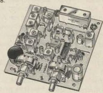
R144/R220 FM RCVRS for 2M, 150–174, or 220 MHz. 0.15uV sens, 8-pole xtal & 10 pole ceramic i-f filters, helical resonator front end for exceptional selectivity. > 100dB at ± 12kHz (best available anywhere!) Flutterproof squelch. AFC tracks drifting xmtrs. Xtal oven avail. Kit \$138, w/t \$198.
