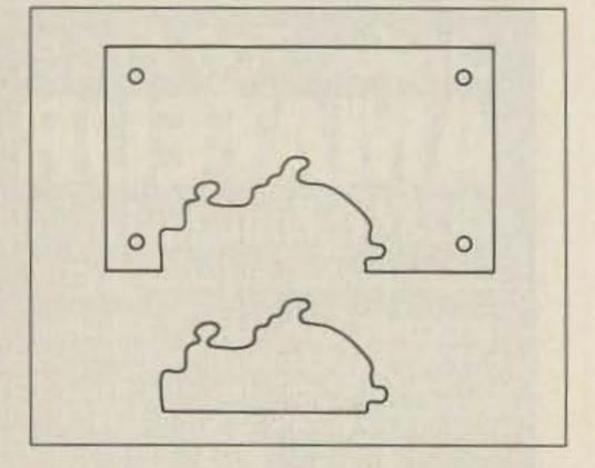
Fig. 1. Patch for a damaged circuit board.
