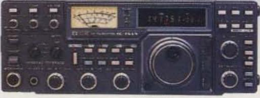
one year warranty. There's more! The IC-751A's receiver boasts 105dB dynamic range for superb listening. The 100% duty cycle transmitter defies abuse and delivers 100 watts of exceptionally stable and clean RF output. Reliability. Quality. One year warranty. That's ICOM.
