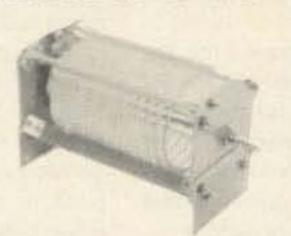
High quality roller inductor used in 1 KW HF transmitter; 21 non-linear turns of 0.25" silver-plated ribbon which forms 4.75"Lx3.63" dia coil, approx. 21 UH. Fiberglass end-plates; shaft 1"Lx0.375" dia. 0/a 8.75x4x5, 3 lbs sh. Harris #938-0505-001, NEW.....\$45.00
