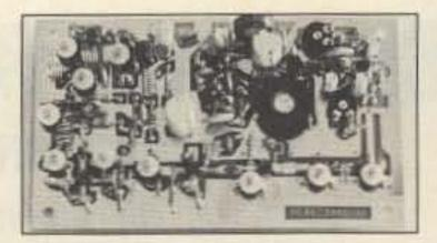
The TXA5-33 exciter/modulator board for the 33-cm ATV band.
