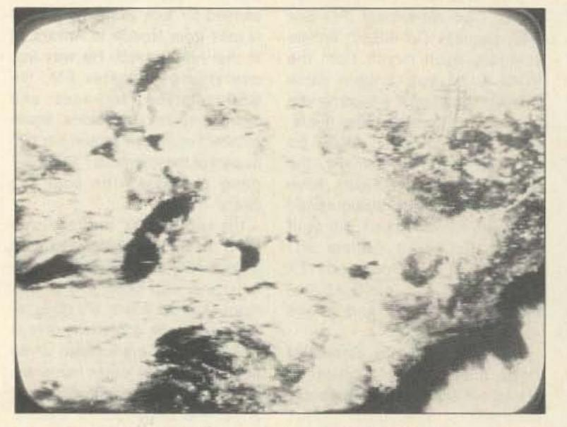
Photo A. The default full-frame display of a METEOR 2-15 pass obtainable with any CoCo model using the 120-lpm mode. Michigan and the Great Lakes are near the center of the image, the East Coast is angling upward in the lower right, and most of the upper half of the picture shows Ontario and Quebec.
