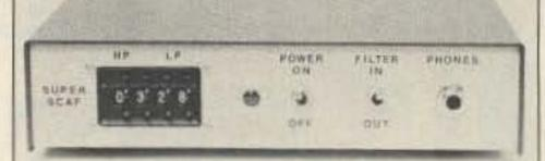
SuperSCAF is an innovative, high performance audio filter. SuperSCAF incorporates state-of-the-art switched capacitor filter technology to achieve unprecedented receiver selectivity and unwanted signal and noise rejection. Upper and lower passband cutoff frequencies are digitally programmed via front-panel thumbwheel switches at increments of approximately 100Hz between 200 and 3900 Hz...
