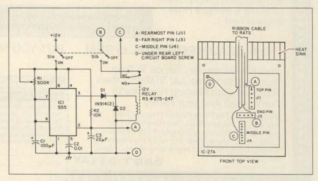
Fig. 1. Schematic and connections for RATS, the resume-after-transmit scanner.
