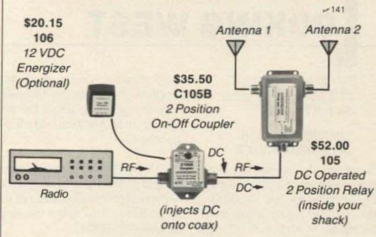
This system operates from 1.5 to 180 MHz and handles 1250 RF watts.
