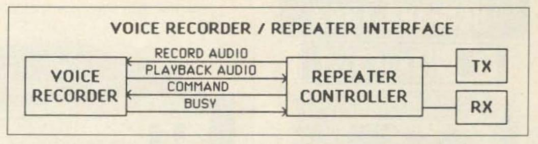
Fig. 4. Voice-recorder/repeater interface.
