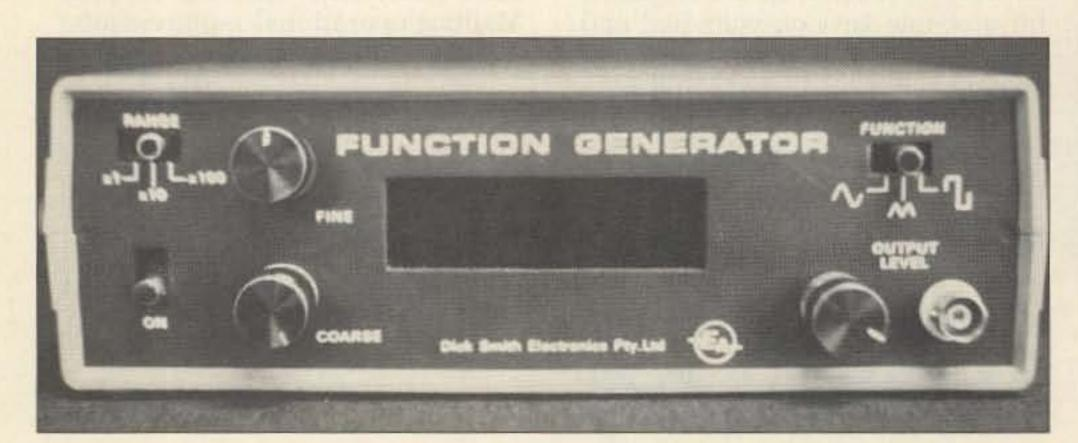
Photo A. Front panel of the Dick Smith Electronics Function Generator.
