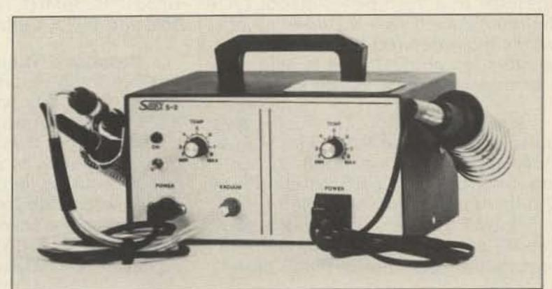
The Sibex S-2 temperature-controlled soldering/desoldering station.
