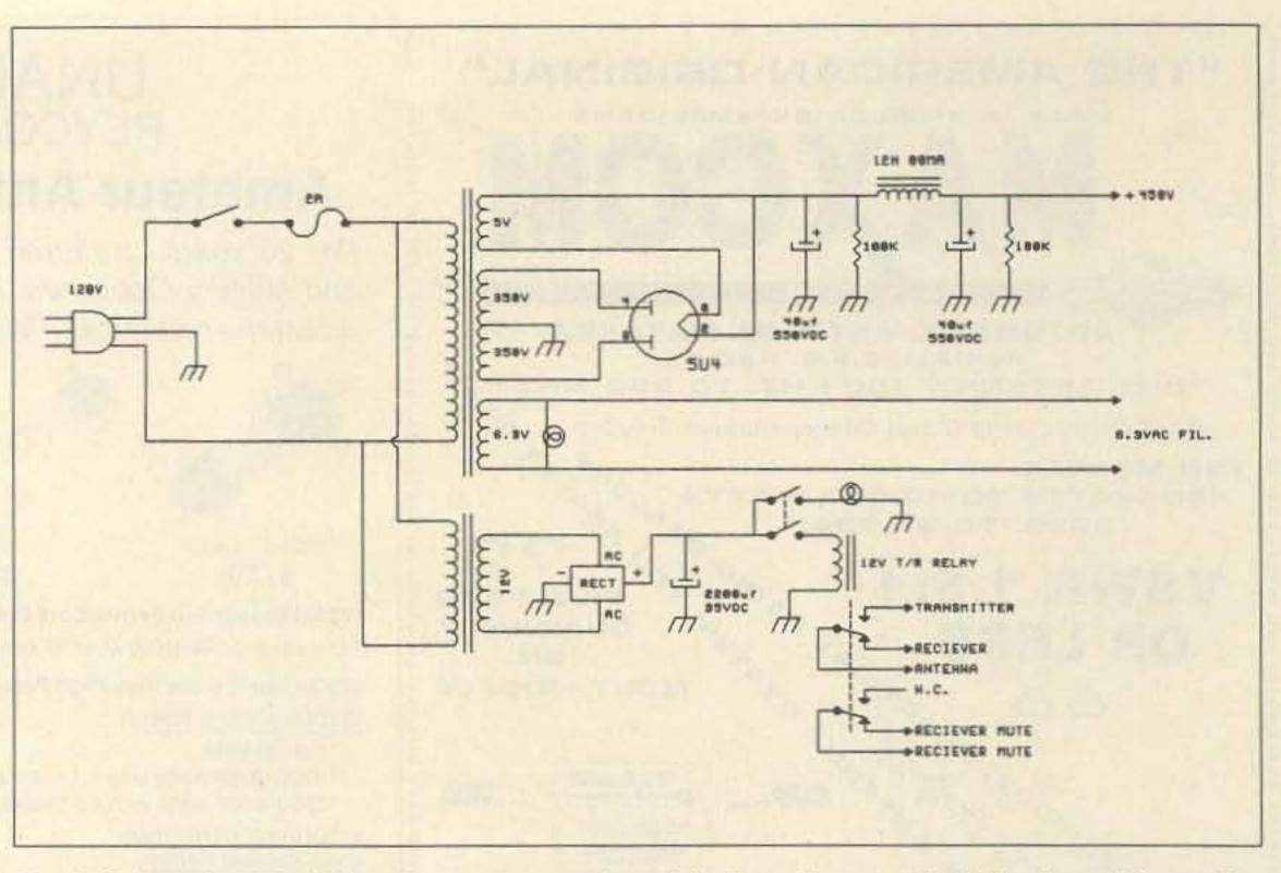
Fig. 2. Schematic of the high-voltage power supply and the low-voltage supply. Relay is used for receiver muting and antenna switching.
