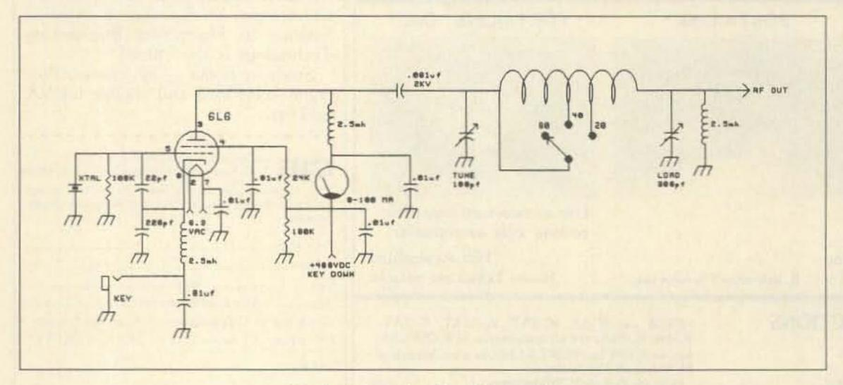
Fig. 1. Schematic of the 6L6 Special.
