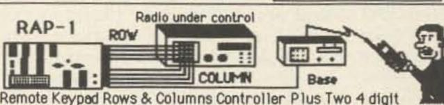
Remote Keypad Rows & Columns Controller Plus Two 4 digit decoders (on/off)/Will control frequency of any keypad entry radio such as the Kenwood 7950/2530/ICO4-AT. Easy to install in parallely with existing keypad/Use with ComShack 64 as a freq. controller or with Pro Search rotor control box/A versatile board for all remote control applications. The latches may be used for on/off or momentary.
