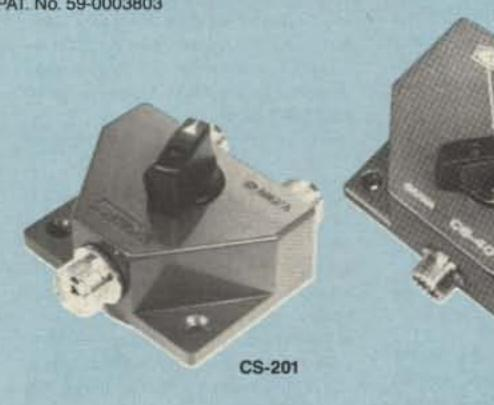
CS-4 CS-401G CS-201 CS-201G CS-401 4 Position 4 Position 4 Position 2 Position 2 Position 1.5 GHz 1.3 GHz 800 MHz 800 MHz 500 MHz Frequency: **BNC** type SO-239 N type SO-239 N type Connectors: +60 dB +50 dB +50 dB +60 dB +60 dB Isolation: 500 W PEP 2.5 kW PEP 2.5 kW PEP 2.5 kW PEP 2.5 kW PEP Power Rating: 1 kW CW 250 W CW 1 kW CW 1 kW CW 1 kW CW
