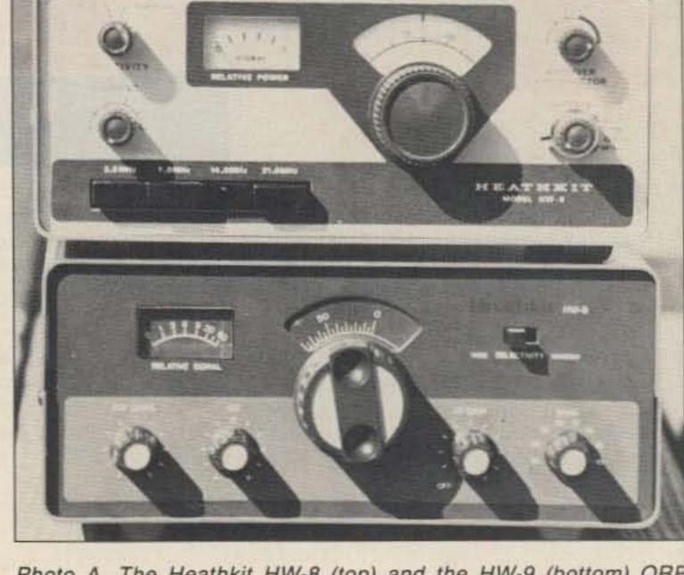
Photo A. The Heathkit HW-8 (top) and the HW-9 (bottom) QRP transceivers.
