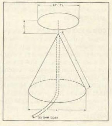
Fig. 6. Discone antenna. L = wavelength/4 (free space) at lowest operating frequency. S = 1-6 inches.
