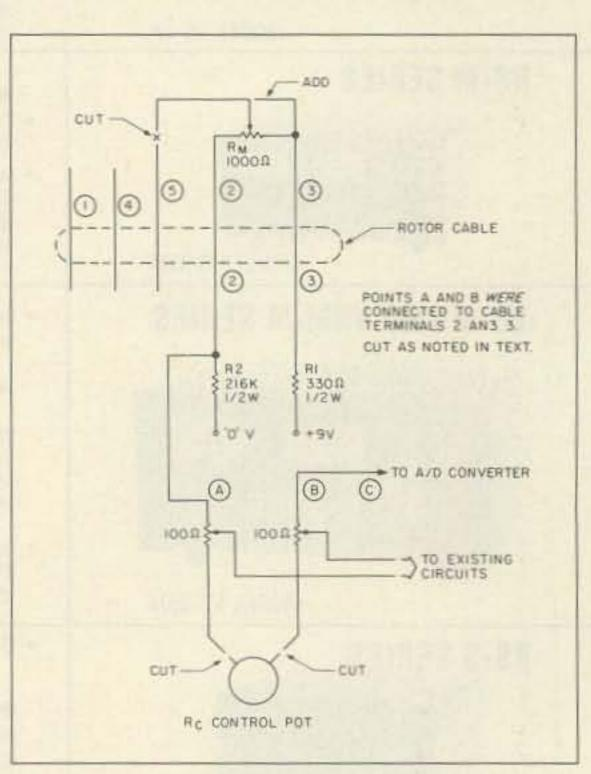
Fig. 3. The new bridge circuit.
