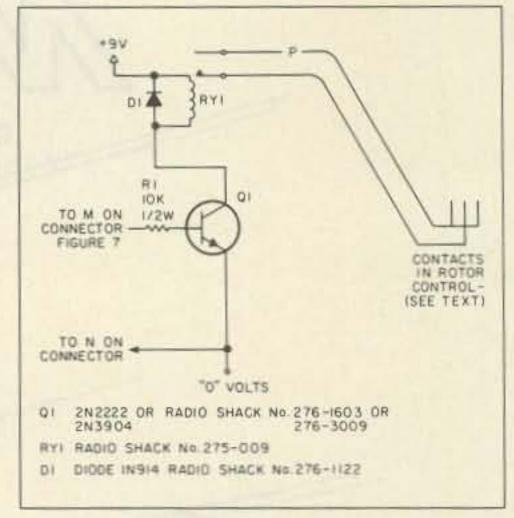
Fig. 8. Relay circuit to maintain current to rotate the rotor until the bridge circuit is balanced.
