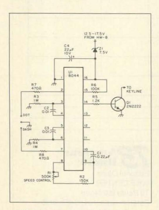
Fig. 1 Schematic for the Cubic-inch Keyer.
