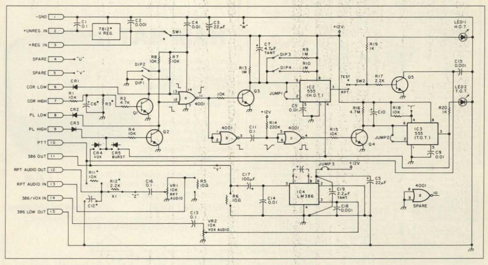
Fig. 1. Schematic for the repeater controller board.
