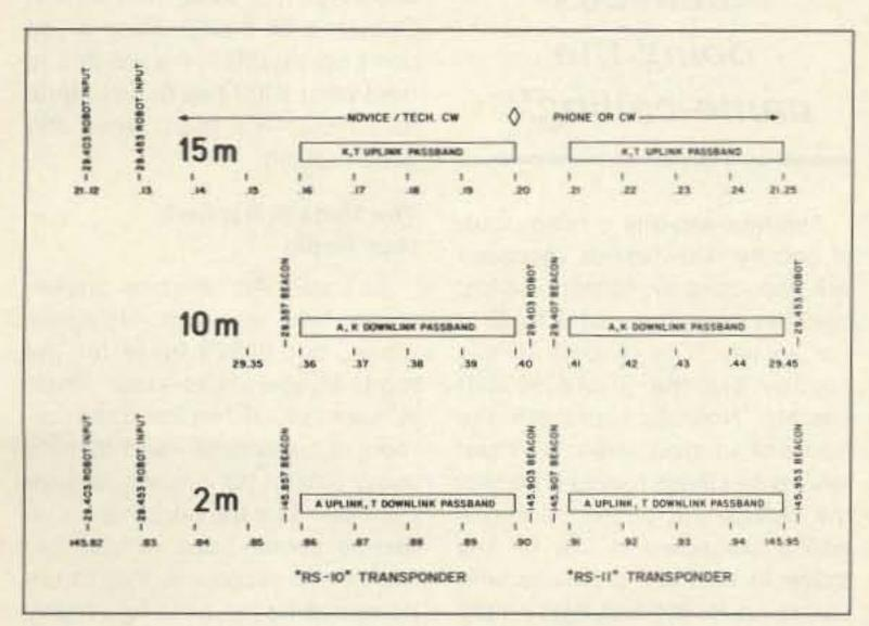
Fig. 1. Frequency chart for RS-10 and RS-11.
