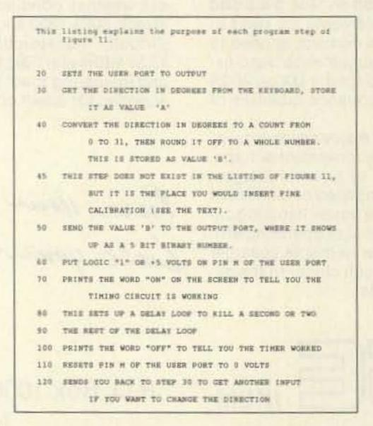
Fig. 10. Program flow, in BASIC, for the VIC-20.
