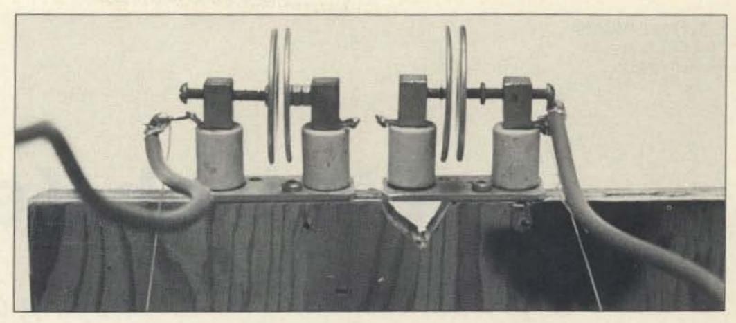
Photo C. Tesla primary spark gap setup as described in text.
