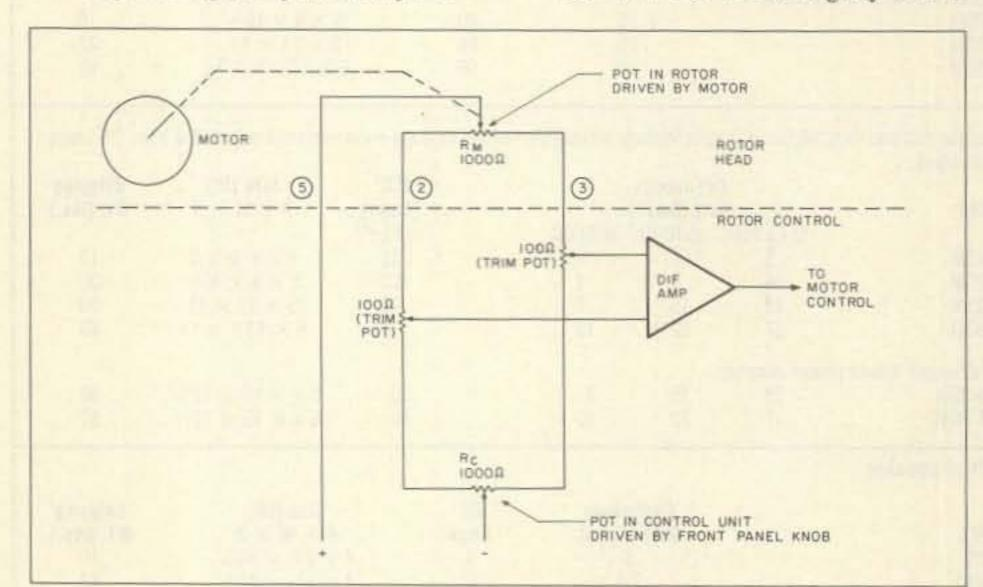
Fig. 2. Basic circuit of the five-wire connected rotor.
