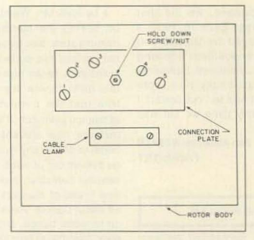
Fig. 4. The connecting rotor terminal board.
