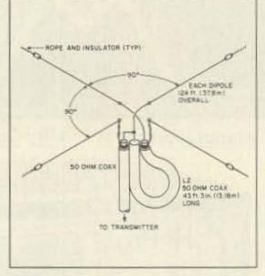
Fig. 2. The 80m wideband antenna at ZS6ZO. Two dipoles spaced 90 degrees apart are fed 90 degrees out-of-phase with an electrical quarter-wavelength interconnecting line. Shields of lines are all soldered together at dipole feedpoint and connected to adjacent antenna sections.
