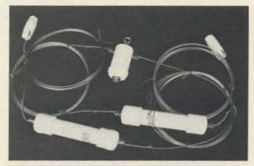
The Spi-Ro multi-band trap antenna.
