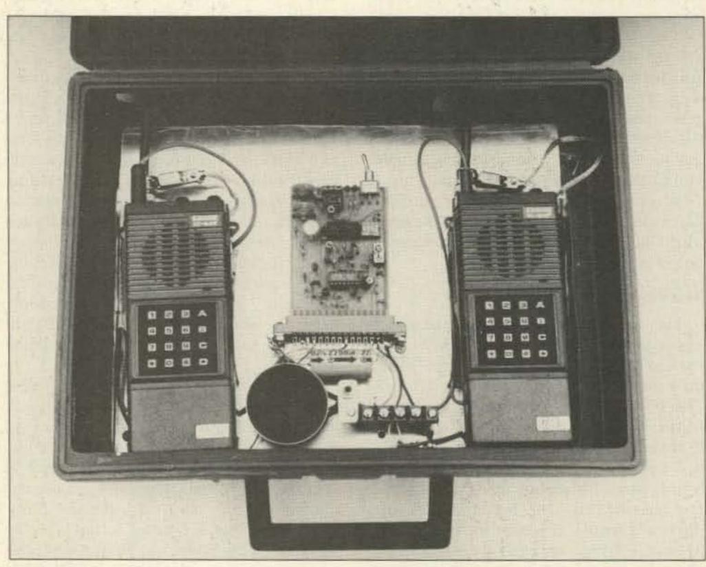
Photo A. Repeater controller PC board with 2 ICOM 4ATs in a portable repeater package, mounted on an aluminum plate.
