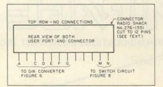
Fig. 7. Pin wiring.
