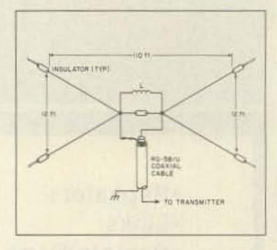
Fig. 4. Broadband fan dipole for 80m. Wires may be either in the horizontal or vertical plane. The inductive reactance (X<sub>L</sub>) is 64 Ohms. At 80m, L = 2.7 uH; this is achieved by winding 8-1/2 turns of #12 wire around a 2"-long, 2"-diameter tube.
