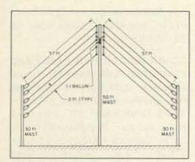
Fig. 5. W7IS's 80m wideband dipole.
