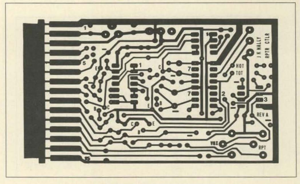
Fig. 3. Positive of circuit board layout.
