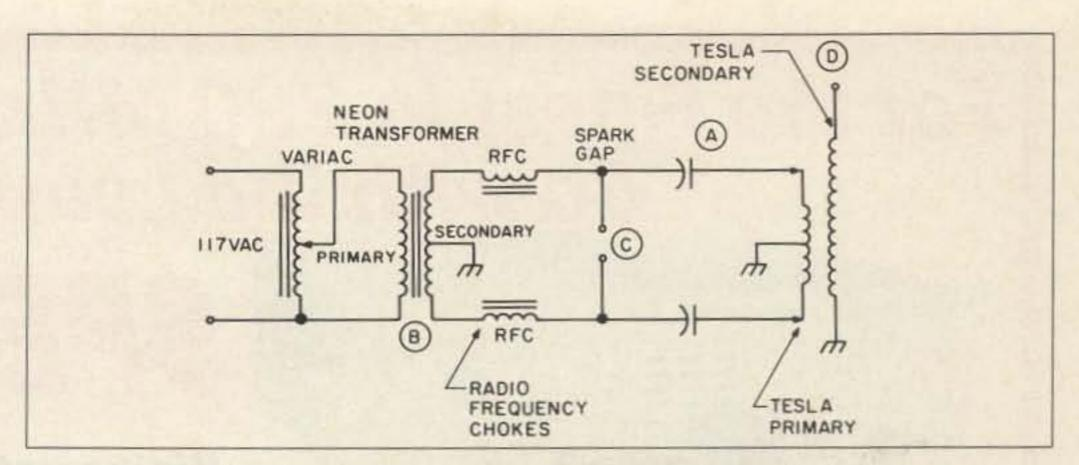
Fig. 2. Construction diagram for the Tesla high-frequency transformer.
