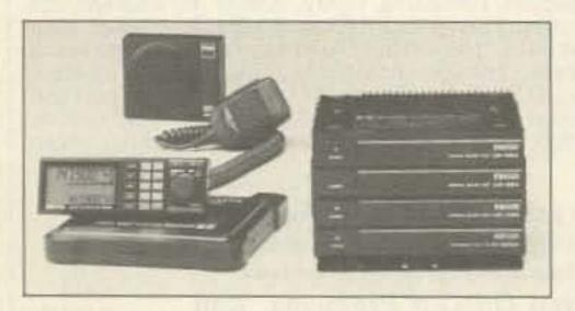
ICOM's IC-900A VHF/UHF mobile transceiver.
