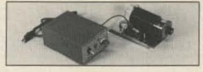
designs use high frequency crystals with ICs that divide the frequency to come out at the desired frequency. Most use power FETs, such as the IRF series or the VN types, as a final amplifier. When using ICs, the only coil normally required is the antenna loading/coupling coil. This coil should have a high "Q." Most Lowfers use Litz wire for the coil.
