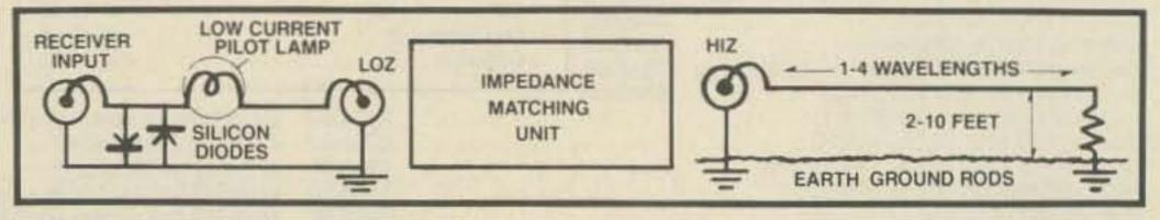
FIG. 1: Front end protection circuit and beverage receiving antenna for low frequency DX'ing.
