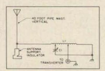
Figure 5. The author uses this antenna configuration, which allows operation on both 160 and 1750 meter bands. selected to resonate the antenna at the desired frequency, using C1 for additional flexibility. Again, erect the antenna as much in the clear as possible.
