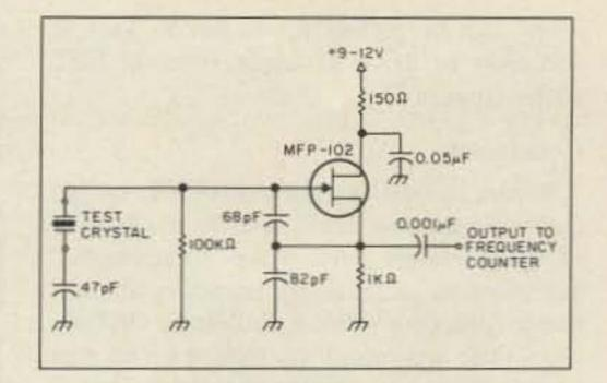
Fig. 2. Test oscillator for characterizing surplus crystals.
