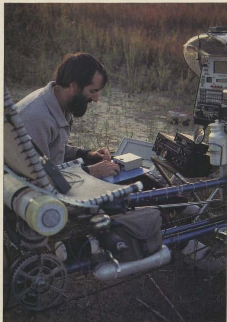
include a pair of 2-meter rigs, a 10-meter handheld, a full HF QRP system, and a packet station complete with mailbox software for unattended operation.
