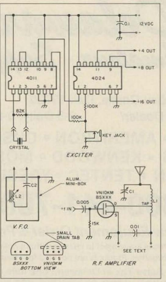
Figure 1. Medium frequency transmitter. NOTE: All resistors are ¼ watt rating and capacitors, 50 volts.
