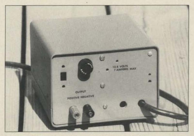
Photo D. Fuse in foreground is for the primary of the transformer. 73 Amateur Radio • February, 1988 81
