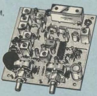
•R451 UHF FM RCVR. Similar to above. Tuned line front end, 0.25uV sens. (0.1uV with optional hel. res. preamp). Kit \$149, w/t \$229.
