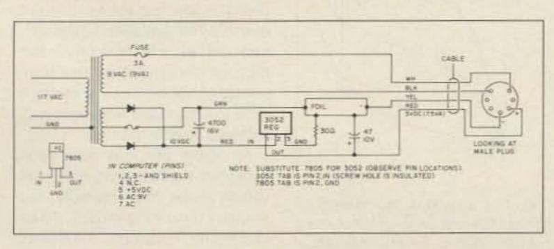
Figure 1. Power supply schematic for Commodore 64.
