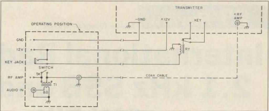
Figure 3. Remote control wiring. RY... 12 volt DC relay with normally closed contacts (SPDT can be used) T1... Audio output transformer.
