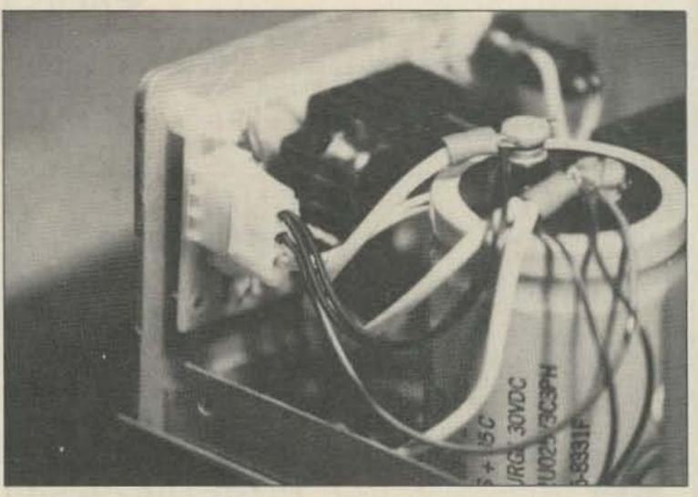
Photo B. Inside the supply. Note the Molex connector for input and output connections. Filter capacitor in foreground.
