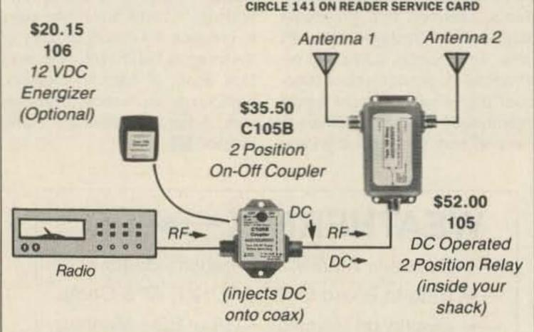
This system operates from 1.5 to 180 MHz and handles 1250 RF watts.
