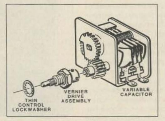
Fig. 1. The position of the vernier drive assembly.
