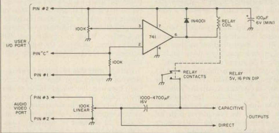
Fig. 2. Schematic for the audio/video port interface. Ludvigson does not supply this interface.
