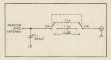
Figure 4. A simple random wire antenna tuner used for reception. Figure 4 shows a simple tuner that works well for general listening using a wire antenna from 50 to 200 feet in length. The coil is
