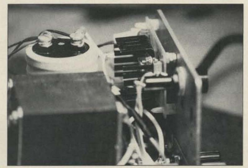
Photo C. Rear view of the supply. The extra hole is for a battery charging option.
