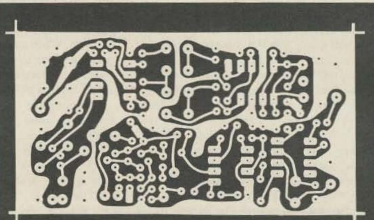
Figure 6. Printed circuit board negative for the 20 meter receiver.
