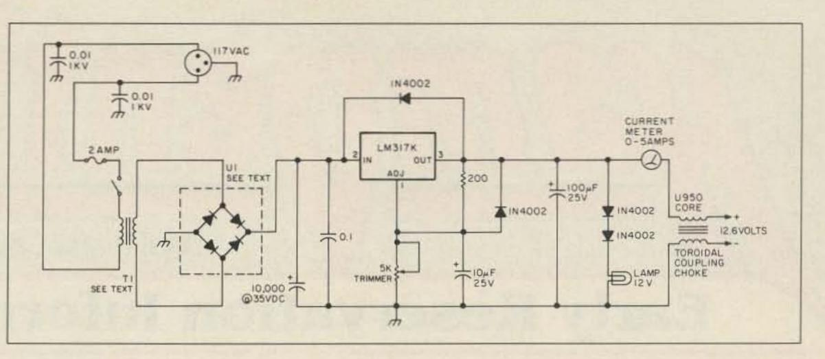
Figure 1. The schematic for the power supply. The core for the filter on the output can be just about anything. Use a large toroid or a ferrite rod.
