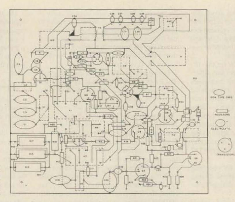
Figure 3. Parts placement for the transverter. A circuit board and parts kit are available. See text for details.
