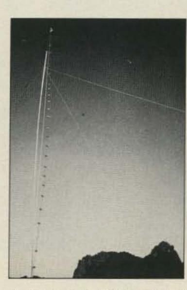
The homemade G5RV multiband antenna and telescoping pole extended to 10 meters.
