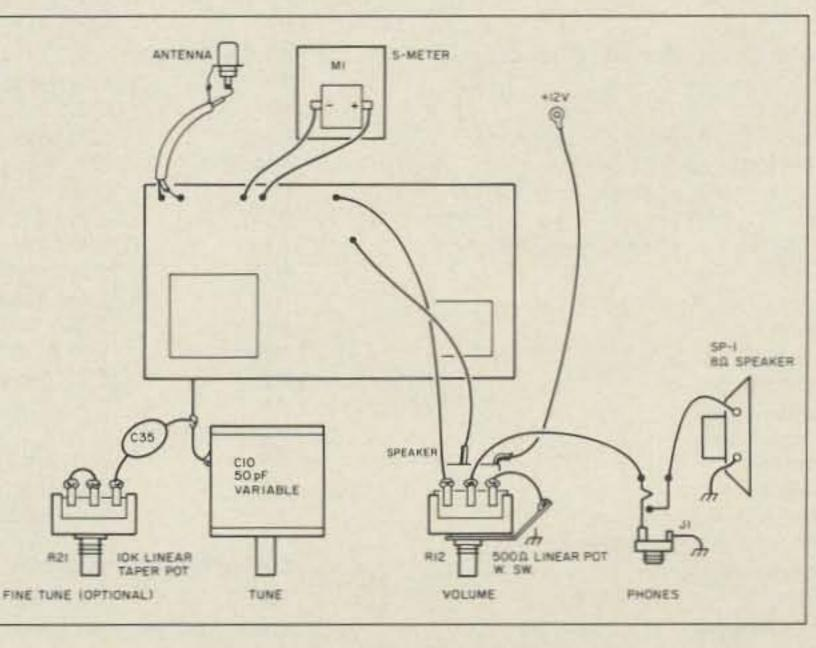
Fig. 4. Module connections.
