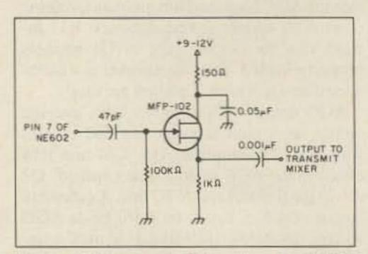
Fig. 5. Buffer circuit. This allows the NE602 on-board oscillator to drive other stages such as a transit mixer.
