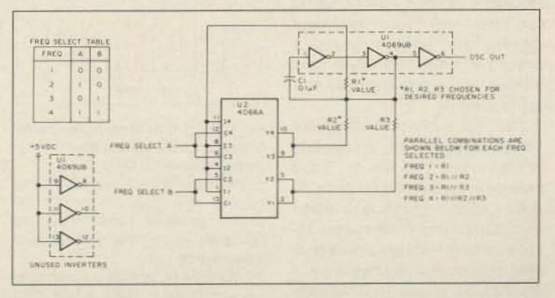
Figure 2. Variable CMOS oscillator. The U2 transfer gate switches additional resistors in and out, varying the circuit's frequency.
