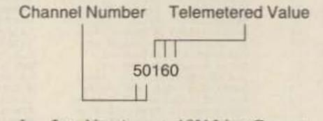
$I = 3 \times N mA = +10V$  Line Current  $I = 3 \times 160 = 480 \text{ mA}$
