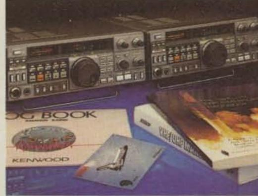
Versatile scanning functions. Programmable band and memory scan (with channel lock-out). "Center-stop" tuning on FM. An "alert" function lets
