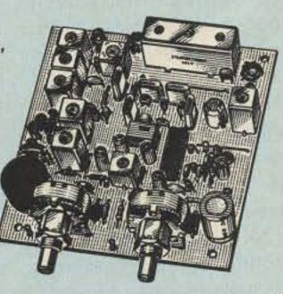
•R451 UHF FM RCVR. Similar to above. Tuned line front end, 0.25uV sens. (0.1uV with optional hel. res. preamp). Kit \$149, w/t \$229.
