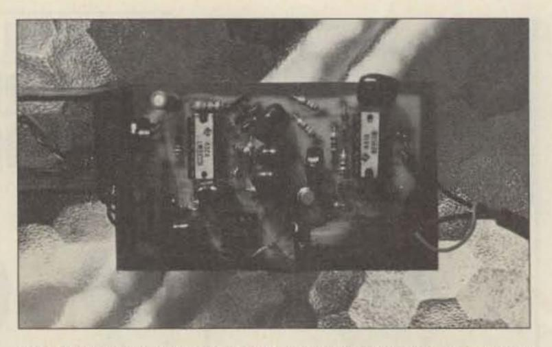
Photo B. It may not be much to look at, but my CW decoder allows high speed CW up to 100 wpm when connected to a computer.
