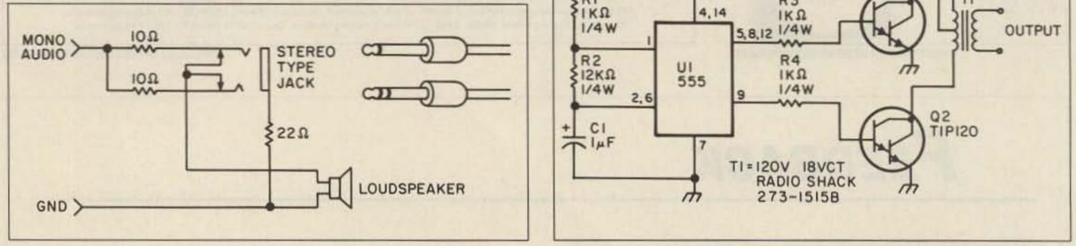
down the oscillator. The two transistors drive the transformer push-pull fashion. When one transistor is baised on the other is cut off.
