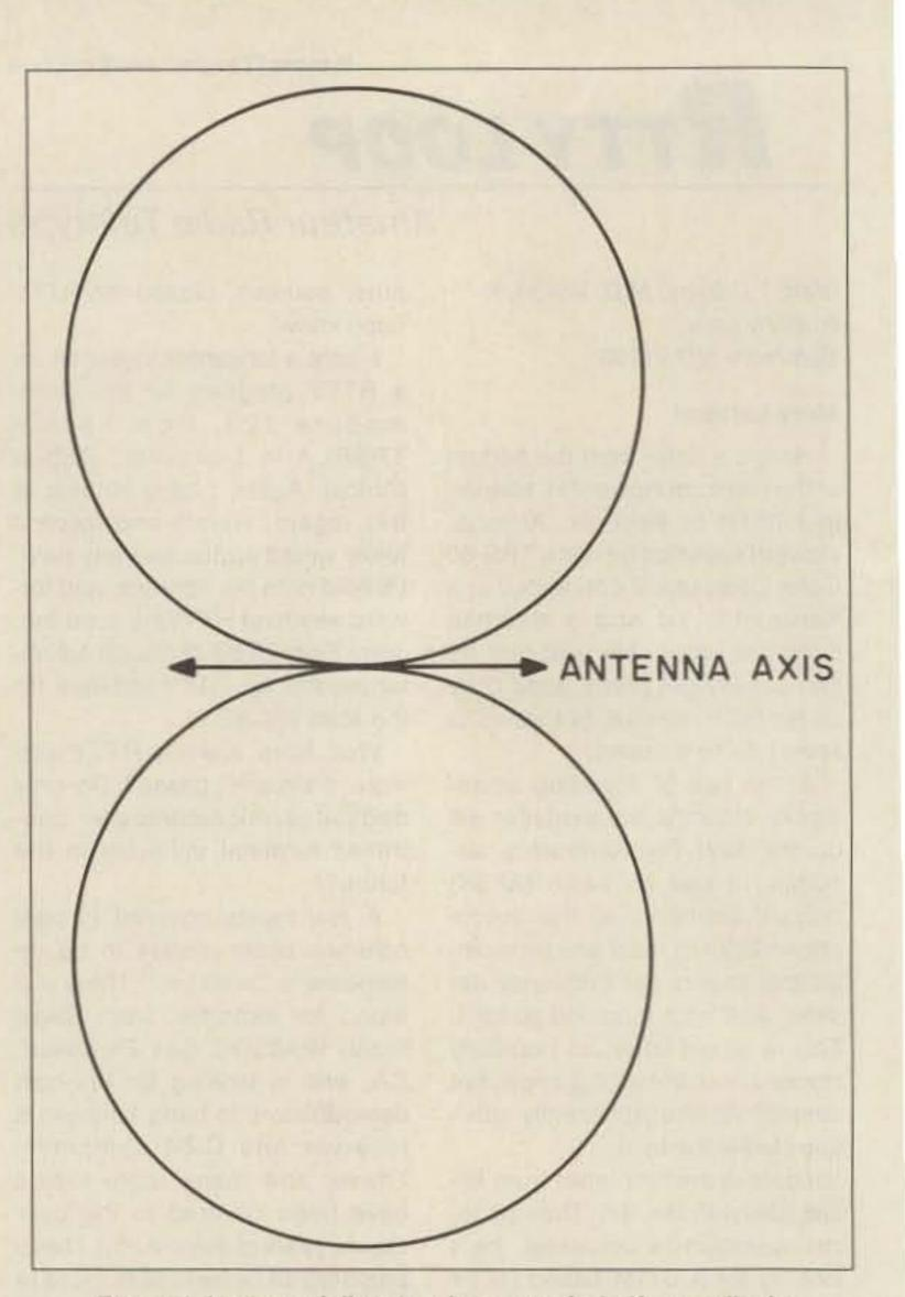
"Low antenna heights tend to reinforce high angles of radiation while producing cancellation of low-angle radiation."
