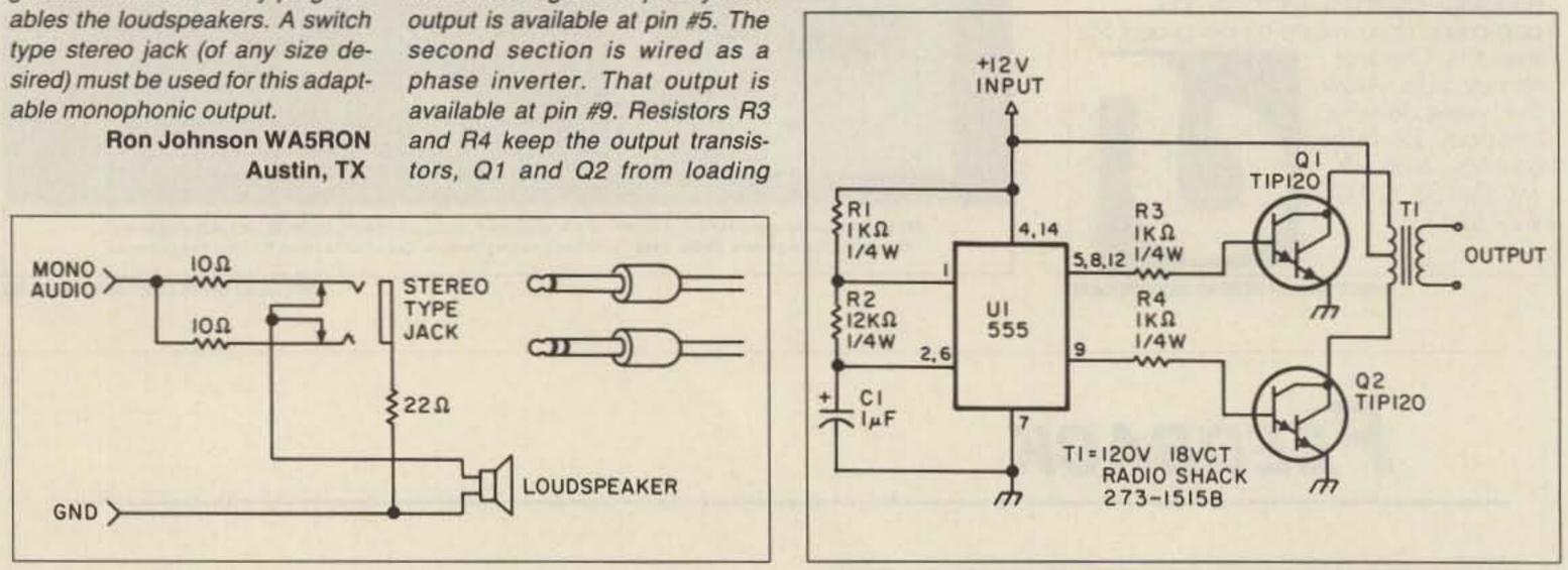
Figure 1. Adaptable monophonic output.
