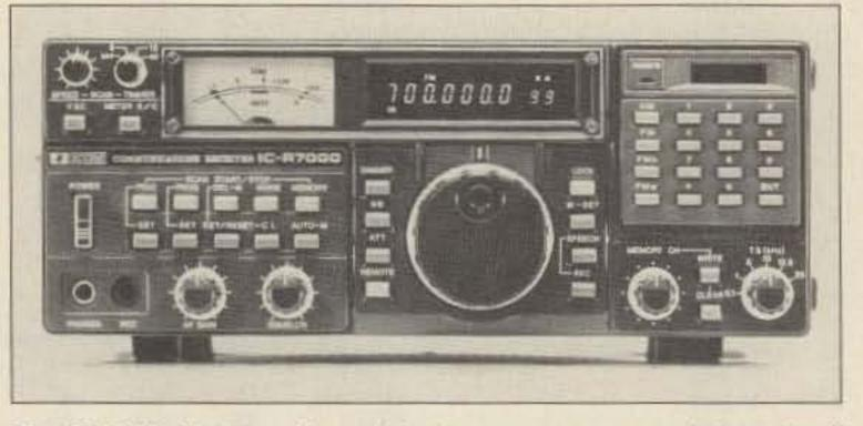
filters are varicap tuned, while stripline techniques are used from 512 to 1000 MHz. The wideband RF amplifiers are protected by tuned traps which suppress birdies from the first local oscilla-
