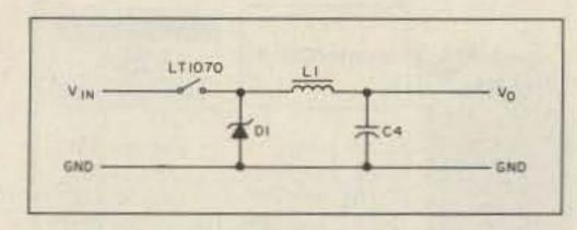
Figure 2. Positive buck converter.
