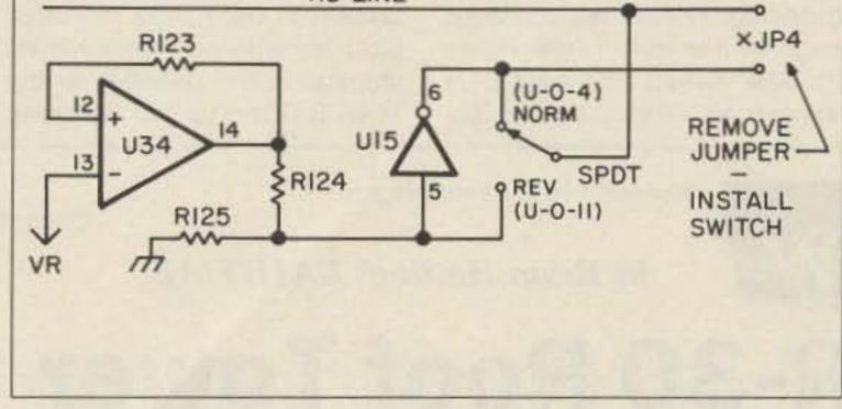
Figure 2. Hardware modification to the AEA PK-232 for U-O-9 or U-O-11 data reception.
