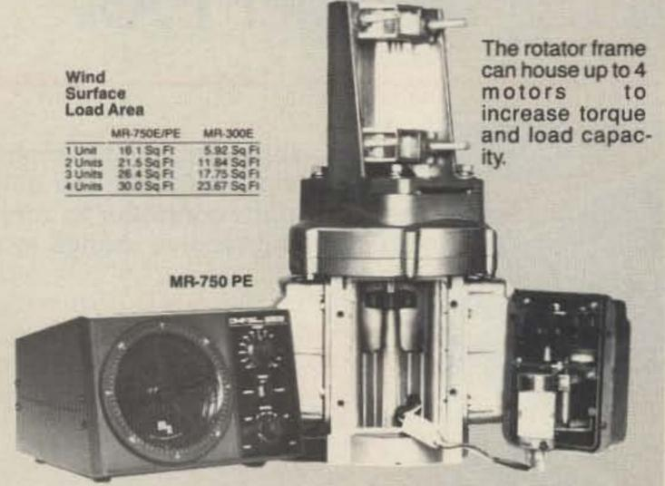
Each motor is equipped with a Super Wedge and Clutch brake system (Slip clutch type) that works independently from the main frame gear train and protects the rotator mechanism from excessive torque.
