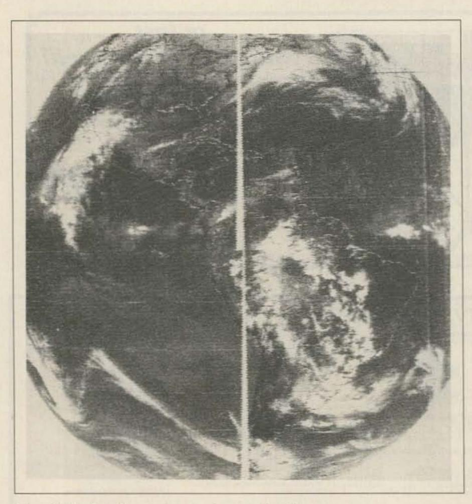
rest is just manual labor. Each quad overlaps its neighbor by just a small amount, so the four images can simply be overlapped slightly to reconstruct the earth disk image.
