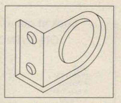
Fig. 5. Bracket for coax socket.
