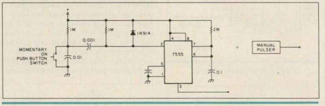
Figure 8. A handy manual pulser (pulse duration 1/3 second).
