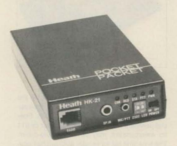
hen I saw the ad for the Heathkit HK-21 TNC, I knew I just had to have one. Heath calls the HK-21 a "Pocket Packet" for a very good reason. It's a compact, self-contained TNC with a built-in personal packet bulletin board system (PBBS). It was just the excuse I needed to put together a portable 21 and to the back of my HT, and mounted the TNC to my HT (see Photo C).
