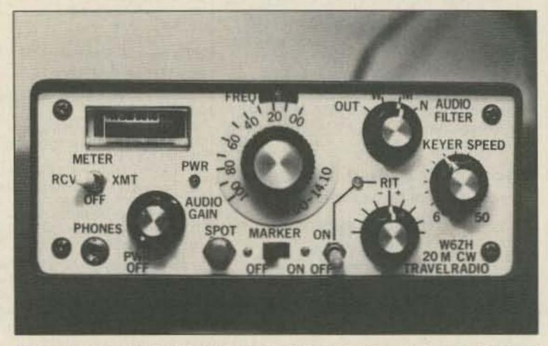
Photo B. Closeup of the front panel of the travel radio. The travel radio
