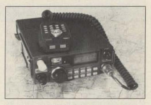
The Yaesu FT-790RII is ideal for mountaintop UHF operation and makes a light package with the accessory FBA-8 battery case.
