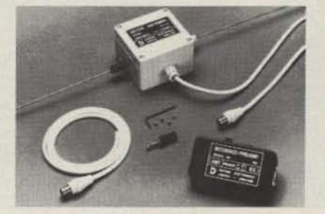
DATONG ACTIVE RECEIVER ANTENNAS FOR BIG PERFORMANCE ANYWHERE 3-meter (9¼') dipoles with low-noise amplifiers at the dipole and at the interface. Indoor model (AD-270) uses flexible wire elements; outdoor model (AD-370) uses stainless steel whips. Mount anywhere. 6 dB gain at the dipole, 12 dB at the interface. 100 kHz-70MHz. AD-270 \$114.50 (+\$3); AD-370 \$129.50 (+\$4.50); power converter \$15,95.
