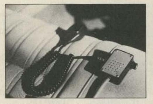
Photo A. A control head for the front seat of your car to access your Kenwood TS-440S in the trunk.
