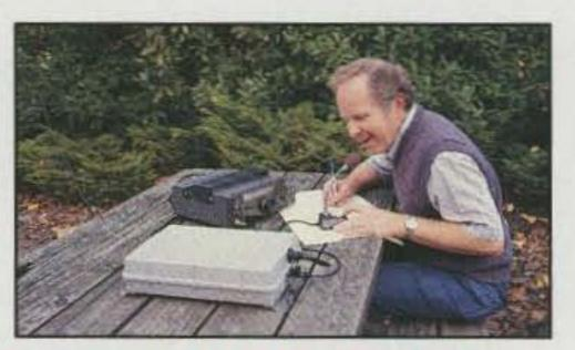
Optional AH-2 Automatic Tuning Mobile Antenna System covers 3.5MHz-30MHz and tracks with the IC-735's tuned frequencies.
