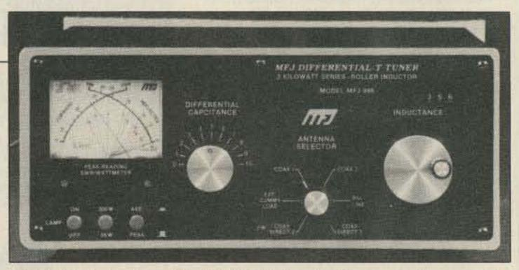
Photo A. Front view of the MFJ-986 showing the two tuning controls, antenna selector switch, and the cross-needle meter.
