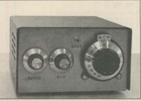
Photo A. Front panel of the QRP transceiver. The Receive Incremental Tuning (RIT) control allows you to adjust the receive frequency without changing your transmit frequency.
