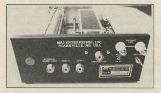
Photo B. Rear panel provides feedline, ground, and 12 volt DC connectors.
