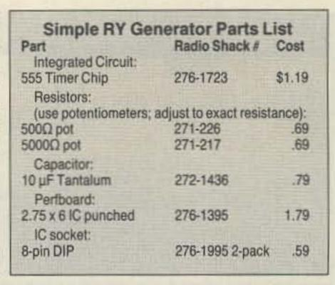
pending upon the exact frequency rate. That is why I suggested you never put it over the air! But for local testing and alignment, or to provide a frequency shifted signal to set a demodulator, it can't be beat!
