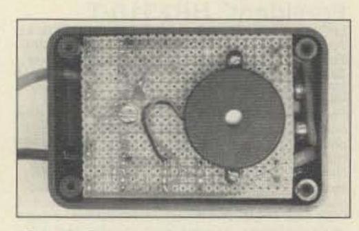
Photo B. Speaker side of the continuity checker board.
