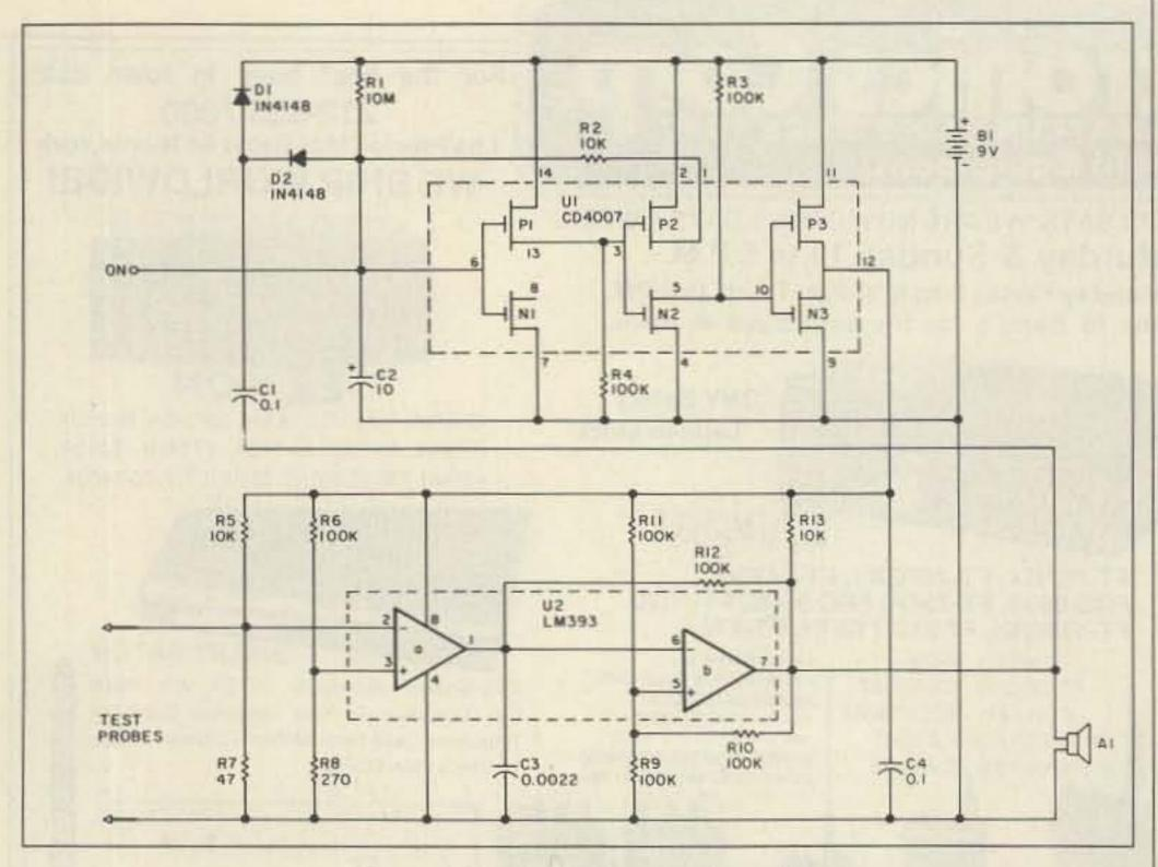
Figure 1. Continuity beeper schematic.
