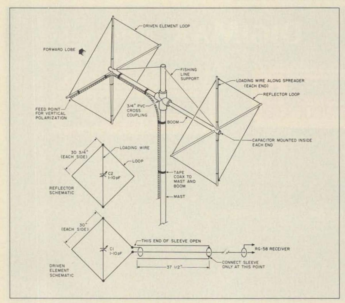
Figure 1. Construction details for the 6 meter shrunken quad. See text for additional dimensions.
