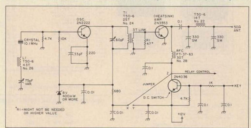
Figure 1. Schematic for the 30m QRP transmitter.
