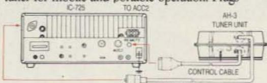
directly into the IC-725. Wide impedance matching range. Mating whip unit (AH2-B) bolts to auto's frame, works 80-10 meters.
