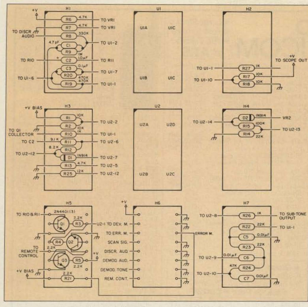
Figure 2. Parts placement for the Monitor.
