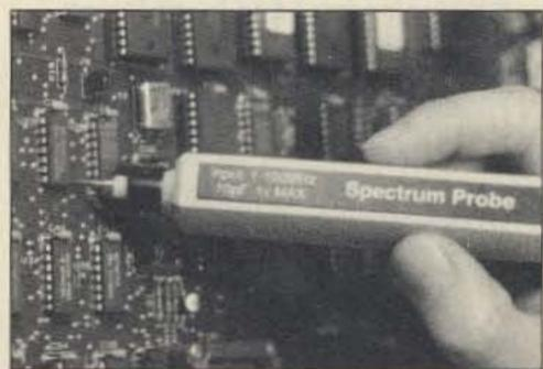
The Smith Design spectrum analyzer probe.
