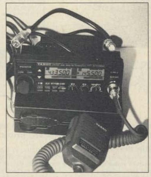
Photo A. Control head and main unit ready for installation. Note dummy front panel with remote connector.
