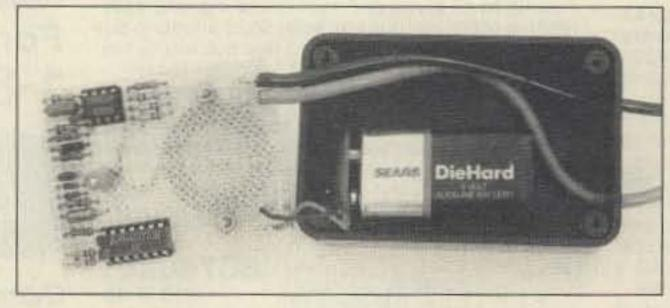
Photo C. Component side of the continuity checker board.
