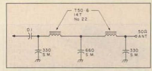
Figure 2. Alternative low-pass filter for greater attenuation of harmonics.
