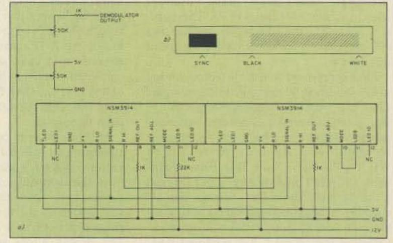
Figure 13. Visual signal tuning aid. a) shows the schematic, and b) is a diagram of the LED display.
