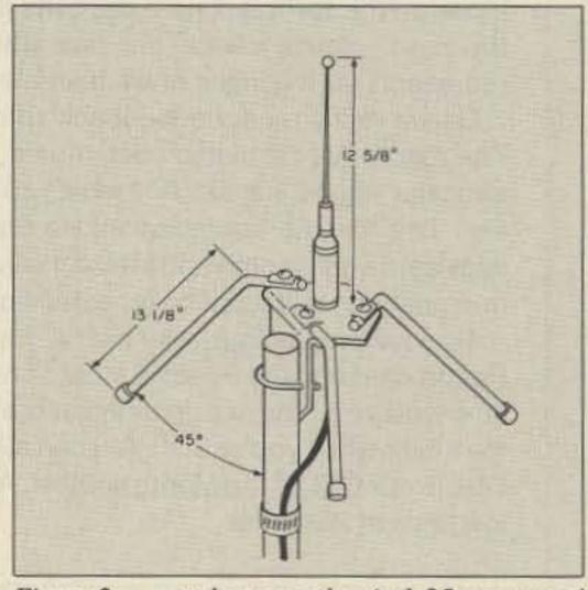
Figure 2... and as a good-gain 1.25m antenna!
