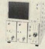
plug-ins. Performs to 65 MHz but 100 MHz mainframe accepts standard 7000-series plugins for full versatility. Deflection 5 mv to 10 V/div in 11 steps. Sweep 0.05 us to 5 S/div in 25 steps; delay to 0.5 s/div. 11.5x9.7x25.2, 52 lbs sh. Used-checked w/book.....\$495
