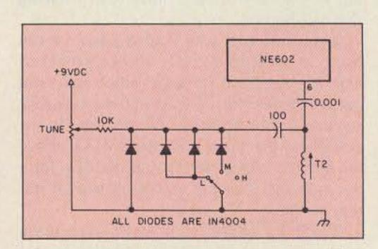
Figure 2. The HR-4 tuning circuit modified for greater coverage.
