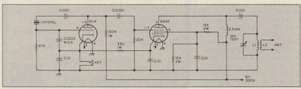
Figure. A 6C4 is used in a Pierce oscillator driving a 6AQ5 as an amplifier or doubler.
