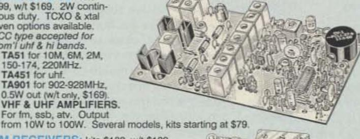
FM RECEIVERS: kits \$139, w/t \$189. R144/R220 FM RECEIVERS for 2M, 150-174, or 220MHz. GaAs FET front end, 0.15uV sensitivity! Both crystal & ceramic if filters plus helical resonator front end for exceptional selectivity: >100dB at ±12kHz (best available anywhere!) Flutter-proof hysteresis squelch; afc tracks drift.
