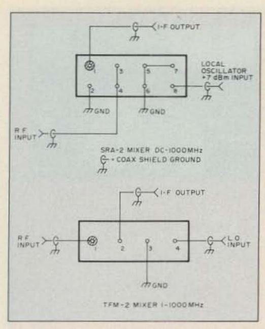
Figure 2. Typical mixer connections.
