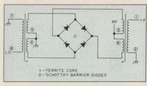
Figure 3. Schematic for basic mixer.
