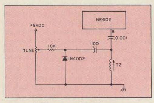
Figure 1. The original HR-4 tuning circuit.
