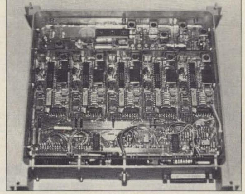
Photo B. The WEBERSAT module before final assembly.
