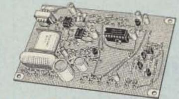
AP-3 AUTOPATCH kit. Use with above for repeater autopatch. Reverse patch & phone line remote control are std . \$79
