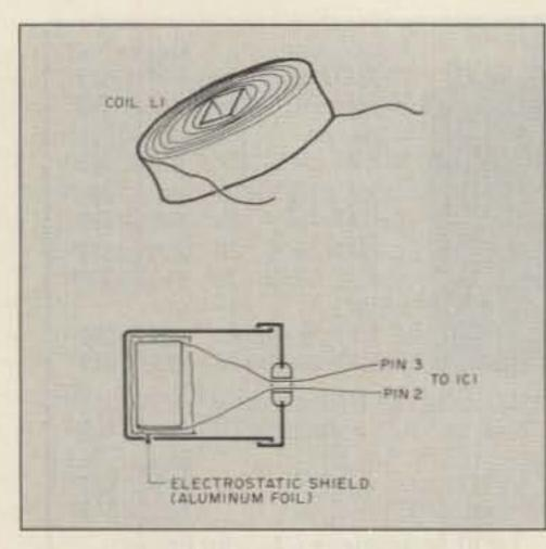
Figure 2. The probe, showing the coil and L1 mounted in a 35mm film can.
