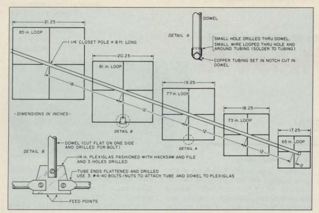
Figure 1. Constructing the 2 meter beam.
