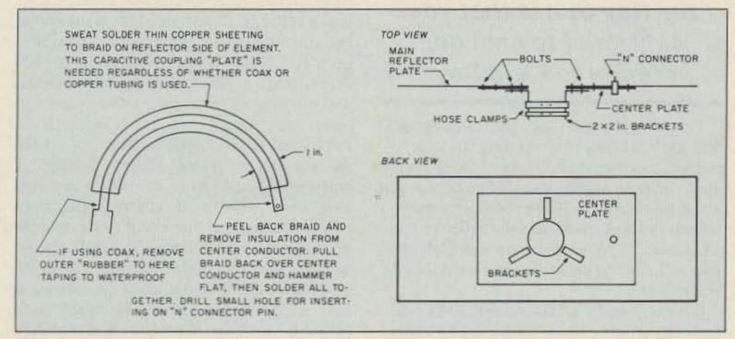
Figure 3. Final construction details.
