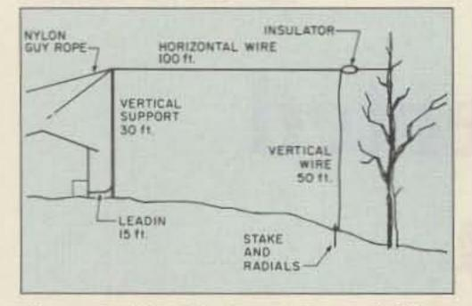
Figure 2. The "backward inverted L" or "inverted U." Note that the far end is grounded, ensuring a current maximum along a vertically polarized part of the antenna. (Radials not shown.)
