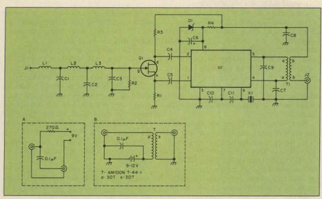
Figure 1. Schematic for the 80AU converter.
