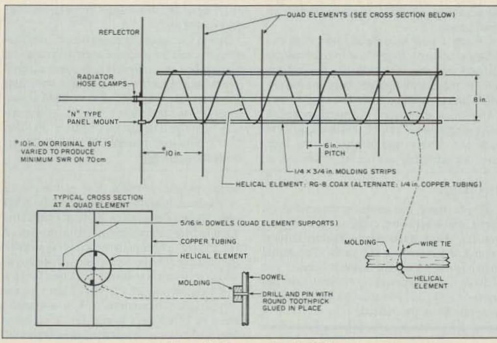
element supports are made from 5/16" dowels. (Again, their diameter is not critical.) The insulator on the driven element was fashioned from a piece of plexiglas. The elements are connected to the dowel supports by the system Jim McKim W0CY used in his helix. (See Figure 1 for details.) The dowel supports are mounted to the "boom" by drilling 11/32" holes ½" deep in the boom. Fill the holes with fresh carpenter's glue and force the dowels into place.
