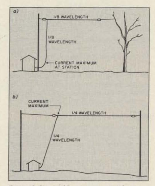
the top of the support to the treetop, and 45 feet to the grounded far end, for a total of 190 feet. Since I have a wide-range antenna tuner, I was not especially concerned about the impedance at the feedpoint.
