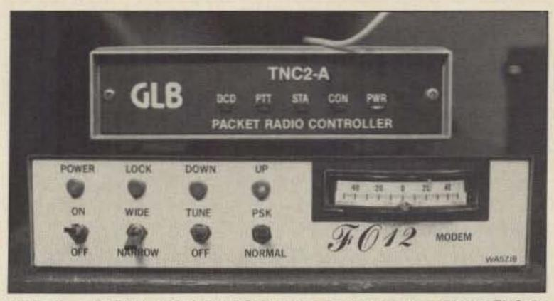
Photo A. A G3RUH 1200 baud PSK modem hooked up to a packet TNC for Microsat or Fuji digital communications.
