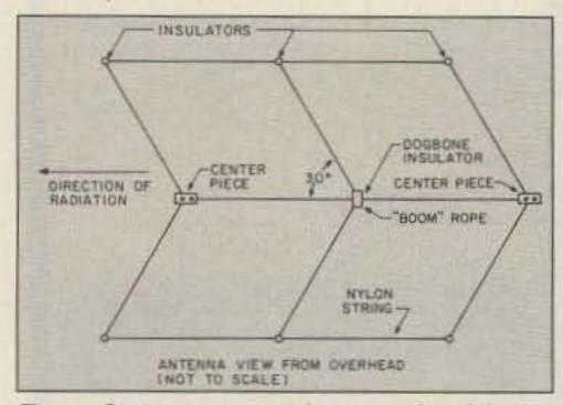
Figure 2. Antenna view from overhead (not to scale).
