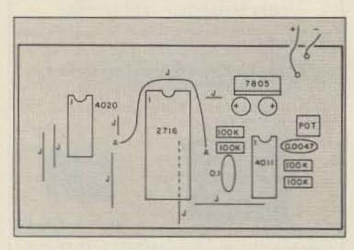
Figure 2. Parts placement, component side.
