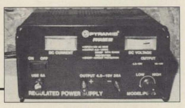
construction is quite excellent, and a schematic was included with the supply. The circuitry uses an integrated regulator chip with standard RCA 2N3055 NPN pass transistors.
