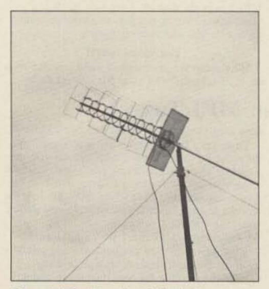
Photo A. The ''Ray Gun'' Mode B concentric combo antenna installed for Field Day operation. Note the string (horizontal line from the mount, lower right corner of the photo) used to adjust the elevation.
