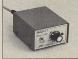
IsoLoop LC-1 control box with variable speed tuning.
