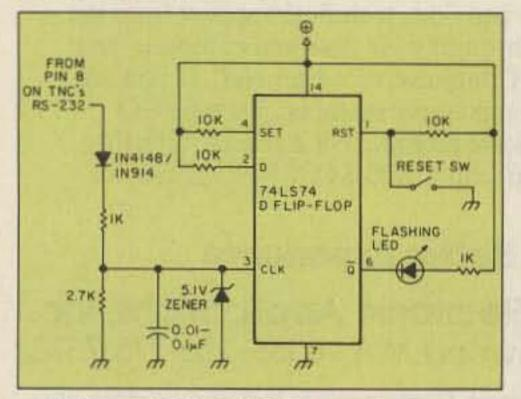
Schematic of the TNC connect alarm.
