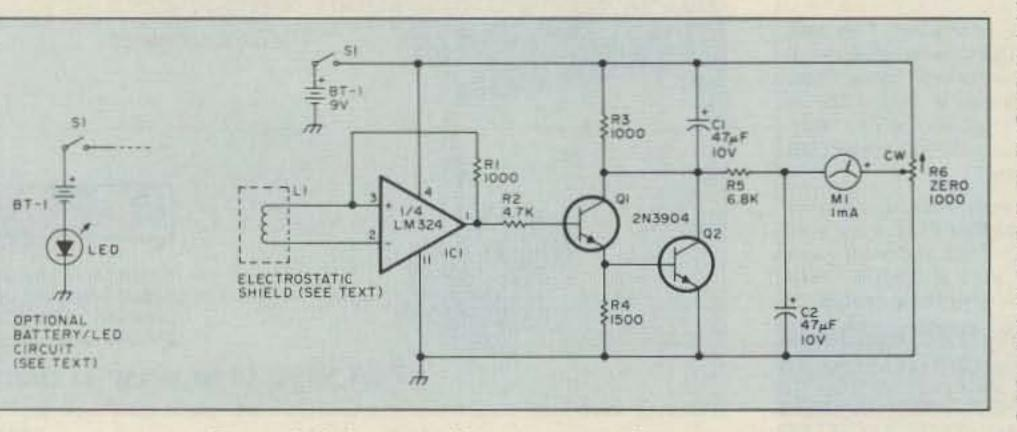
Figure 1. Schematic of the experimental gaussmeter.
