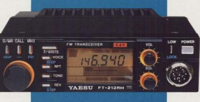
• Frequency Range: 140-174 MHz on receive (144-148 MHz TX—Modifiable for MARS and CAP). Specifications guaranteed on amateur bands only.
