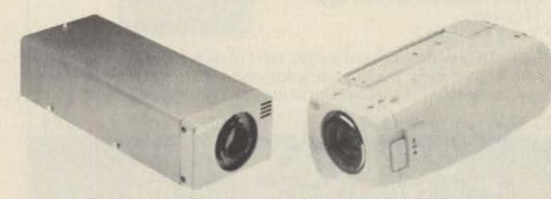
Photo B. The Sony HVM-322-BNC (left) and CCD-G1S (right).
