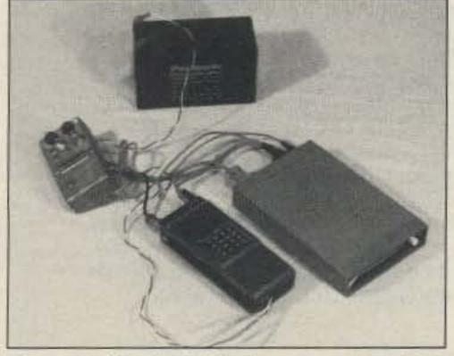
Photo A. The individual components of the BackPacket.
