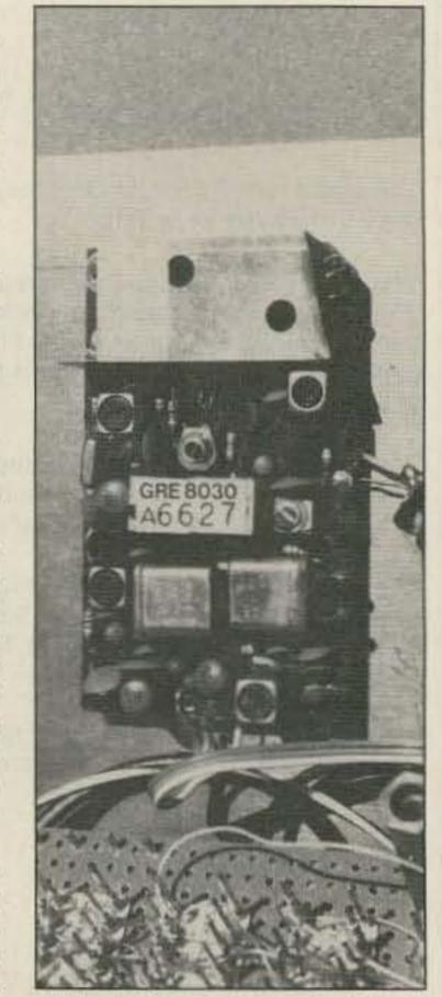
Photo A. The matchbox-size LJE receiver mounts under the aluminum cover plate with adhesive foam. Keep the lead to the antenna connector short.
