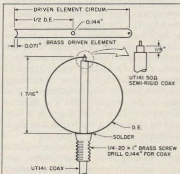
Figure 3. Driven element construction.
