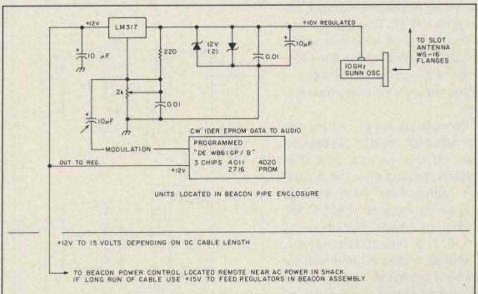
Figure 1. 10 GHz beacon showing CW ID'er and power supply. Regulator/modulator audio from ID'er feeds to adjust terminal of regulator for modulation on input on regulator output voltage to Gunn oscillator, which produces high quality wideband FM on 10 GHz (See "Above and Beyond" in the June 1990 issue of 73 for CW ID details).
