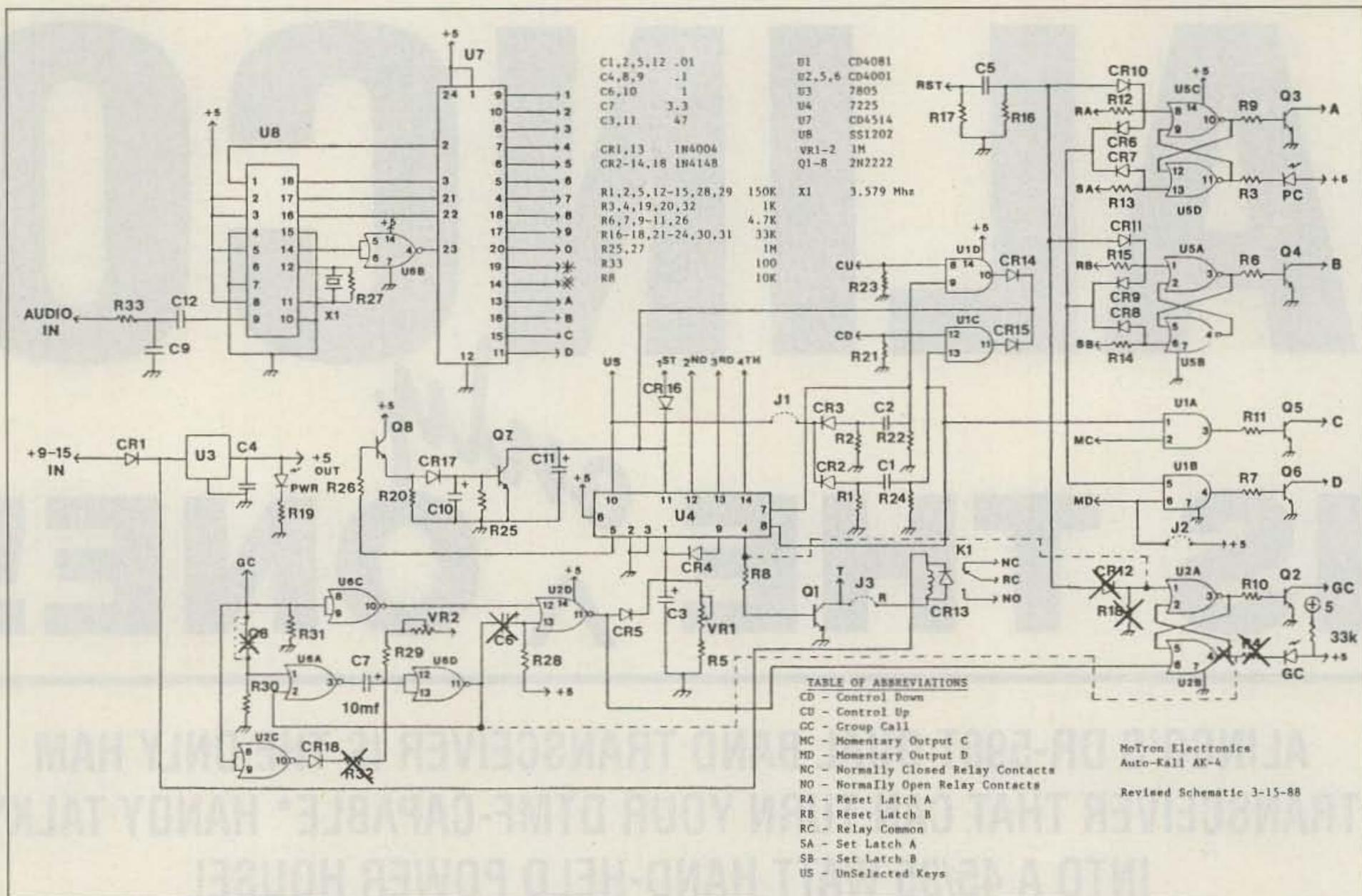
Figure 5. Modified AK-4 schematic diagram.
