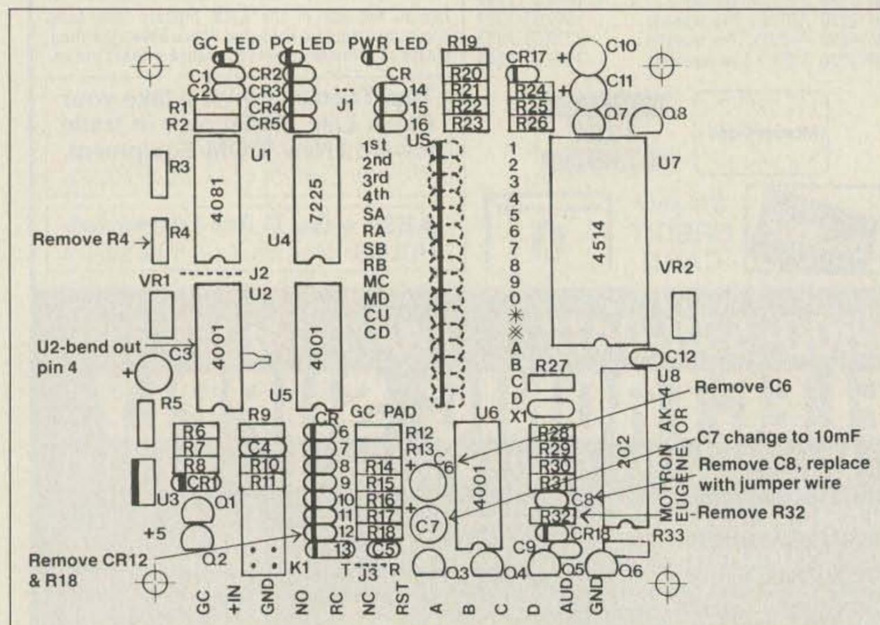
Figure 4. AK-4 modifications (circuit board details).
