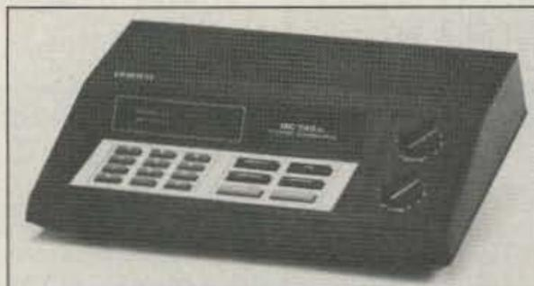
Photo B. The Uniden BC-145 scanner modified for weather satellite receive.
