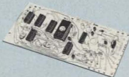
**COR-4 kit.** Complete COR and CWID all on one board for easy construction. CMOS logic for low power consumption. Many new features. EPROM programmed; specify call .....\$99
