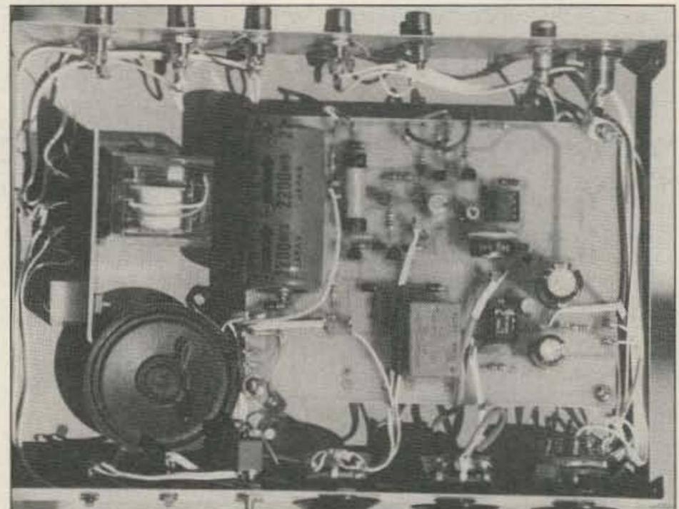
Photo B. Inside view of the T/R controller. Notice the relay mounted off of the board next to the speaker. There is one relay mounted on the board in this version of the controller.
