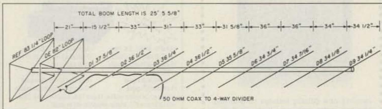
Figure 1. Modified W5UN quagi (optimized for 144.050 MHz - gain of 13.25 dBd). All directors are 1/8" solid aluminum rod cut to within  $\pm 1.16$ ". Reflector and driven elements are shaped into square loops using number 12 solid copper wire with TW type insulation. Leave the insulation in place. Boom is either non-conductive sealed wood or Fiberglass™.
