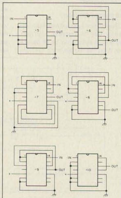
uary 1991, p.27). The figure shows the connections which allow the 7490 to divide by 5, 6, 7, 8, 9 and 10.
