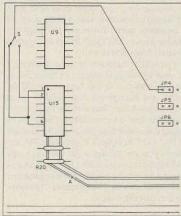
Figure 1. PK-232 modification for UoSAT-11 telemetry reception.
