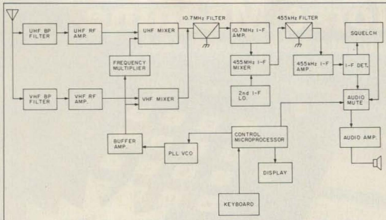
Figure 1. Generic FM scanner block diagram.
