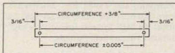
Figure 2. Loop yagi element dimensions.
