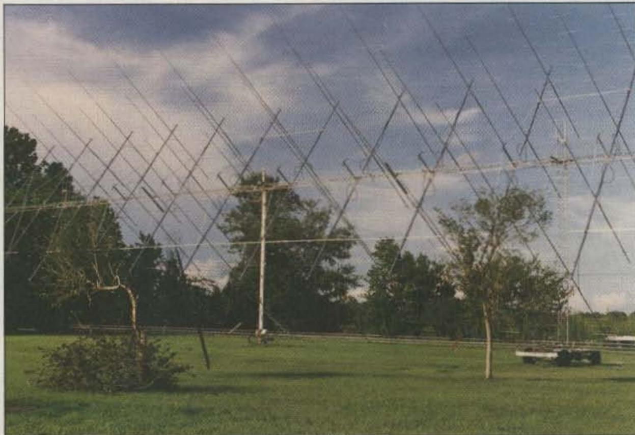
*Photo B. The W5UN EME array is rotated via 2 truck chassis (powered via an electric motor on the driveshaft of one of the vehicles) which literally drive the antenna around a large circular roadbed. The array pivots around a rotating pole in the center. An electric winch along with a series of pulley and cables provide elevation control.*
