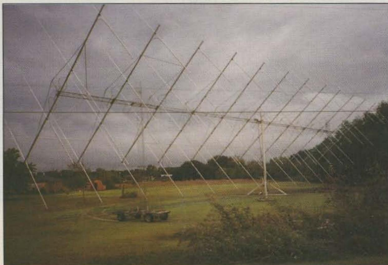
*Photo A. The new W5UN EME antenna array providing 30.75 dBd of gain (the old array was destroyed by a tornado last March). Dubbed the "Mighty Big Array" or MBA, it consists of a total of 48 stacked long boom yagis (modified M<sup>2</sup> model 2M5WL).*
