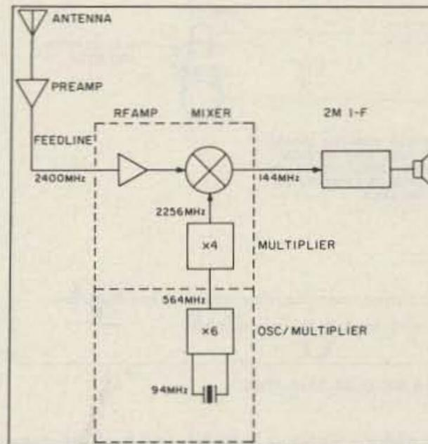
Figure 1. Basic 2400 MHz receiving converter.
