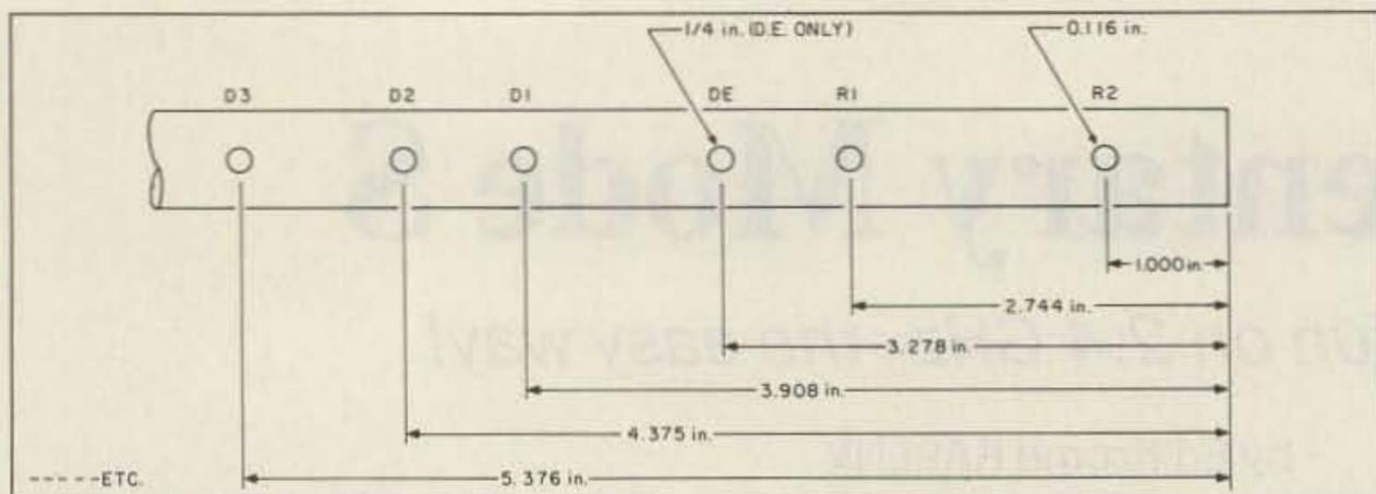
Figure 4. 13cm loop yagi boom drilling.
