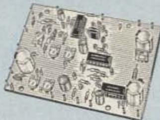
**COR-3 REPEATER CONTROLLER kit.** Features adjustable tail & time-out timers, solid-state relay, courtesy beep, and local speaker amplifier .....\$49
