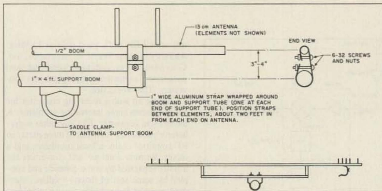
Figure 5. 13cm antenna and support assembly.
