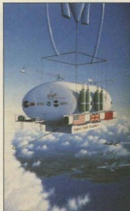
Photo B. Pressurized gondola which will be used for the round-the-world flight at 35,000 feet this November. Artist rendering by Stan Stokes.
