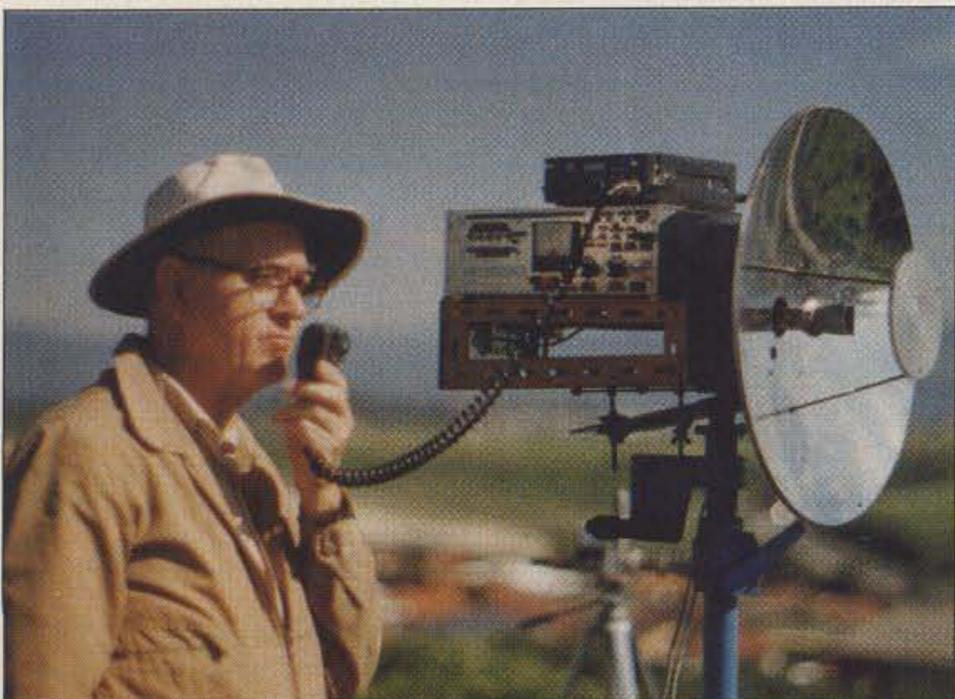
Photo A. Lyle Patison VK2ALU of Wollongong, Australia, operating a 10368 MHz transceiver on SSB, testing over 80 km to VK2ZAC (who can receive on SSB but only transmit on NBFM). Note sighting telescope mounted below dish. A Cassegrain subreflector feed is used allowing more efficient illumination. The 20 inch dish is a searchlight reflector.
