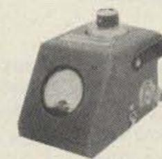
AN/URM-120 WATTMETER measures RF output over 2-30 MHz from 10 to 1000 watts and up to 1000 MHz at 500 W using three plug-in coupler elements with selectable power ranges. Max-insertion VSWR 1.08 except 1.05 on highest power ranges above 30 MHz. Has 3.5" dia meter with 0-10-50 W scale and N connections; similar to Sierra 164. Includes meter, coupler elements, transit case, and book. 4x4.8x7.3, 20 lbs sh. Used-repairable ..... \$137.50
