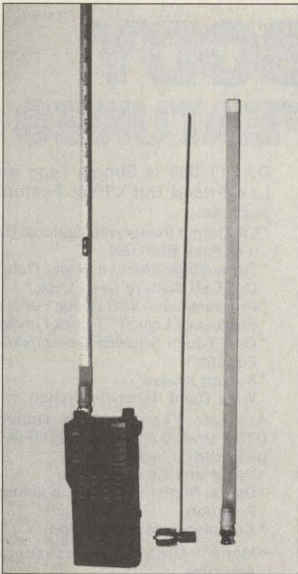
Photo C. The finished antennas.
