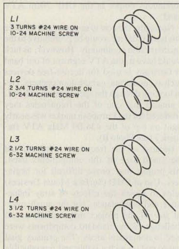
Figure 4. Coil winding details.
