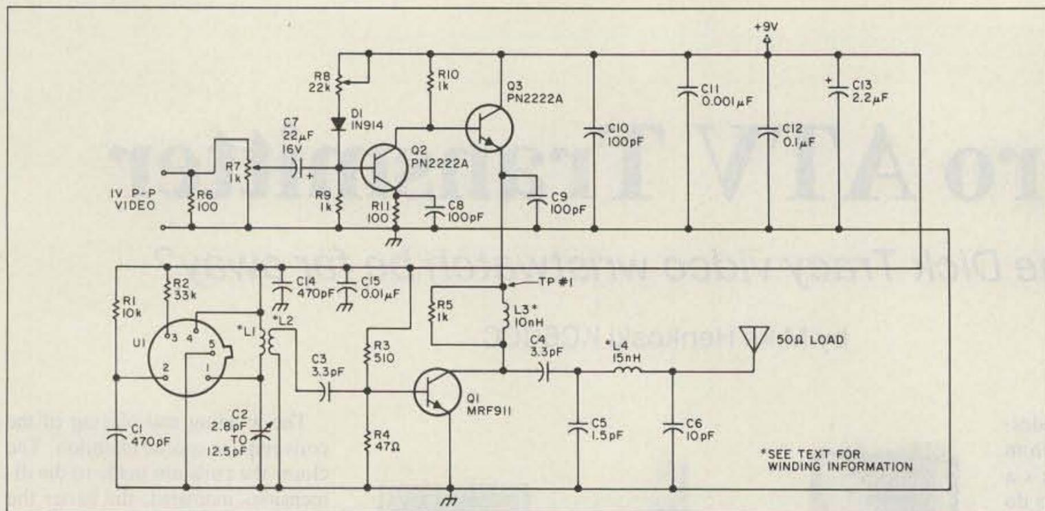
Figure 1. Schematic diagram of the micro TV transmitter.
