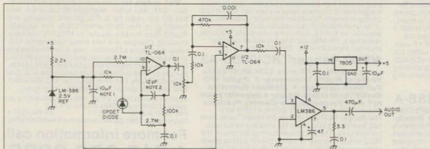
Figure 1. The Laser receive system. Note 1: The 10  $\mu$ F capacitor removes the low frequency component (AC) from the optodetector. Note 2: The 12 pF capacitor on the first stage of the TL-064 prevents oscillations and improves stability. Note 3: Adjust the feedback network on the first stage of the TL-064 to maximize at your frequency (approx. 1 kHz). Response is broadband in nature.
