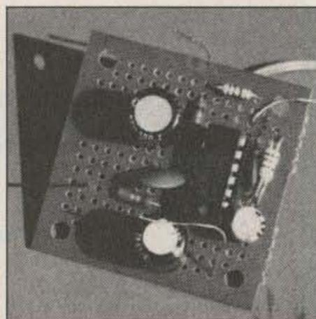
Photo B. The 2 watt audio amplifier assembled on perboard.
