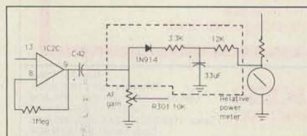
Figure 1. An S-meter for the HW-8.
