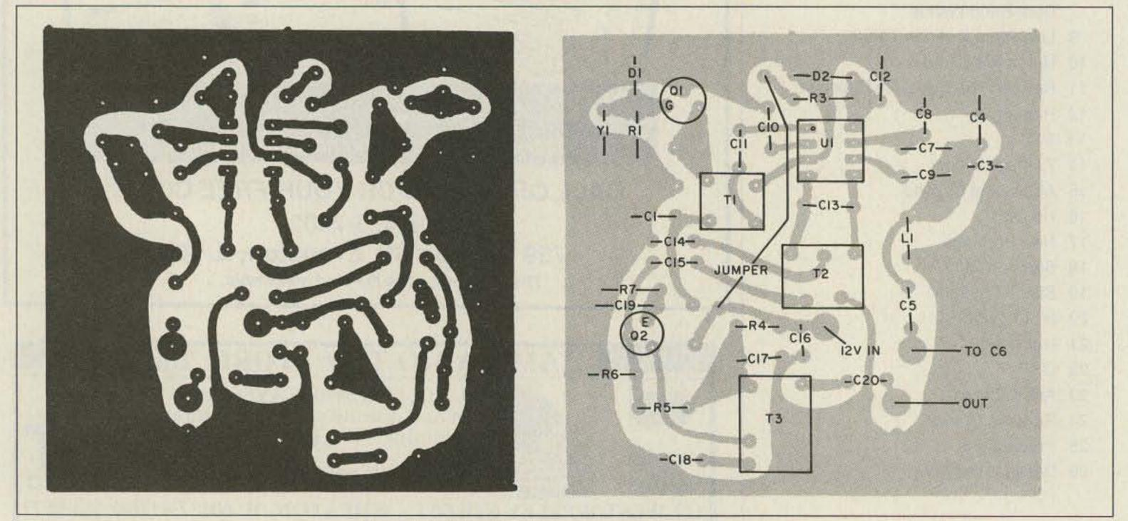
Figure 5 (a) The VFO foil pattern. (b) Parts placment.
