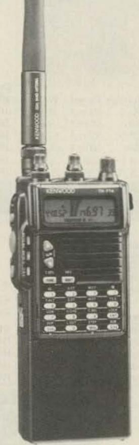
is easy to wind up with VHF volume and UHF squelch on one control, with the situation reversed on the other! It's not serious, but it can be confusing. Since squelch tends to be a set-and-forget operation, perhaps it would be better if the squelch controls were small, recessed knobs on the back of the radio. Overall, the rig feels like
