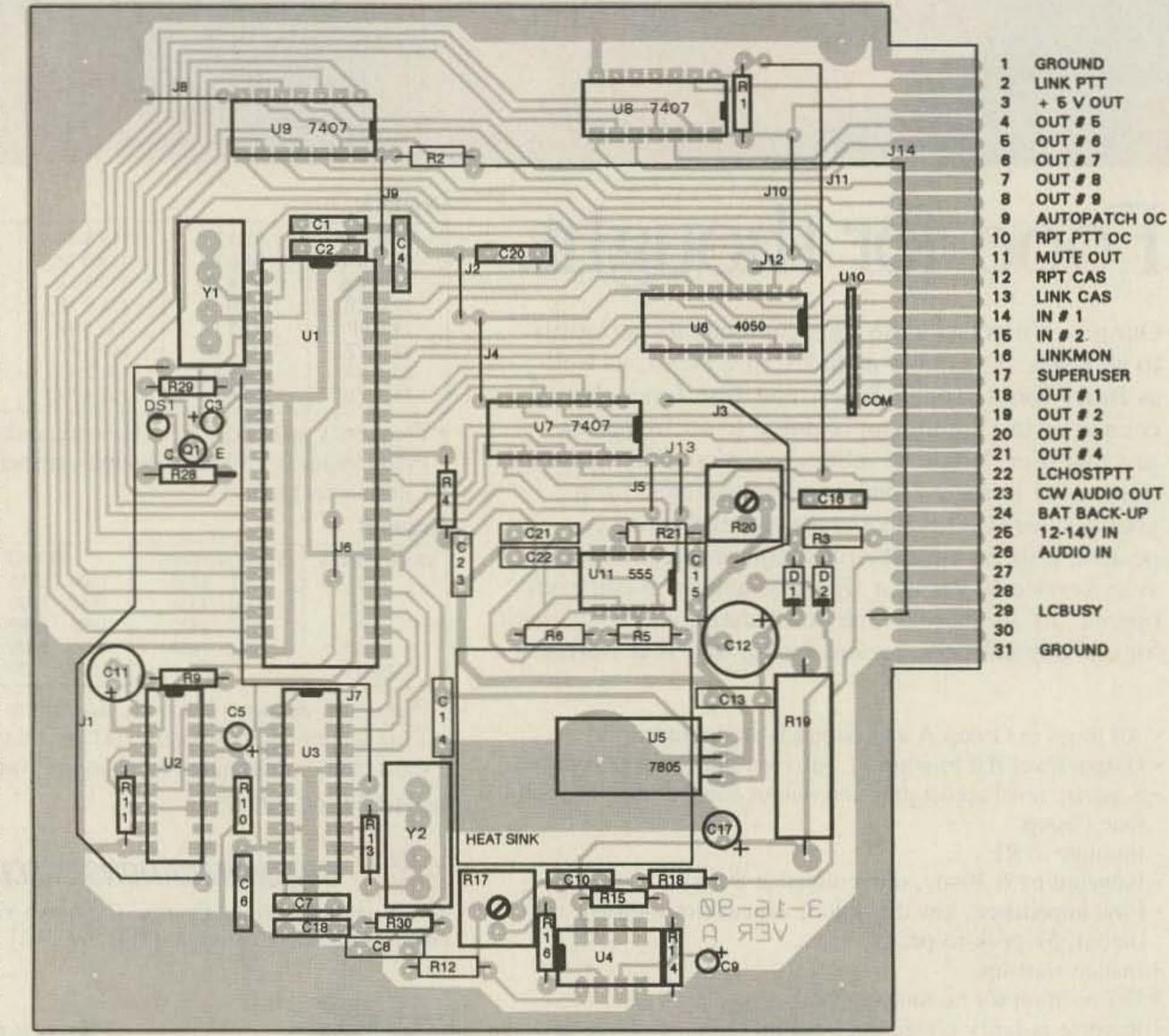
Figure 4. Computer board parts placement.
