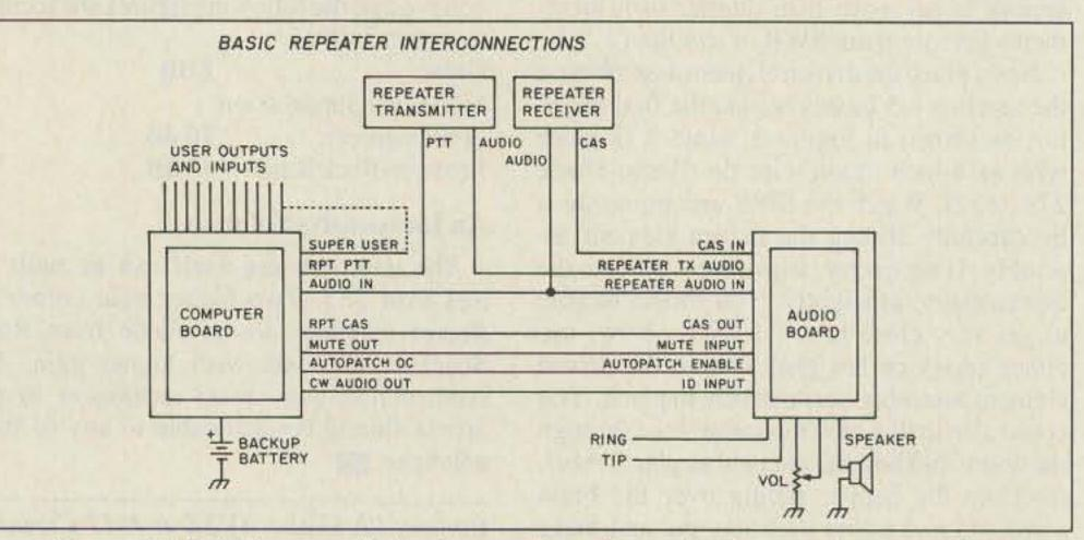
Figure 1. Block diagram of a basic repeater system using the repeater controller.
