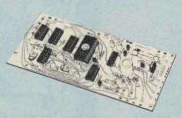
COR-4 kit. Complete COR and CWID all on one board for easy construction. CMOS logic for low power consumption. Many new features. EPROM programmed; specify call ..... \$99
