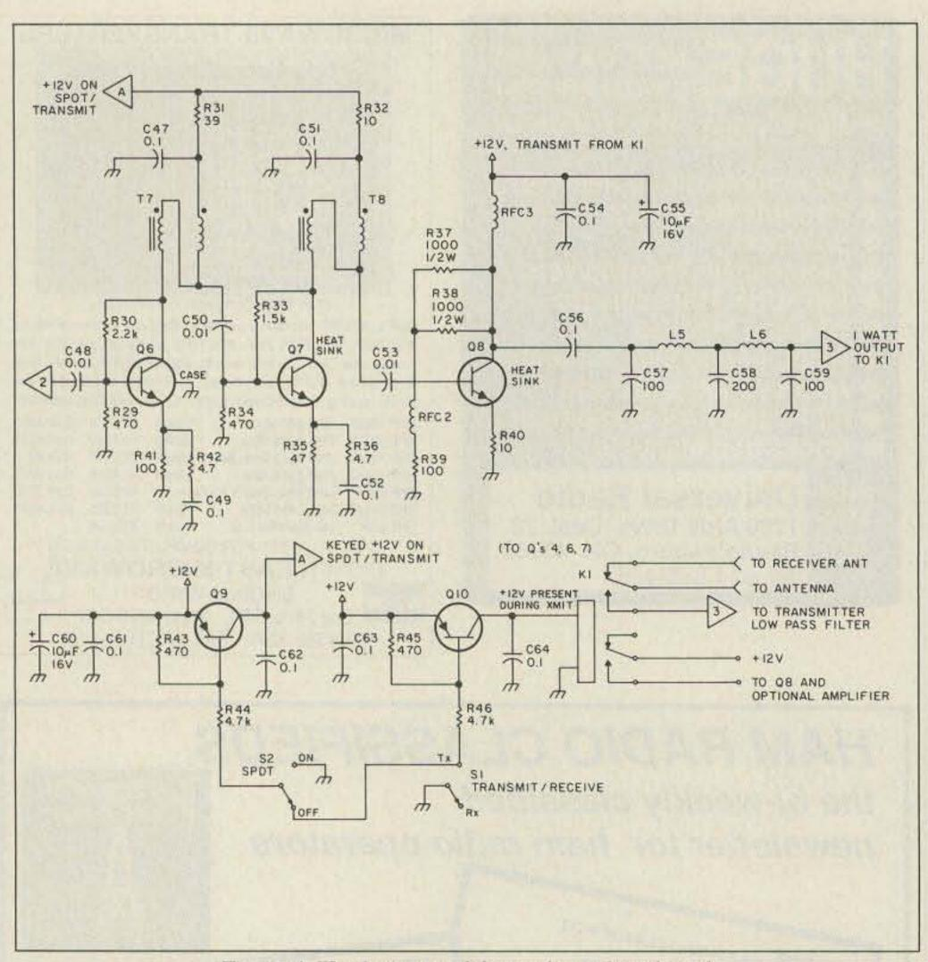
Figure 4. The 1 watt amplifier and switching board.
