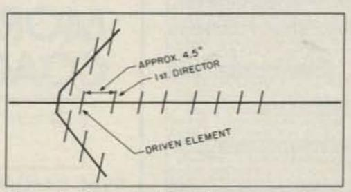
Figure 3. Mount the driven element to the boom about 4.5 inches behind the first director.
