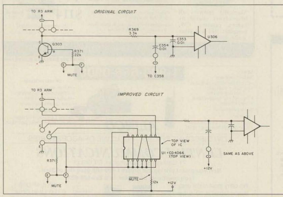
Figure 1. The key-thump suppressor for the HW-9. Courtesy of Paul Levesque KB1MJ.
