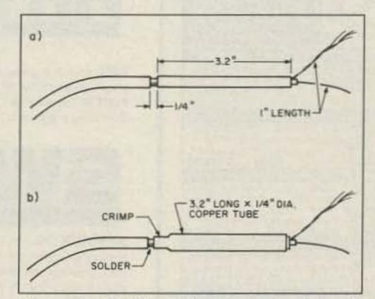
Figure 2. (a) Sleeve balun construction. (b) Crimp the balun and solder equal length leads onto the balun sleeve and center conductor.
