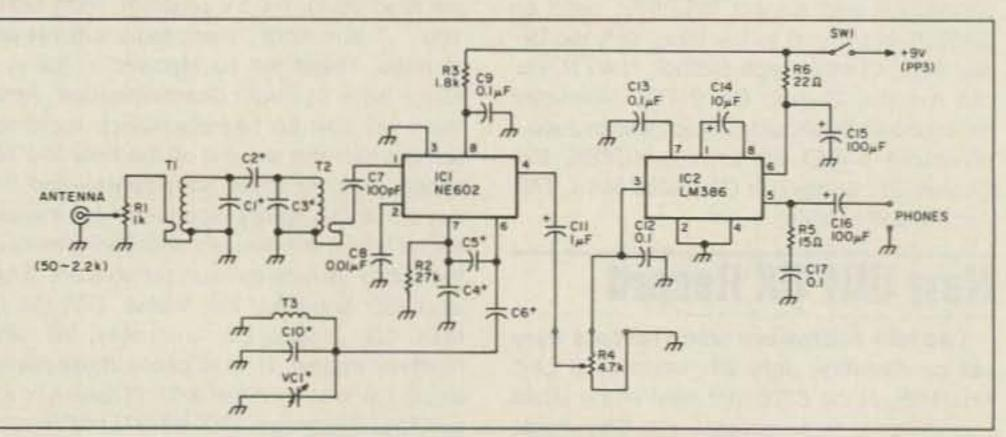
Figure 2. Schematic of the Sudden Receiver circuit.
