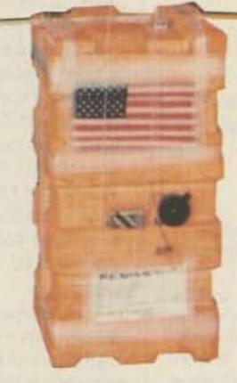
Photo C. The second (and third) BLT payload. The weathervane helped maintain stability during the flight. Note the Radio Shack beeper which helped the chase team to hear the downed payload. The TV camera/mirror is on the other side of the payload.
