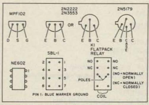
Figure 8. Base diagrams, all bottom view.
