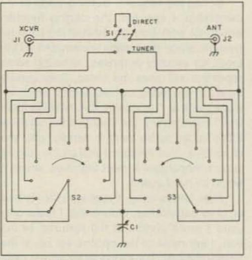
Figure 1. Schematic for the low-pass antenna tuner.
