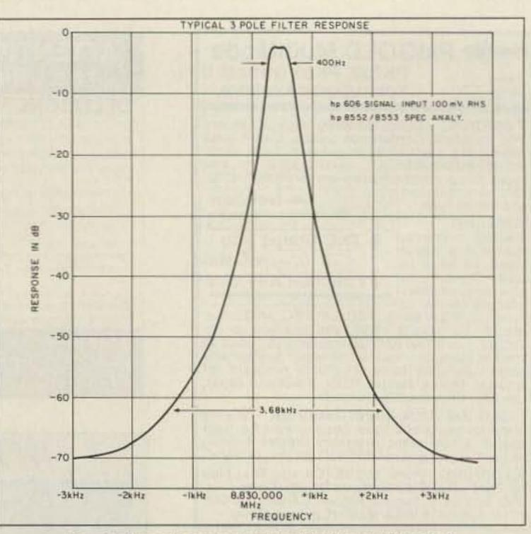
Figure 2. The audio response with the KB1MJ crystal filter circuit.
