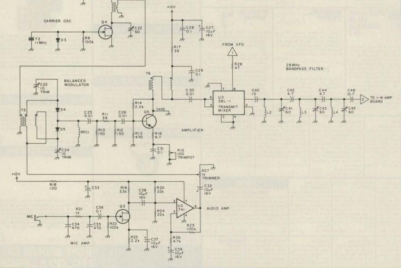
Figure 3. The balanced modulator/mixer board.
