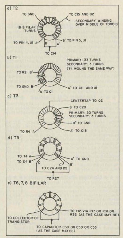
Figure 10. Winding specific toroids: (a) T2, (b) T1, (c) T3, (d) T5, and (e) T6,7,8.
