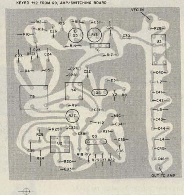
Figure 6 (a) The balanced modulator/mixer foil pattern. (b) Parts placement.
