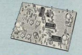
COR-3 REPEATER CONTROLLER kit. Features adjustable tail & time-out timers, solid-state relay, courtesy beep, and local speaker amplifier ..... .....\$49
