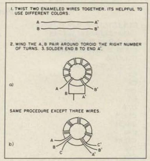
Figure 9. Winding the (a) bifilar transformer, and the (b) trifilar transformer.
