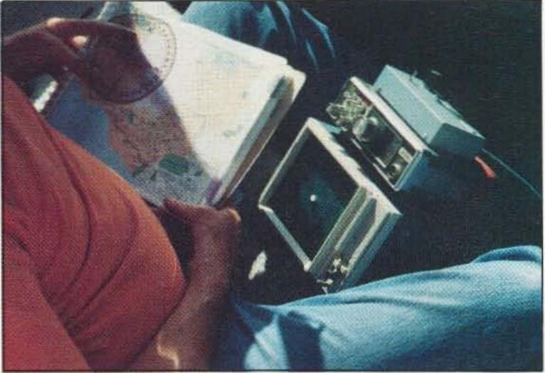
Photo A. KK6CU shows how his mobile CRT display is used. The storage scope is in a very deep cabinet, so it goes on the floor in front of the passenger/navigator.
