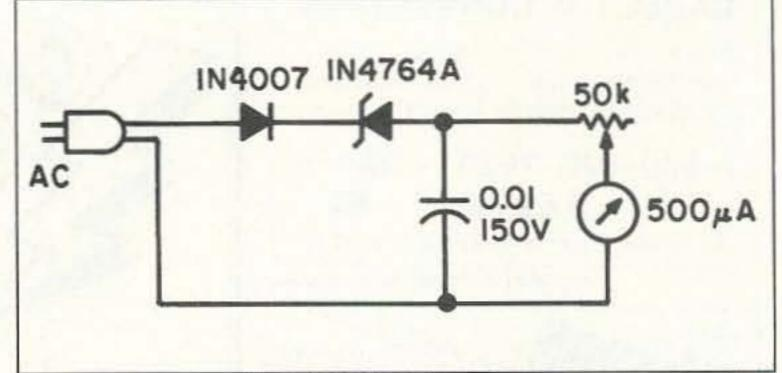
Figure 1. AC line voltage monitor.
