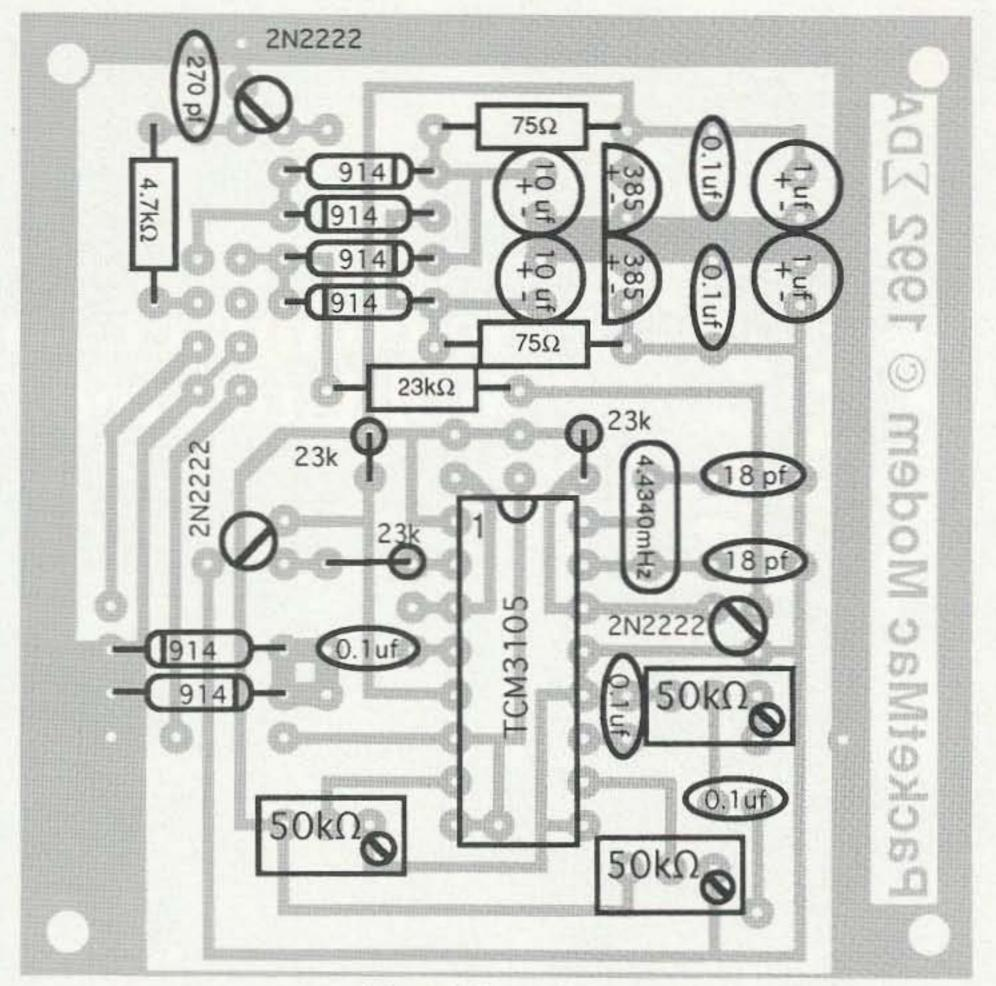
Figure 3. Parts placement.
