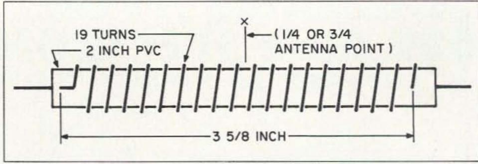
Figure 3. Coil winding details.
