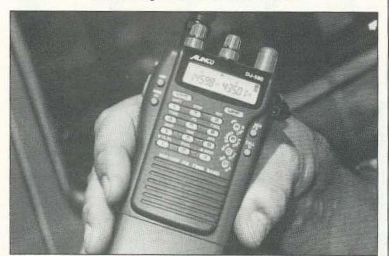
Photo B. The Alinco DJ-580T set up for full duplex, FM crossband operation via A-O-21.
