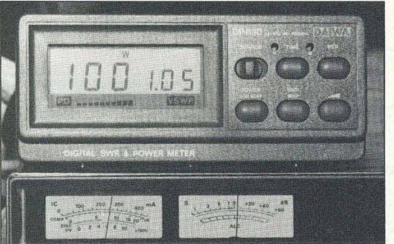
Photo B. The DP-830 happily sitting on a transceiver. Note the simultaneous display of power and SWR. Relative power is also shown by the bar graph.
