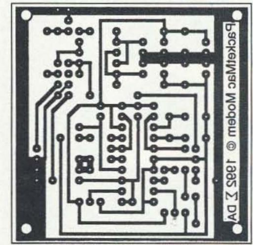
Figure 5. Inverted PC board foil pattern for use with TEC-200 film only. This pattern will eliminate the transparency inversion step required in the TEC-200 procedure. Do not use this foil pattern if using standard photographic methods (use Figure 2 instead).
