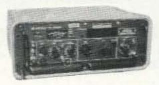
Rugged military version of HEWLETT-PACKARD 8640B; covers 500 KHz - 512 MHz AM/FM/Pulse in 10 ranges. Output: 0.013 uv to 2 V (-144 to +19 DBM). Modulation 400, 1K and 5K Hz. Has 6-digit display, phase-lock, external count capability and 50 W reverse power protection. Mounted in transit case; w/manual copy. Requires 108-127/207-242 VAC 48-440 Hz; 7.8x19.5x22.4, 70 lbs sh.
