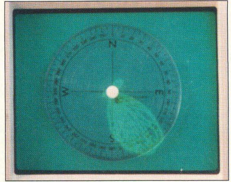
Photo D. Once 20 sweeps have built up on the storage scope, it's clear that the correct bearing is 145 degrees.
