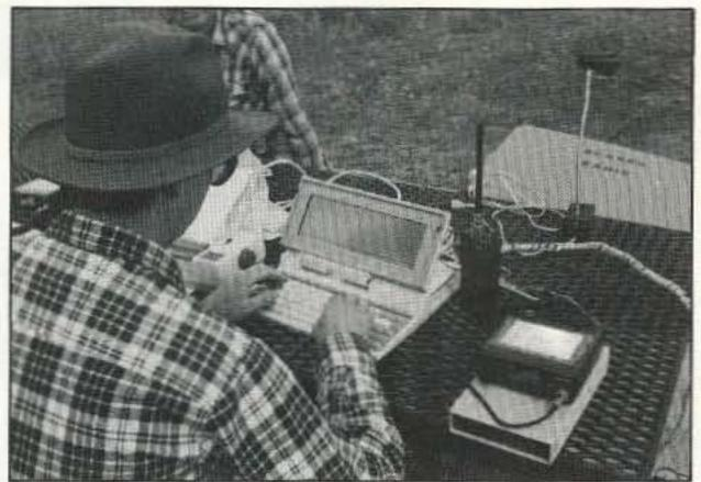
Photo B. Tim Groat KRØU transmits a packet message from the simulated fire line to the Boulder Public Safety building. Each packet field station consists of a laptop computer, printer, VHF radio, TNC and a gel-cell battery pack. Photo by David Fetter KA3HBK.
