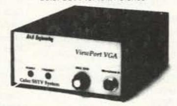
Features: Receives 8, 12, 24 and 36 B/W, 36 or 72 and M1, M2, S1, S2 FULL COLOR in REAL TIME, the pictures appear on the screen as received. Transmits 8, 12, 24, and 36 B/W and 36 or 72 COLOR. The software is shareware and was created by John Montalbano, KA2PYJ.
