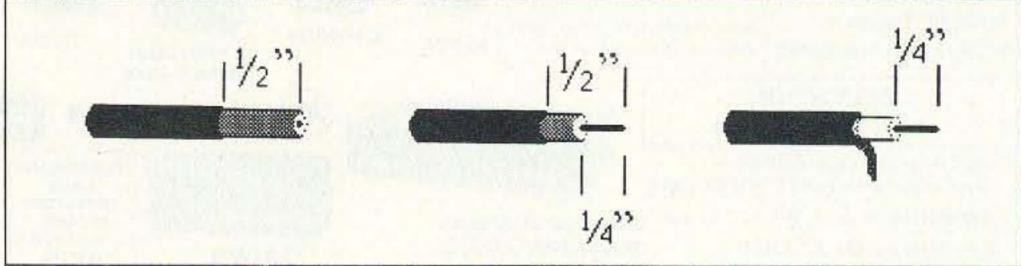
Figure 3. Preparation of the coaxial cables.
