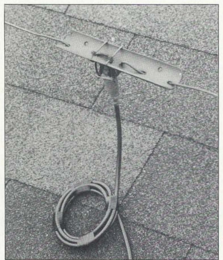
Photo C. The feed point of the baby loop antenna. A strip of PVC pipe (cut down the middle) was used to mount a SO-239 female connector and to support the antenna wire. Note also an RF air balun (1:1) formed out of coils of the feedline.
