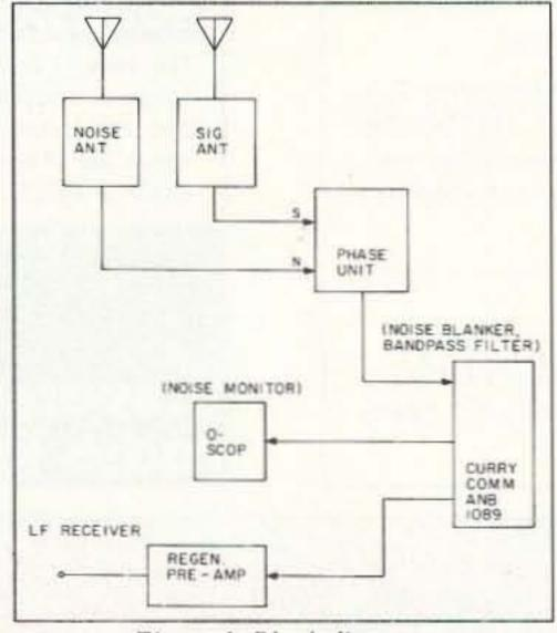
Figure 1. Block diagram.
