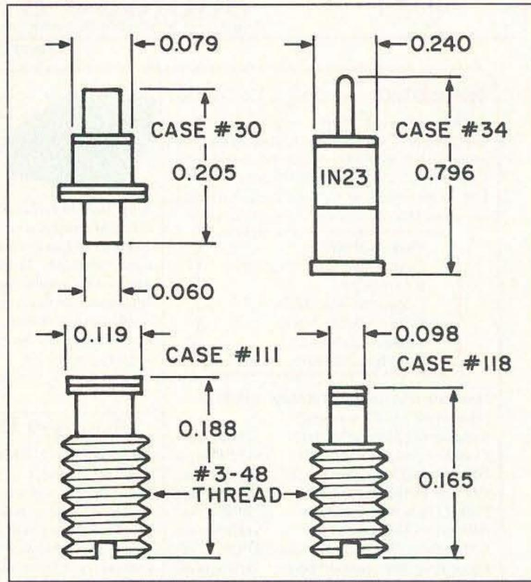
Figure 4. Various case styles for microwave diodes, detectors, and Gunn devices.
