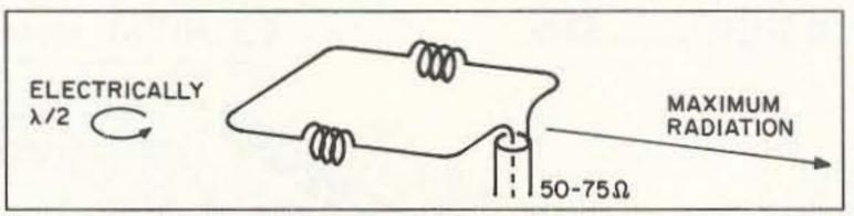
Figure 1. Diagram of the baby loop antenna.
