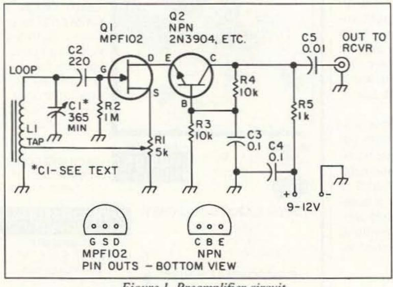
Figure 1. Preamplifier circuit.
