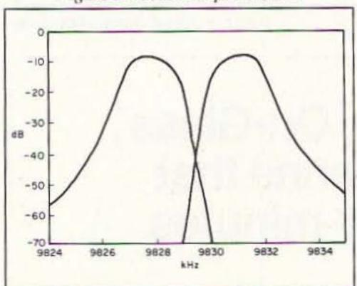
Figure 8. Calculated passbands with series resistance included.
