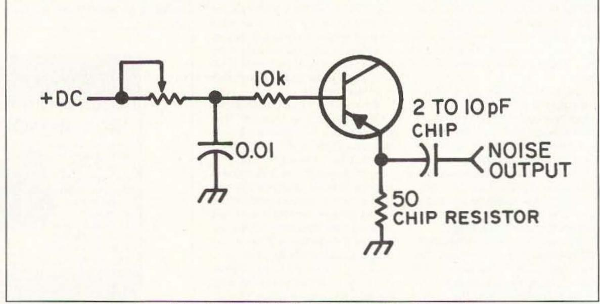
Figure 3. Possible alternative to the circuit shown in Figure 1 (see text).
