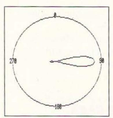
Figure 3. Rotating a high gain beam produces this pattern on the computer screen when there are no fluctuations, reflections, or multipath. (Of course, this never seems to happen on an actual hunt!)
