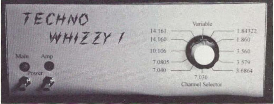
Photo A. The front panel of the Techno-Whizzy I DDS transmitter.
