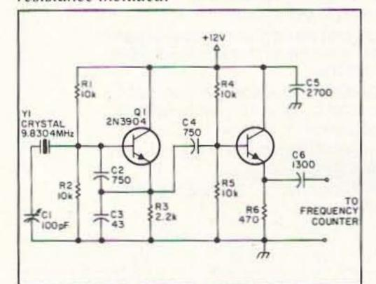
Figure 9. Oscillator circuit for use as a BFO or transmitter carrier.
