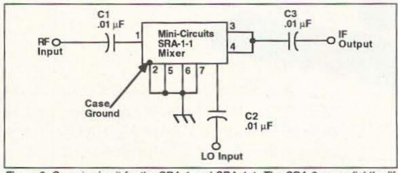
Figure 3. Generic circuit for the SRA-1 and SRA-1-1. The SRA-2 uses slightly different pinouts.
