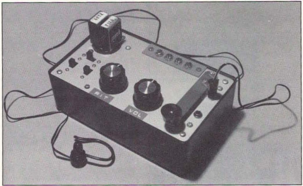
Photo A. The SP-1 portable CW transceiver.
