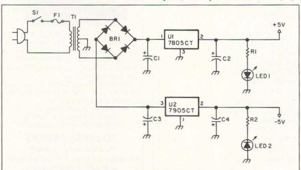
Figure 4. Schematic diagram of the +/- 5 volt power supply.
