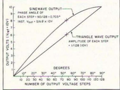
Figure 3. Comparison of one-quadrant output voltages from a DAC.
