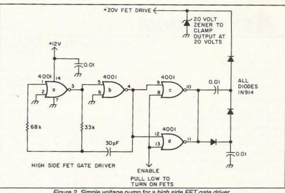
Figure 2. Simple voltage pump for a high side FET gate driver.
