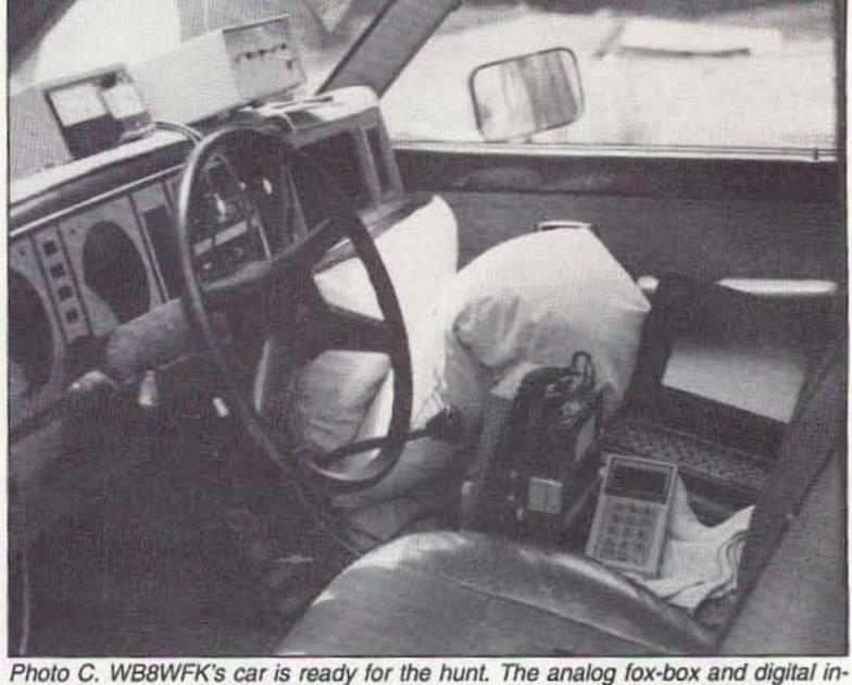
Photo C. WB8WFK's car is ready for the hunt. The analog fox-box and digital interface unit are on the dash. The computer (protected by pillows) has replaced a human in the passenger's seat. (Photo by WB8WFK.)
