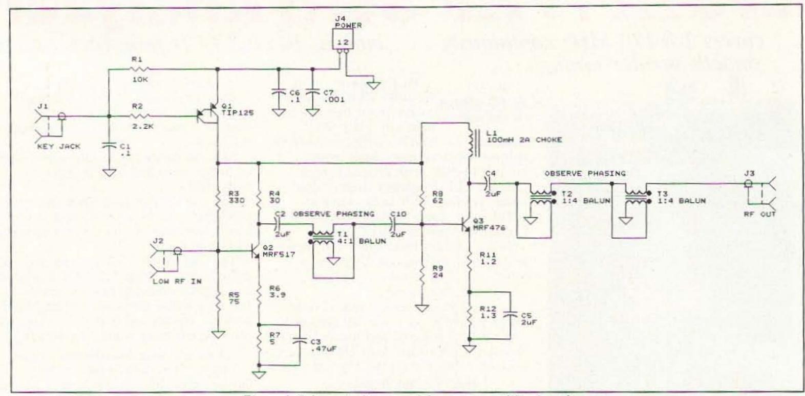
Figure 1. Schematic diagram of the power amplifier board.
