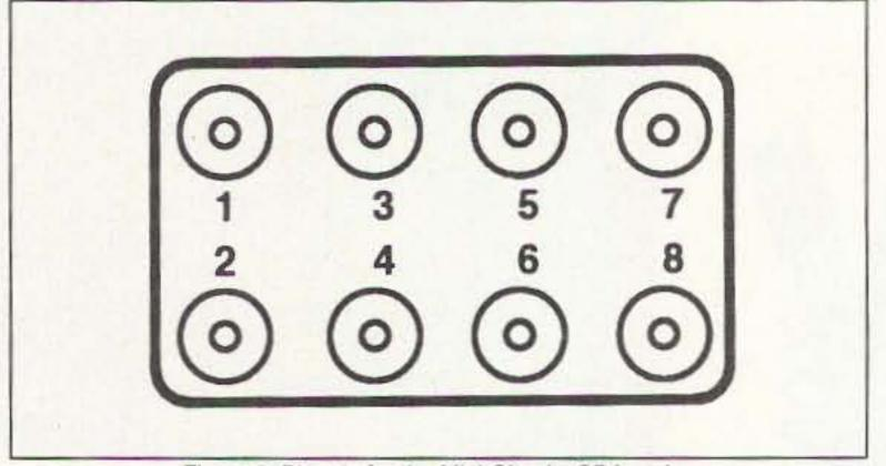
Figure 2. Pinouts for the Mini-Circuits SRA-series.
