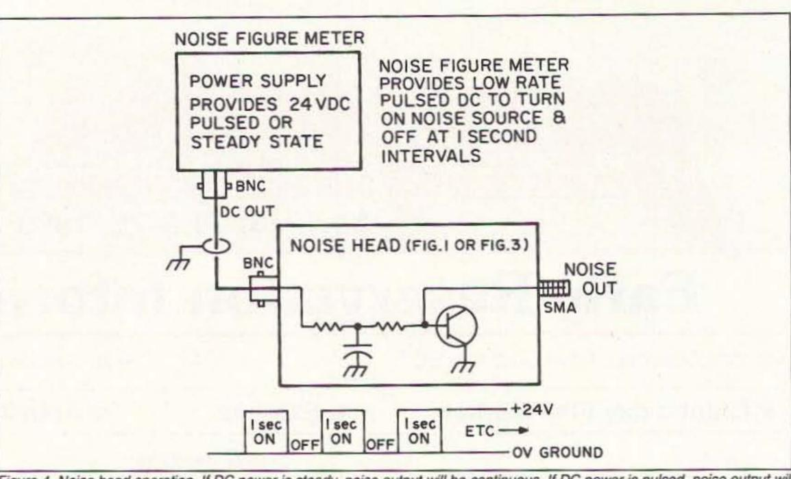
Figure 4. Noise head operation. If DC power is steady, noise output will be continuous. If DC power is pulsed, noise output will be pulsed. A pulsed noise source is useful to determine the difference between noise to no noise for the noise figure ratio.
