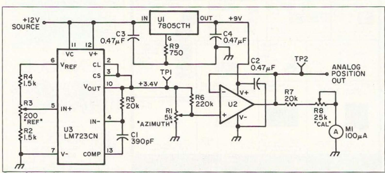
Figure 1. Schematic of the antenna position display unit. R1 is the continuous-turning potentiometer. M1 indicates direction. The analog output goes to the MUX and A/D converter.
