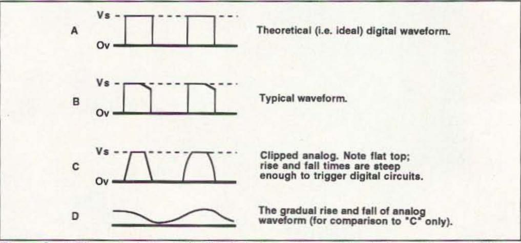
Figure 3. a) Theoretical (i.e. "ideal") digital waveform. b) Typical waveform. c) Clipped analog. Note flat top; also, rise and fall times ("up" and "down" ramps) are steep enough to properly trigger digital circuits. d) Note gradual rise and fall of analog waveform (for comparison only to diagram "c").
