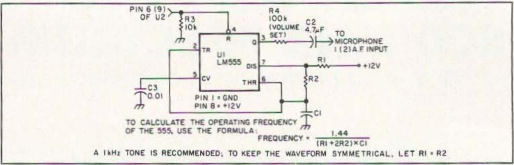
Figure 2. Audio oscillator circuit for use in a modulated CW beacon application.
