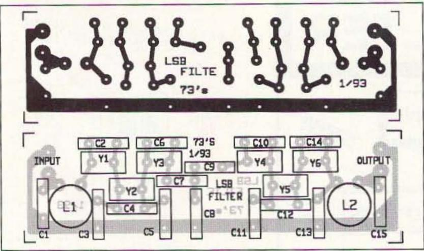
Figure 4 (a). PC board foil pattern for the lower sideband filter. (b). Parts placement diagram.
