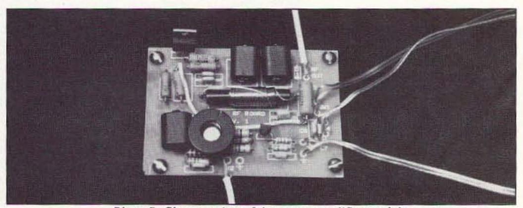
Photo B. Close-up view of the power amplifier module.
