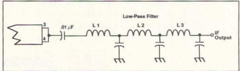
Figure 4. Low-pass filter output circuit.
