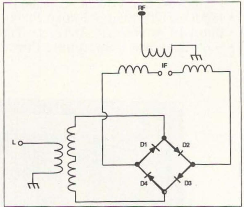
Figure 1. Circuit for a double-balanced mixer.
