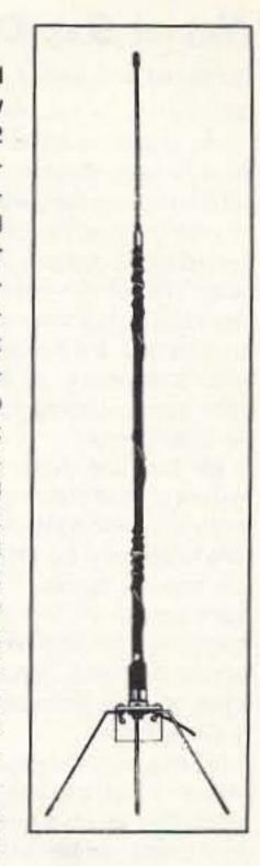
radials, 21" long, attached underneath the bracket with screws. The total height after assembly is 10-1/2 feet.
