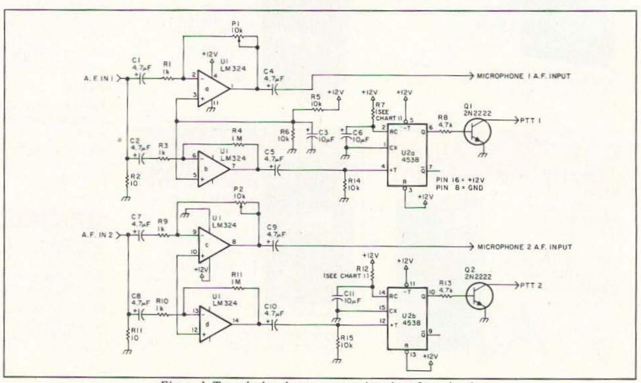
Figure 1. Tape deck to beacon transmitter interface circuit.
