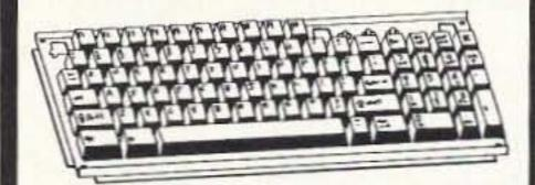
Honeywell# 85ST23-L-J. 85 key computer-type keyboard. Standard QWERTY keyboard with 10 function keys across the top and number pad on right side with other function keys. Solid 14" X 5" metal frame. Charcoal keys with white lettering. Terminates to two vinyl ribbon cables, 25 conductors. Logic board with 3 green leds can be easily removed if desired.
