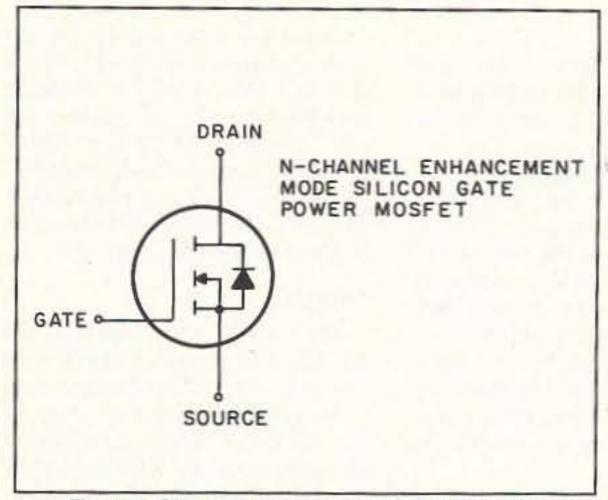
Figure 1. Schematic drawing for a power MOSFET.
