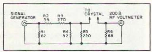
Figure 3. 50-ohm test circuit.
