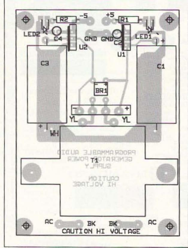
Figure 8. Parts placement for the power supply.
