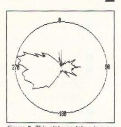
Figure 5. This plot was taken in a supermarket parking lot on an Albuquerque T-hunt. The spikes at zero degrees represent noise from power lines ahead of the vehicle. The hidden T is to the left and there is reflected signal from the right.
