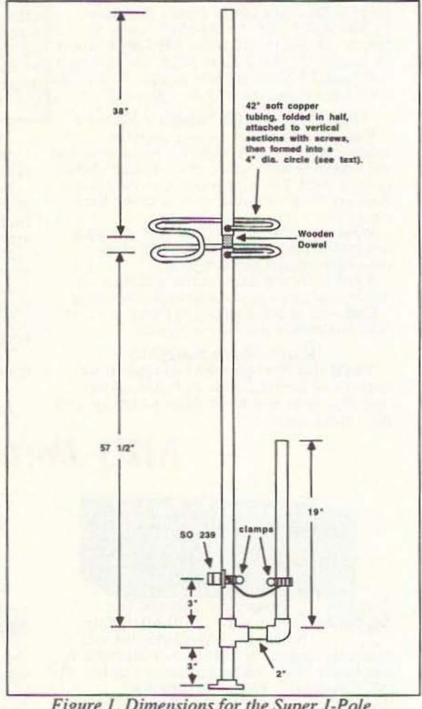
Figure 1. Dimensions for the Super J-Pole.
