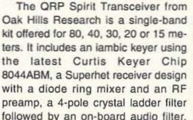
and a switchable HP AGC circuit with manual RF gain control. It also offers 2 watts of audio output with an external speaker jack, VFO tuning with an 8:1 vernier dial covering 100 kHz and RIT, and a sine wave oscillator with frequency and level controls. The kit measures 4" x 6-1/4" x 6-7/8" and weighs 47 oz.
