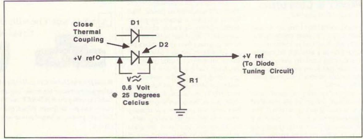
Figure 5. Simple diode thermal compensation circuit.
