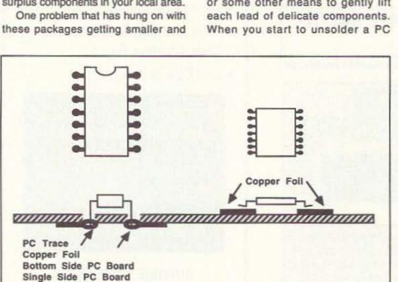
Figure 1. Standard 14-pin DIP, compared to a surface mount IC. The 14-pin DIP mounts through holes drilled in the PC board. Surface mount means just that—it is soldered on the component side of the PC board (no holes).
