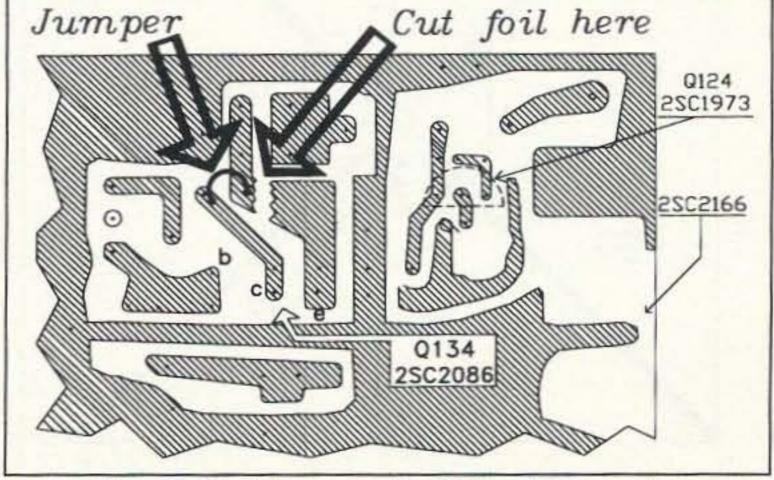
Figure 2. Modifications to the PC board, bottom view.
