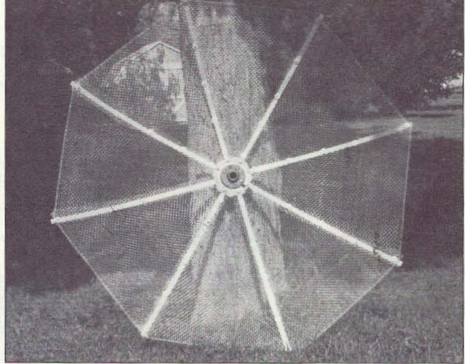
Photo B. Hardware cloth mesh attached to ribs.
