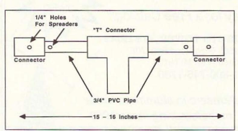
Figure 1. Boom construction.
