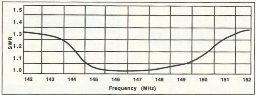
Figure 2. Antenna SWR curve chart for 142-152 MHz.
