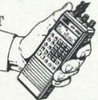
coverage 1300MHz 500KHz to programmable hand held. Ten scan banks, ten search banks. Lockout on search and scan. AM plus narrow and broadcast FM. Priority, hold, delay and selectable search increment of 5 to 995 KHz. Permanent memory. 4 AA ni-cads and wall plus cig charger included along with belt clip, case, ant. & earphone. Size: 6 7/8 x 1 3/4 x 2 1/2. Wt 12 oz. Fax fact document # 205
