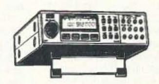
Five banks of 20 channels each. Covers 29-54, 118-174, 406-512 and 806-954MHz (with cell lock). Features scan, search, delay, priority, CTCSS option, lockout, service search, & Includes AC/DC cords, mounting keylock. bracket, BNC antenna. Size: 4 3/8 x 6 15/16 x 1 5/8. Weight: 4.5lbs. Fax fact document #550
