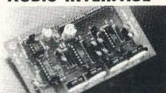
Detailed application manual Low power operation, 19ma @ 12v CTCSS decoder on the UAI-20 only Assembled, tested, one year warranty Link monitor-mix/monitor mute control Adjustable repeater/link/DTMF audio outputs Selectable DTMF mute on repeater and link audio Repeater, link, auxiliary and control audio inputs
