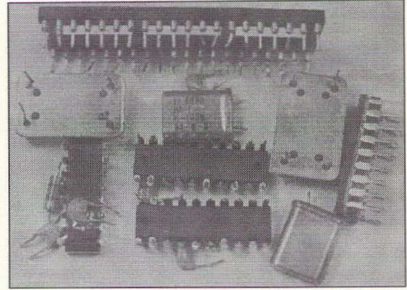
Photo A. Components removed with a heat gun. Note the clean pins, even on a 40-pin socket removed from a 386-25 PC board. The 20-pin chips under the 16 MHz crystal show dirty solder leads. These chips were pulled too soon—not all of the solder was allowed to flow before the chip was pulled.
