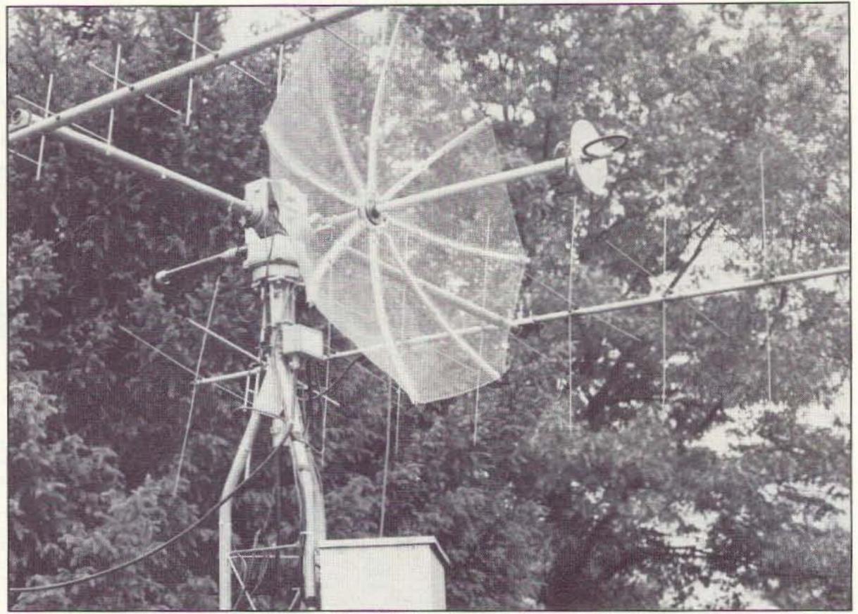
Photo C. Completed dish in place on the rotating bar.
