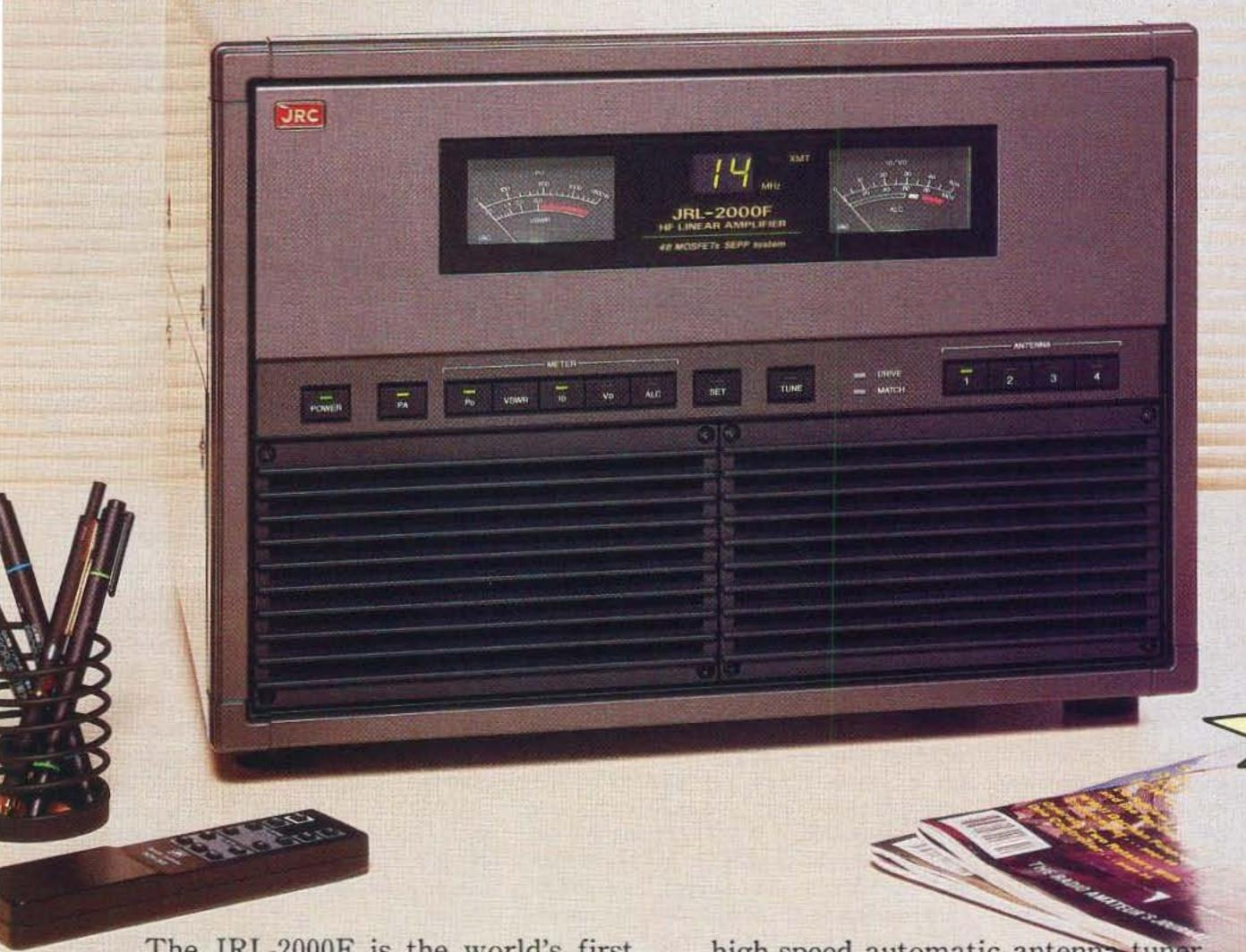
The JRL-2000F is the world's first MOSFET HF linear amplifier, designed using the same high technology found in JRC's professional high-power radio transmitters. Featuring a heavy-duty power amp that incorporates 48 RF power MOS-FETs to ensure low distortion and clean output up to 1,000 watts (100% duty cycle, 24 hour) SSB/CW, plus a
