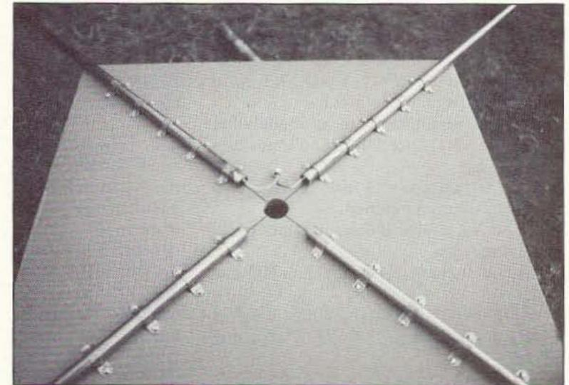
Photo B. Close-up of the coax connector soldered to the driven element arms.
