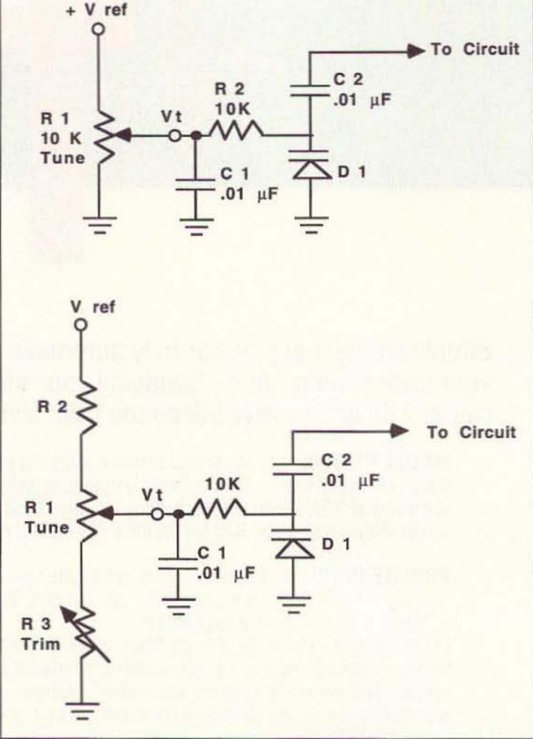
Figure 3. Varactor diode tuning voltage circuits.
