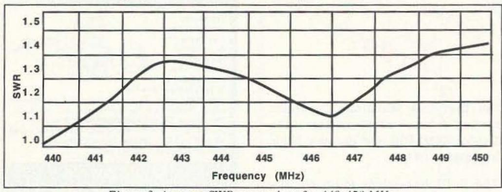
Figure 3. Antenna SWR curve chart for 440-450 MHz.
