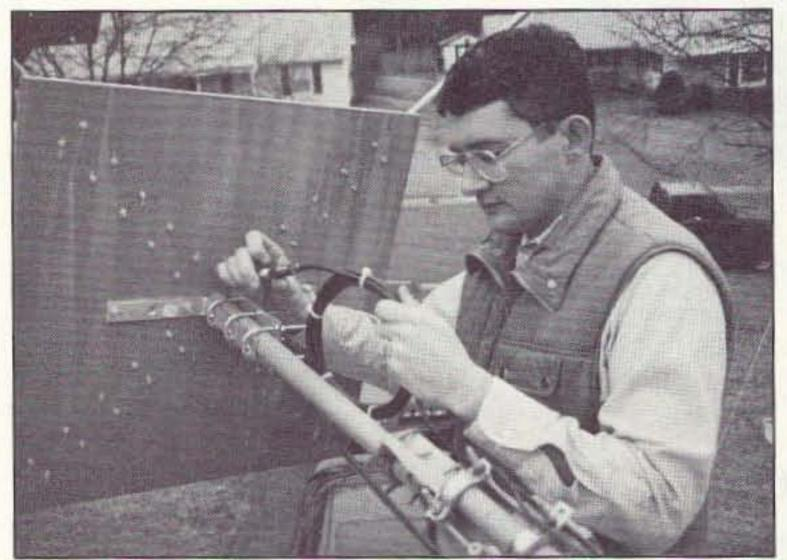
Photo E. Bottom view of center board. John making current balun (RF choke).
