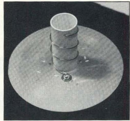
Photo E. Helix mounted to the tubing.
