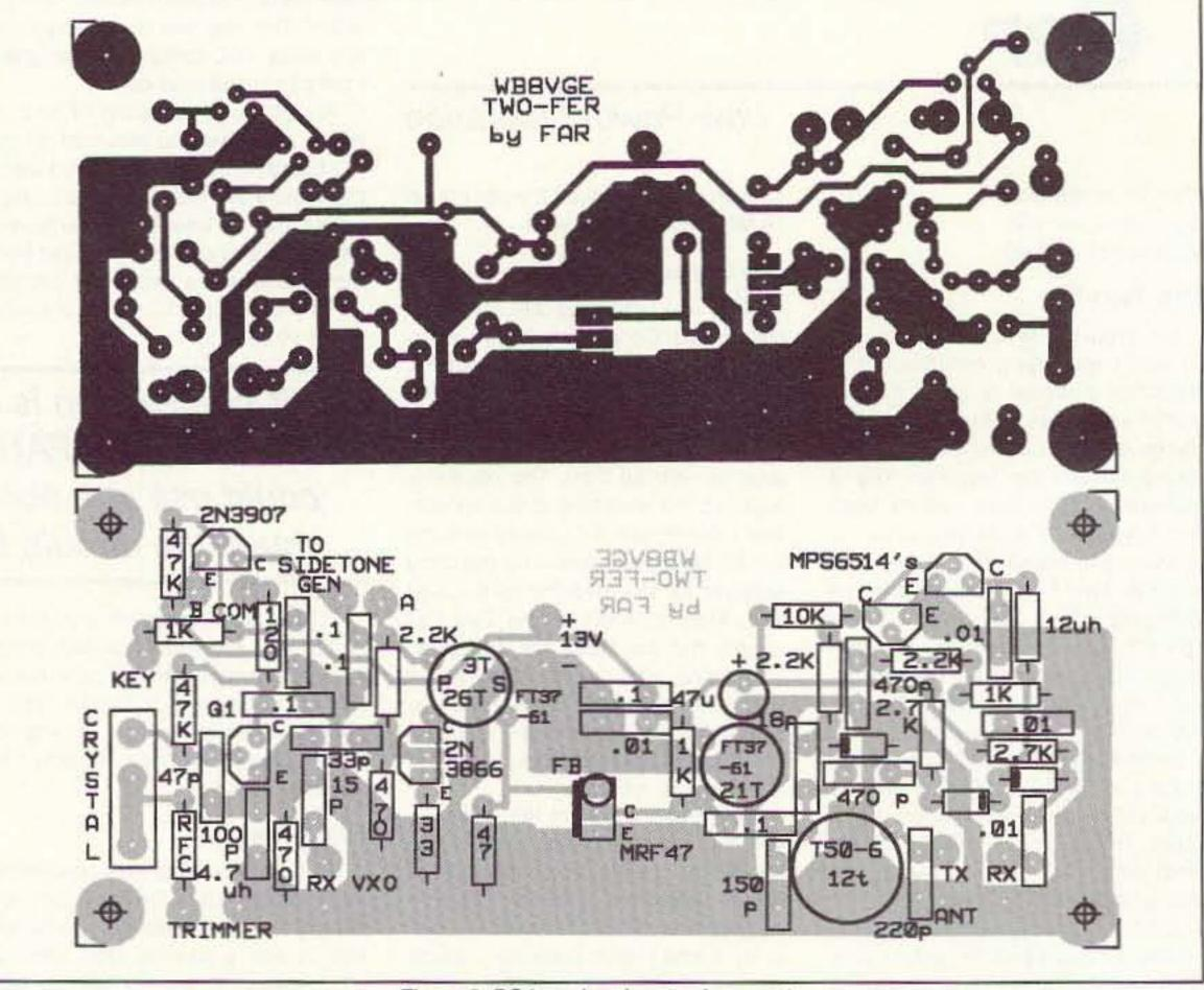
Figure 2. PC board and parts placement.
