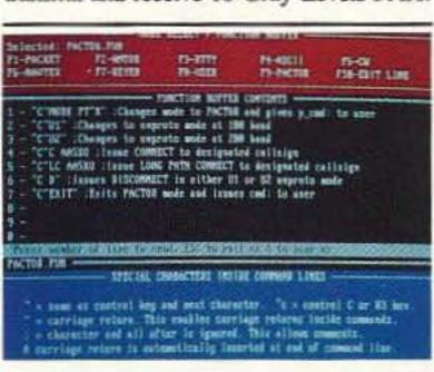
Easy and simple . . . MultiCom<sup>TM</sup> Operating menu-each mode gives you 10 programmable function buffers.
