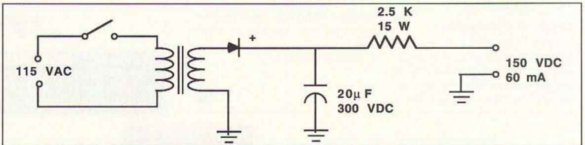
Figure 3: Basic RTTY Loop supply circuit.
