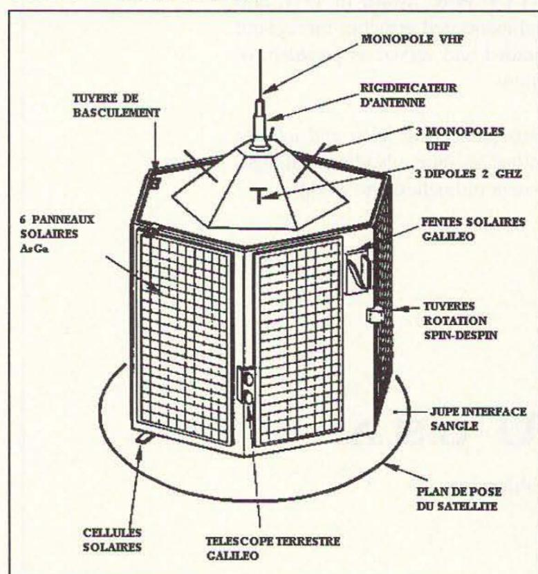
Figure 1. External ARSENE configuration.
