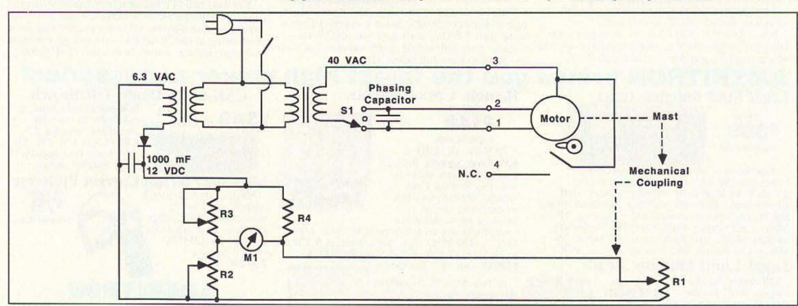
Figure 2. Simple "manual" controller and display. S1 is a center-off toggle. R1 and R2 should be equal, approximately 10k; R3 and R4 should be equal, approximately 5k. M1 should be 0-1 mA, up to 0-10 mA. If a less sensitive meter is used, decrease R1-R4. Adjust R2 and R3 for zero and full scale as R1 varies over its range. Duplicate the circuit if a second rotator is used.
