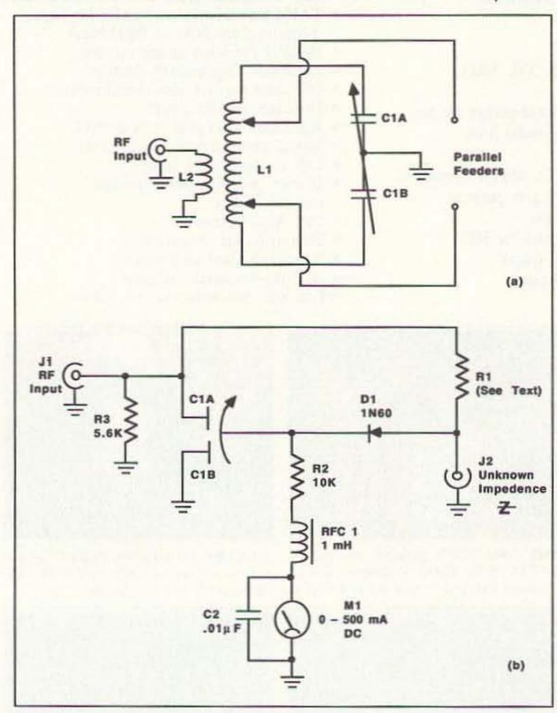
Figure 2. A) ATU circuit using split-stator capacitor; B) Antenna RF bridge using differential capacitor.
