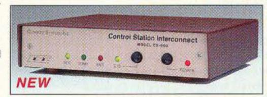
in unsurpassed simplex performance. A 90 memory speed-dialer and Remote base mode are also included. The only required connections are to the Mic and Speaker jacks of your simplex transceiver. Fully FCC and DOC approved. This is the best deal going in a simplex patch!
