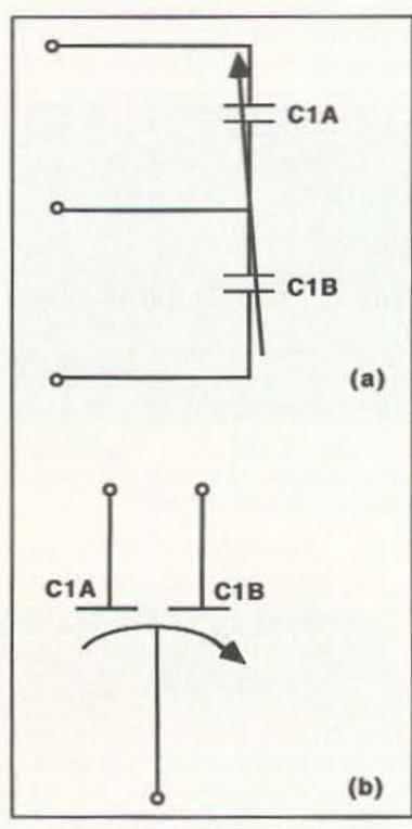
Figure 1. A) Split-stator capacitor symbol; B) Differential capacitor symbol.
