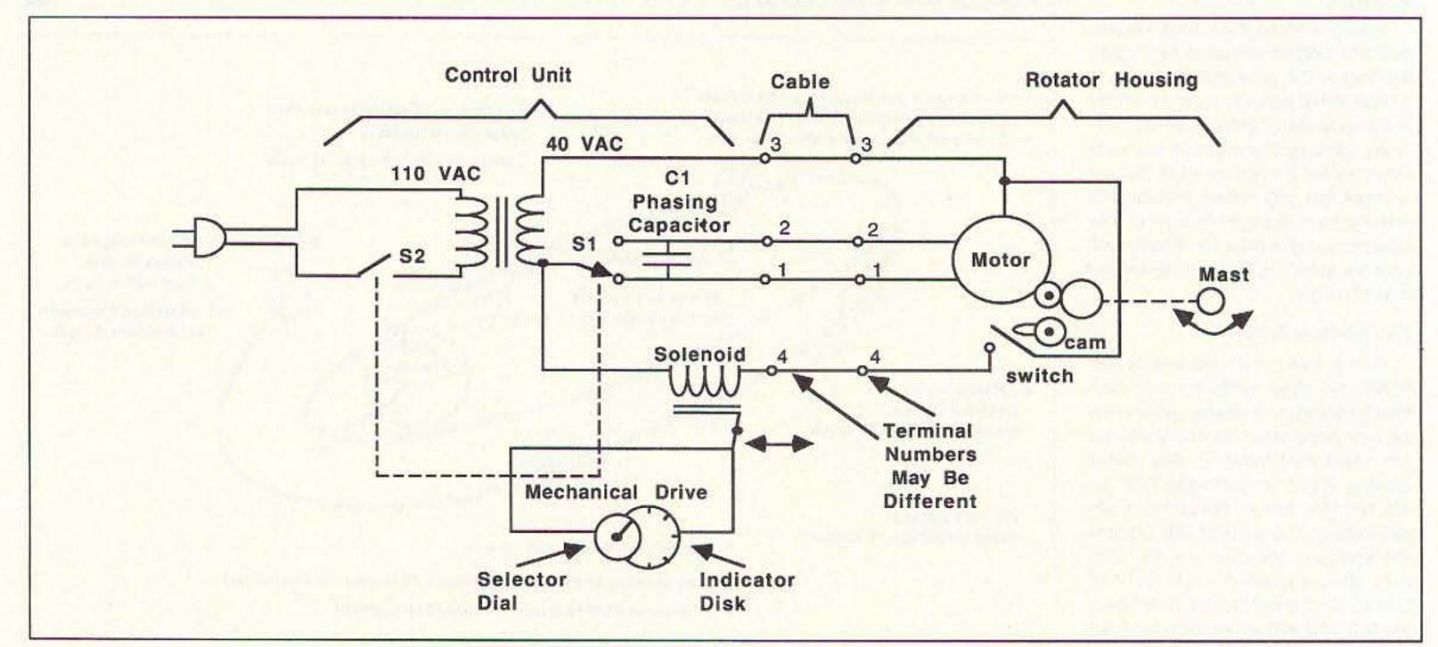
Figure 1. Typical rotator and control box.
