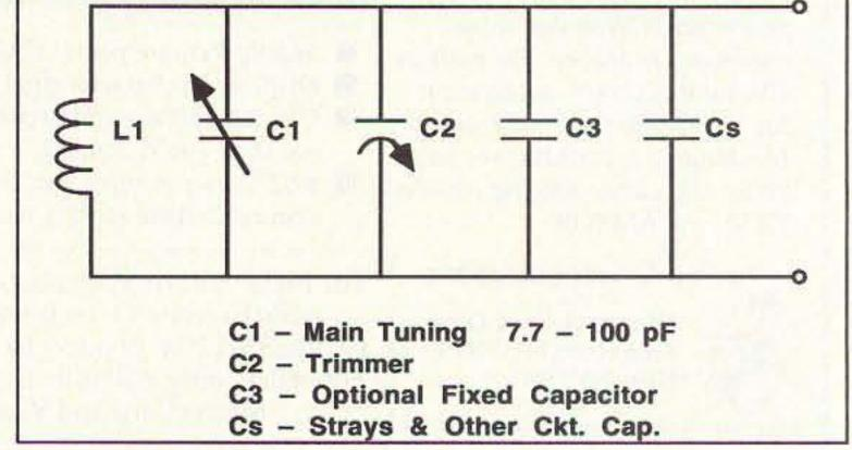
Figure 3. L-C resonant tank circuit for example calculations.
