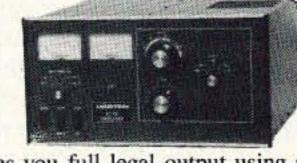
This linear gives you full legal output using a pair of Eimac 3-500Zs. Some competing linears using dual 3-500Zs don't give you 1500 watts the tubes to their full potential.
