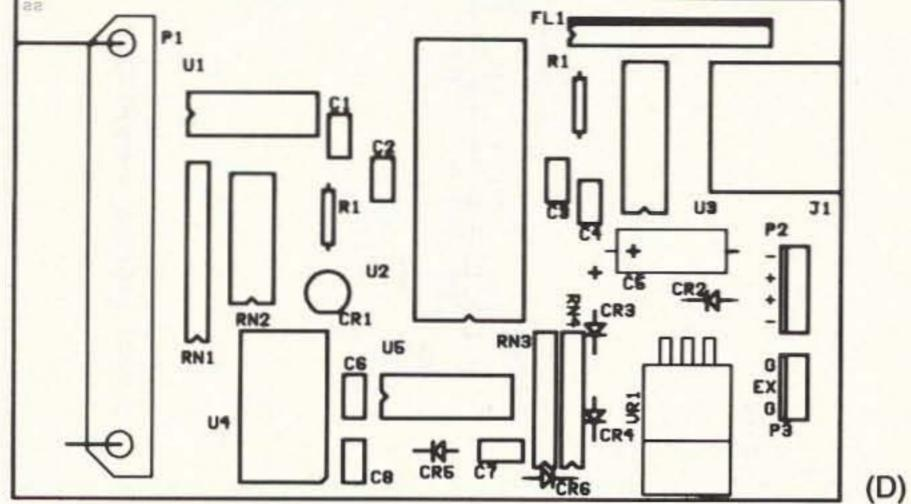
C) PC drilling template; D) parts placement diagram.
