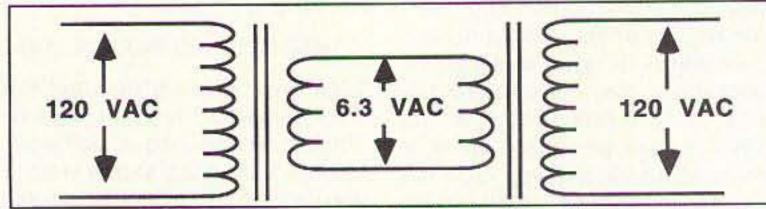
Figure 2: Line Isolation with back-to-back transformers.
