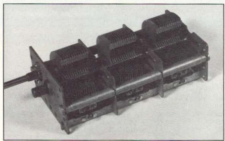
Photo B. Three-section 3X-365 pF variable capacitor.
