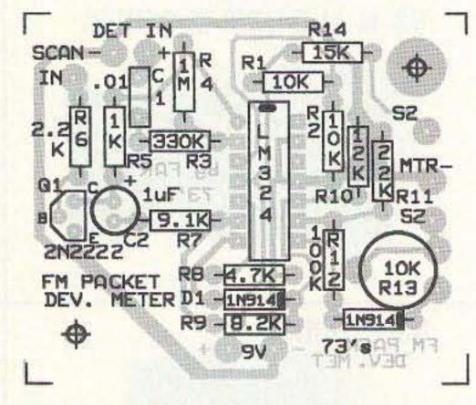
Figure 2. PC board pattern and parts placement diagram.
