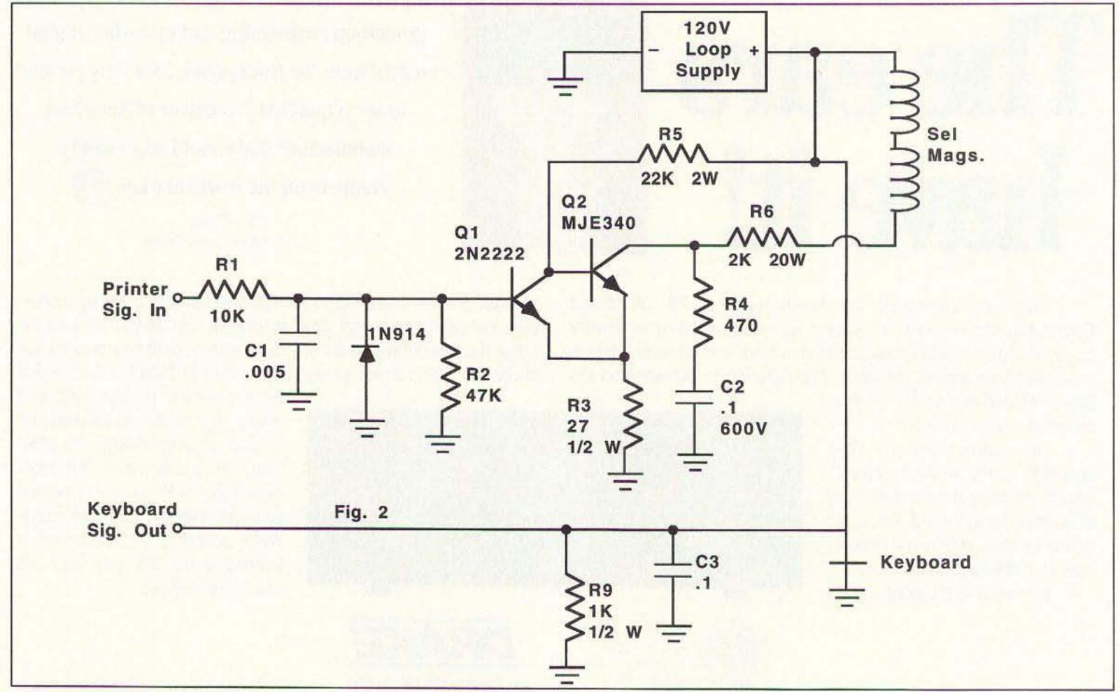
Figure 1: Selector Magnet Driver Circuit.
