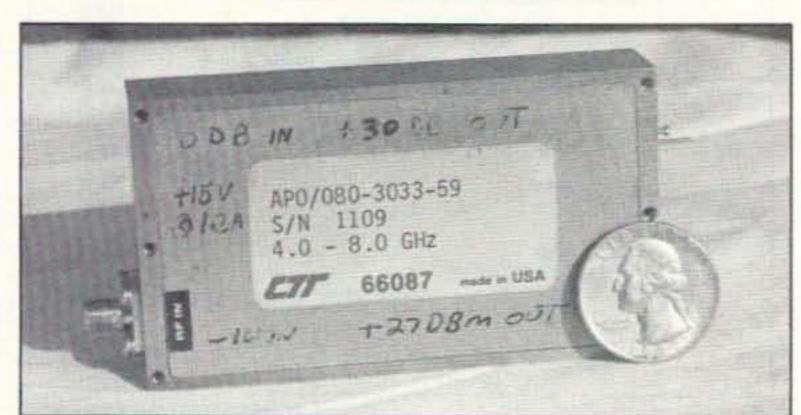
Photo C. A compact CIT 4.0 to 8.0 GHz, 1 watt amplifier.
