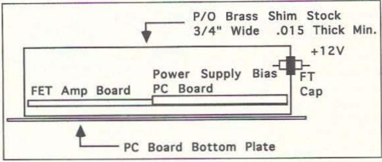
Figure 2. Amplifier container construction. Solder the bottom of the PC boards to brass shim stock sides. Solder amp PC board and bias PC power supply board together. Locate the holes for coaxial connectors for the amp and feedthrough cap for the power supply before soldering the boards together. Use aluminum foil or copper foil for the top of the container.
