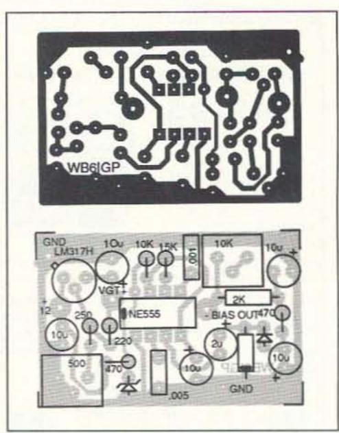
Figure 4. PC board layout and parts placement diagram. Drilled and etched PC boards are available for \$3.50 plus \$1.50 S&H from FAR Circuits, 18N640 Field Ct., Dundee IL 60118.
