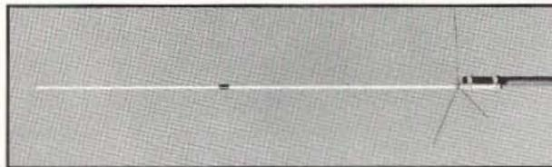
CX-902 Tri-Band 146/446/1200 MHz Gain & Wave: 146MHz 6.5dB 5/8 wave x 2 446MHz 9.0dB 5/8 wave x 3 1200MHz 9.0dB 5/8 wave x 5 VSWR: 1.5:1 or less Max Power: 200 watts Length: 10' Weight: 3 lbs. 3 ozs. Connector: N-Type Construction: Fiberglass. 2 sections
