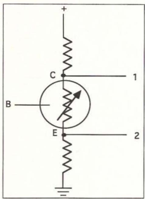
Figure 3. Another theoretical model for a transistor is composed of resistors. This model is like a potentiometer with the base-fed signal wiggling the wiper.
