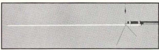
CX-725 Tri-Band 50/146/446MHz Gain & Wave: 50MHz 2.15dB 1/2 wave 146MHz 6.2dB 5/8 wave x 2 446MHz 8.4dB 5/8 wave x 4 VSWR: 1.2:1 or less Max Power: 200 watts Length: 7' 6" Weight: 3 lbs. Connector: SO-239
