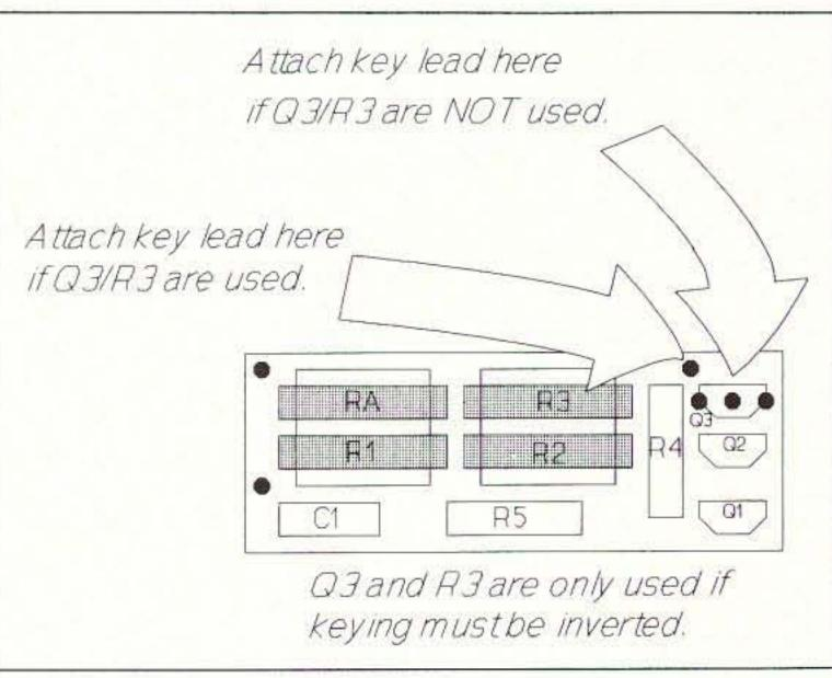
Figure 7. Key wire placement on completed Micro IDer.
