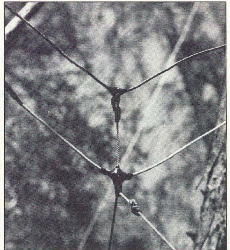
Photo B. The bottom apex of the Hula Loop's diffector. Note that nylon cord is used to secure the antenna.
