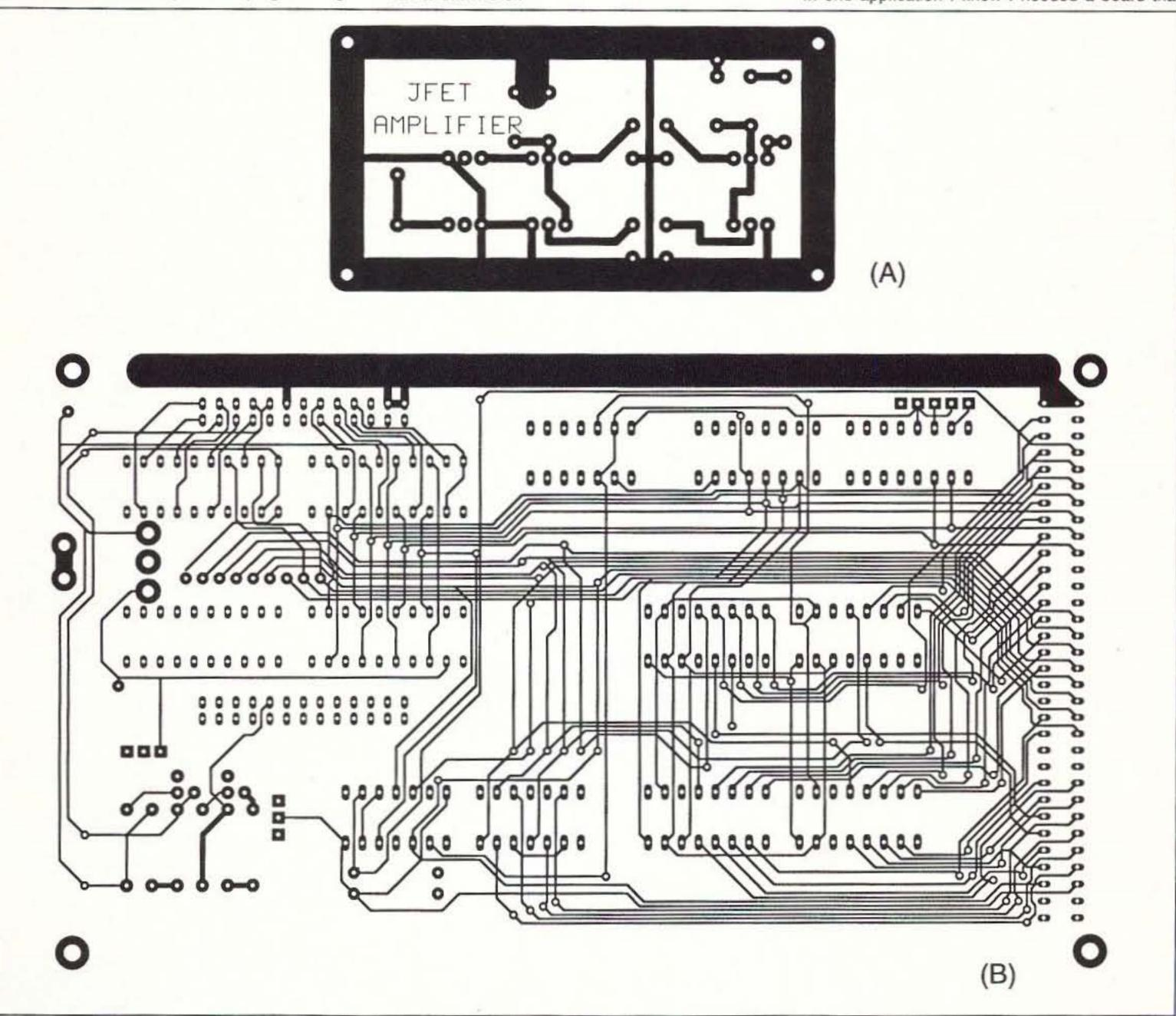
Figure 4. A) JFET preamplifier PCB I designed; B) Complex board from the tutorial package of EASY-PC.
