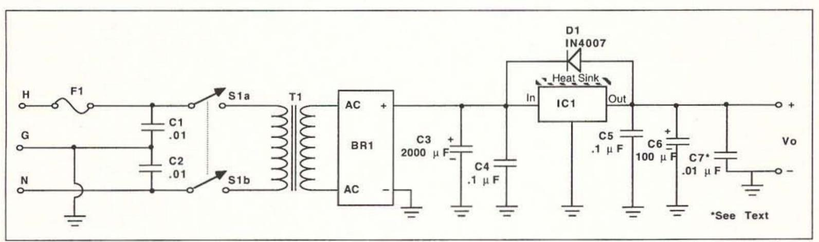
Figure 2. Circuit for the basic voltage regulator power supply.
