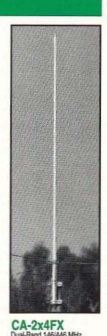
Impedance: 50 ohms VSWR: Less than 1.5:1, 144-148MHz 440-450MHz Max Power: 200 watts Length: 5' 11" Weight: 2 lbs. 12 ozs. Mounting Mast Dia: 1 1/2 - 2 1/4" Connector: SO-239 Construction: Heavy duty fiberglass
