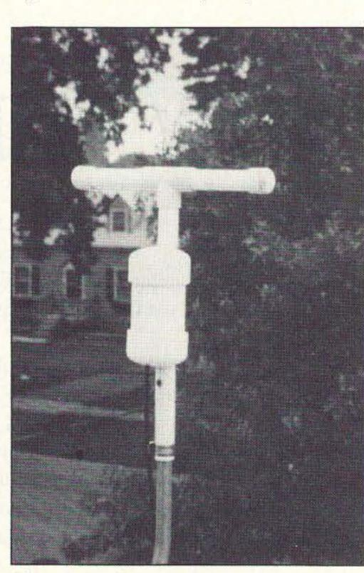
Photo B. Outdoor version of rod antenna and preamp in waterproof housing.
