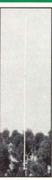
446MHz 9dB 1/2 wave x 12 VSWR: 1.5:1 or less Max Power: 200 watts Length: 10' 5" Weight: 3 lbs. Mounting Mast Dia: 1 1/2 - 2 1/2" Connector: N-Type Construction: Heavy Duty Fiberglass
