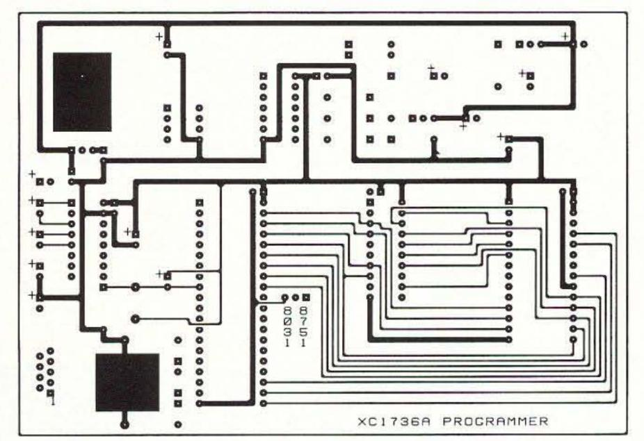
Figure 6. Programmer component side circuit pattern @ 70%.
