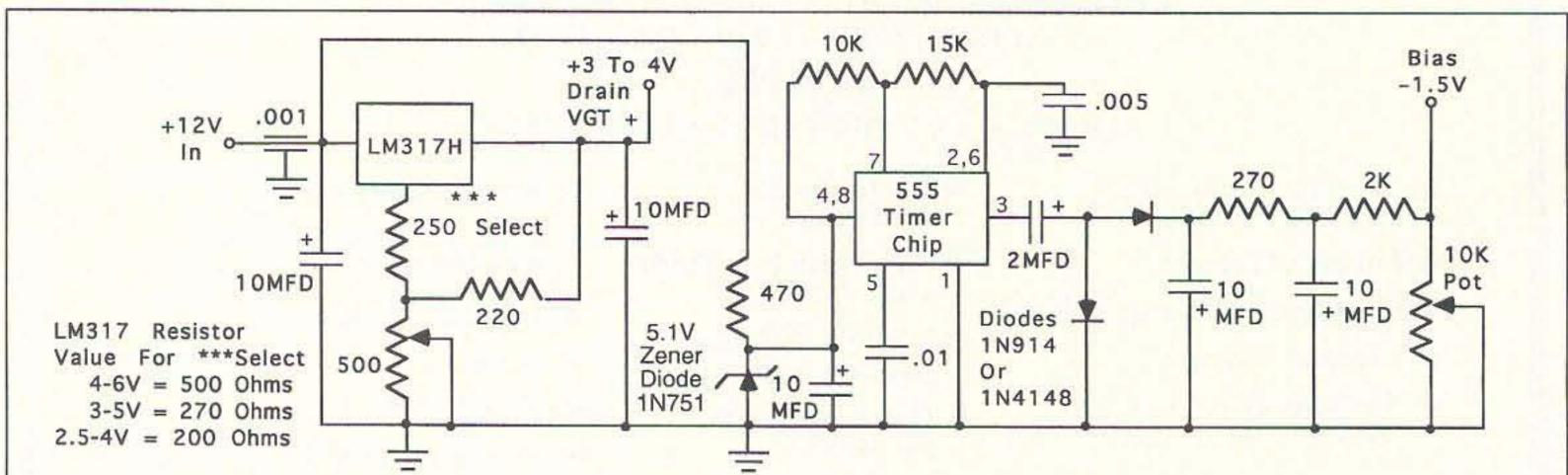
Figure 1. Schematic for bias power supply. Adjust positive voltage with selection of LM317 resistor as indicated by \*\*\*. Note: 470 ohm resistor at the imput of the 555 chip (pins 4 & 8) is mounted on the PC board to +12 volts. This maintains a stiff -1.5 volts bias output at minimum pot output from the negative bias supply.
