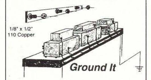
Solid Copper Buss Stainless Steel Hardware Grounding Stud Every 6 Inches Top or Back Installation
