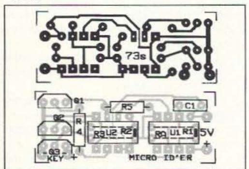
Figure 2. Parts placement outline and circuit board pattern.
