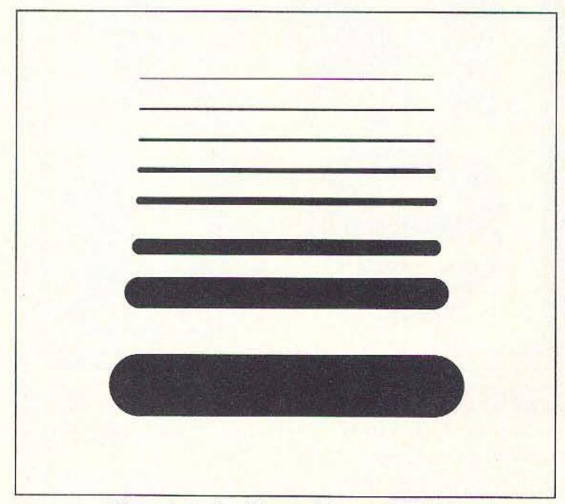
Figure 1. Track widths available on EASY-PC.
