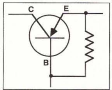
Figure 4. A common configuation for a PNP transistor includes a resistor connecting the emitter to the base.
