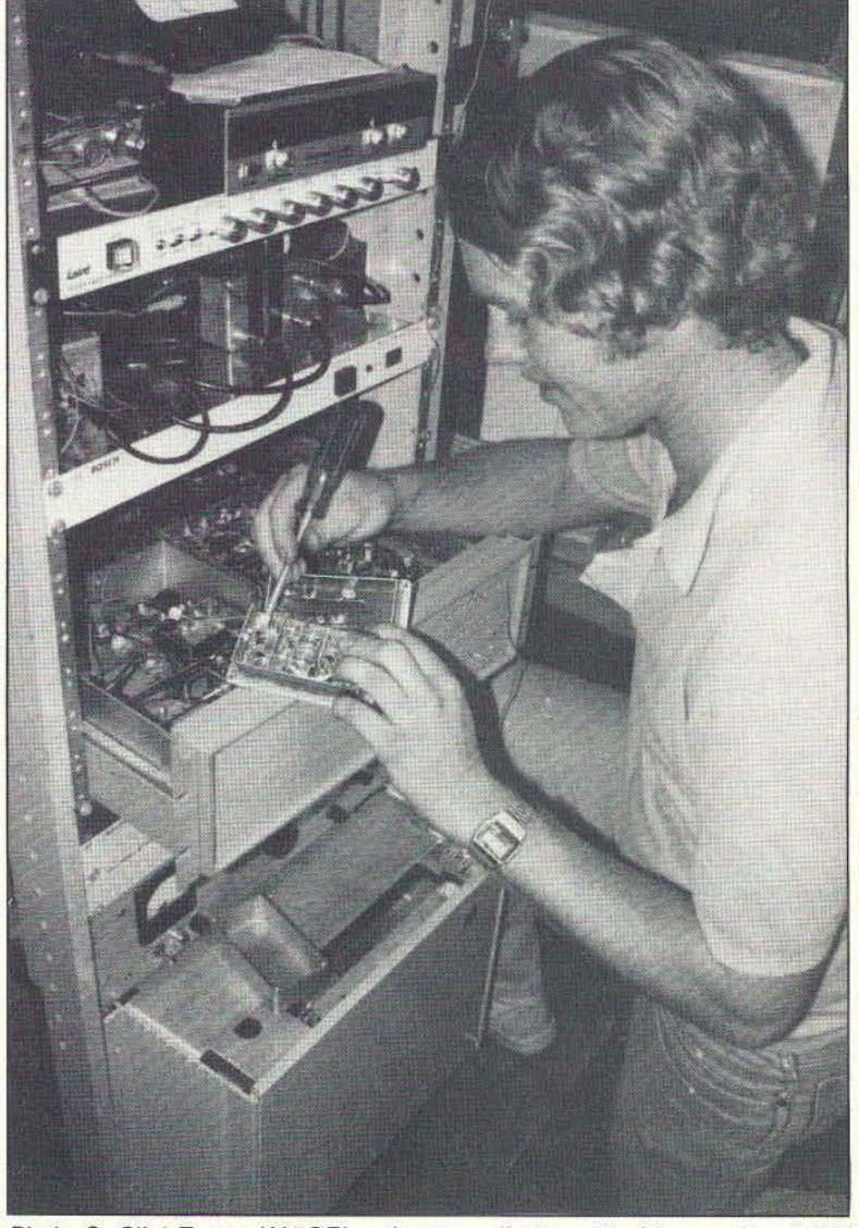
Photo C. Clint Turner KA7OEI makes an adjustment to his crossband ATV repeater located in the radio club of the University of Utah.
