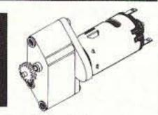
Excellent motor for displays, robotics and other mechanical applications. No load ratings: 48 RPM @ 6 Vdc 92 RPM @ 12 Vdc. Motor dimensions: 1.08" diameter X 1.4" long. Gearhead dimensions: 1.34" X 0.93". Final drive shaft is 1/8" diameter X 0.35" long. A 0.55" diameter gear is press-fit onto the shaft.
