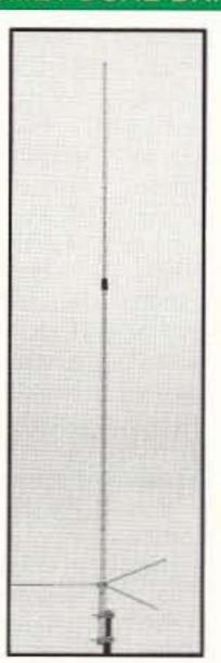
146MHz 6.5dB 5/8 wave x 2 446MHz 9.0dB 5/8 wave x 5 VSWR: Less than 1.5:1, 144-148MHz 440-450MHz Max Power: 200 watts Length: 10' 2" Connector: SO-239 Construction: Heavy duty fiberglass, 2 sections
