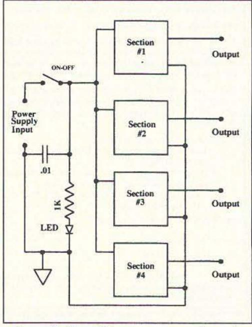
Figure 2. Quad Charger system schematic.
