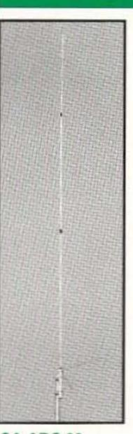
CA-ABC 23 146MHz 7.8dB 5/8 wave x 3 VSWR: 1.5:1 or less Max Power: 200 watts Length: 13' 4" Weight: 3 bs. 8 ozs. Mounting Mast Dia: 1 - 2 1/2" Connector: SO-239 Construction: All Aluminum
