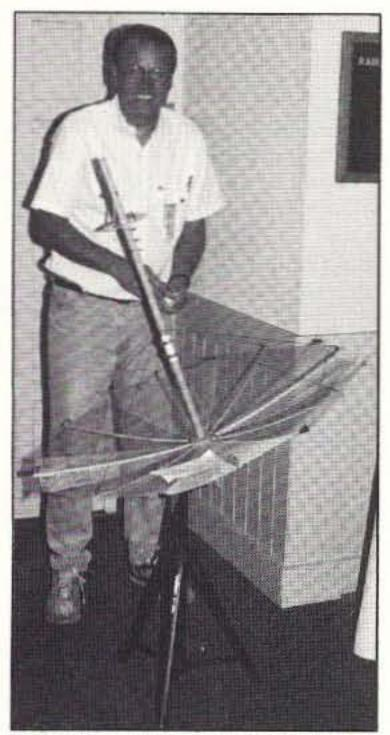
Photo D. Ed Krome KA9LNV demonstrated his portable 2.4 GHz receive system for Mode "S" via OSCAR-13.
