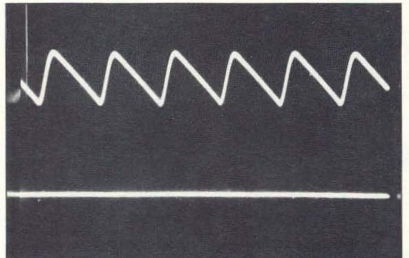
Photo A. Top trace is ripple at the input of the regulator, and the bottom trace is
