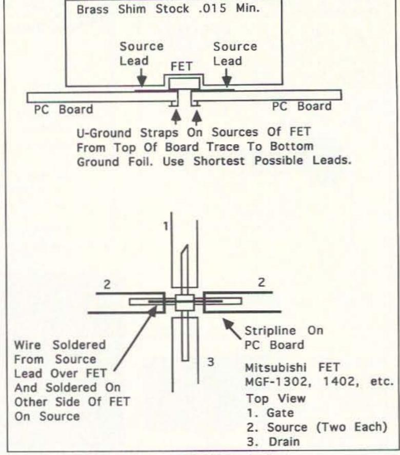
Figure 3. FET shielding details.
