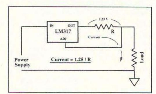
Figure 1. LM317 as a constant current source.
