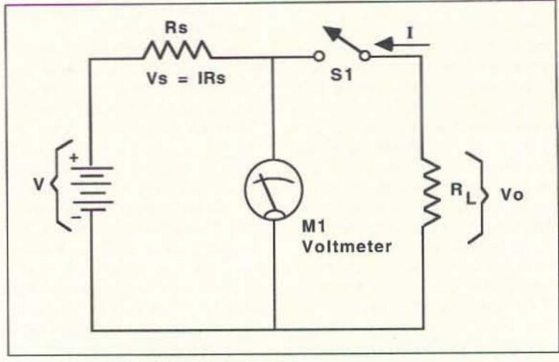
Figure 1. Equivalent circuit showing how voltage variation occurs.
