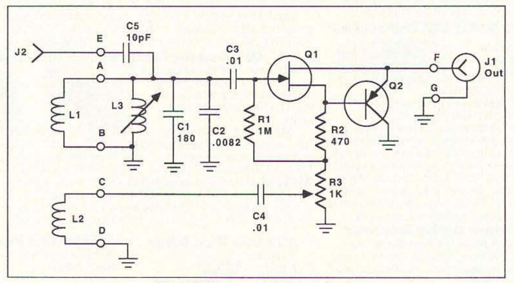
Figure 2. The antenna/preamp circuit.
