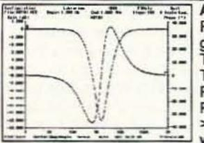
ANALYSER III and ANALYSER III Pro. Powerful linear circuit simulators have full graphical output, handle R's,L's,C's, Bipolar Transistors, FET's, Op-Amp's, Tapped Transformers and Transmission Lines etc. Plots Input and Output Impedances, Gain, Phase and Group Delay. Covers 0.001 Hz to >10GHz. Runs on PC/XT/AT/286/386/486 with EGA or VGA displays.
