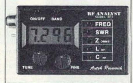
is 2.5% to 5% over most of its range. The instrument fits into a shirt pocket and runs on a 9 volt battery.
