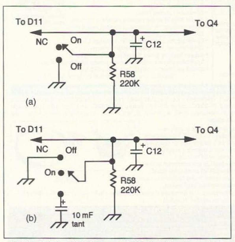
Figure 2. a) Simple AGC for the Argosy. b) ACG with fast/slow time constants.
