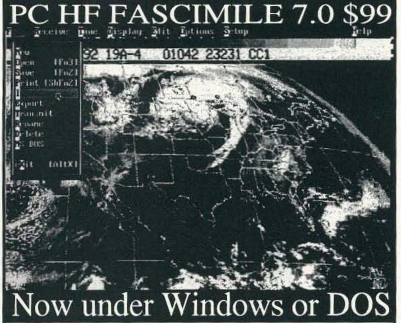
PC HF Facsimile is a simple, yet comprehensive shortwave fax system for the IBM PC and compatibles. It includes an FSK demodulator, advanced signal processing software, tutorial cassette, and complete reference manual. With your PC and SSB revelver getting FAX is a snap. Here are just some of the features:
