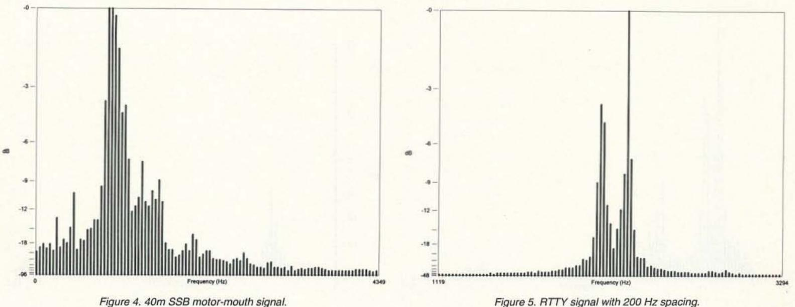
Figure 4. 40m SSB motor-mouth signal.
