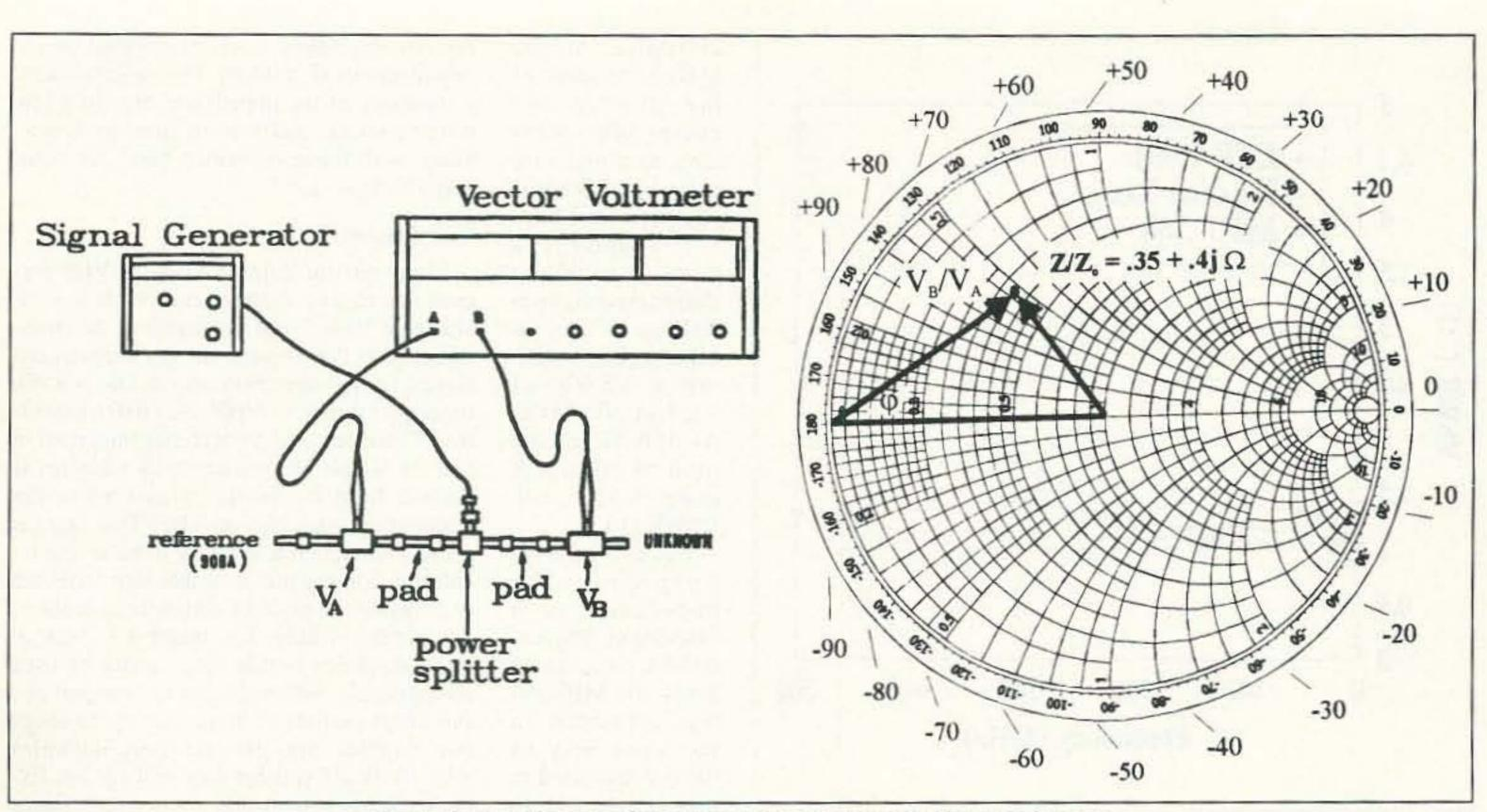
Figure 3. Complex impedance measurement using the Vector Voltmeter.
