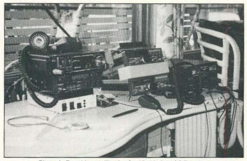
Photo A. Portable satellite rigs for 15, 10, 2 and 0.7 meters.
