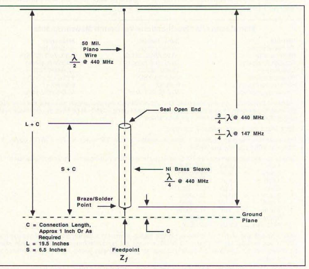
Figure 1. Detailed drawing of the dual-band antenna.
