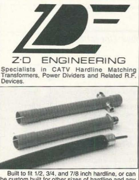
be custom built for other sizes of hardline and any frequency between 50 MHz and 1.3 GHz. When ordering, please include a 4 inch section of your hardline and specify the design frequency you need.
