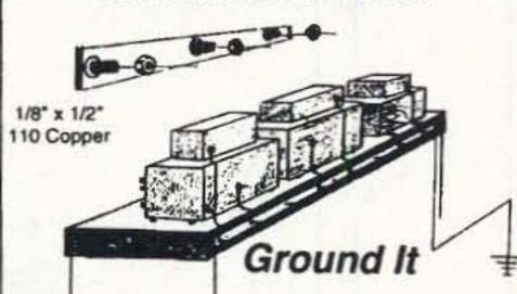
Solid Copper Buss Stainless Steel Hardware Grounding Stud Every 6 Inches Top or Back Installation
