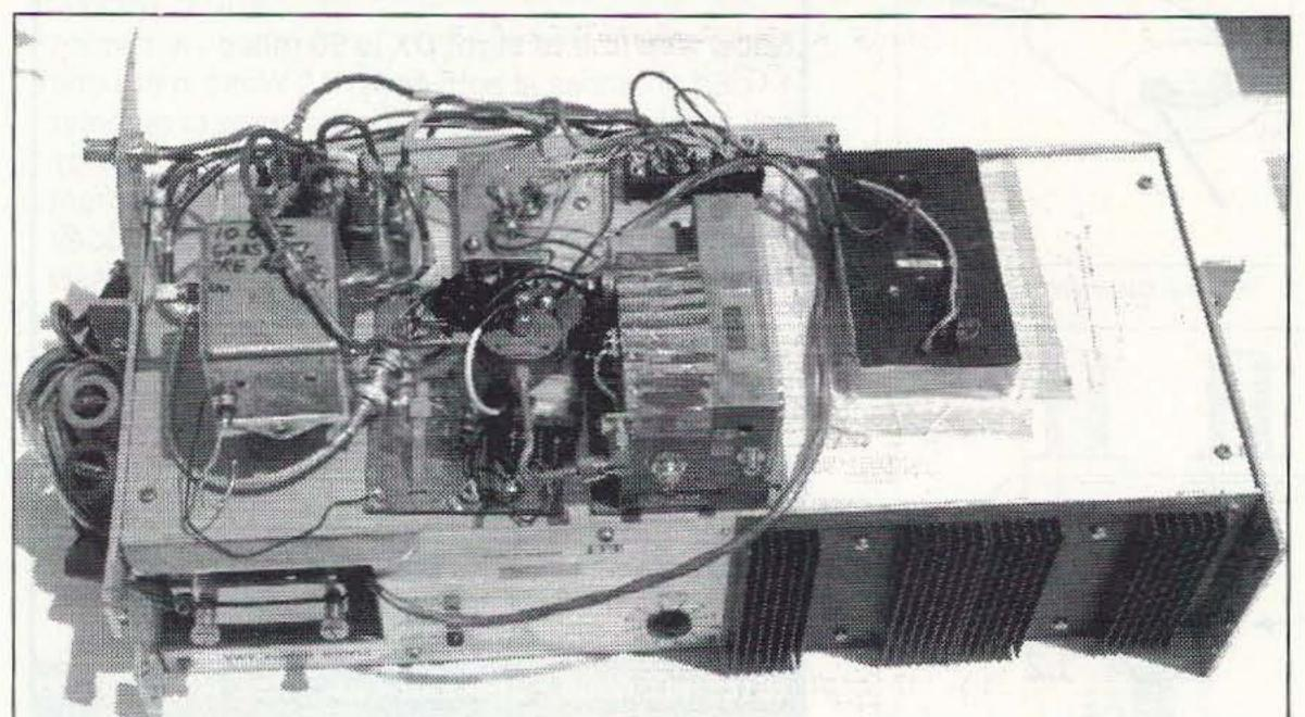
Photo A. In response to many questions asking what my 10 GHz SSB rig looks like, here it is: a 10 watt TWT. The large bottom unit is the power supply for the TWT. The top unit consists of two preamps, a brick oscillator-mixer, and four coaxial relays.
