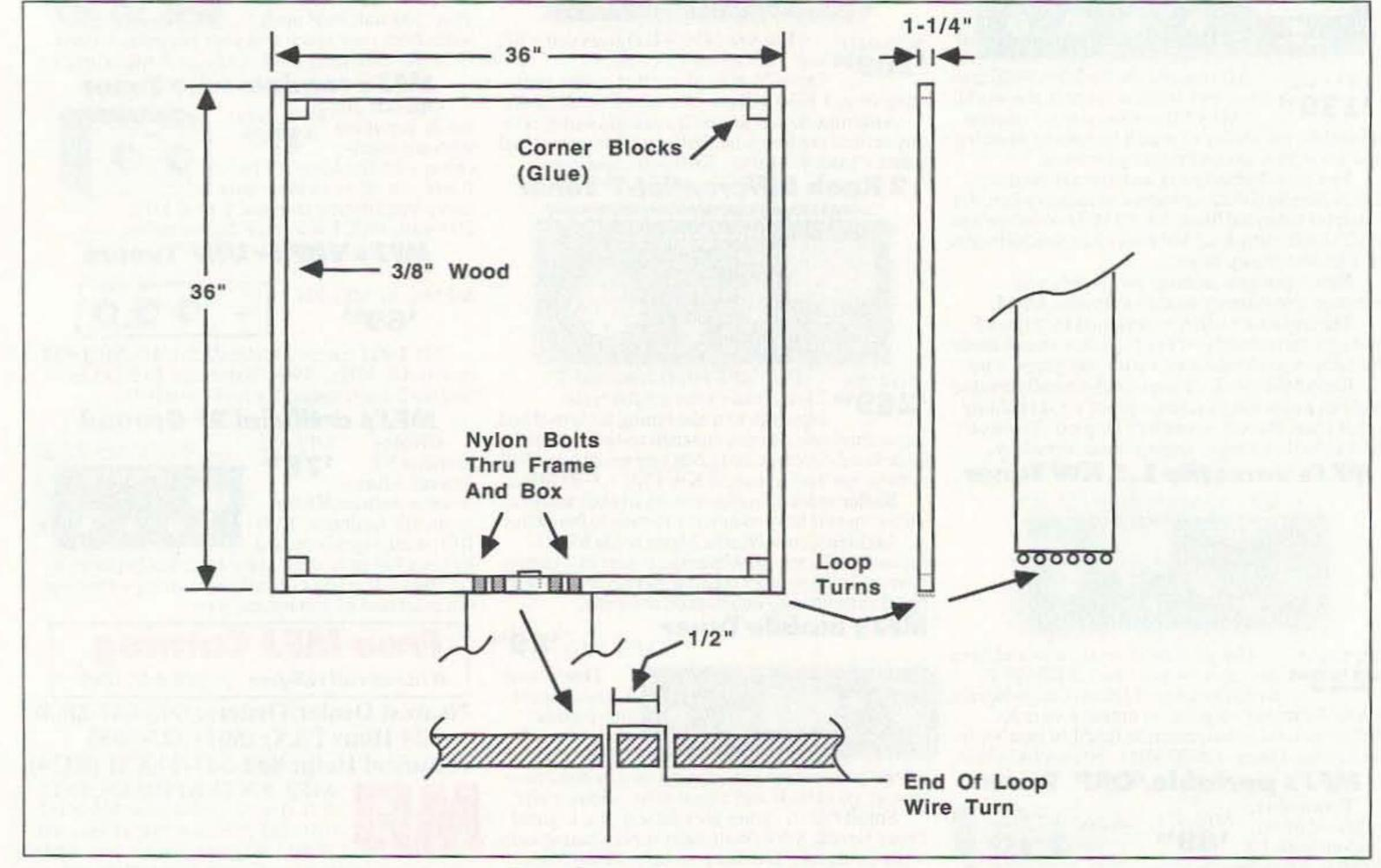
Figure 3. Main frame and loop winding.
