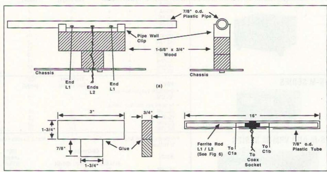
Figure 7. Ferrite rod coil and support assembly.
