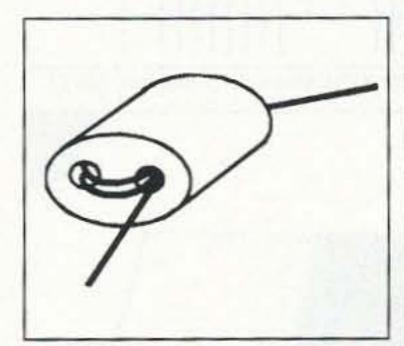
Figure 3. Balun winding details.
