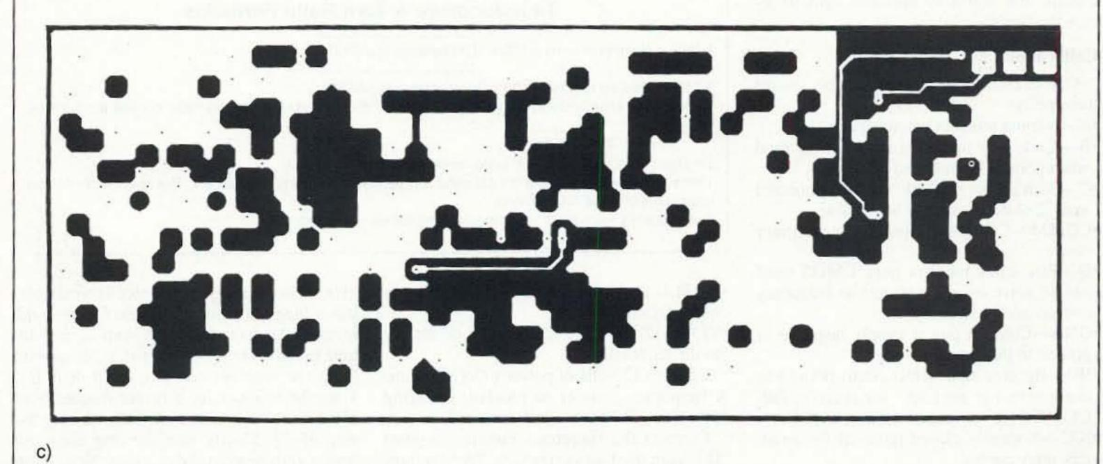
Figure 3. Double-sided PC board: (a)parts placement diagram, (b) top foil pattern, and (c) bottom foil pattern.
