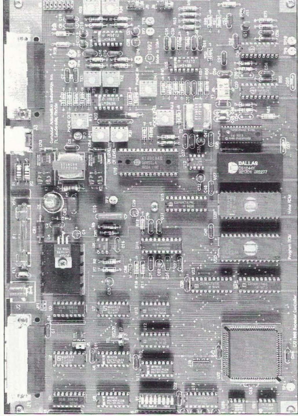
Photo A. The CAT 1000 repeater controller board.
