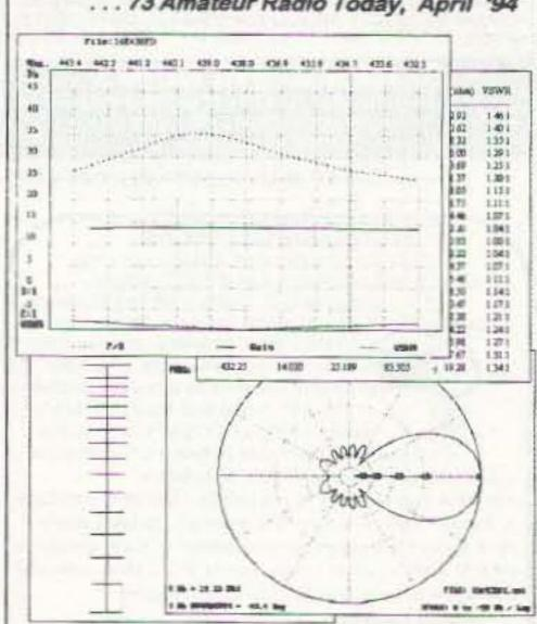
This high speed, easy-to-use yagi software features autodesign, auto-optimize and performance analysis. It will accurately calculate up to 17 elements to 1 Ghz. with boom and tapered element compensations, a folded dipole option, and prints all files, charts and graphs. Includes both co-processor & no co-processor versions.
