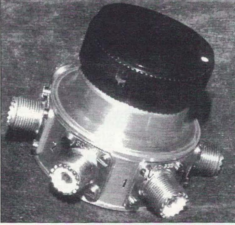
Photo A. The HOFI Model 605 antenna switch.
