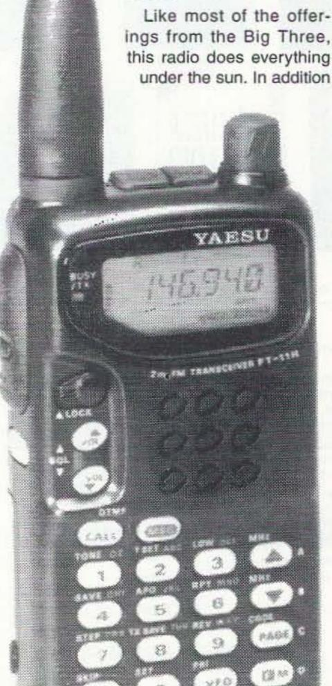
to the now-standard autodialer memories, generous memory capacity (150 of them!), CTCSS encode (decode is optional) and digital paging features, this diminutive pocketful incorporates a few new goodies: alphanumeric labels for each memory, message paging, and knobless volume and squelch adjustment.
