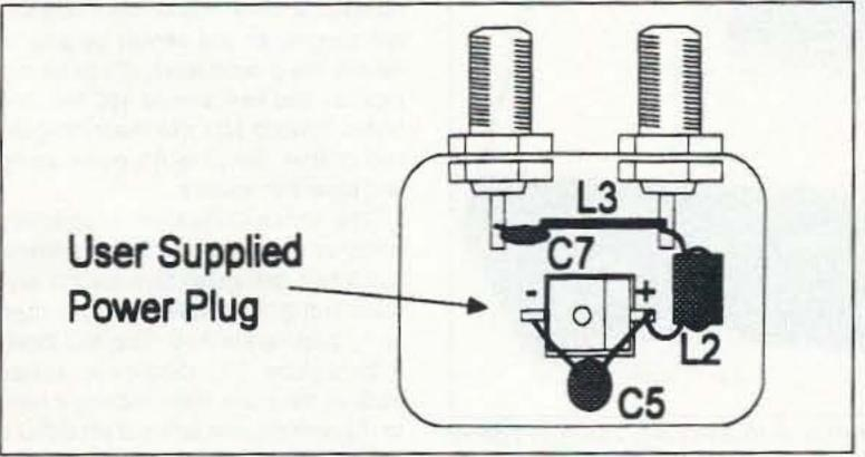
Figure 4. DC power injector final assembly.
