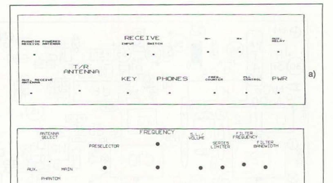
Figure 4. Face plate templates: (a) front, and (b) rear, reduced 50%.
