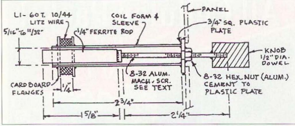
Fig. 2. Construction details.
