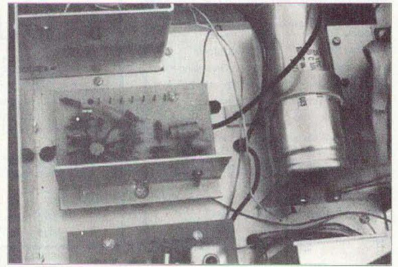
Photo B. The low level RF driver is mounted to a small heat sink. This board plugs into a chassis-mounted socket.
