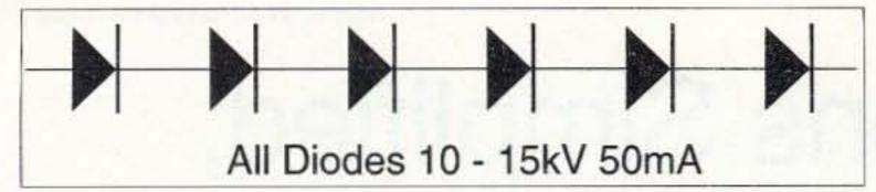
Fig. 2. Series diode rectifier before addition of voltage multiplication circuitry.
