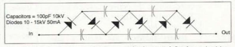
Fig. 3. Complete circuit of voltage multiplier used for laser ignition. Voltage required: approximately 10 kV.
