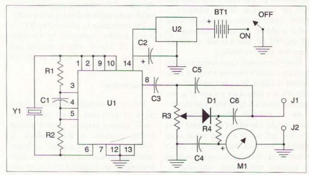
Fig. 1. Schematic diagram for the simple capacity meter.
