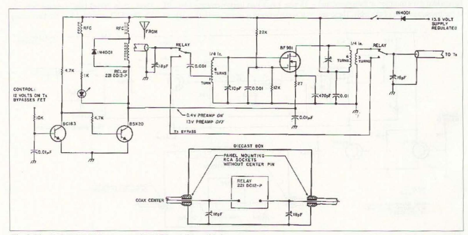
Fig. 2. The AMSAT-UK FET preamp with RX-TX switching added.
