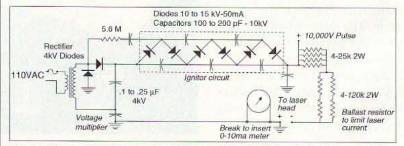
Fig. 1. Basic laser power supply showing rectifier, voltage multiplier, ignitor and ballast resistor circuit.
