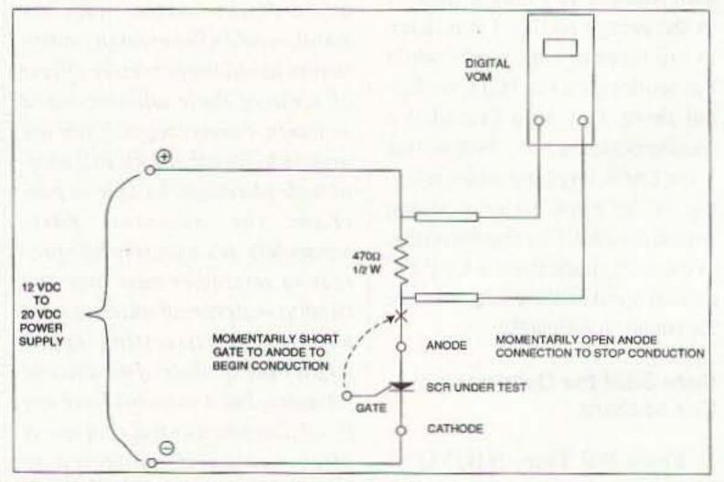
Fig. 1. AD4UA's simple SCR test circuit.
