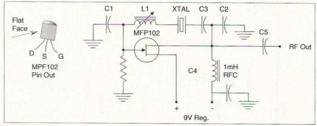
Fig. 1. Oscillator circuit.
