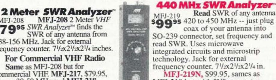
read SWR. Uses microwave integrated circuits and microstrip technology. Jack for external frequency counter. 71/2x21/2x21/4 in.
