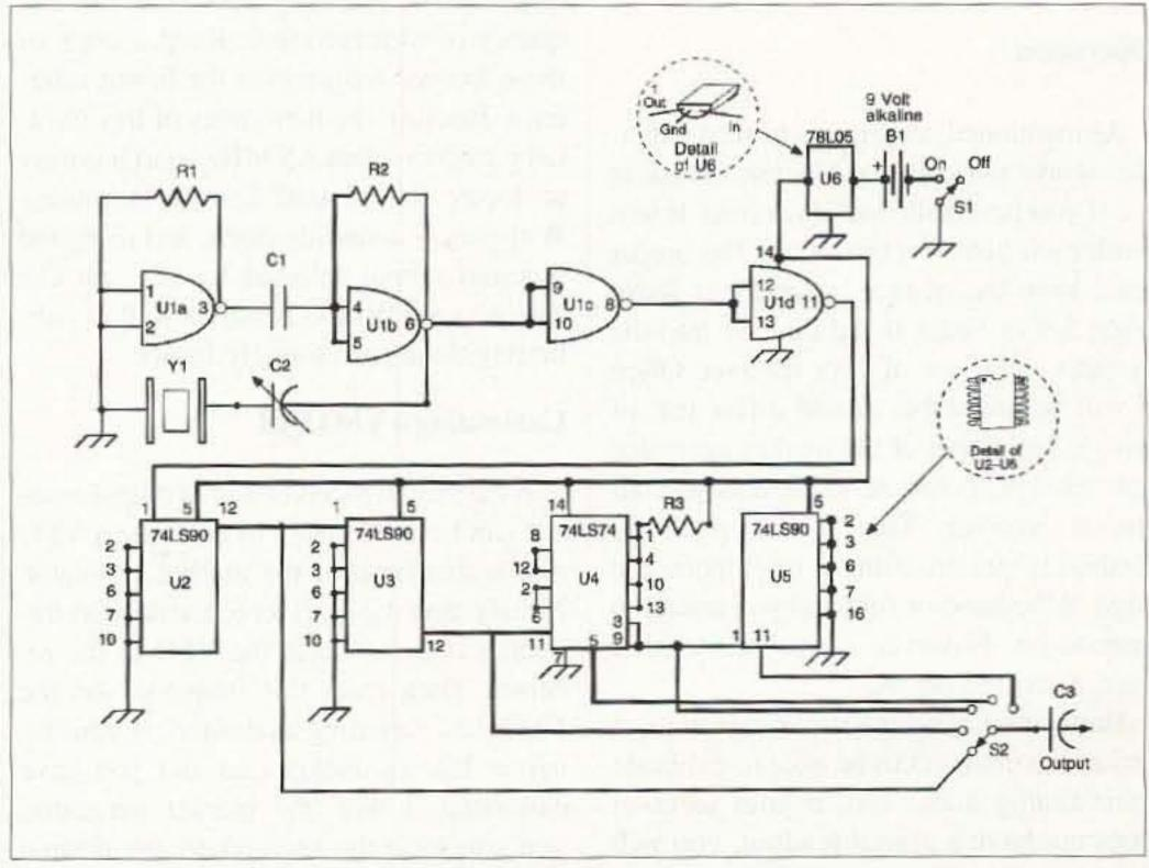
Fig. 1. Schematic for the simple secondary frequency standard.
