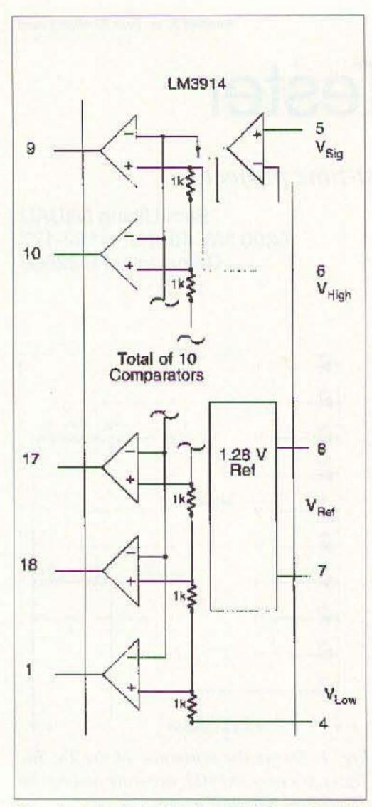
Fig. 2. A look inside the LM3914, the chip has a total of 10 comparators.
