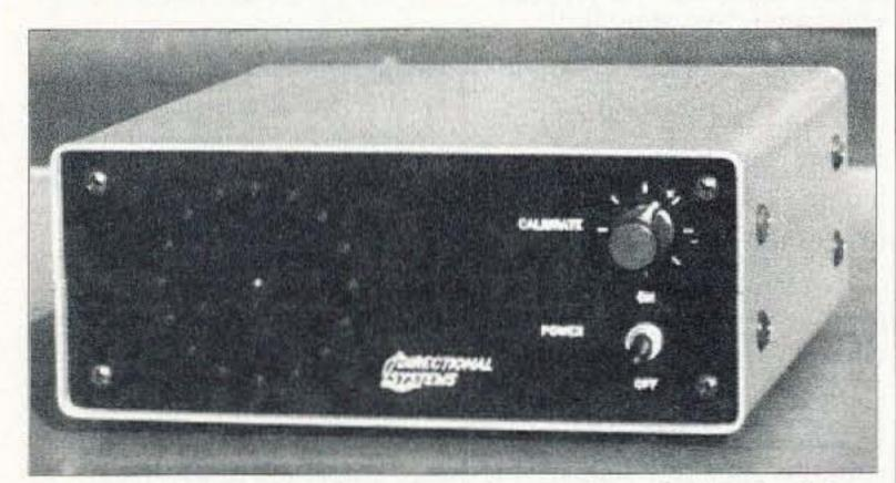
Photo D. The complete Directional Systems Doppler display is in a 7-1/2 x 6-1/2 x 2-1/2 inch enclosure.
