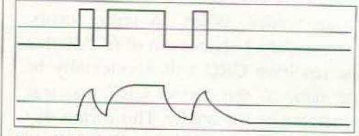
Fig. 3-2. A digital signal, before and after distortion
