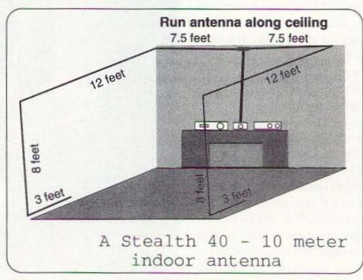
Fig. 1. Antenna installation diagram.
