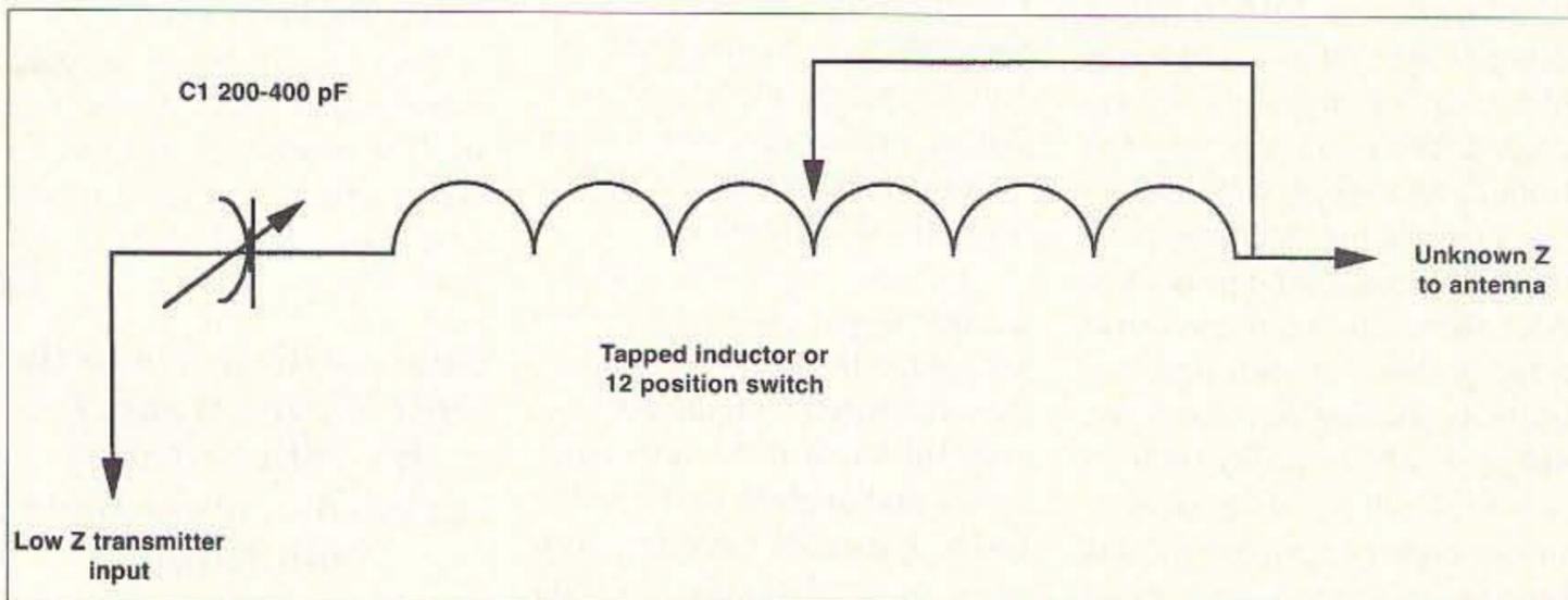
Fig. 1. Schematic for the tuner.
