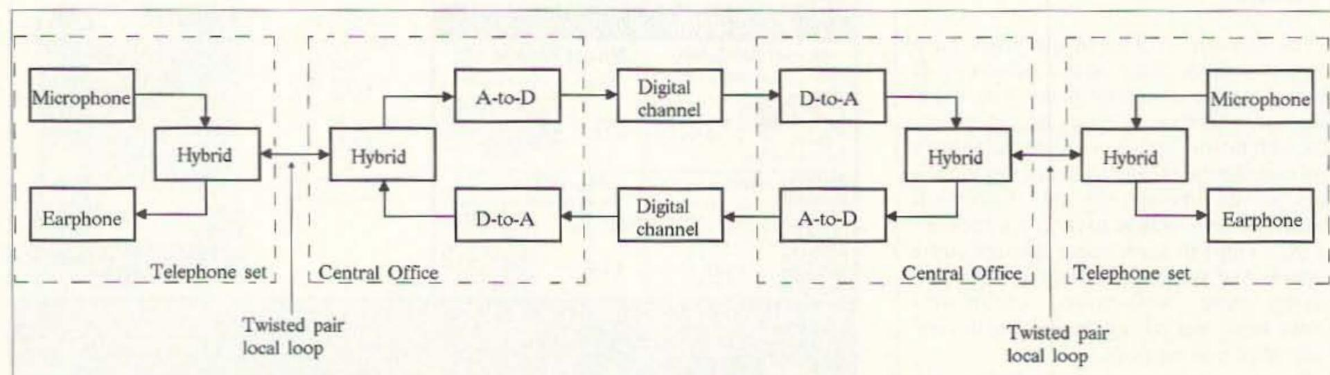
Fig. 1. Signal path through the POTS network.
