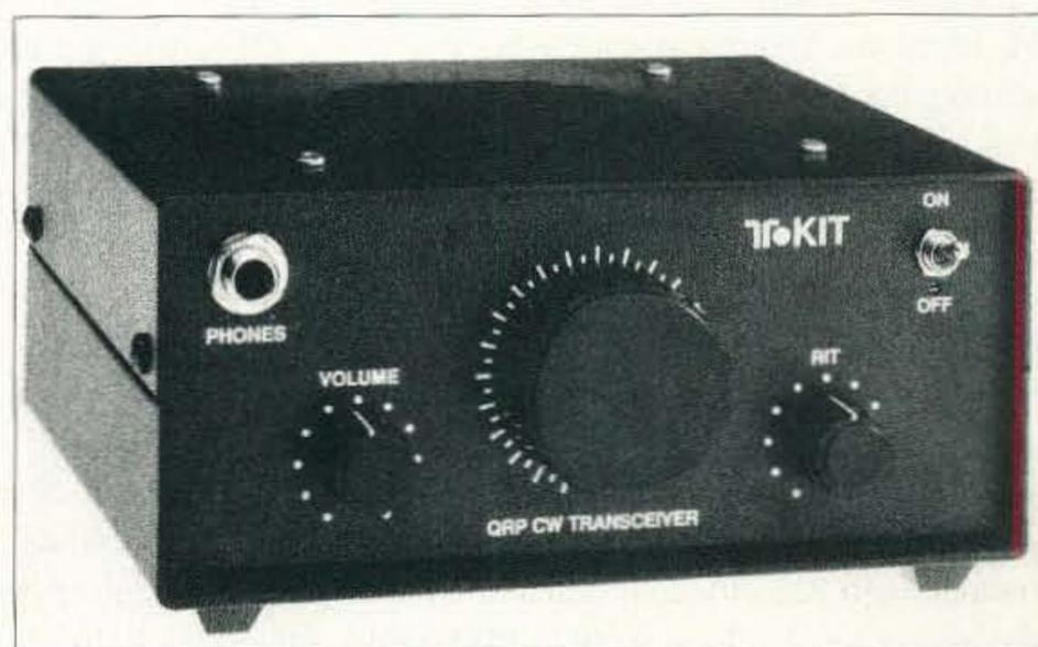
Photo A. The Ten-Tec 1340 QRP transceiver.
