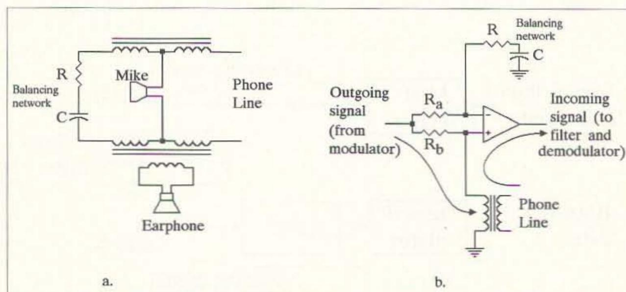
**Fig. 4.** The hybrid/duplexer circuit.
