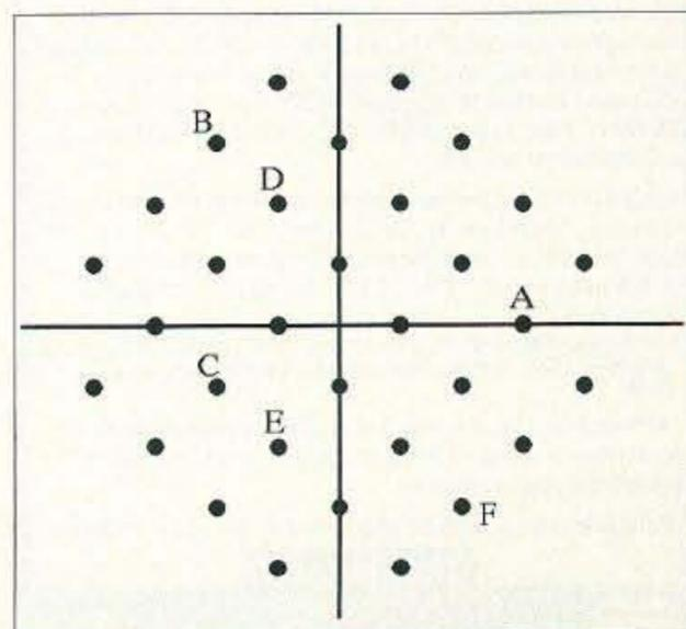
Fig. 9. Trellis constellation for a 9600-bps modem.
