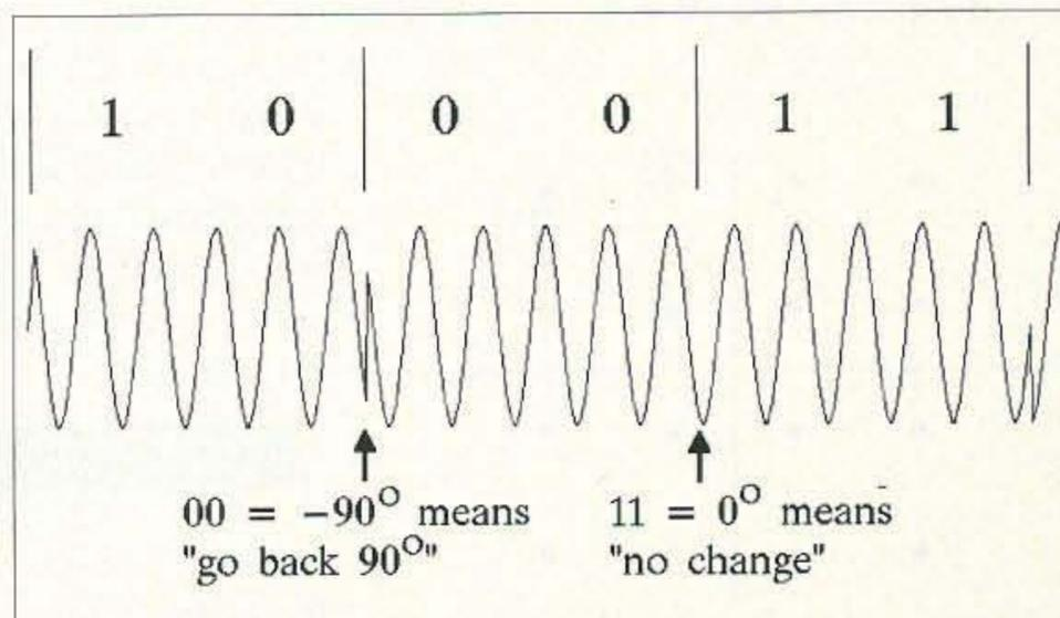
**Fig. 6.** DPSK-4 with four phase angles.
