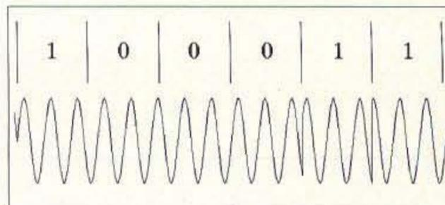
**Fig. 5.** DPSK-2 with two phase angles.
