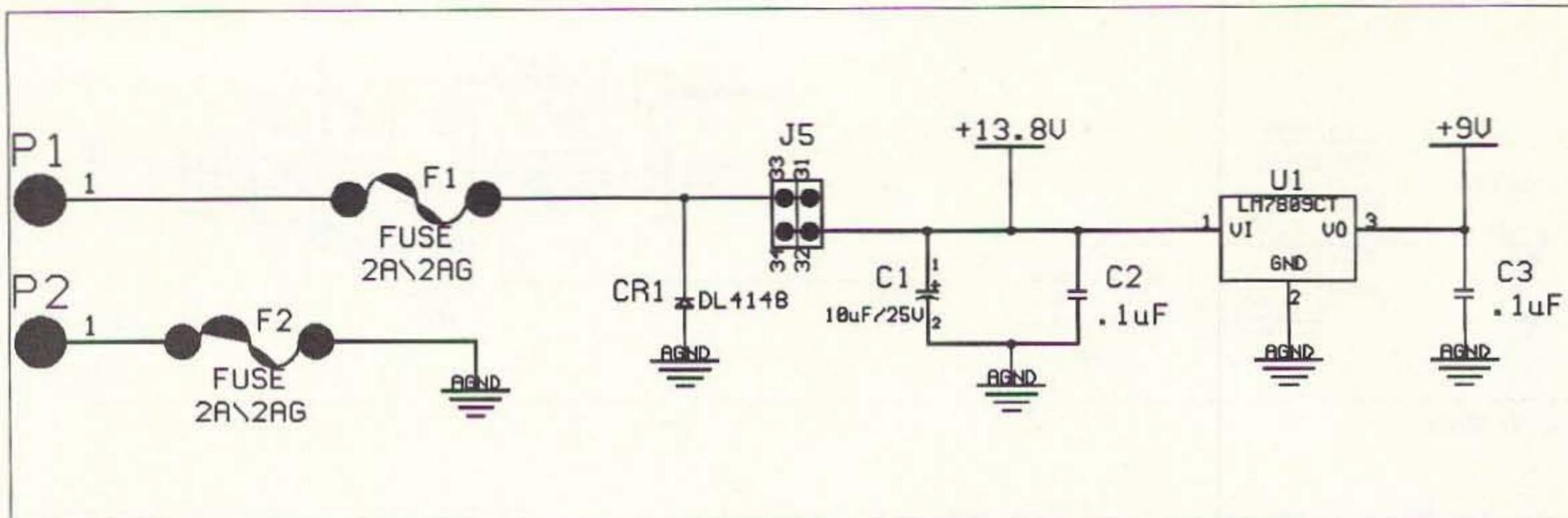
Fig. 5. Power input section.
