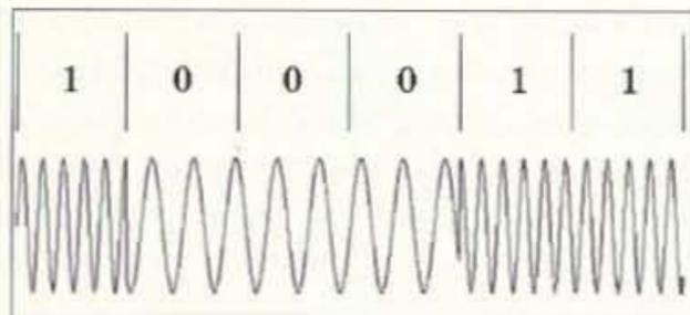
Fig. 2. Frequency-shift keying (FSK).
