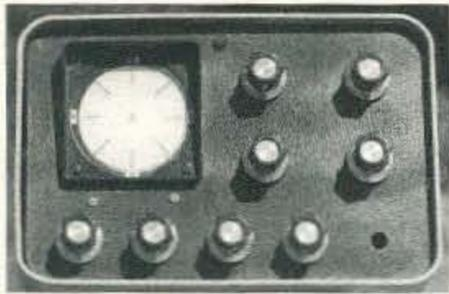
**Photo A.** The Heathkit Scanalyzer after repainting the front panel and replacing the grid screen under the CRT bezel with a transparent compass overlay. Next comes labeling. The hole at lower right will be filled by a future control.
