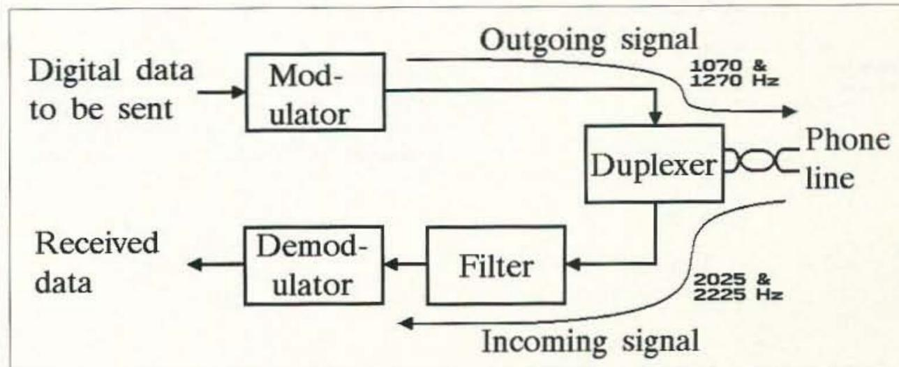
Fig. 3. Bell 103 modem block diagram.
