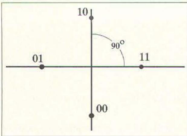
Fig. 7. A DPSK-4 constellation diagram.
