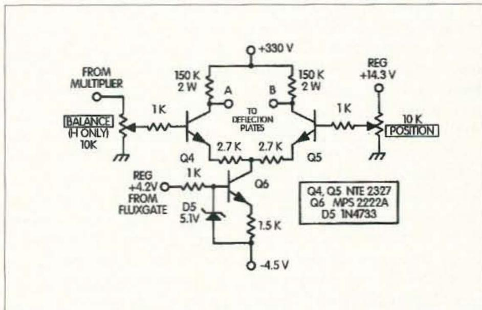
**Fig. 1.** Schematic of the new deflection circuits. Two are required, each with a spot positioning potentiometer on the front panel. A and B outputs of the horizontal (X) circuit go to the orange and yellow CRT socket wires, respectively. A and B outputs of the vertical (Y) circuit go to white and violet socket wires.
