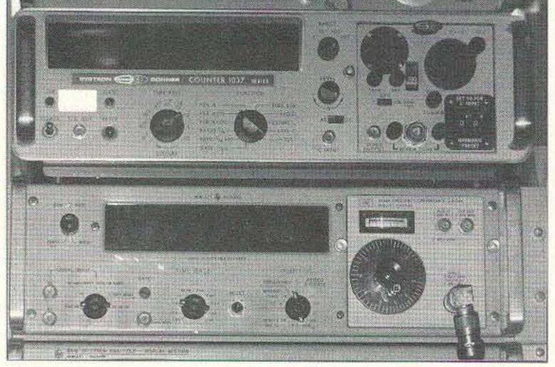
Photo A. The old reliable HP-5245 base counter on bottom, shown with the Systron Downer 1037 on top. Not a match but quite similar in operation for main units and plug-in units. (Note: Plug-ins not interchangeable between units.)
