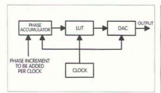
Fig. 2. Block diagram of a basic DDS with the major functions shown.
