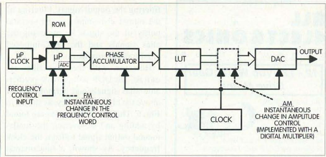
Fig. 4. Microprocessor-enhanced DDS with control points shown for creating AM and FM modulation modes.
