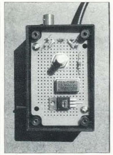
**Photo C.** The circuit board is installed and the input wires are attached to terminal pins.
