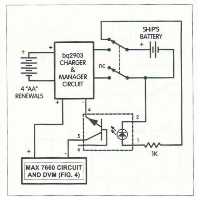
Fig. 7. Using an optoisolator and DPDT switch.
