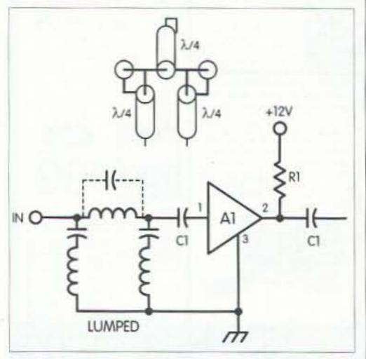
Fig. 5. A notch filter can reduce interfering signals.
