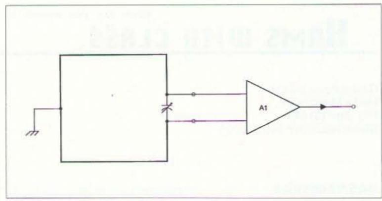
Fig. 1. Basic single-ended loop amplifier.
