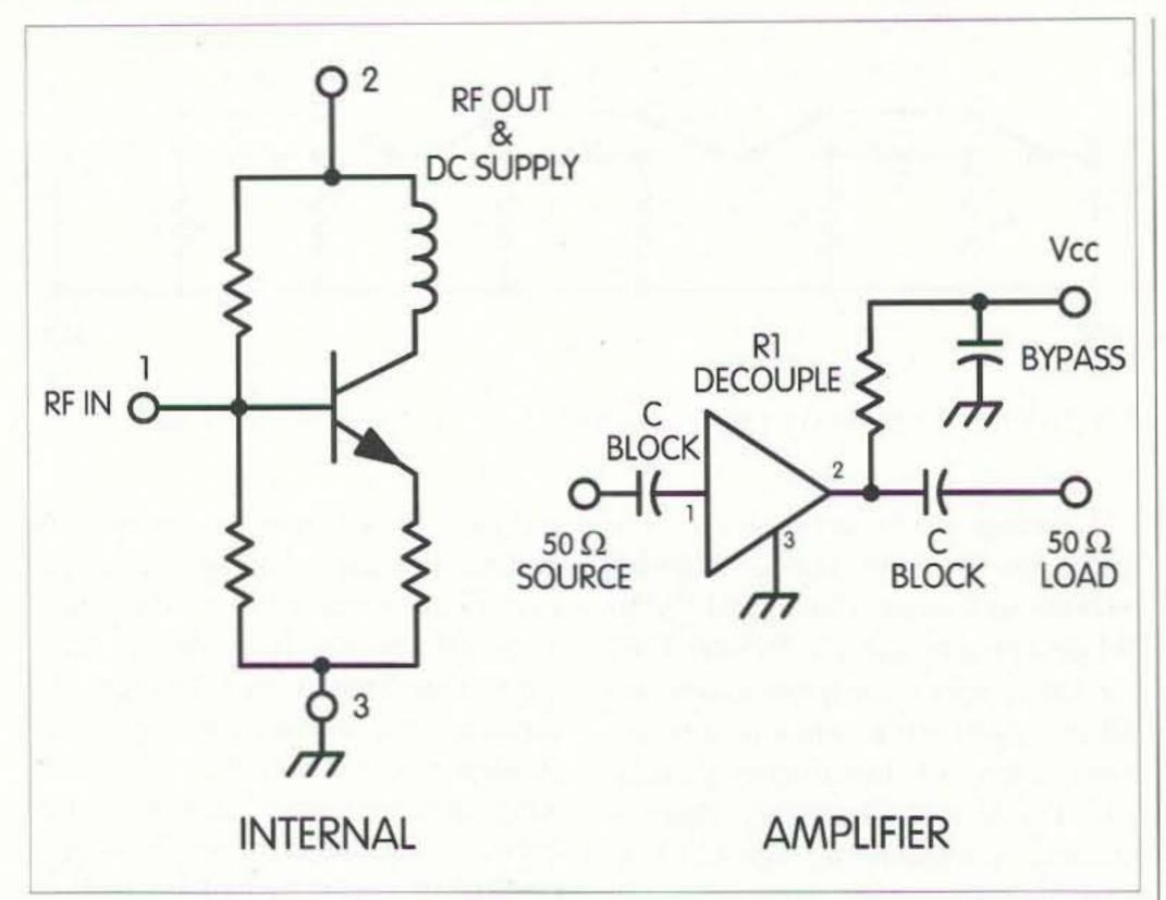
Fig. 2. The internal circuit of the MWA110 and its application as an amplifier.
