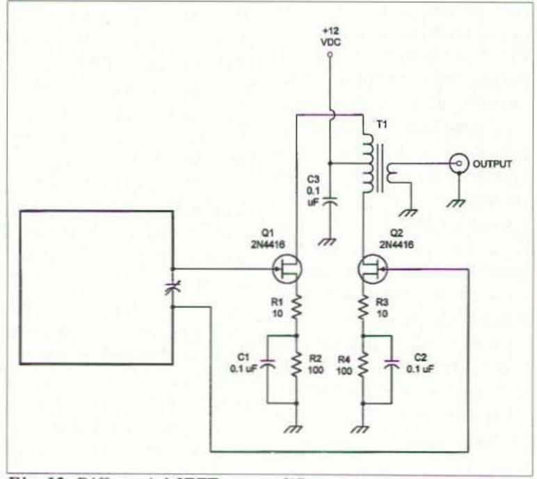
Fig. 12. Differential JFET preamplifier.
