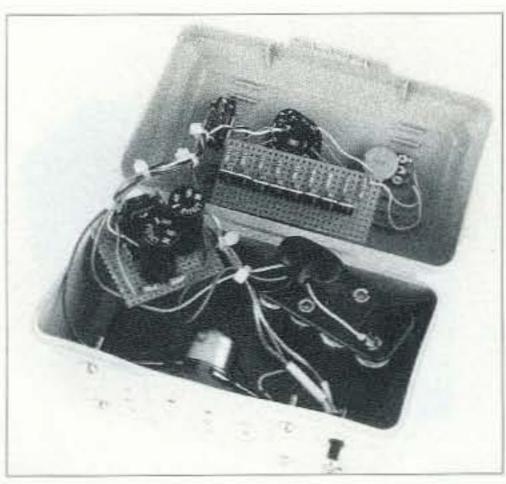
Photo B. Inside a basic, bare-bones, bluebox metronome with perfboard construction and eight preset tempos. A close look at the battery pack will show a tap, one way to get the correct voltage to Q1 and Q2 before trying the regulators. This does work while the batteries are fairly fresh. However, it does not give the best repeatability—sometimes that is a consideration.
