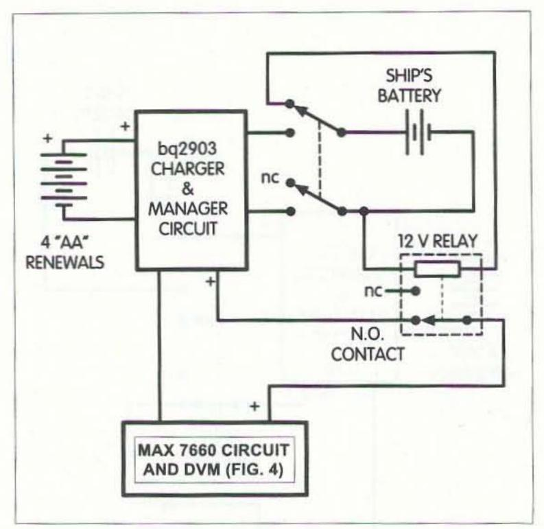
Fig. 6. Using a relay and DPDT switch.
