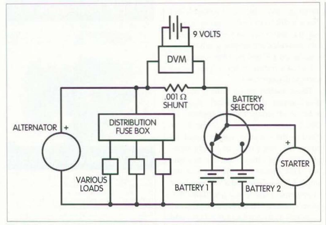
Fig. 3. Connecting the ammeter to a "real-world" circuit.
