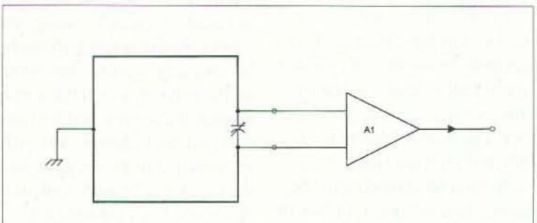
Fig. 3. Balanced loop.
