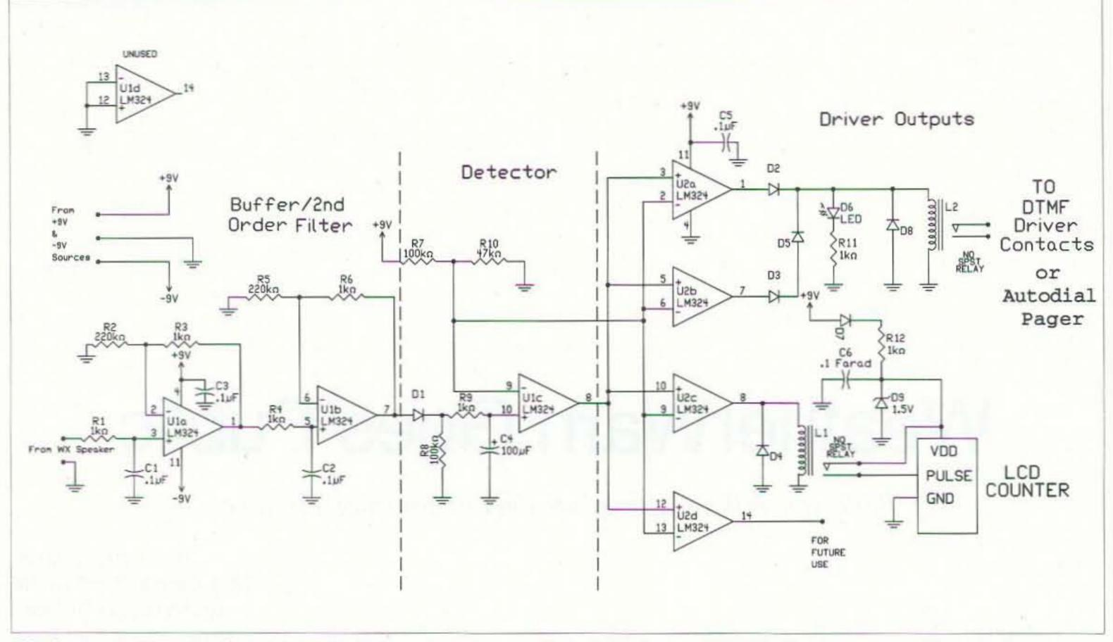
Fig. 1. WeatherWarn interface schematic. Unless otherwise specified, all diodes are 1N4007, all resistors are ±5%, and all capacitors are +16 V.
