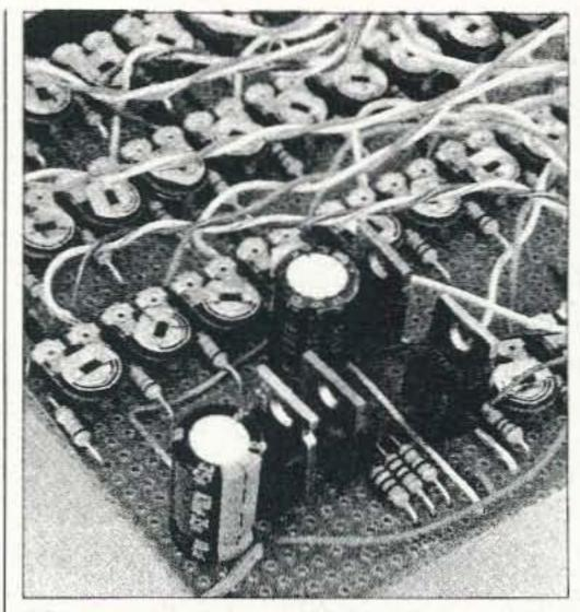
Photo F. Close-up of board in deluxe model. Large caps are C3 and C4. Transistors Q1-Q3 are seen left to right in a row, with the 7805 regulator above Q3.
