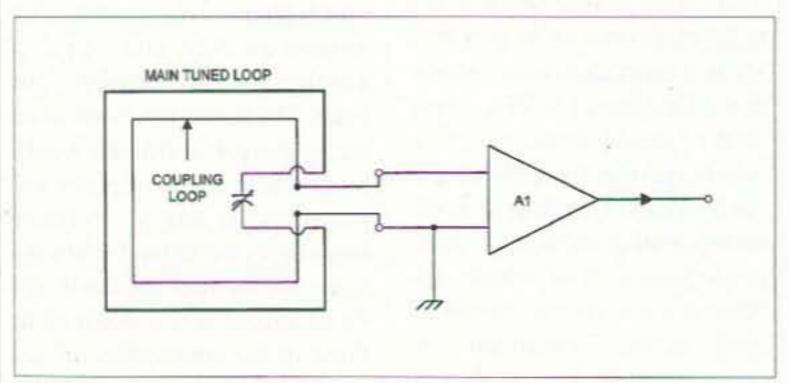
Fig. 2. Single-ended with coupling loop.
