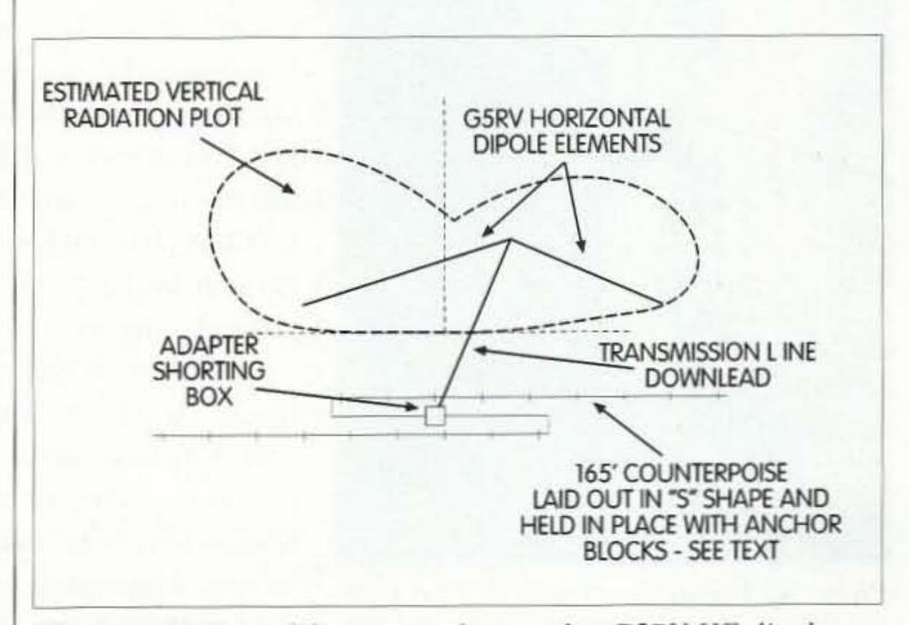
Fig. 2. AD1B's modification to the popular G5RV HF dipole antenna to permit contest weekend operation on 160 meters.
