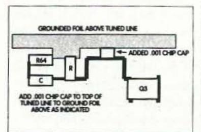
Fig. 3. Modification to VCO circuit on synthesizer board to convert original VCO frequency from 800 MHz range to 1152 MHz. Add .001 µF chip capacitor from top of printed inductor to ground. This bypass capacitor increases VCO frequency from 700 MHz to 1200 MHz.
