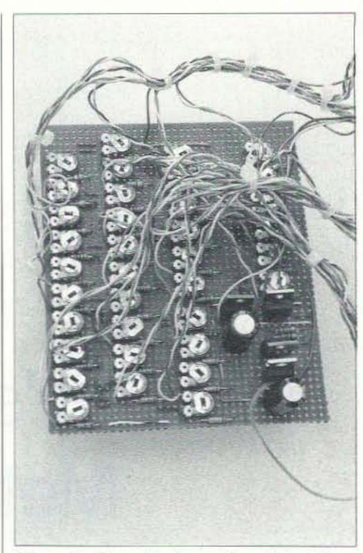
Photo E. Overall view of board in deluxe model. The regulator and pulse generator are on the lower right side of the board, while the fixed resistors and their trimmers take up the rest of the space.
