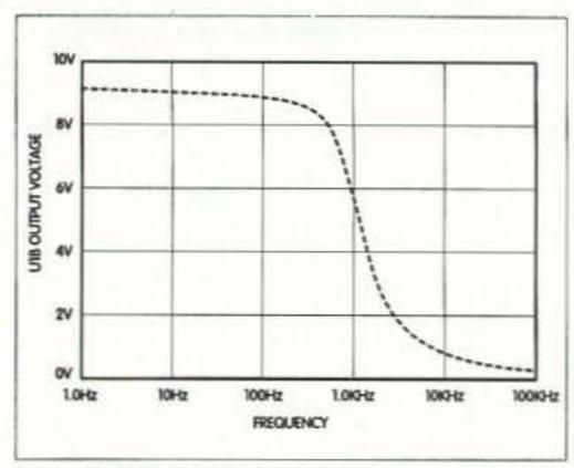
Fig. 2. WeatherWarn frequency response curve.
