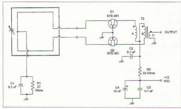
Fig. 11. Loop integrated push-pull preamplifier.
