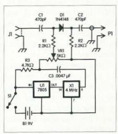
Fig. 1. Schematic diagram of the offset attenuator.
