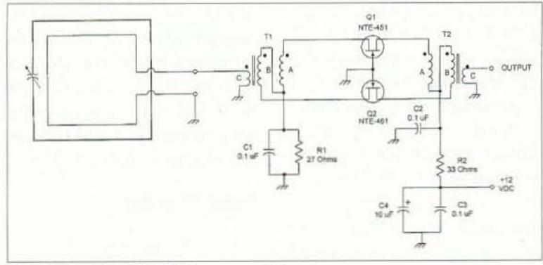
Fig. 8. Push-pull JFET preamplifier.
