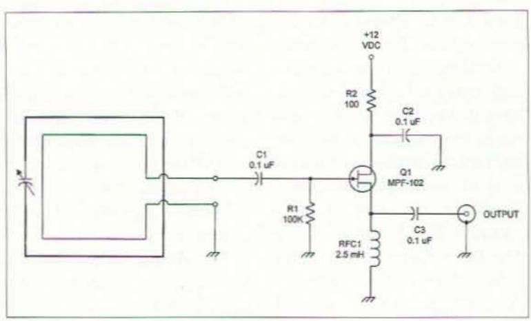
Fig. 10. Common source JFET preamplifier.
