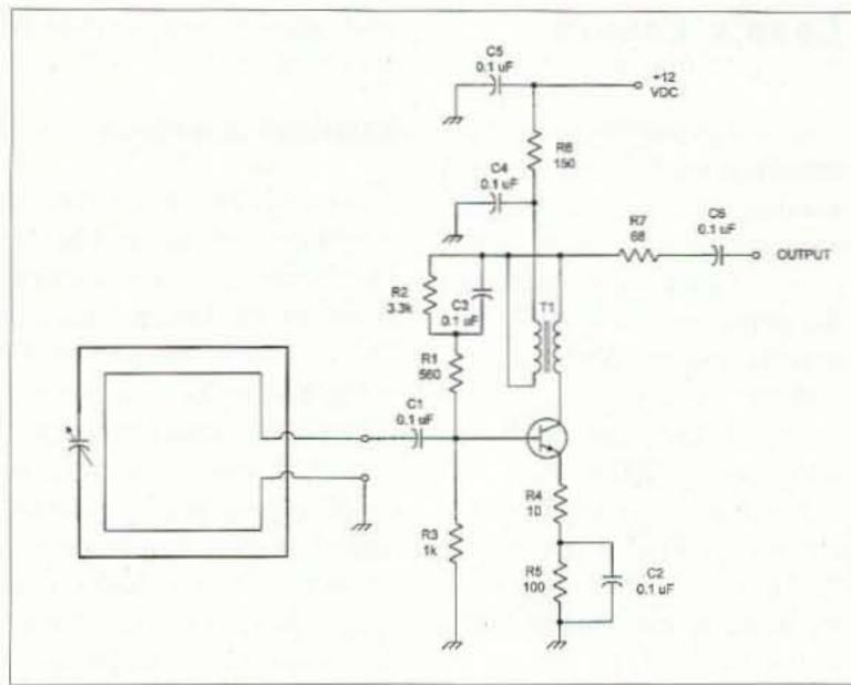
Fig. 6. Bipolar NPN transistor preamplifier.
