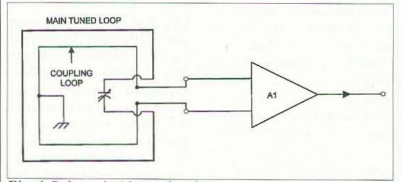
Fig. 4. Balanced with coupling loop.
