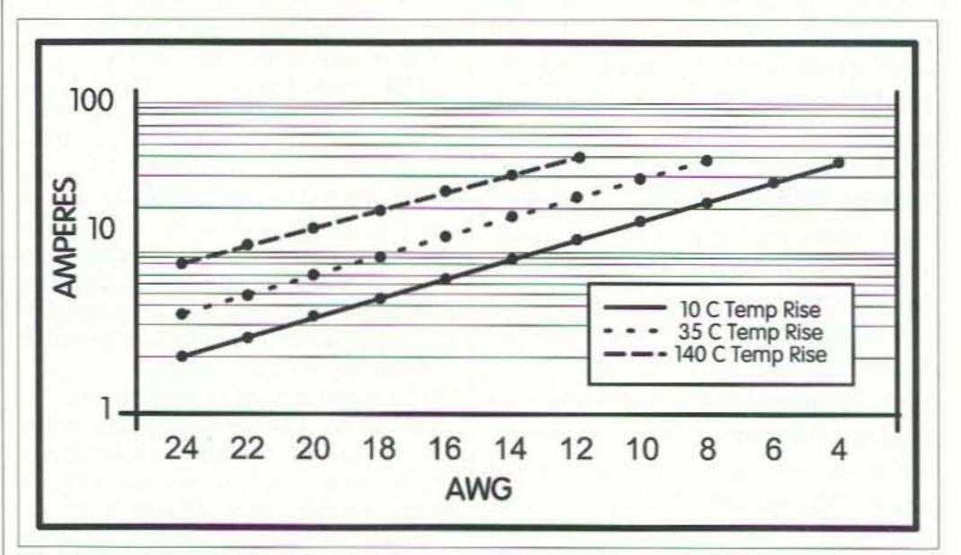
Fig. 2. Current-carrying capacity of wire.
