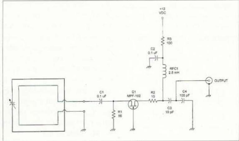
Fig. 9. Common gate JFET preamplifier.
