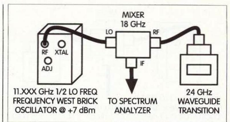
Fig. 1. Block diagram of frequency extension equipment for using low frequency spectrum analyzers to display accurately 24 GHz frequency information using low order harmonic. System uses 1/2 frequency local oscillator and mixer originally made for 18 GHz operation. 24 GHz filtering done by 24 GHz antenna transition using waveguide cutoff for broad filtering.
