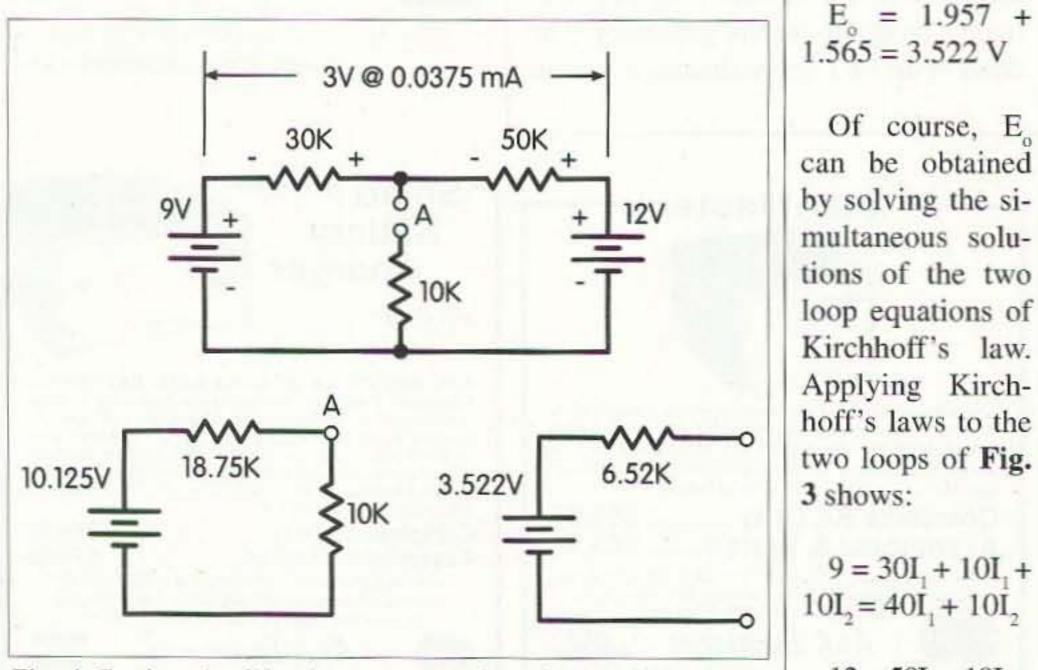
Fig. 4. Further simplifications can ease the solution of two-source networks.
