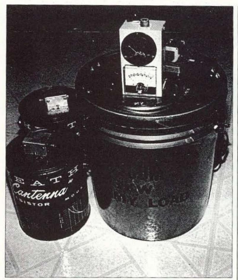
**Photo A.** The 3 kW dummy load all dressed up and ready to go. The optional circuit with the RF (top) and the relative output meters have replaced the Heath minibox on the lid of the gallon container. The meter chassis was mounted vertically so that the rear panel could be removed for convenient access to the circuitry. The sensitivity control
