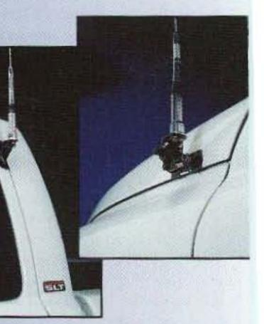
Got a new truck? No problem! The hood or rear doors are perfect for mounting an antenna. Slide the mount over the lip. tighten the set screws, and adjust it to vertical. No holes to drill, the mount is grounded and installation takes only a few minute Choose the deluxe or standard cable assembly in the length required.
