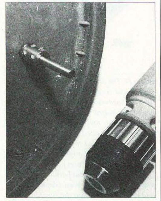
**Photo F.** If you prefer not to install the gearhead motor, pass the stirrer through the bushing from the inside and secure the coupling to the shaft as a stop. Use your hand-held drill to circulate the oil.
