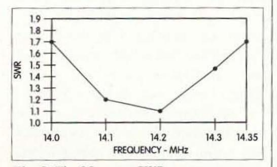
Fig. 3. The 20-meter SWR curve.
