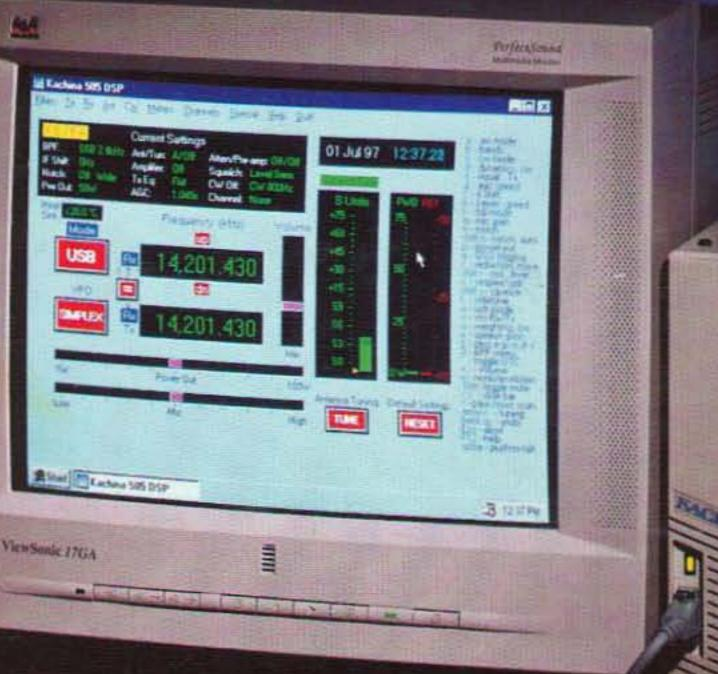
The Kachina **505DSP Computer** Controlled Transceiver
