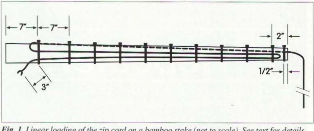
Fig. 1. Linear loading of the zip cord on a bamboo stake (not to scale). See text for details. 16 73 Amateur Radio Today • May 1999
