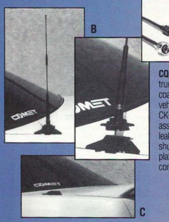
CQ-5M "Quick-disconnect" trunk lip mount. Rubber coasted-base protects the vehicles paint. Includes the CK-3M5 deluxe cable assembly avoiding water leaks or cable damage when shutting the trunk. Goldplated SO-239/PL-259 connectors.
