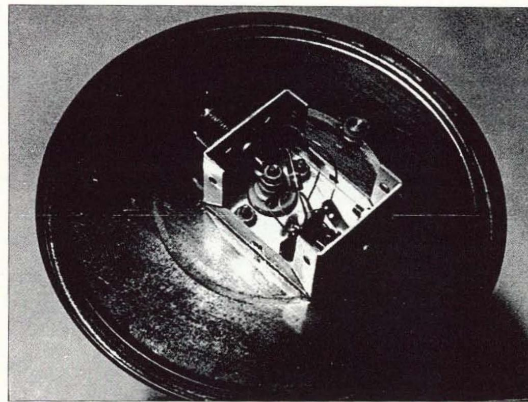
**Photo G.** A view of the stock Heath Cantenna input circuit. Leave this system intact if you prefer not to install a monitoring circuit. The small disk to the upper right of the minibox is the spring-loaded safety valve. The electronic components in the original Heath design accommodated a relative output meter through the RCA phono plug mounted opposite the SO-239.
