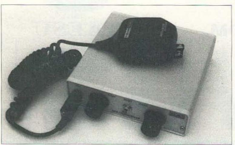
Photo B. The finished WM-20 SSB transceiver.
