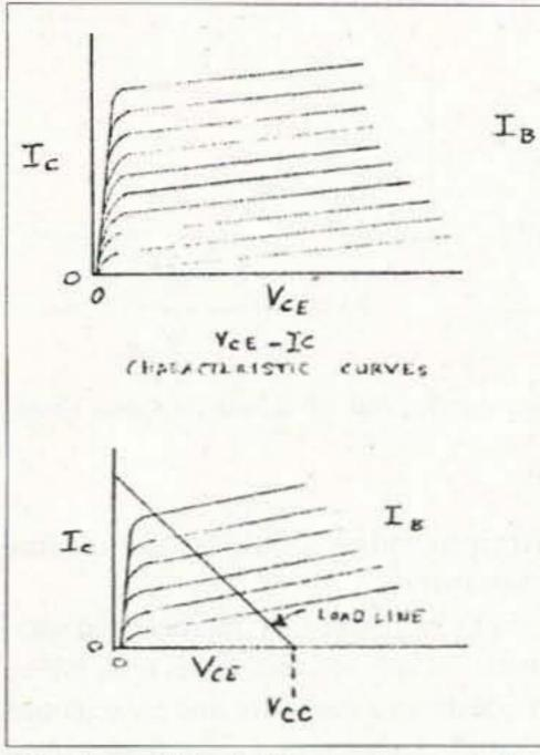
Fig. 2. Load line laid out on a set of characteristic curves. Coordinates for the load line are at the maximum Ic value and the applied Vcc voltage value.
