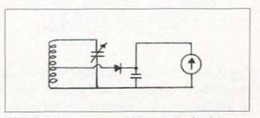
Fig. 2. Wavemeter utilizing a diode detector and a meter to indicate circuit resonance. 73 Amateur Radio Today • August 2001 19
