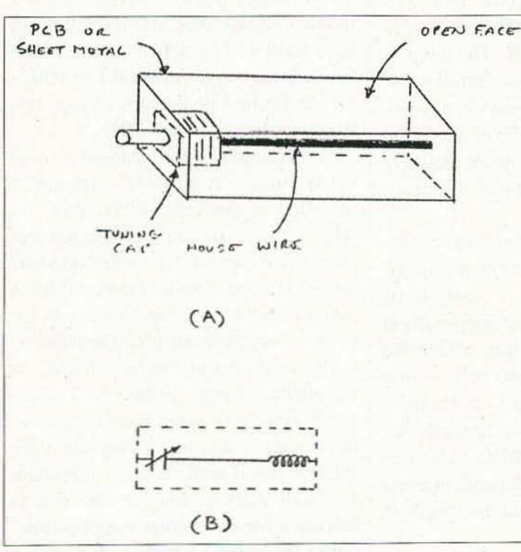
Fig. 7. Pictorial view of a channel resonator used as a wavemeter. (a) A straight wire resonator allowing the circuit to resonate at the highest frequency. (b) A coil may be added to the cold end of the resonator to lower the frequency of a given channel. Notes: Box length contributes to operational frequency. Line length and cap value determine frequency.
