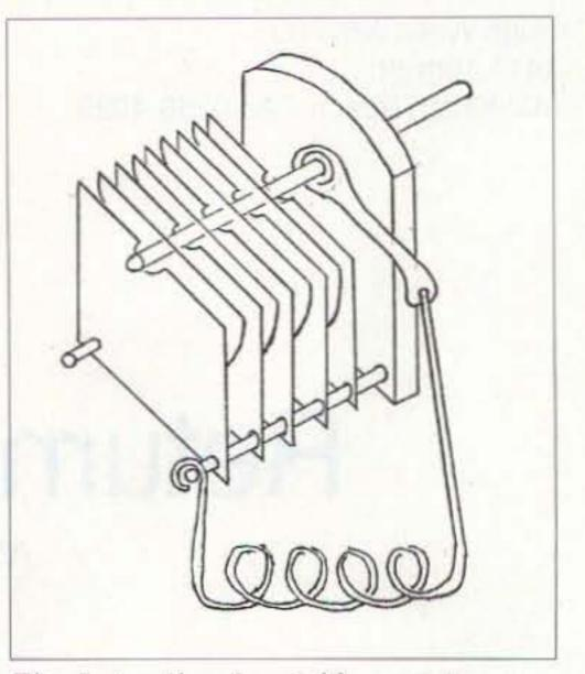
Fig. 5. A coil and variable capacitor connected to form a resonant circuit to be used as a wavemeter. A pointer knob may be mounted on the capacitor's shaft. A calibrated frequency scale may be mounted on the capacitor's mounting plate.
