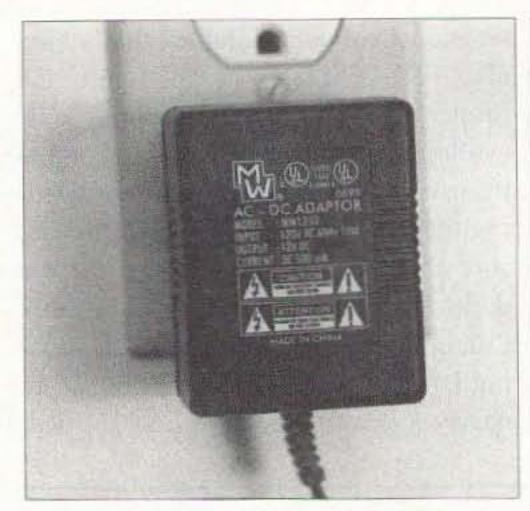
Photo A. A typical "wall-wart" power supply.
