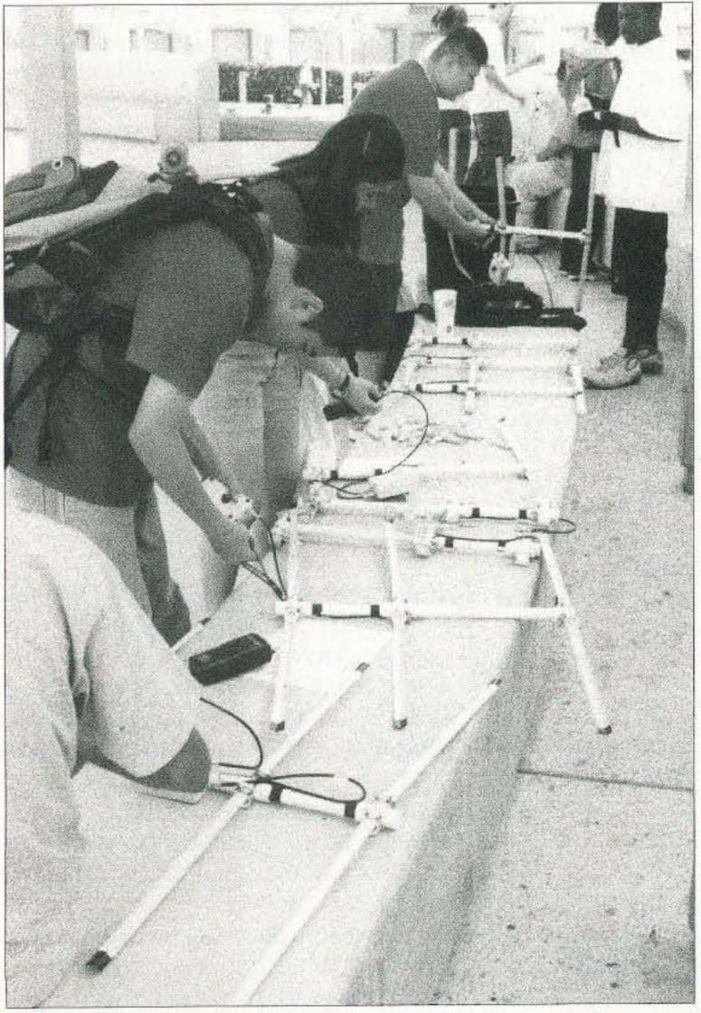
Photo C. At the equipment testing session, students discovered that it's hard to take bearings while carrying a yagi, attenuator and receiver separately. After that, we decided to put handles on the yagis and mount the attenuators to them.
