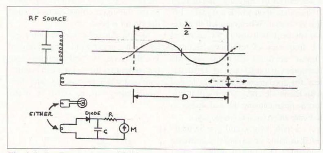
Fig. 4. Lecher Wire system used for determining the relative frequency of a signal source. Detection of the signal null may be done using either a light bulb or a field strength meter. The detector circuit is located on the opposite side of the Lecher Wire pickup loop in order to create the greatest amount of field amplitude change. D in meters: F(MHz) = 150/D. D in inches: F(MHz) = 5905/D.
