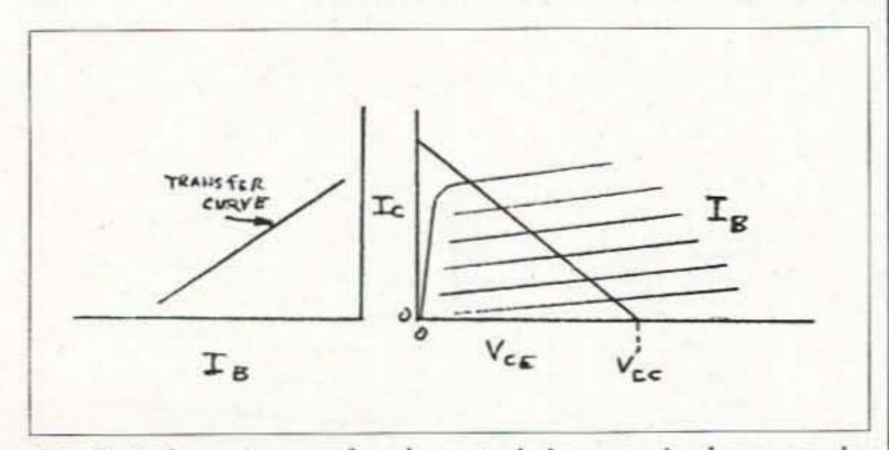
Fig. 3. A dynamic transfer characteristic curve is shown on the left. The transfer curve shows the linearity of the amplifier's response to an input signal where a straight line is preferred. Any curvature in the transfer curve indicates amplitude distortion.
