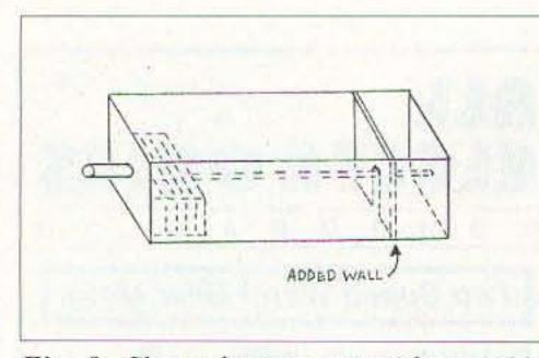
Fig. 8. Channel resonator with an added wall used to shorten up the channel length with the intention of raising the frequency of resonance. The wall must be soldered to the wall and resonator wire to maintain stability.
