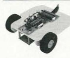
This advanced kit is an 8 x 8" differentially steered base that is excellent for carpet or tiled floor experimentation. It uses the Next Step microcontroller, a BASIC Stamp 2 controller that can use the BS2 or BS2-E (sold separately). A host PC is required to download programs to the robot. This complete kit includes the Rover, programming cable, IR proximity detector, bumper switch kit, and line follower kit. Carpet Rover II Complete Kit \$185.00
