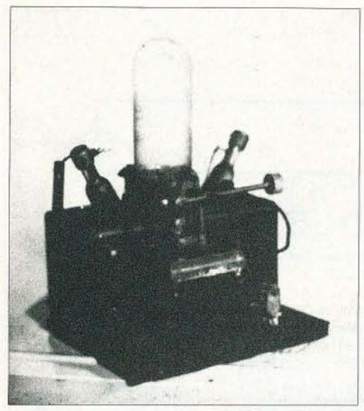
Photo H. A one-kilowatt transmitter.
