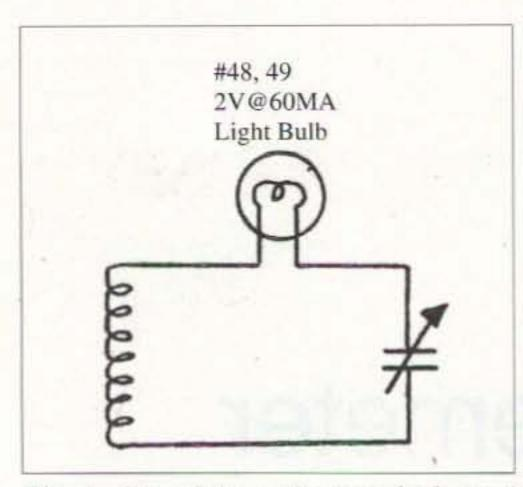
Fig. 3. One of the earliest methods used for indicating resonance of a wavemeter was to employ a light bulb. The bulb's glow was dependent upon the circulating current flow.
