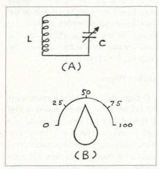
Fig. 1. (a) Basic circuit of a wavemeter. Values for L and C are selected for resonance at the desired band of frequencies. (b) Typical knob and dial used with a wavemeter. Dial is normally calibrated in increments of frequency.
