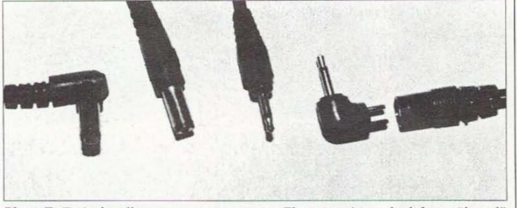
**Photo E.** Typical wall-wart output connectors. The two units to the left are "barrel" types. The next style is a 2.5mm subminiature phone plug. The unit shown on the right is a 2.5mm plug provided on a reversible-polarity adapter to the wall-wart.
