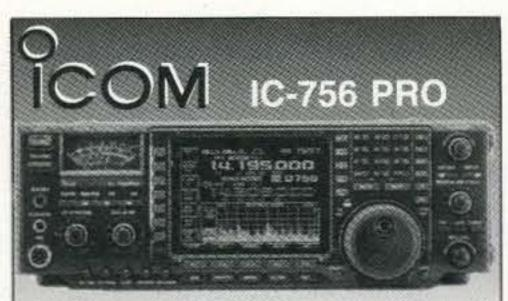
The impressive IC-756 Pro covers HF plus 6 meters. The high resolution 5 inch TFT color display provides more operating information than ever, including a spectrum scope. The 32 bit floating point DSP provides crisp, clear reception with 41 built-in filters. The "Pro" is the choice for serious DXers and contesters.
