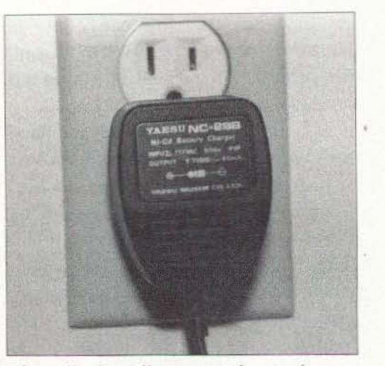
**Photo B.** A wall-wart used as a battery charger for a Yaesu handheld radio.
