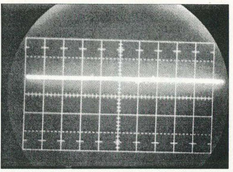
Photo D. The output waveform of a filtered power supply shows 19.5 V of essentially pure DC, with no ripple. The oscilloscope settings are the same as for Photo C.
