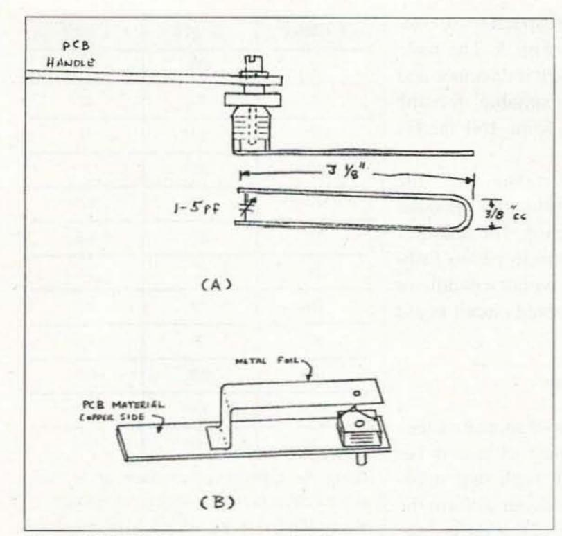
Fig. 6. VHF/UHF wavemeters: (a) Horseshoe resonators made from heavy copper wire (#10-#14) with dimensions shown for the 450 MHz band. (b) Horseshoe resonator made with metal foil mounted on a piece of printed circuit board material.
