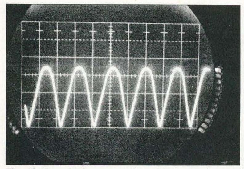
Photo C. The no-load output waveform of the battery charger of Photo B. Vertical scale is 5 V/div, indicating about 17 Vpk; the effective DC voltage as read by the DMM was 11.6 V. Unfiltered 120 Hz ripple is evident.
