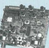
A very sensitive wideband fm receiver optimized for NOAA APT & Russian Meteor weather fax on the 137MHz band.
