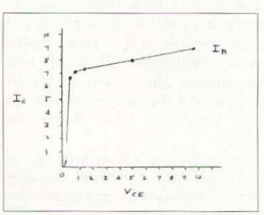
Fig. 1. Example of how several points are plotted to establish a base current curve. A minimum of three points are plotted to define the knee of the curve and two or more points to define the straight portion of the curve.
