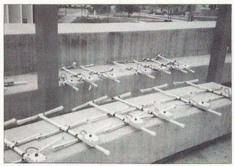
**Photo D.** Some of the completed steel-tape RDF beams with attenuator boxes mounted to the handles, ready for the hunt.
