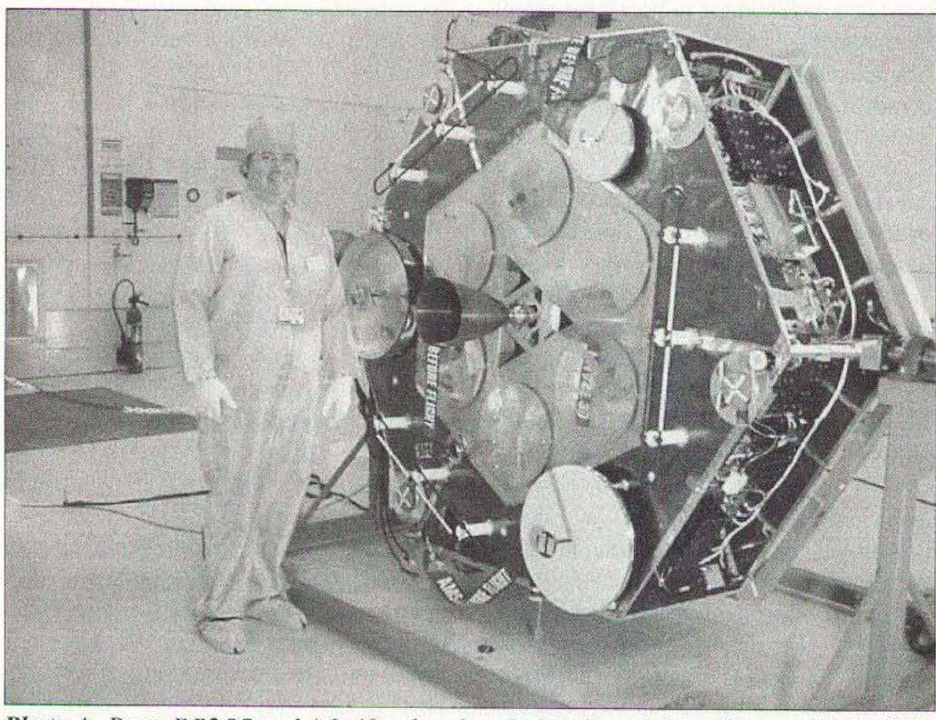
Photo A. Peter DB2OS and AO-40 a few days before launch from Kourou. Most of the antennas are on the same side of the satellite as the main motor. (AMSAT-DL photo)
