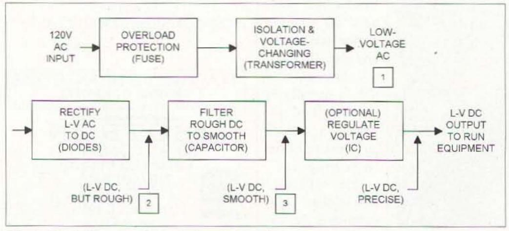
Fig. 1. Block diagram of a typical power supply. 14 73 Amateur Radio Today • August 2001
