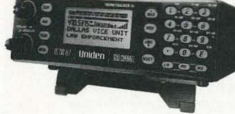
Bearcat® 780XLT Trunk Tracker III Mfg. suggested list price \$529.95 Less -\$190 Instant Rebate / Special \$339.95 500 Channels • 10 banks • CTCSS/DCS • S Meter Size: 75/8" Wide x 615/16" Deep x 213/16" High Frequency Coverage: 25.0000-512.0000 MHz., 806.000-823.9875MHz., 849.0125-868.9875 MHz., 894.0125-1300.000 MHz.
