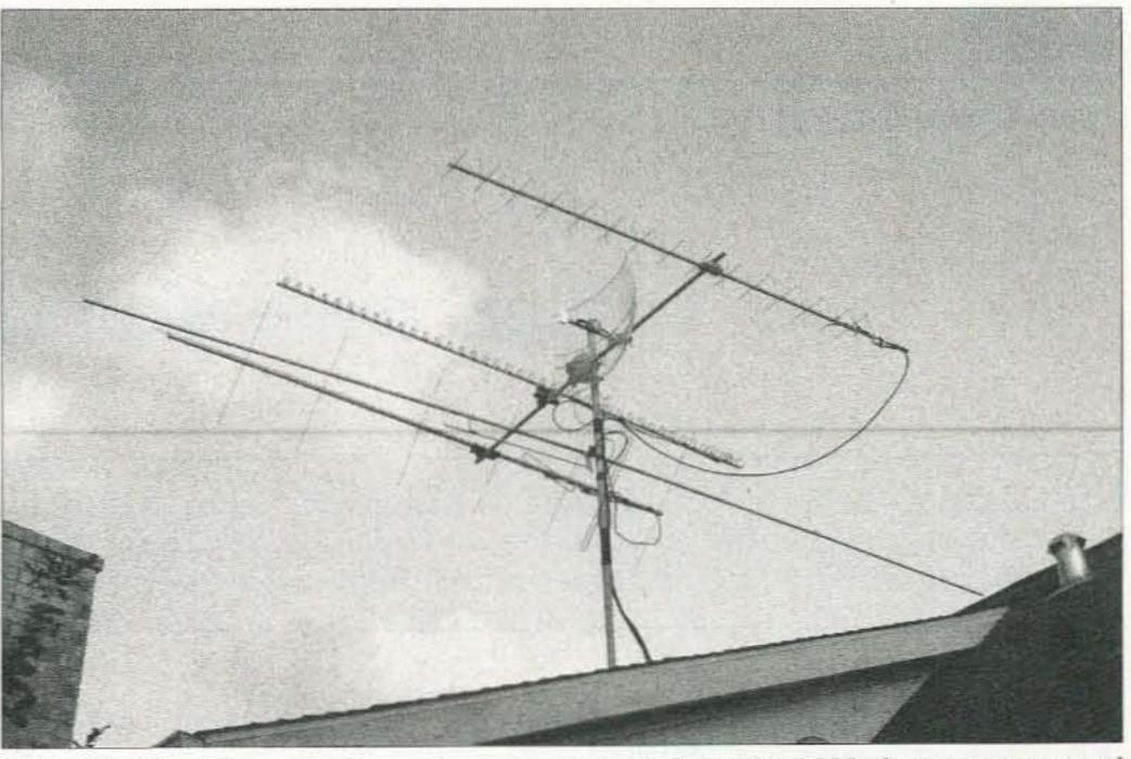
**Photo B.** The 13-cm receive system, complete with Drake 2880 downconverter and "BBQ-grill" reflector, fits easily in this ground-station array which includes antennas for two meters, 70 cm, 23 cm, and even a dipole for 15 meters.
