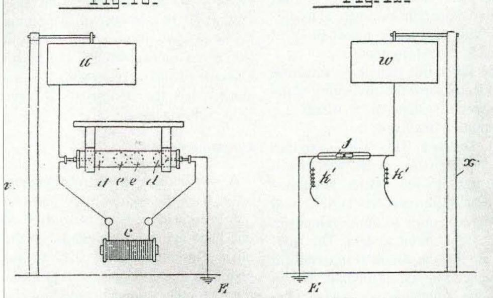
To one skilled in the art a transmitting station is shown at fig. 10, having a Morse key and battery in the primary circuit, not shown, of an induction or Ruhmkorff coil c or other source of high tension, high frequency current. A spark gap d, e, e, d, in the secondary circuit has one side grounded at Eand the other side connected to an elevated wire and plate uinsulated from the earth on the pole v.
