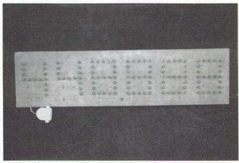
Photo C. Close-up front view of the display panel with a 6-in.-long, 25-wire data cable, and its terminating DB-25 male connector. 12 73 Amateur Radio Today • April 2002
