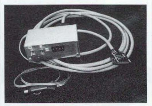
**Photo B.** A view of the control box with an 8-ft.-long 25-wire data cable. The cable is terminated with a DB-25 female connector. A 3-ft. power cable is also shown connected to the control box. This cable is terminated with a cigarette lighter plug.
