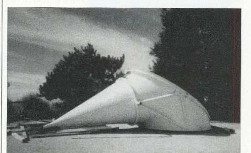
appeared to have served its time and had been relegated to the parking lot for storage (Photos D and E). Although I didn't measure the waveguide dimension, I did estimate the circular guide dimension to be three inches in diameter. It is my estimate that the antenna was designed to support signals in the 3-GHz band.
