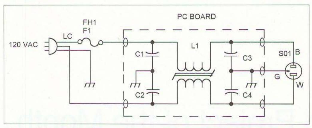
Fig. 1. 400-kHz AC Line Filter schematic.
