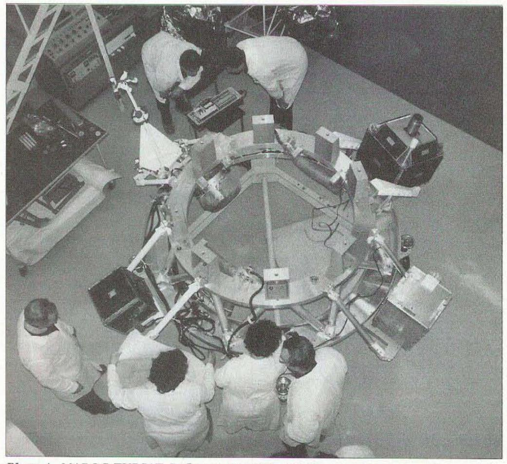
**Photo A.** MAROC-TUBSAT, Reflector, BADR 2, and Kompass are arranged around the periphery of the ZENIT-2 adapter ring prior to the December 10, 2001, launch from Kazakhstan. (TUB photo)
