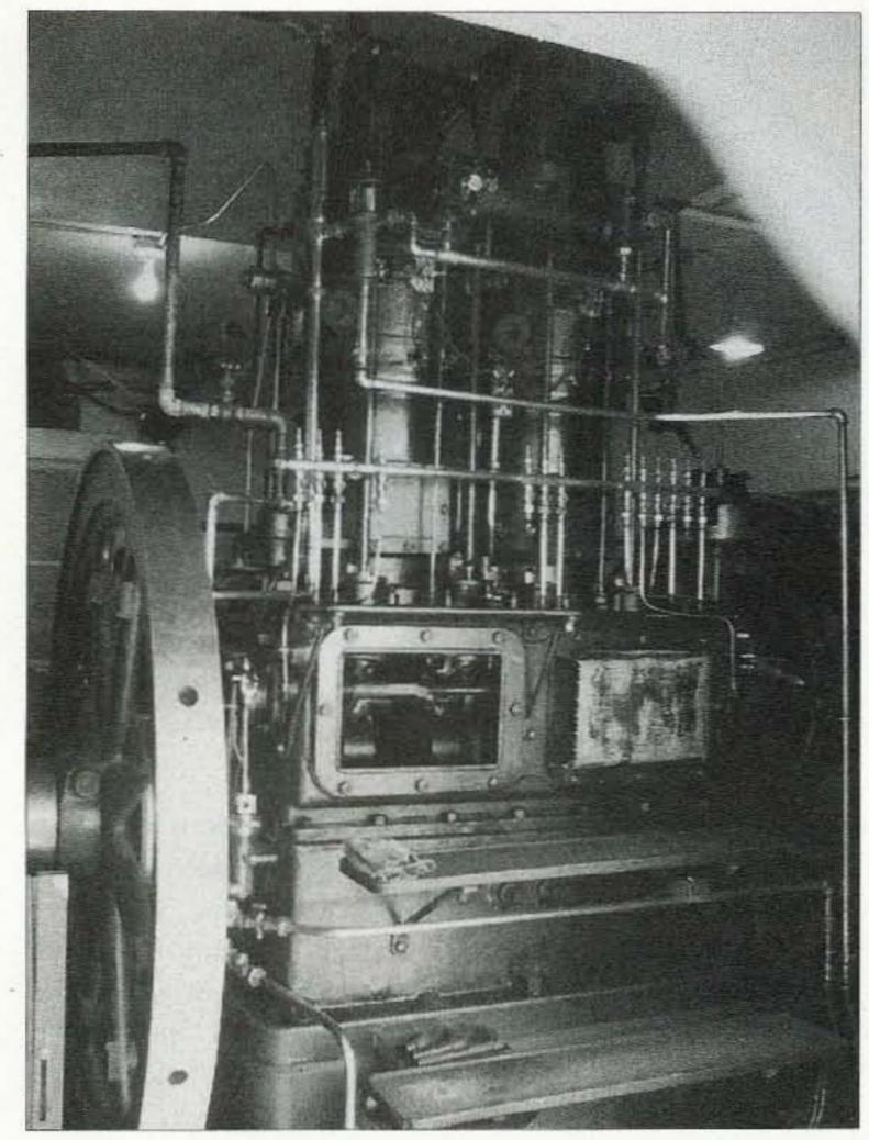
Photo K. 1912 Fairbanks-Morse 2-cylinder 50 HP engine formally used to drive a 40 kW 120 VDC generator. Most all of the
