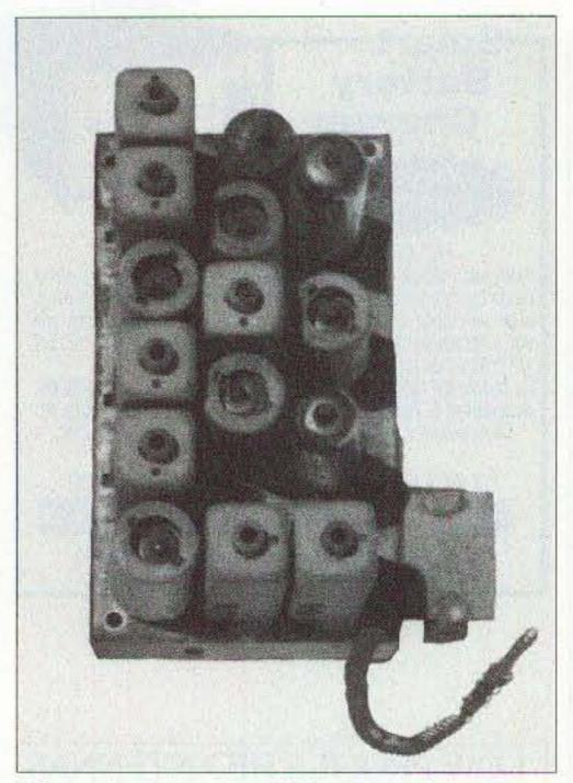
**Photo A.** Top side of the IF module showing the compact design. The audio output transformer is shown on the rear of the chassis.
