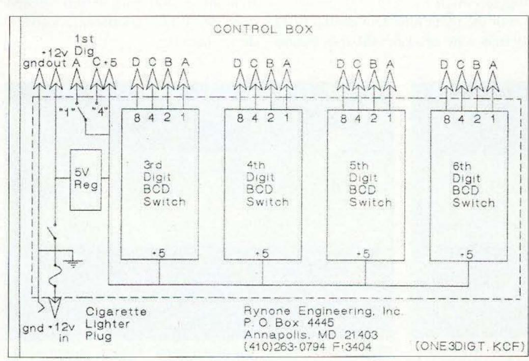
Fig. 2. Control box schematic.
