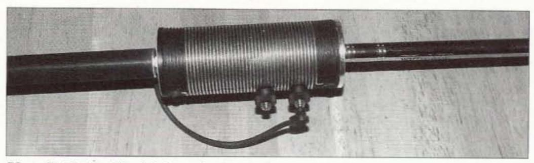
Photo D. The Buddipole's large loading coil.
