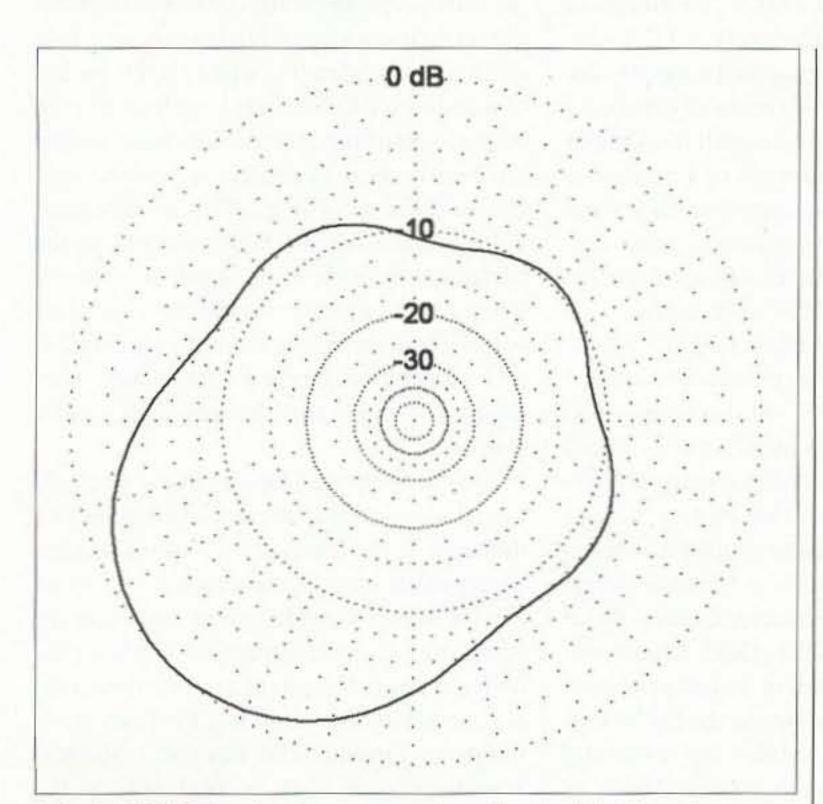
Fig. 2. ELNEC azimuth pattern plot of a 4-whip Doppler array with three whips grounded and one connected to the feedline. The large lobe is in the direction of the active whip, which is in the lower left of the array.
