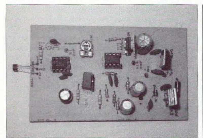
Photo H. Top side view of the clamp-on DC ammeter's evaluation circuit board.
