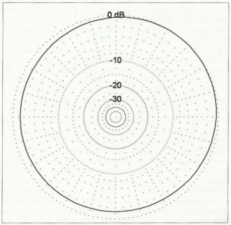
Fig. 3. The undesirable lobe disappears and a nearly perfect circular pattern with no phase anomalies is achieved when the switched-off whips are open-circuited to minimize parasitic effects.
