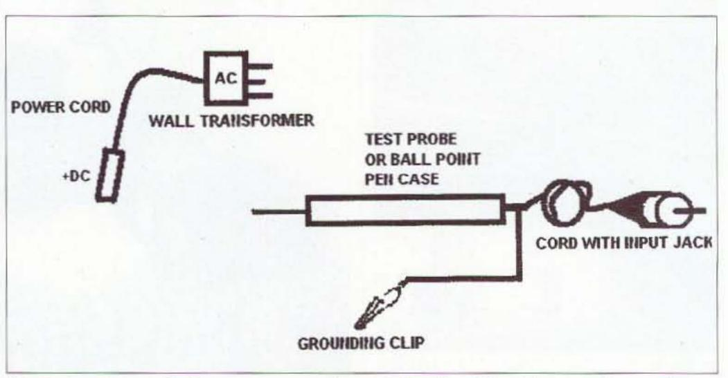
Fig. 2. Attachments, DC power source and modified audio cable with test probe attachment.
