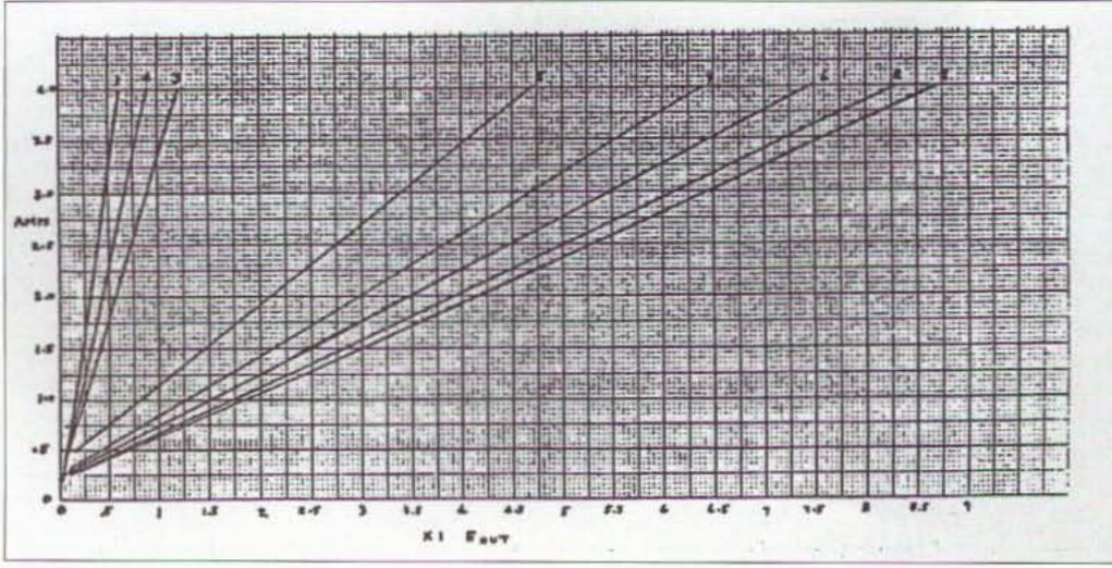
**Fig. 1.** Each of the available cores was evaluated for response with the results shown. Slopes to the left indicate the lowest response and the highest (greatest) response to the right. From left to right, core numbers are 1, 4, 3, 5, 7, 6, 2, and 8.
