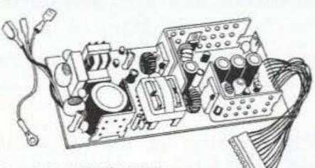
Lambda # PWG0079D. Input: 100-240 VAC @ 2 Amp. Output: 5 Vdc 7 A, 3.3 Vdc 15 A. Openframe switching power supply. 8" x 3.5" x 1.25" high. Prepped with 4" leads on input and 6" leads on output with a 12 pin female socket connector (0.156" spacing). UL, CSA.
