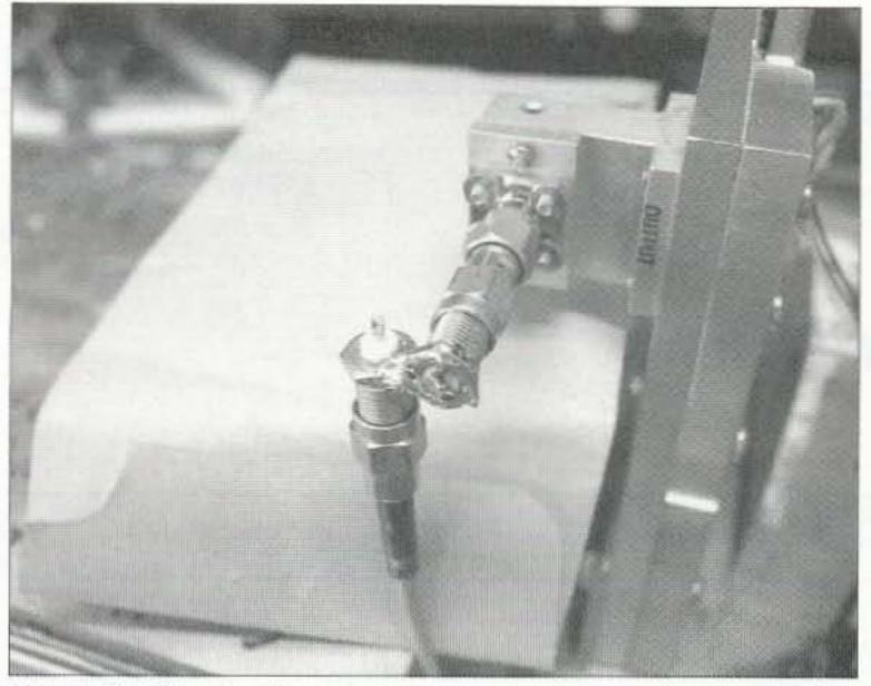
**Photo C.** Close-in shot of system mixer showing fly spec diodes and IF cable (145 MHz) and SMA connector pointing downward in this test configuration.
