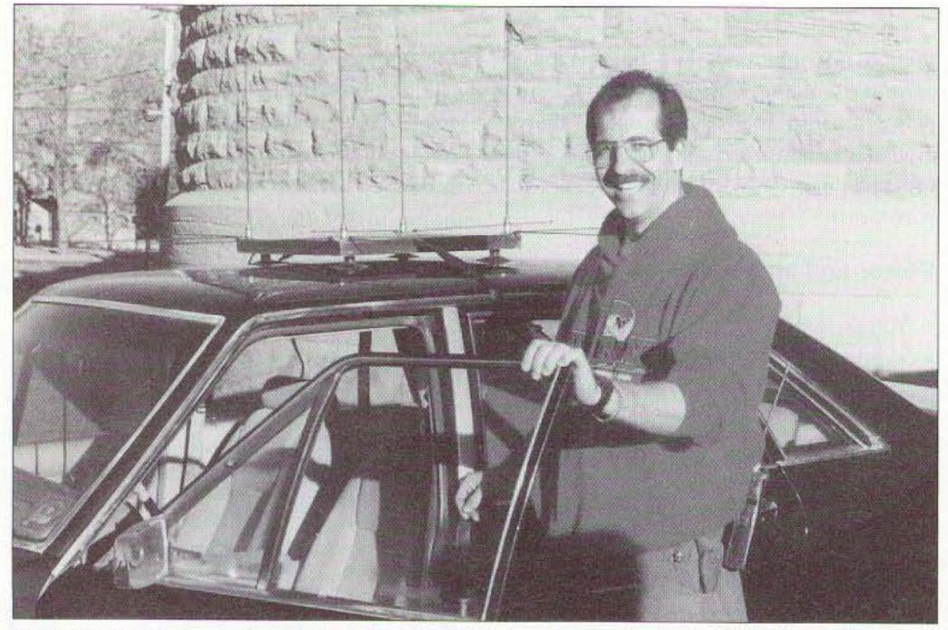
**Photo A.** Many Doppler builders choose a one-band antenna array like this one for two-meters used by Louis Tremblay VA2JX of Montreal. It has four quarter-wavelength whips in an 18-inch square pattern on a metal plate, plus eight radials to provide a symmetrical ground plane under each whip. The one-piece assembly mounts quickly and the whips are always perfectly spaced and aligned. (KØOV)
