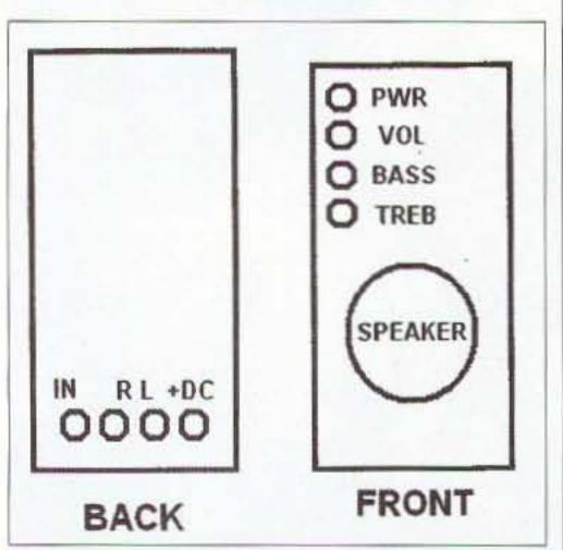
Fig. 1. Typical computer speaker pair. Inside is an audio amplifier.
