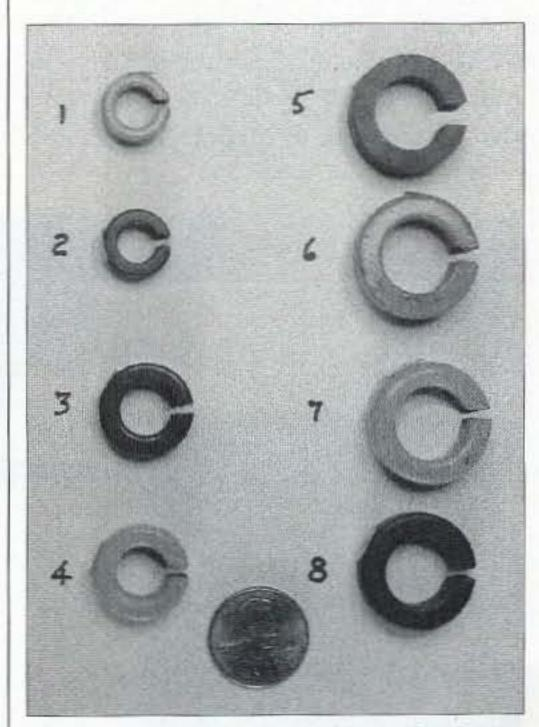
Photo E. Shown are eight randomly selected cores that were evaluated for use in the clamp-on DC ammeter project. A penny is shown for size comparison.
