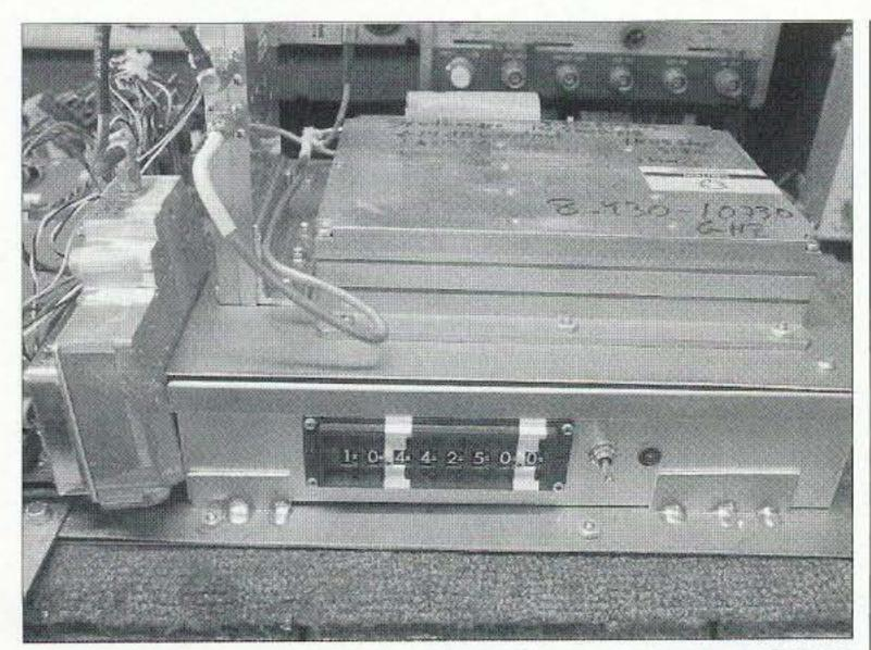
**Photo A.** Front view of synth top right, sitting on top of BCD controller chassis. Synth capable of operation from 8930 to 10730 MHz with +14 dBm output. Frequency steps as fine as 1 kHz throughout its frequency range set by BCD switches on control panel. Close in phase noise better than -90 dB.
