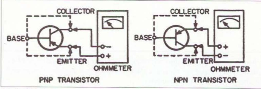
**Fig. 3.** With ohmmeter in R x 100 scale (assuming that the meter uses a 1-1/2 volt battery), a good transistor will be indicated by a decrease in resistance when the base lead is touched to the collector and a small increase in resistance when the base lead is touched to the emitter.
