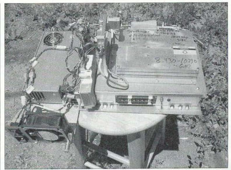
**Photo B.** Top view of total system main synth to right, 2640 MHz synth bottom left in aluminum cutout shield compartment. Pecom TX module just above 2640 MHz synth. Switching regulated power supply to far left with cooling fan in front of power supply.
