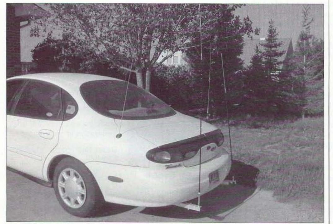
Photo A. Fashion experts say that the multiple antenna look is "in" this year. Besides the 2-meter/440-MHz antennas glass-mounted and on the trunk, there's an Iron Horse 6-meter antenna on the right and a matching 20-meter antenna on the left.
