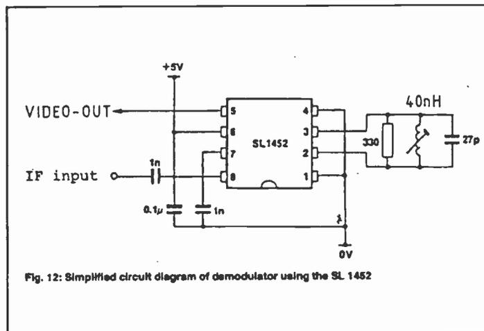
Fig. 12: Simplified circuit diagram of demodulator using the SL 1452
