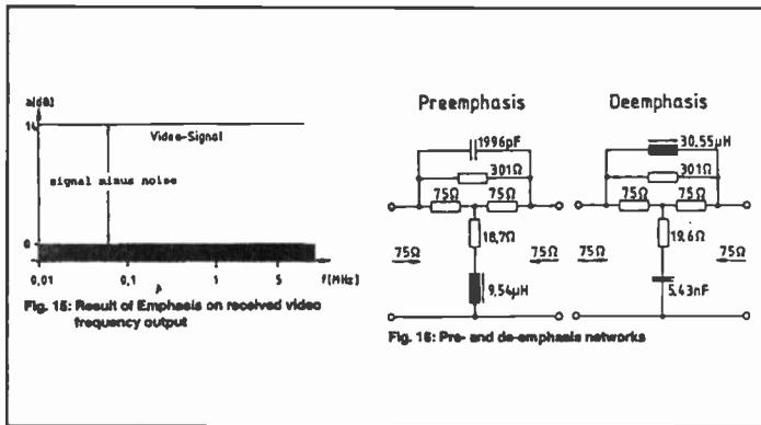
Fig. 15: Result of Emphasis on received video frequency output
