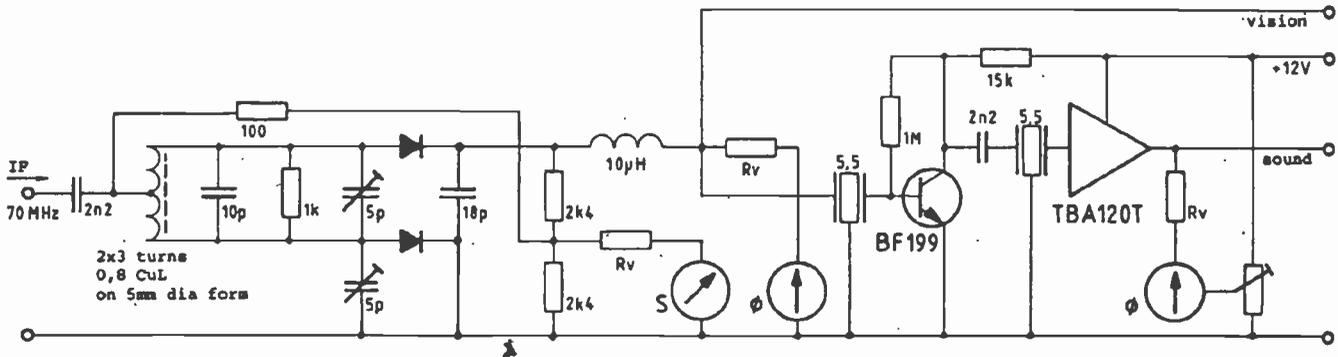
**Fig. 10: FM TV diode discriminator showing vision and sound demodulators**
