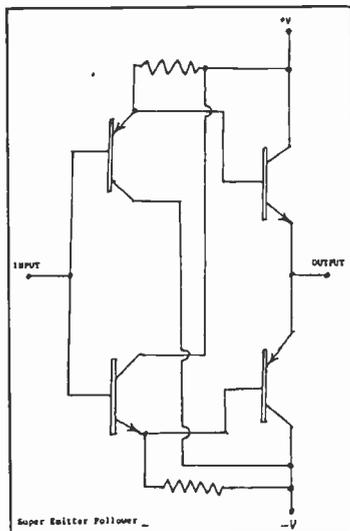
drive transistor cancel out the .7 of the output transistor so that the input bases can be tied together. See diagram. This circuit has the additional advantage of having a very high input impedance due to darlington connection. This allows DC restoration at the input with very little leakage. A driven clamp can work quite well clamping to the back porch.
