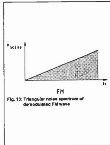
Fig. 13: Triangular noise spectrum of demodulated FM wave
