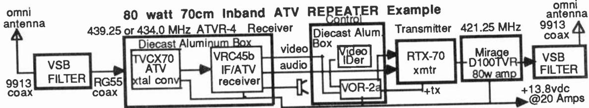
Select an RTX Transmitter and a ATVR Receiver for the bands you want, add the appropriate linear amp, VSB filters & antennas, ID & VOR-2a, power supply and coax for your own repeater. We suggest low in / high out for crossband. Ask for a copy of our ATV Repeater article before you start so you will do it right the first time. Also listed are recommended sources of filters, antennas, IDers, etc. Most can put together a good working ATV repeater for under \$2000.
