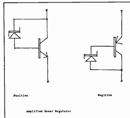
Either polarity of transistor can be used depending on your needs. Another advantage is that if you need tight regulation from a Zener this circuit can reduce the current change in the Zener by the beta of the transistor used.
