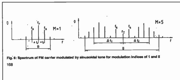
Fig. 6: Spectrum of FM carrier modulated by sinusoidal tone for modulation indices of 1 and 5
