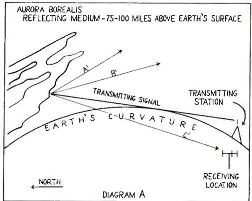
**AURORA REFLECTION . . .** The transmitted signal reflects from the rapidly oscillating Aurora surfaces (to the north) and back towards the south, providing reception close to the origination point, as well as over distances of 200-1,000 miles. C1 indicates a returned signal. A1 and B1 reflect off the Aurora into space.
