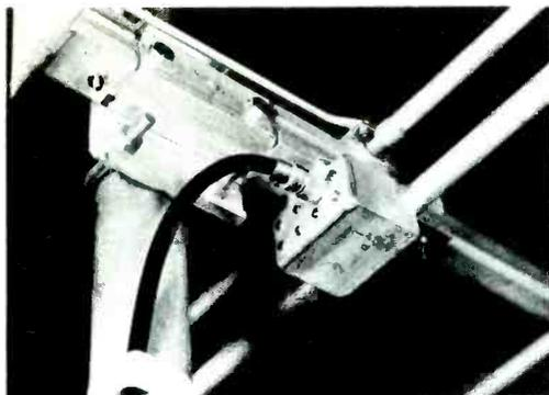
This close-up of connector and antenna termination illustrates the construction of the antenna and housing. To protect the balance and connector from moisture, the housing is foam-filled after all connections have been completed.
