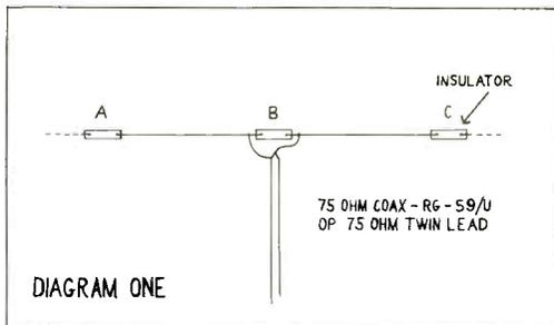
The single wire dipole, fed with 75 ohm coaxial cable, or 75 ohm twin lead. Distance A to C (minus the length of the insulator at B) is one-half wave length. Insulators at A, B and C are E. F. Johnson 104's, or a unit equally suitable.
