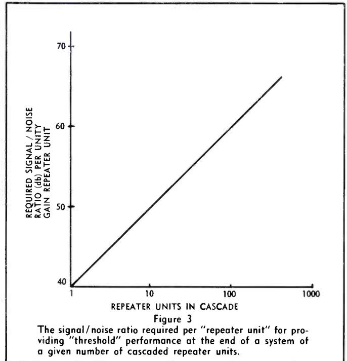
Based on the foregoing, Figs. 3 and 4 are rather interesting as they show the noise and intermodulation specifications respectively required at each repeater unit to give threshold performance over a system of X number cascaded units. As we have already seen, a "per unit" signal-to-noise ratio of 60dB would result in the noise being at the 40dB threshold after 100 units, while for a similar inter-
