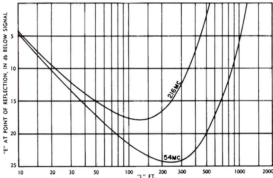
Figure 1. Minimum permissible return loss in RG 11/U coaxial cable as a function of the distance between point of observation and source of echo.
