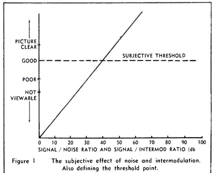
Figure 1 The subjective effect of noise and intermodulation. Also defining the threshold point.
