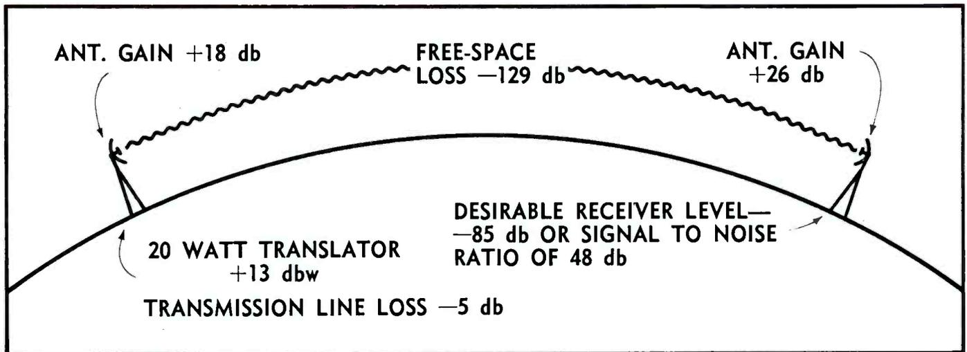
about 450 microvolts across 50 ohms or 1100 microvolts across 300 ohms. This is in agreement with practical experience with preamplifiers of this type. Desirable preamplifier signal is thus set at  $-85$  dbw.
