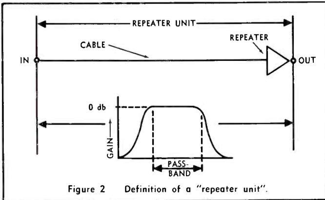
Figure 2 Definition of a "repeater unit".
